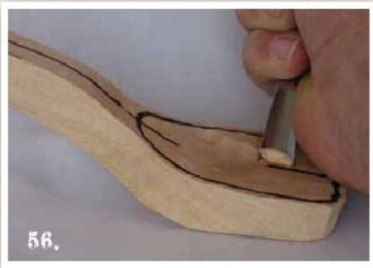
I grip the gouge as shown, with just a little bit of the sharp end protruding past my hand. Then I put the heel of the tool holding hand on the work piece and just rotate my wrist to make the cut as shown. If just a little bit of the tool protrudes past my hand and the heel of the hand is kept in contact with the work, this is a very safe way to cut. Little cuts only! Do not strain. Straining leads to slips. We don't want those!
