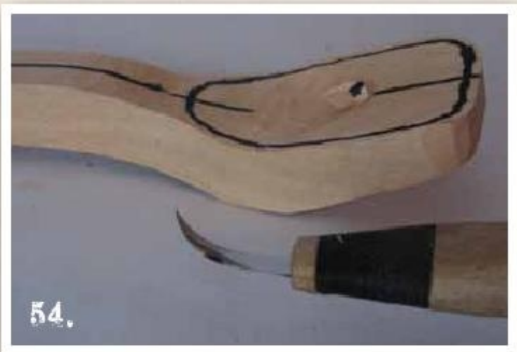
I use a bent knife for this work on occasion, and it works fairly well. Some spoon makers prefer them.
