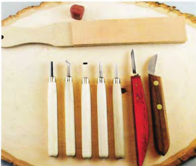
Basic beginner's carving kit from left: V-gouge, skew chisel, straight chisel, large round gouge, medium round gouge, bench knife, and a large chip carving knife. At top: leather strop and stropping compound.
