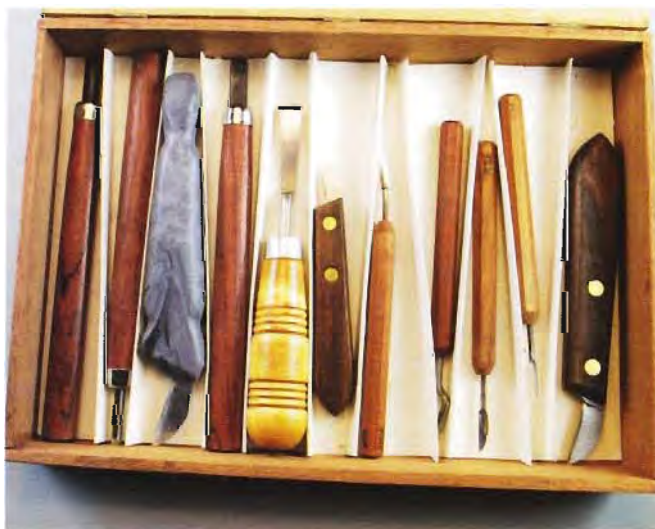
Storage. This simple knife storage box is made from a wooden craft box. The bottom of the box has been lined with tag board that has been folded to create individual storage spaces.
