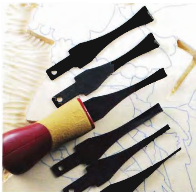
Gouges. Top to bottom: flat wide-sweep gouge, medium wide-sweep gouge, small wide-sweep gouge, large U-gouge, medium U-gouge, and small U-gouge (also called a veining tool).
