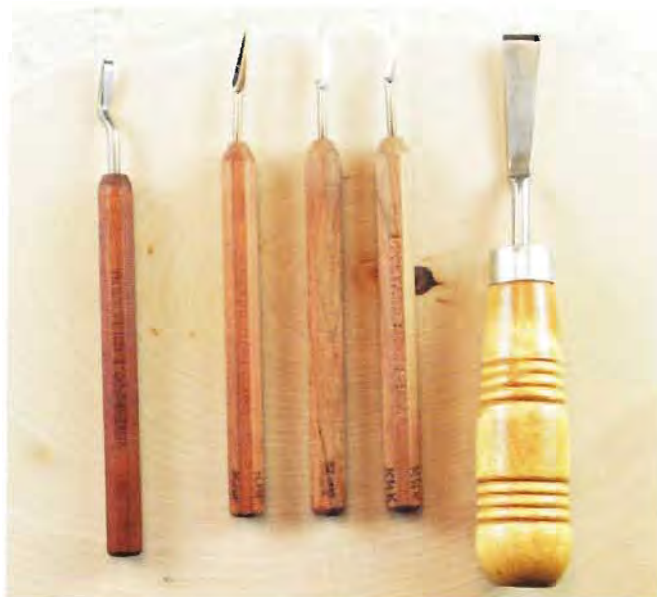
Tool kit expansion. Left to right: dogleg chisel, skew detail knife, straight detail knife, curved detail knife, and large dogleg chisel.
