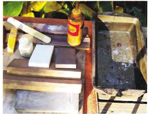
Keep carving tools sharp. A sharpening kit includes stones of various grits, emery cloth, leather or synthetic strops, and honing/roughing compounds.
