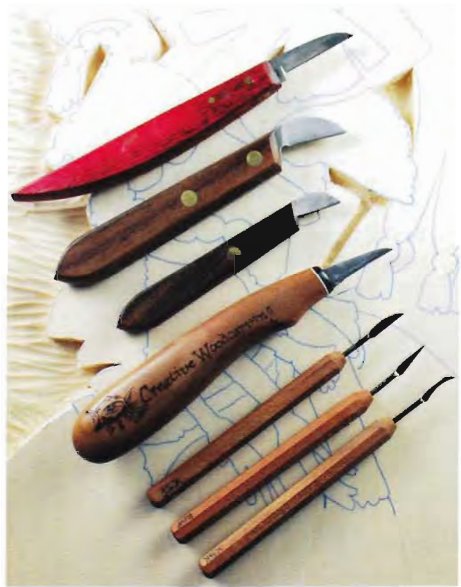
Knives. Top to bottom: bench knife, large chip carving knife, small chip carving knife, whittling knife, straight detail knife, fine point detail knife, and concave detail knife.
