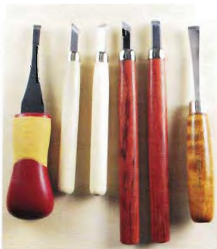
Chisels. Left to right: palm handle interchangeable straight chisel, Japanese skew and straight chisel, rosewood long handle skew and bull-nose chisel, and bent-shaft bull-nose chisel.
