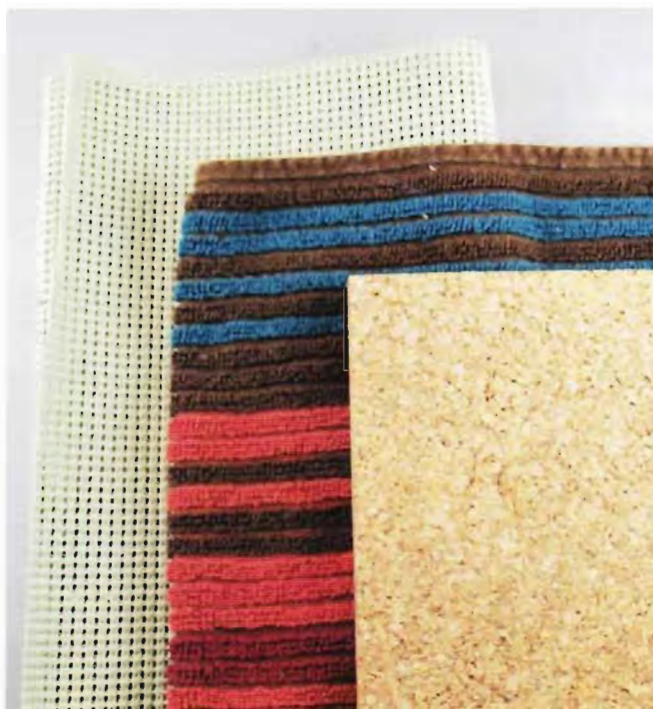
Keeping wood in place. Non-skid mats, heavy terrycloth towels, and even corkboard squares hold the carving wood to the work surface.
