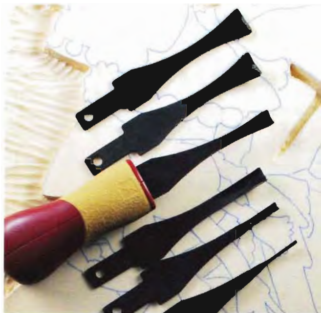
Gouges. Top to bottom: flat wide-sweep gouge, medium wide-sweep gouge, small wide-sweep gouge, large U-gouge, medium U-gouge, and small U-gouge (also called a veining tool).
