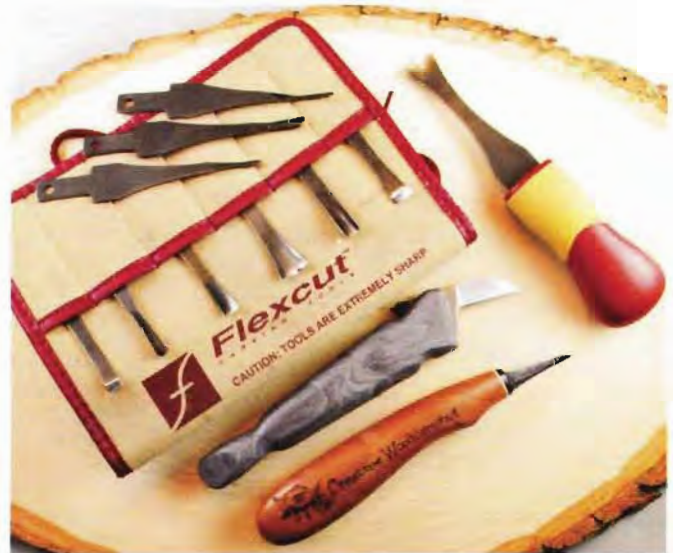
Advanced beginner's carving kit. Interchangeable tool tip set: tight, medium, and large U-gouges; veining tool; V-gouge; straight chisel; wide, medium, and small sweep gouges; round gouge; chip carving knife; detail and bench knives; leather strop (not shown); and rouging compound (not shown).
