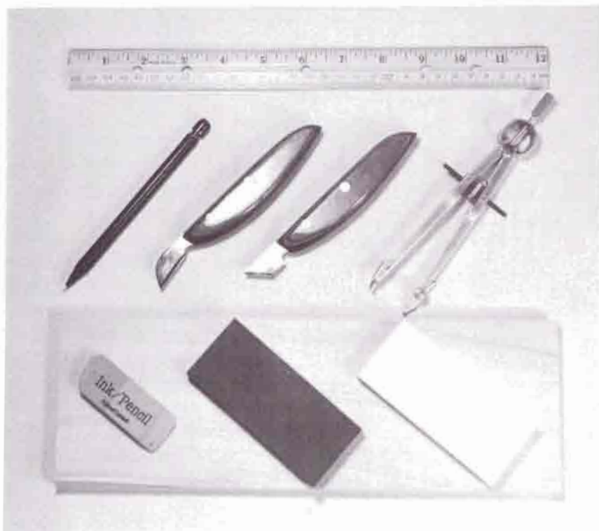
1-2 The tools needed for chip carving: ruler, pencil, cutting and stab chip-carving knives, draftsman's compass, eraser, and ceramic sharpening and polishing stones.
