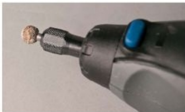
\frac{1}{4} " (6mm) round red Typhoon bit, properly seated deep in the tool shaft.
