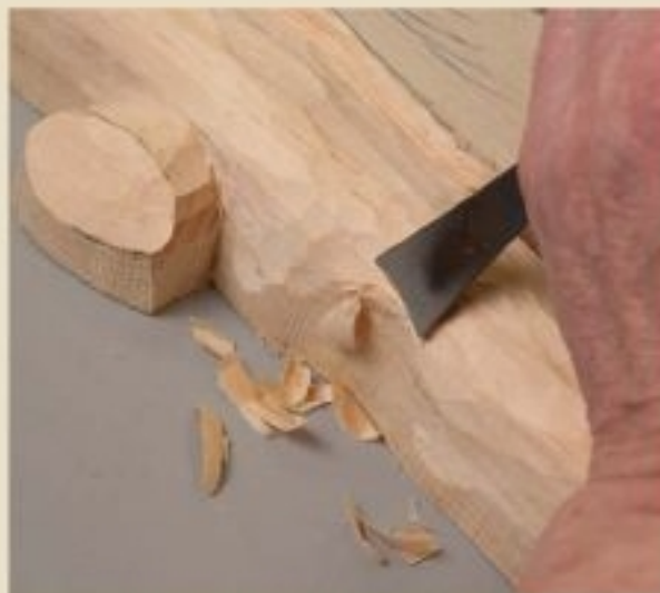
Come at it from a right angle to the original cuts.
