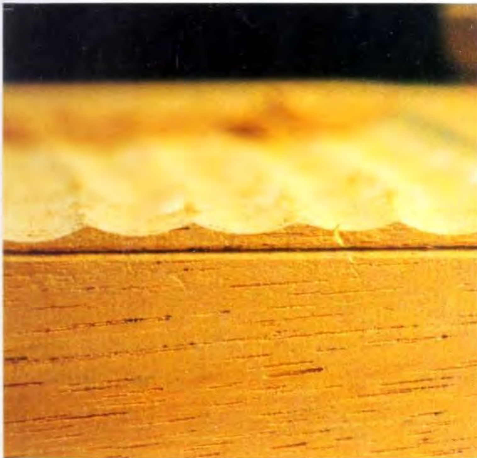
Fig 8.13 Magnified view of the line made by the marking gauge (which represents the final level of the ground) and the channels from the lowering stage. Note the consistency of depth. Levelling off will be quick, as you will need only to remove the small amount of waste down to the line.
