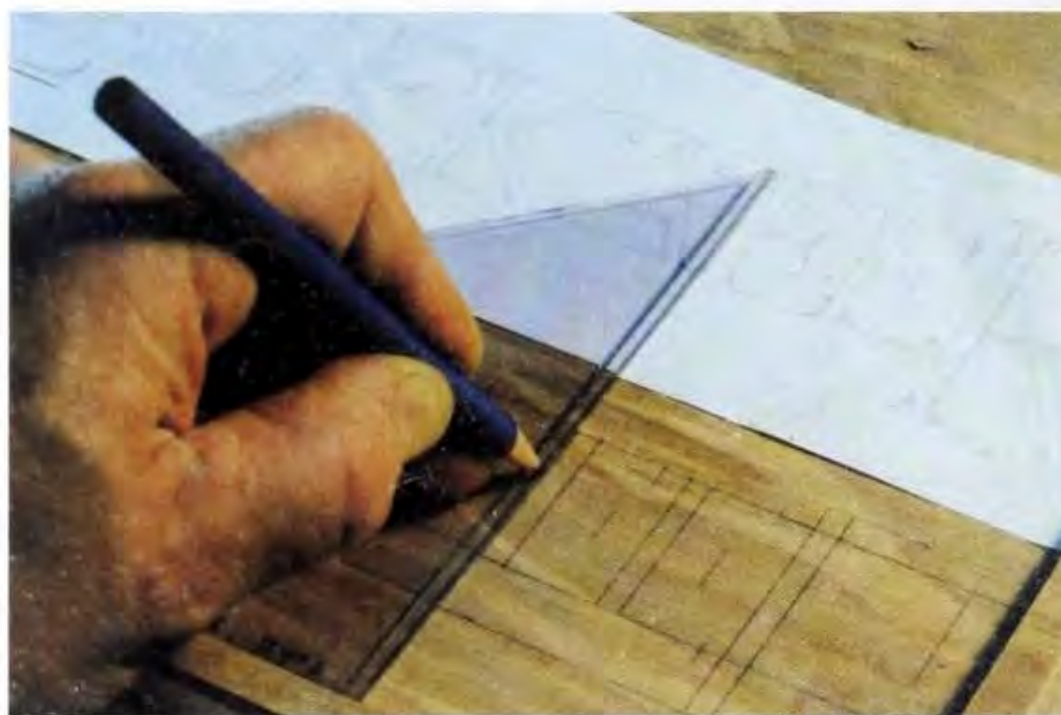
Fig 11.24 Setting out on to the wood.
