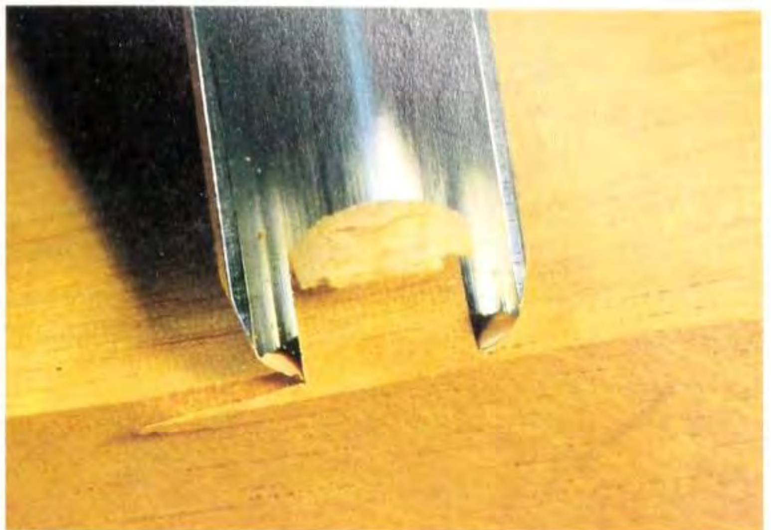
Fig 8.10 Unsupported wood is torn out as the gouge exits the far side. Always work into supported wood.
