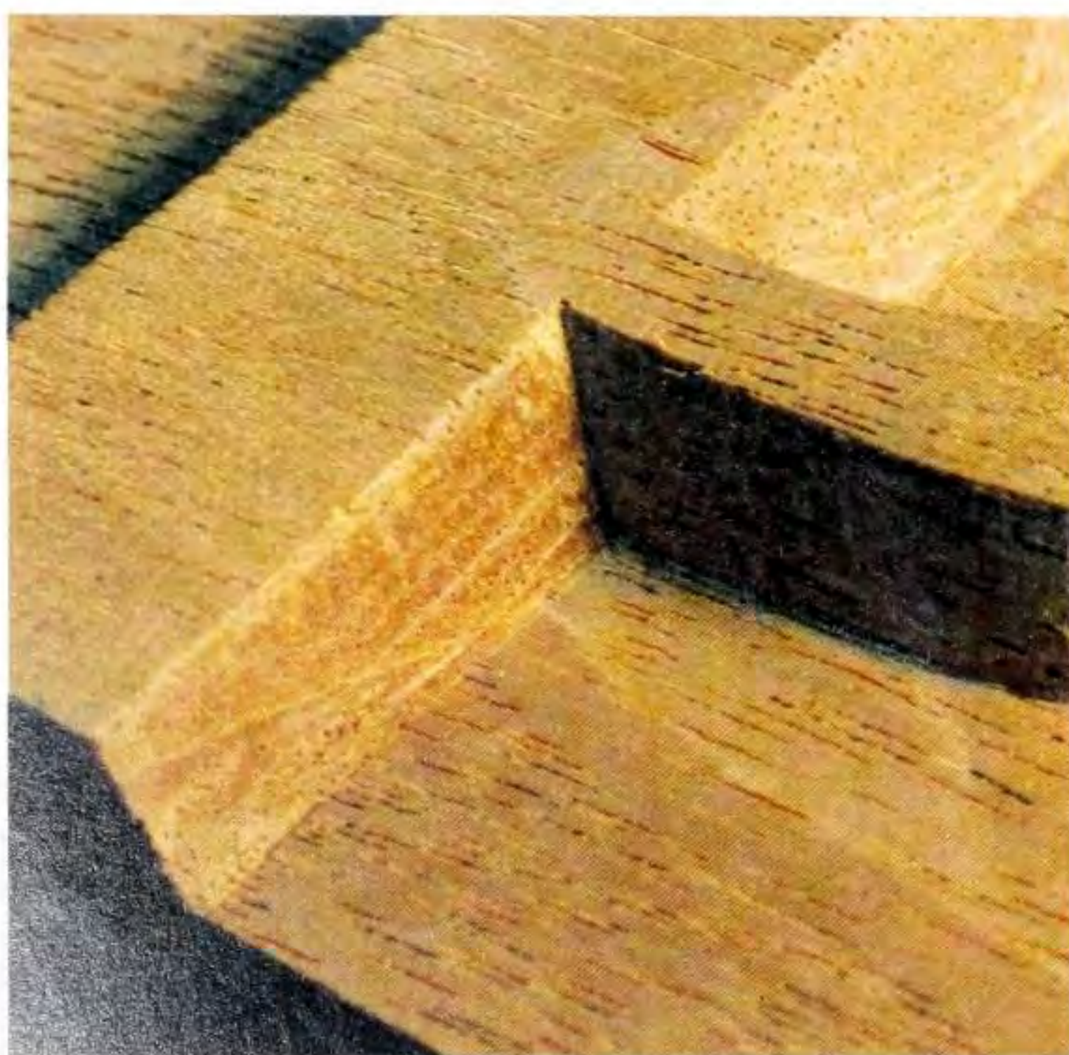
Fig 7.13 Try to get the junctions of side walls and ground as neat and clean as possible, without stab marks.
