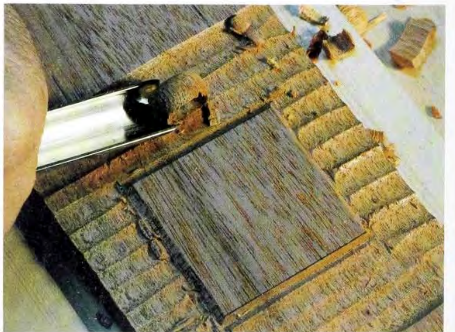
Fig 8.20 Lowering the ground with the deep gouge.
