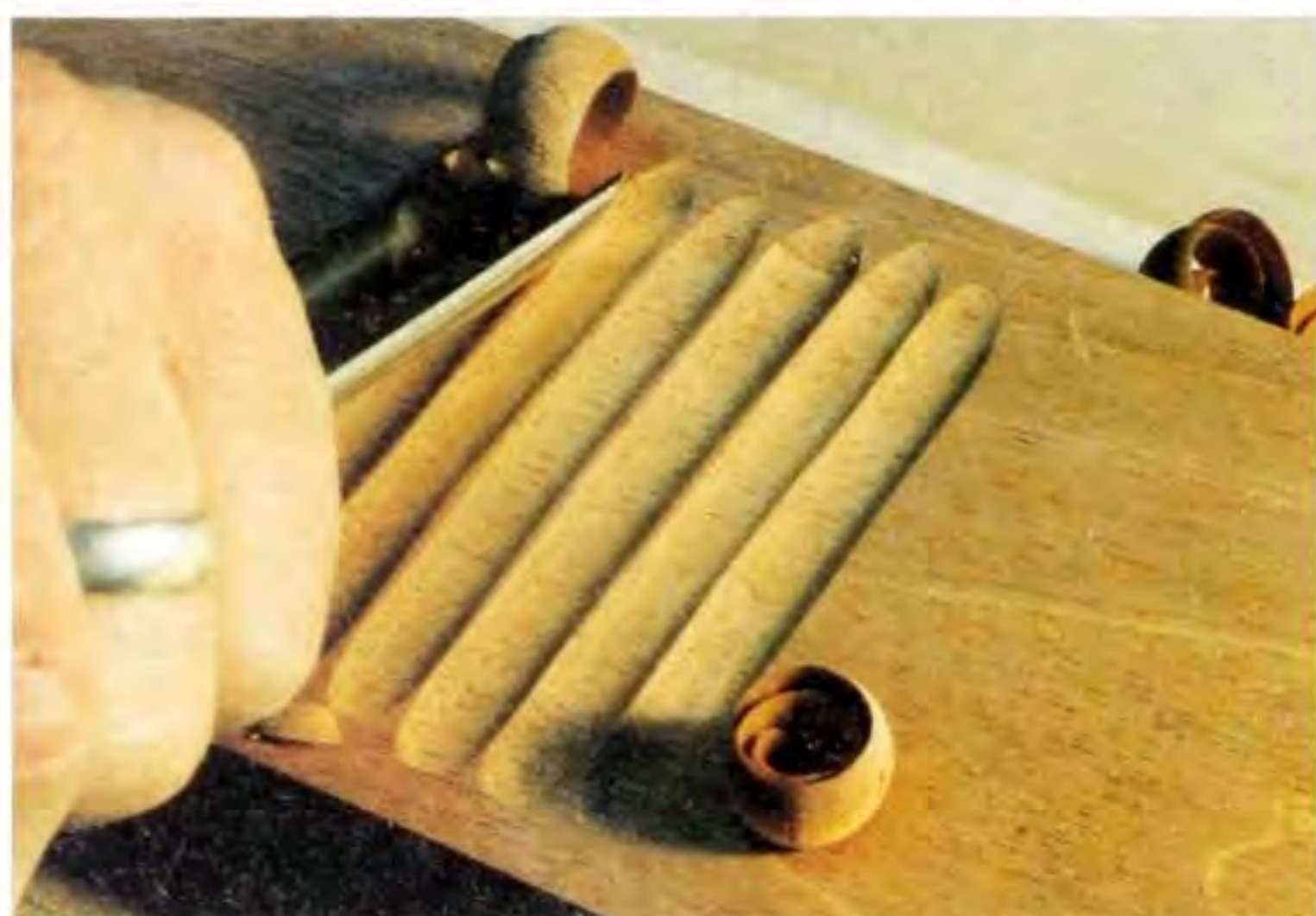
Fig 8.6 Making a series of parallel channels. This consistent way of working is the most efficient, and quickly gives a uniformly lowered ground.
