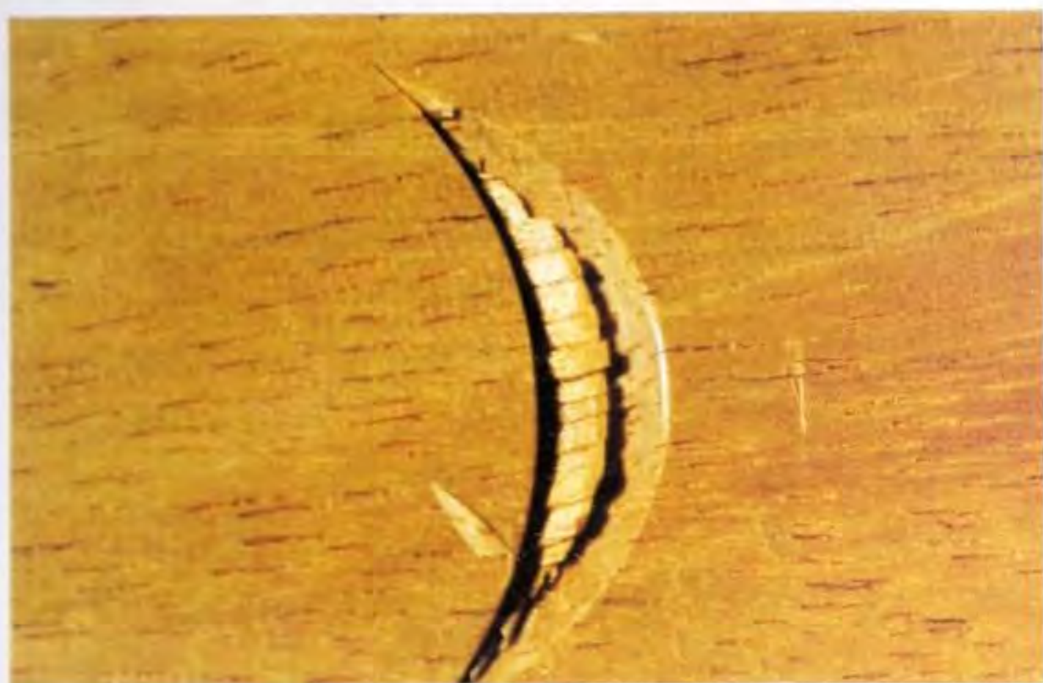
Fig 5.83 The angled cut cannot meet both the centre root of the crescent and the corners at the same time, so waste is left in the middle, which will have to be cleaned up by hand.
