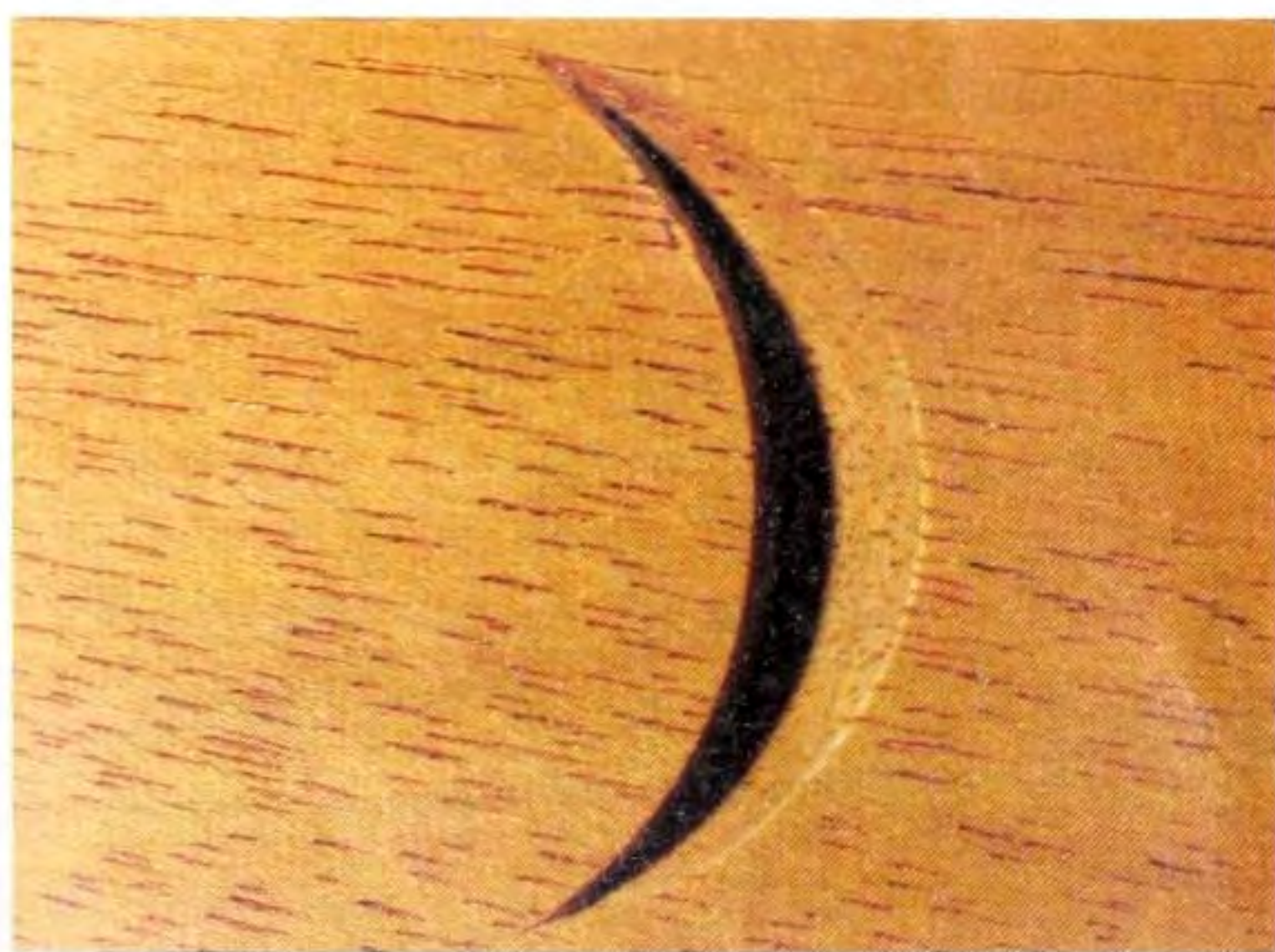
Fig 5.85 Close-up of cleaning the crescent root, starting by deepening the vertical wall. You can see that it is the corner of the tool which does the work, producing a clean crescent with a vertical inner wall, like that shown here.
