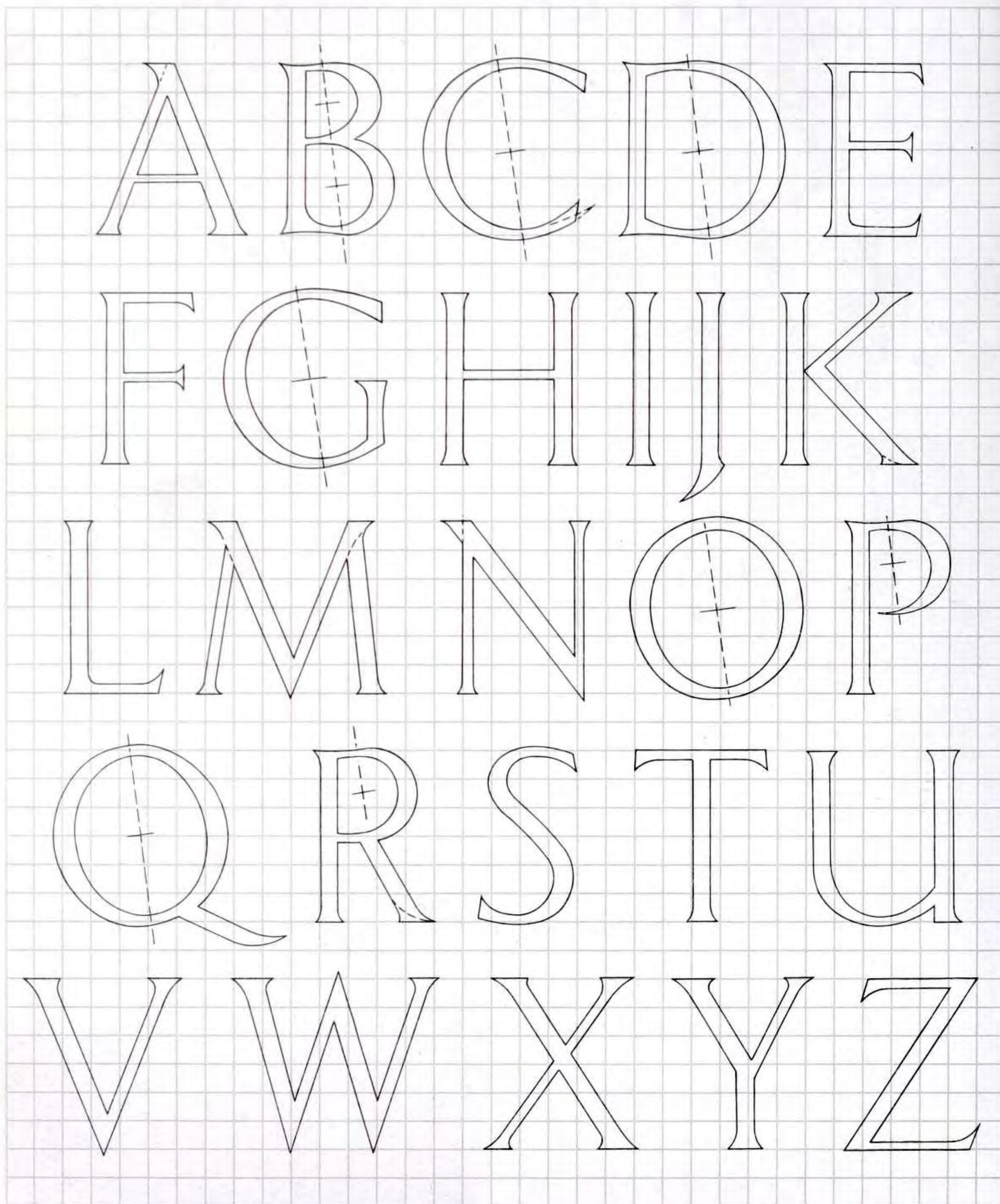
Fig 10.2 The Trajan roman alphabet. Waisting and curving of elements are not included for ease of carving in wood.
