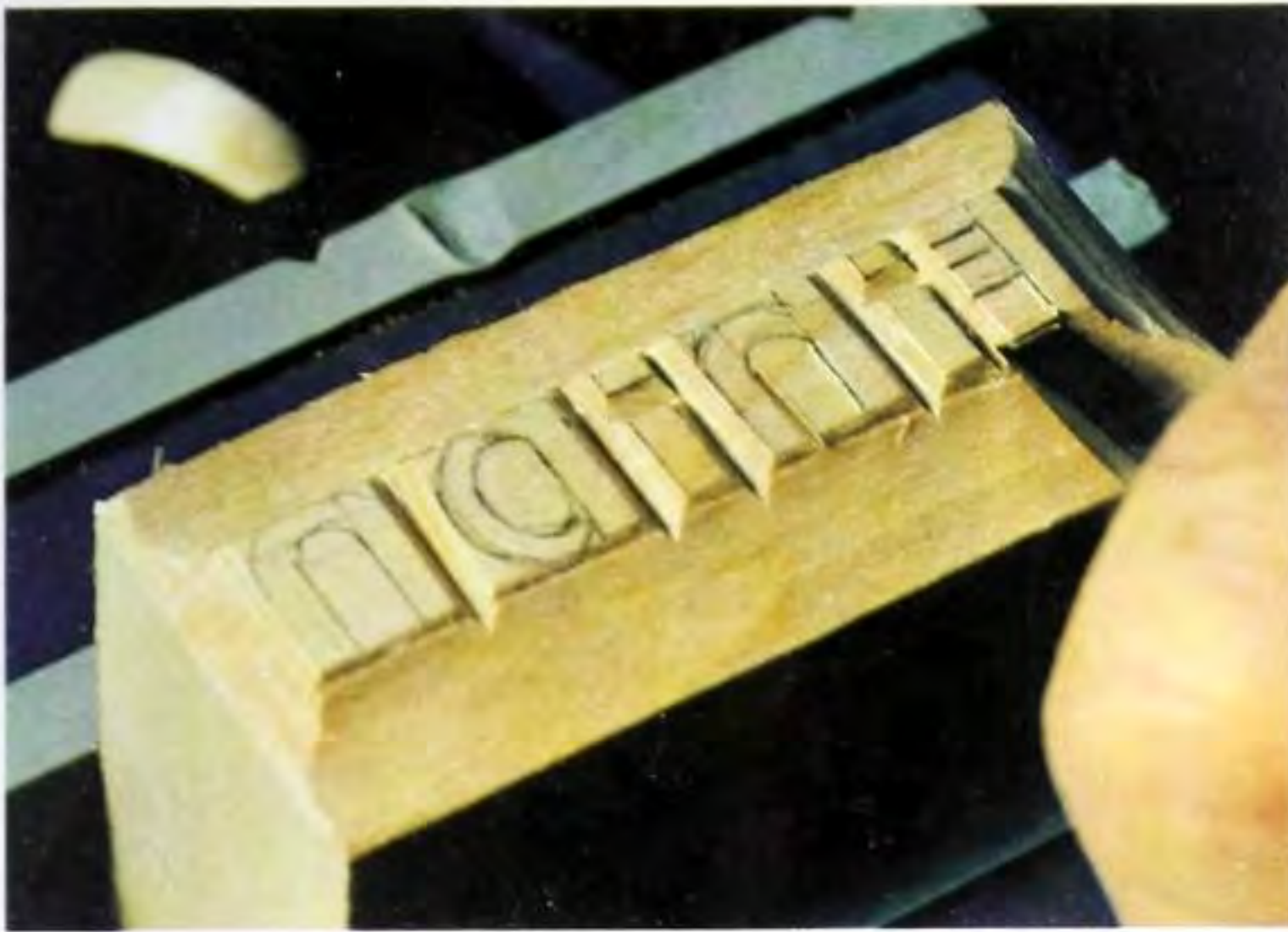
Fig 12.25 Removing the square counters. A stop cut on the insides of the legs prevents the grain breaking out.
