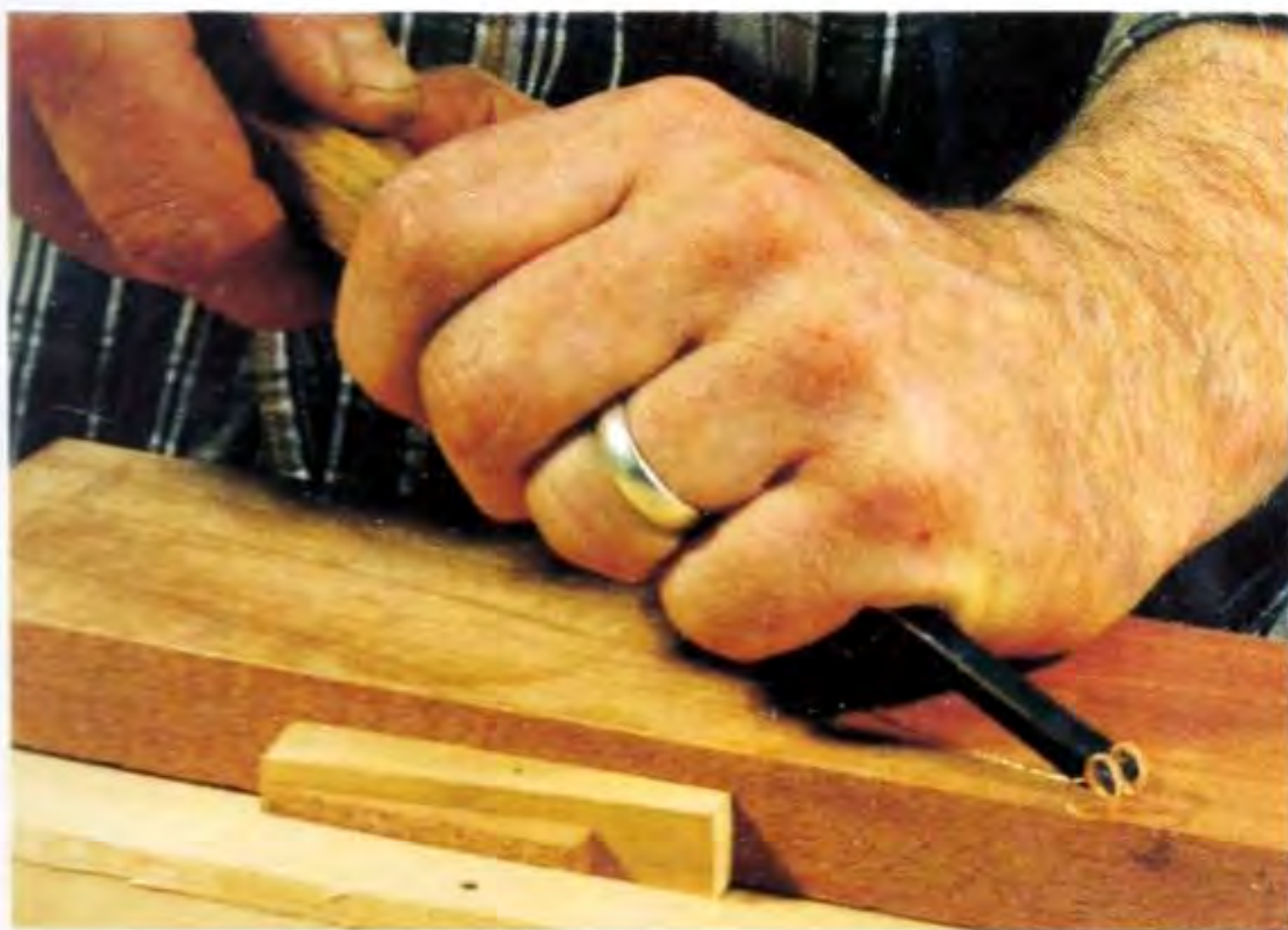
Fig 5.118 Running grooves with the V tool. Both hands work together to control and manipulate the cut.
