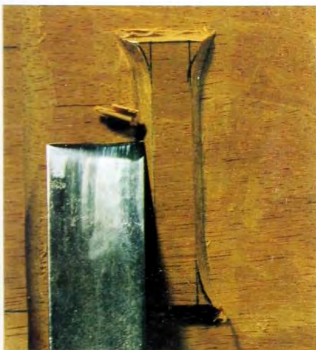
Fig 8.46 Levelling the ground, using the wall as a fence.
