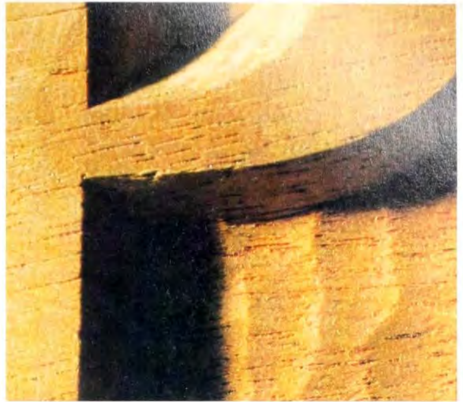
Fig 7.15 The background in Fig 7.13 (page 116) was created using a flat gouge. Here, the same area has been lightly textured using a deeper gouge.
