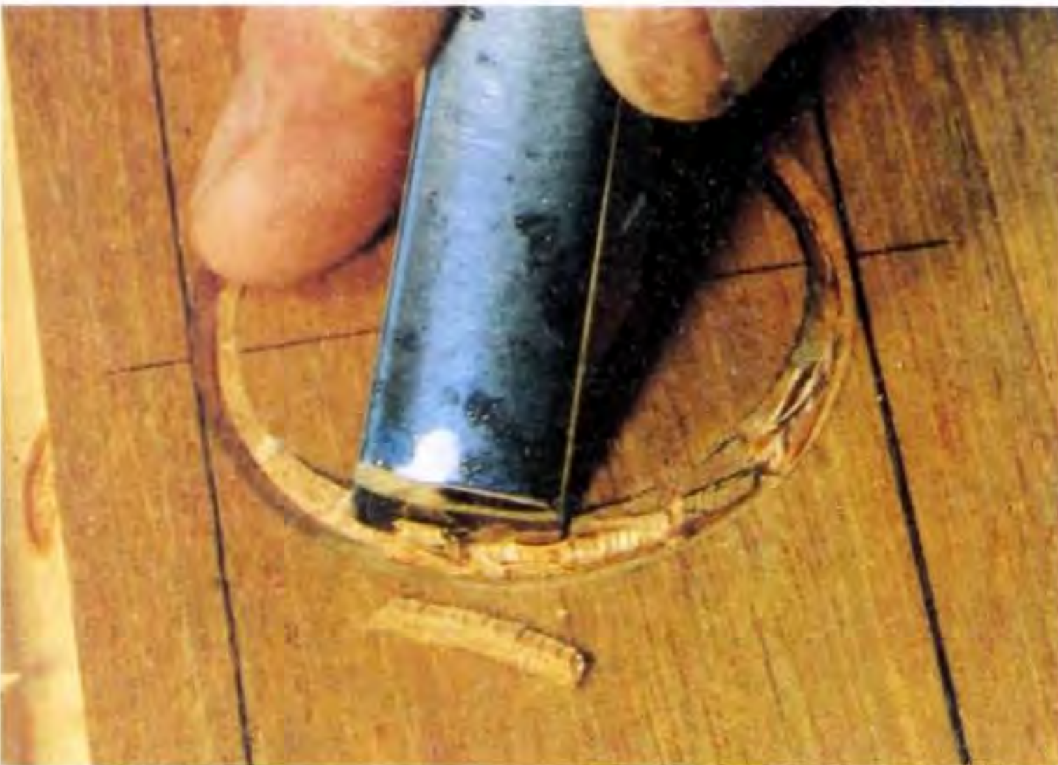
Fig 5.94 Then swap to a flatter gouge for the middle section.
