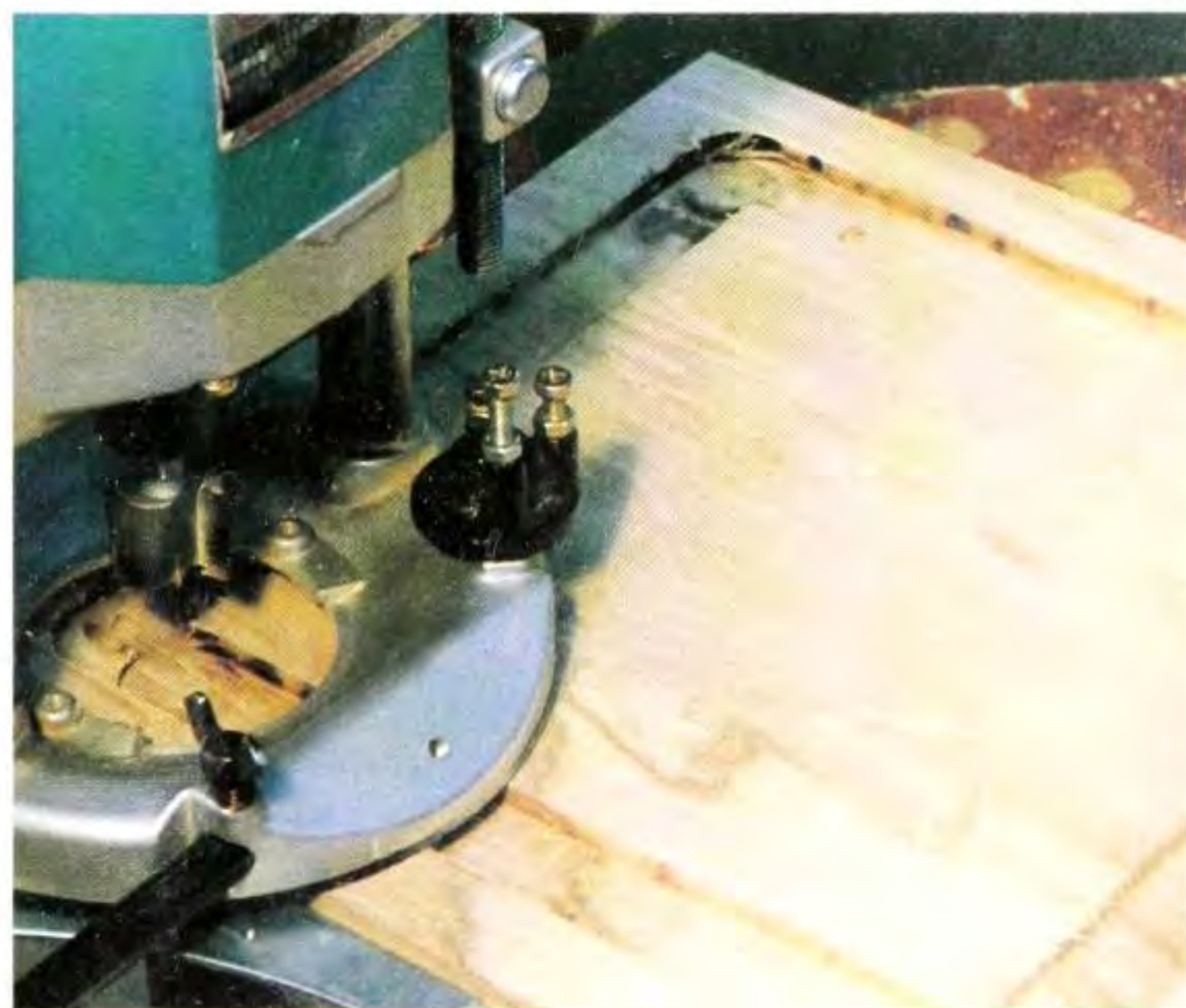
Fig 11.21 Routing the recess for the glass. After removing the waste wood the surface was carefully flattened with a scraper.
