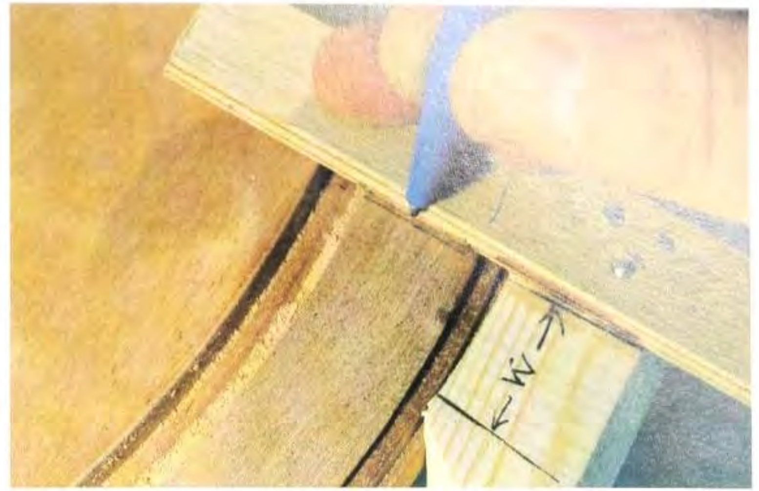
Fig 12.12 The jig I used to make the upright lines along the radii. You can see that the letters were designed to taper a little towards the cap line.
