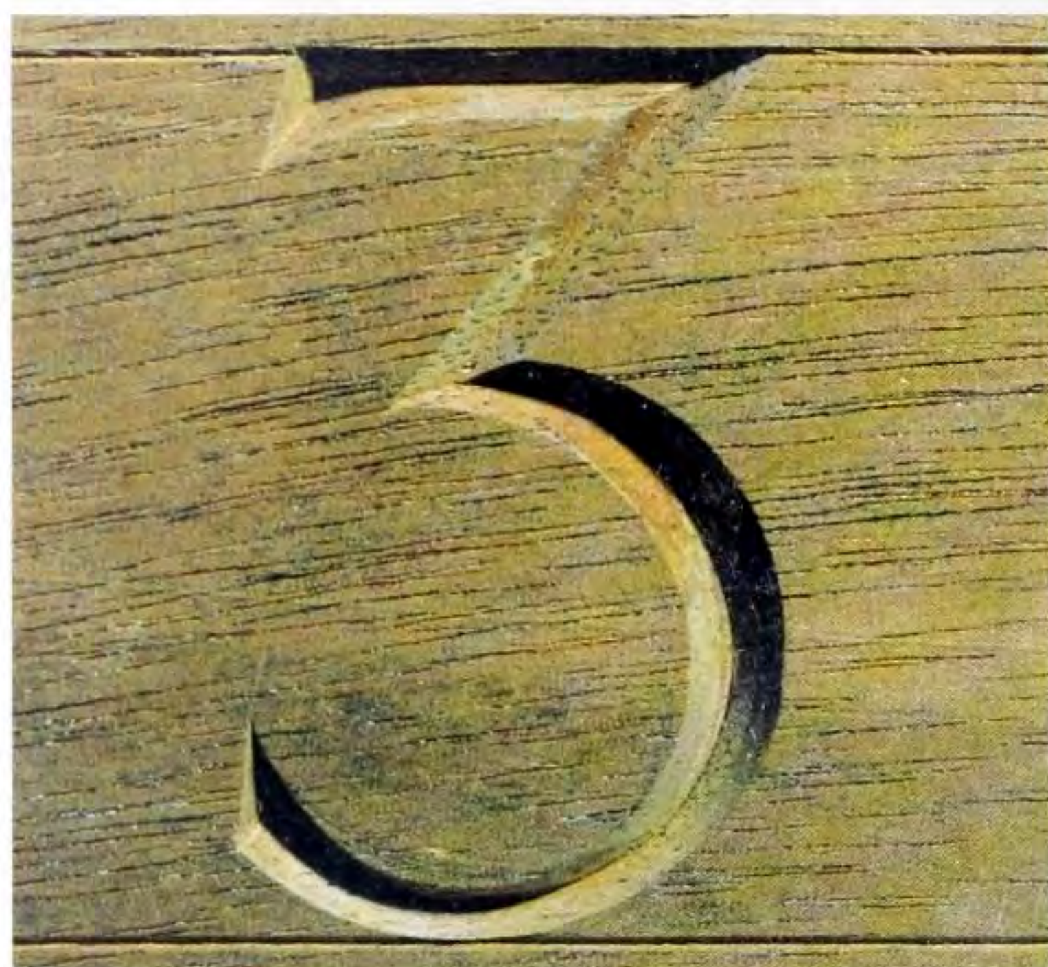
Fig 6.36 Numbers can be incised with exactly the same techniques as letters.
