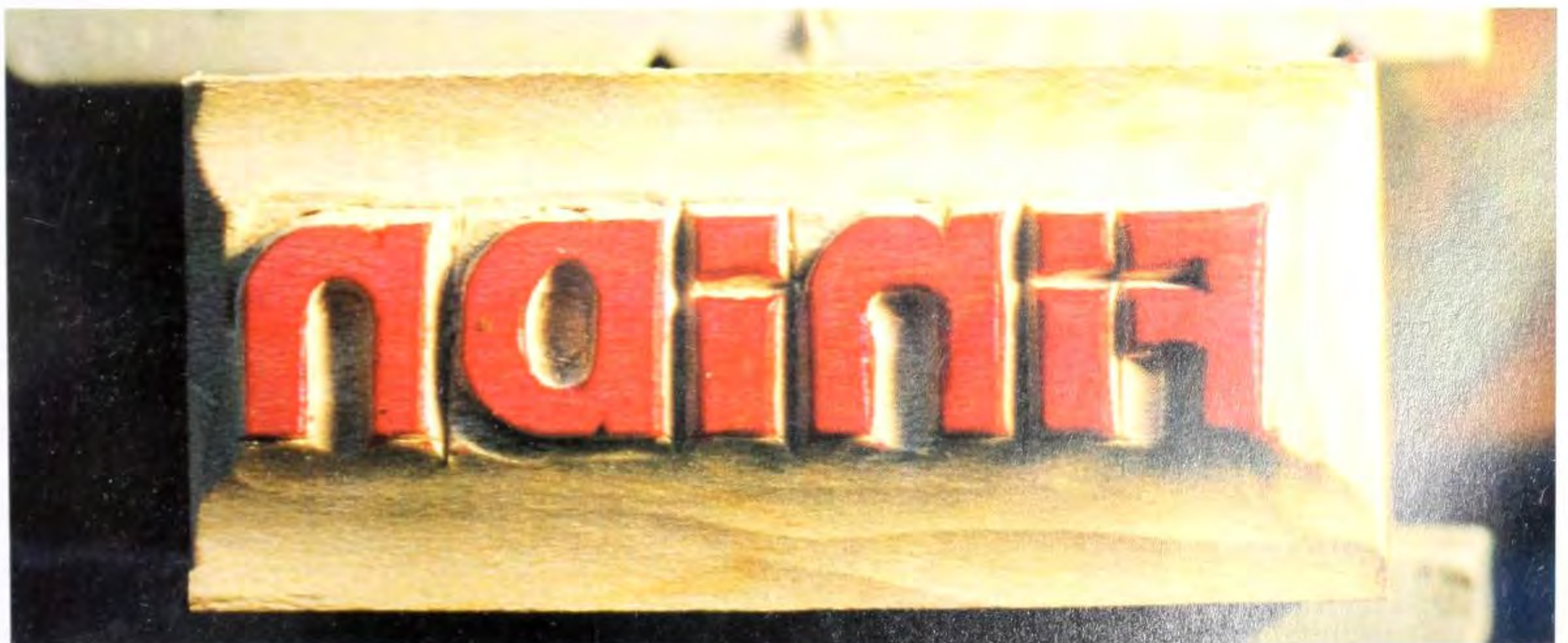
Fig 12.26 Finishing off the rounded counters using a small gouge.
