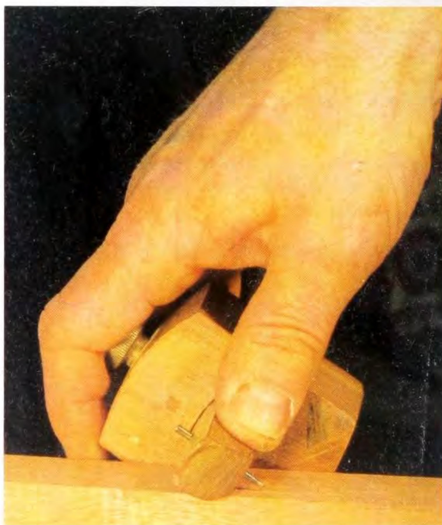
Fig 8.12 Using the marking gauge: start at an angle and rotate the pin down on to the wood surface as you push it away from you. Always keep the face of the gauge against the back of the wood.
