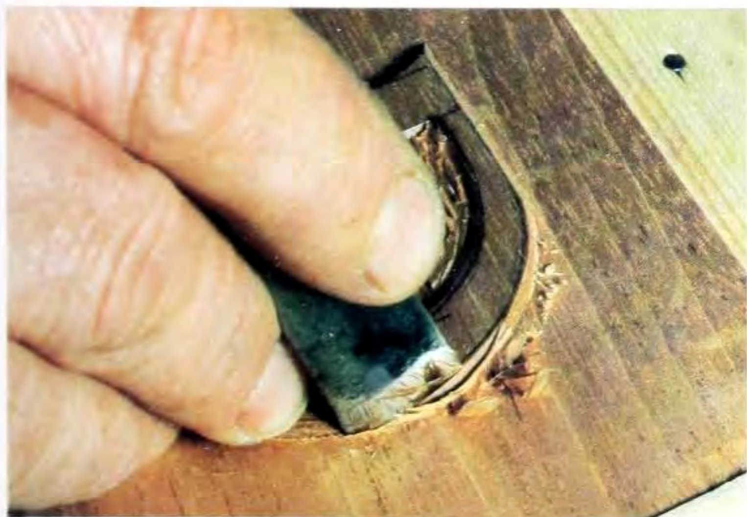
Fig 8.66 Setting in the outer curve using the no. 4 x 15mm (7/16in) gouge, after levelling.
