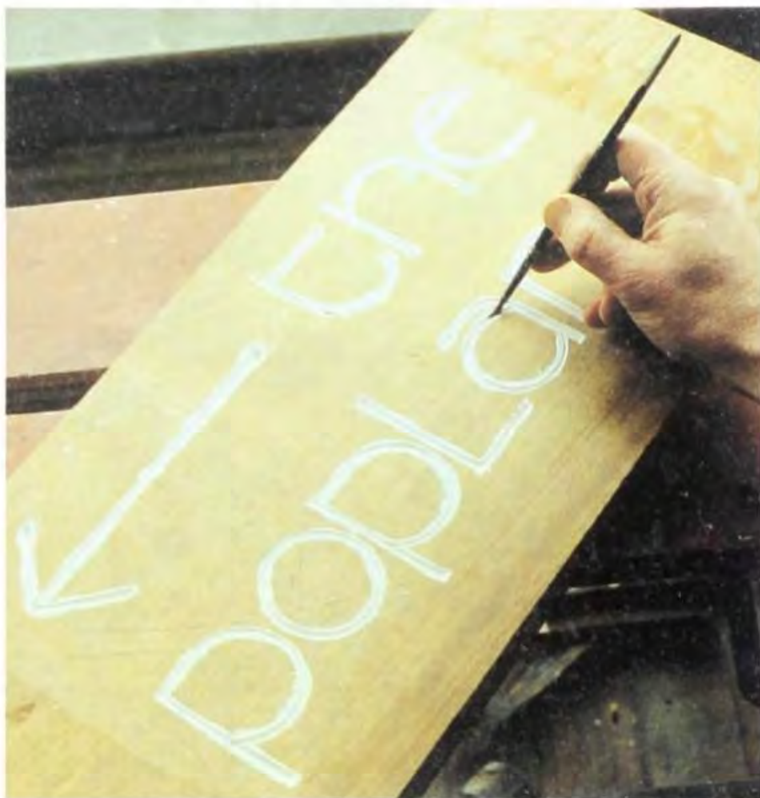
Fig 11.35 Painting the letters for extra clarity in an outdoor setting.
