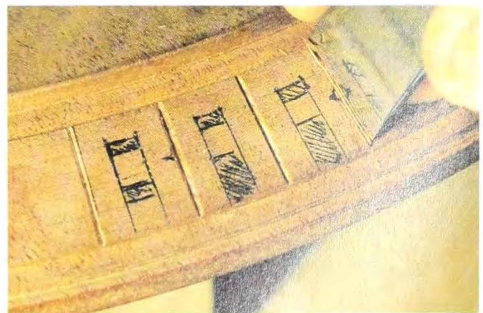
Fig 12.14 Separating the letters with a chisel by carving a V trench between each.
