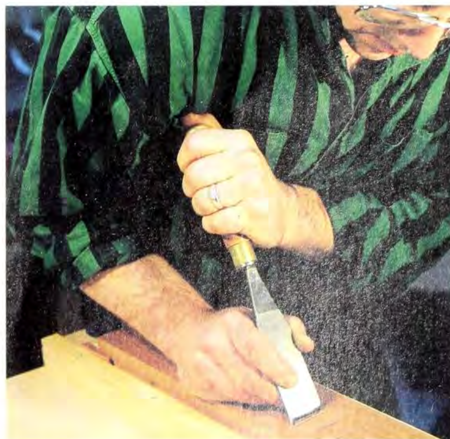
Fig 5.16 Cleaning up the trench by hand. The root often needs attention at this stage.
