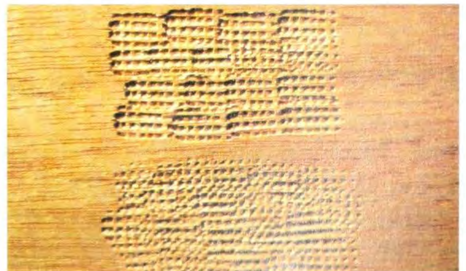
Fig 7.17 The effect of heavy (top) and light (bottom) frosting.
