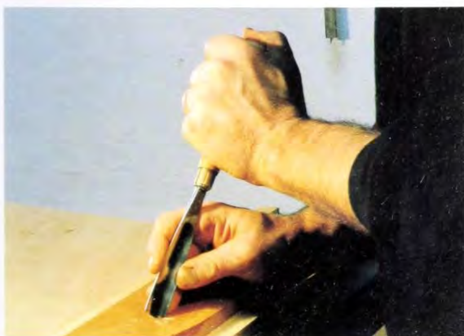
Fig 5.84 Here you can see the starting position, with the corner of the gouge positioned at the near corner of the crescent (above). The gouge is then rotated, and the handle lowered, to lead the gouge corner along the root of the crescent to clean it (below).
