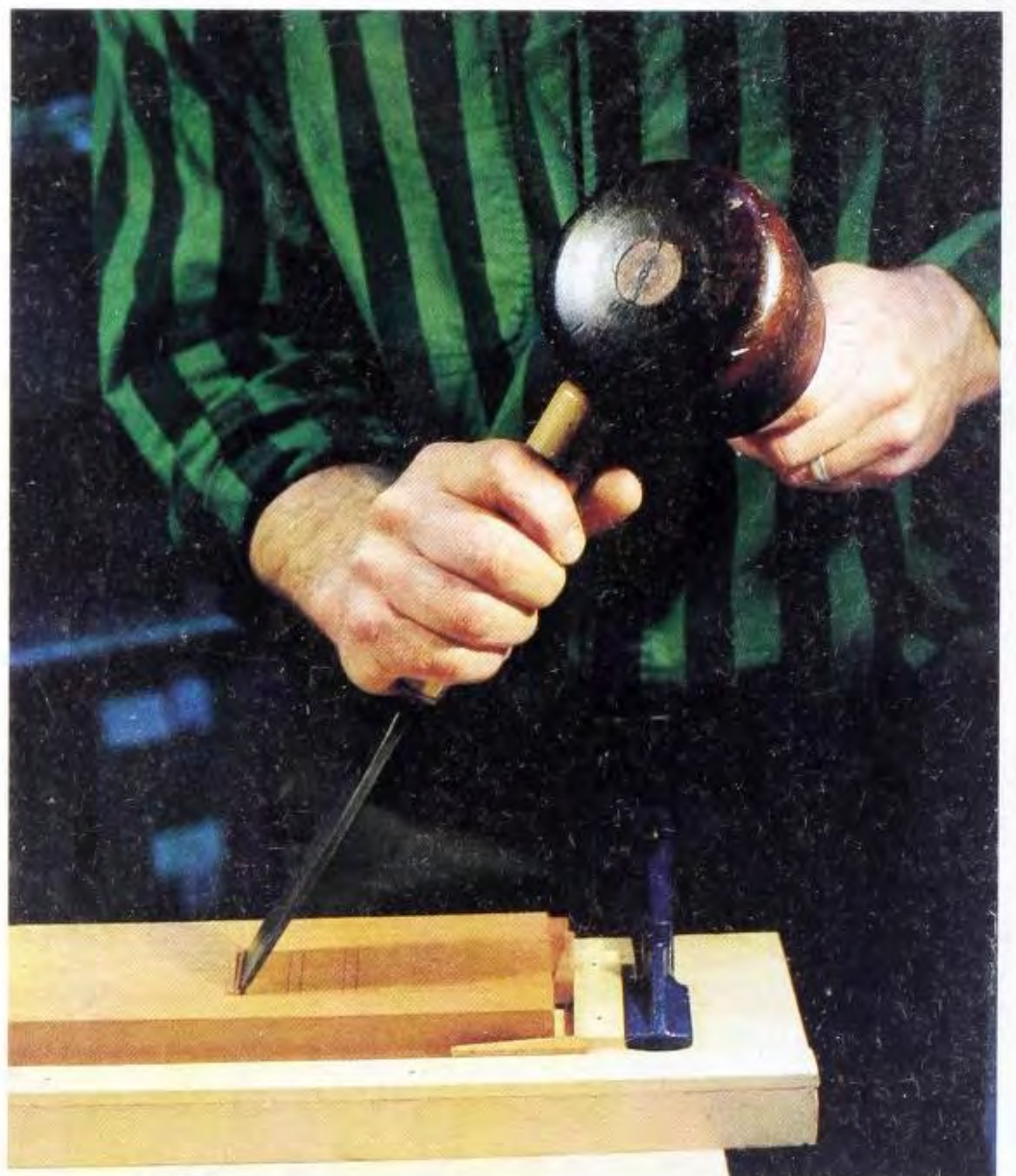
Fig 5.15 Combining what you have learned so far to cut a neat trench with the aid of the mallet: the stop cut, followed by the two angled cuts, reversing hands for the second of these.
