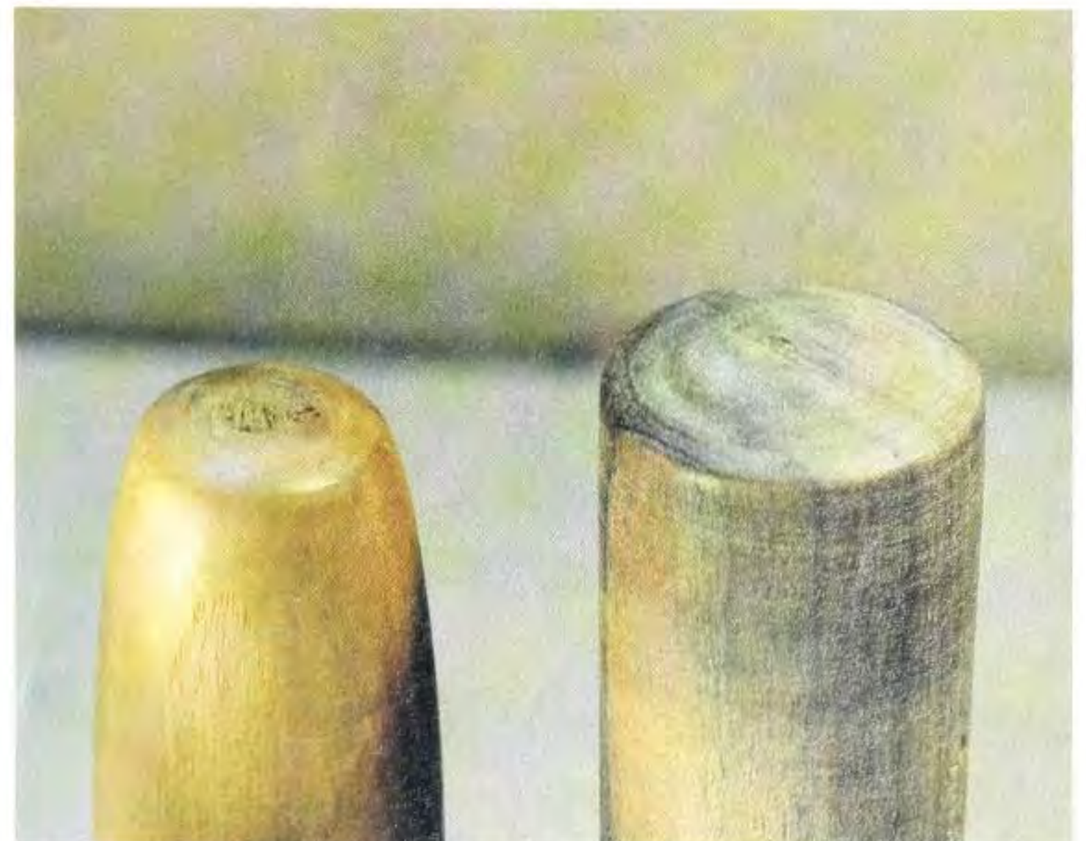
Fig 2.2 The handle on the left, as supplied with the tool, has a small end and is less easy to hit with the mallet compared with that on the right.
