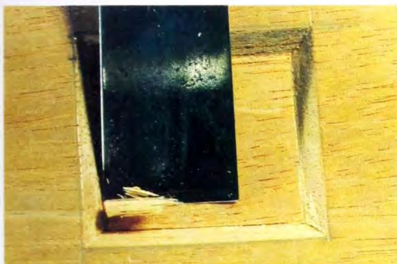
Fig 8.41 Levelling the counter using as wide a flat gouge as is possible.
