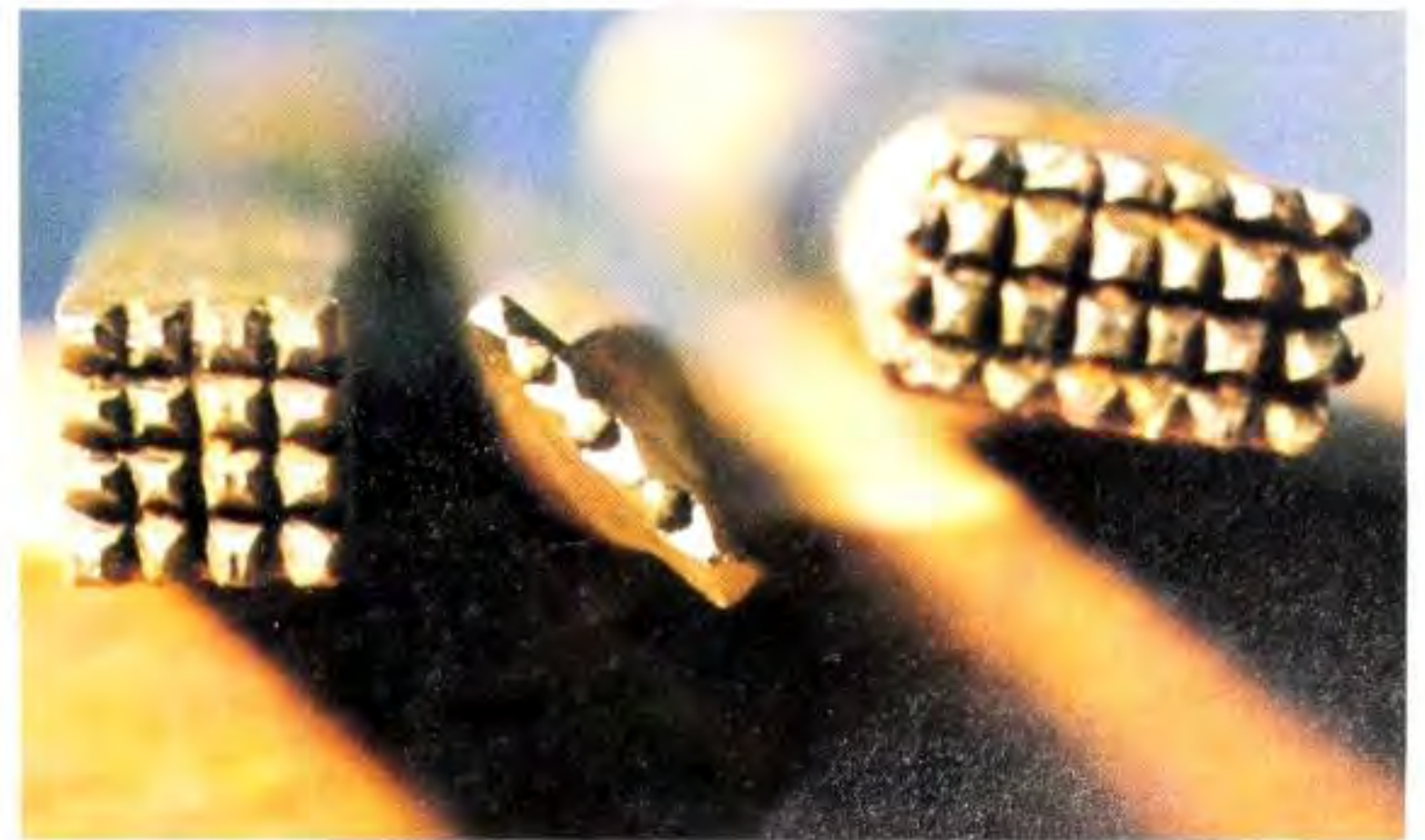
Fig 7.16 The working ends of frosting or matting tools. The two on the right have been made by filing nails with a triangular file.
