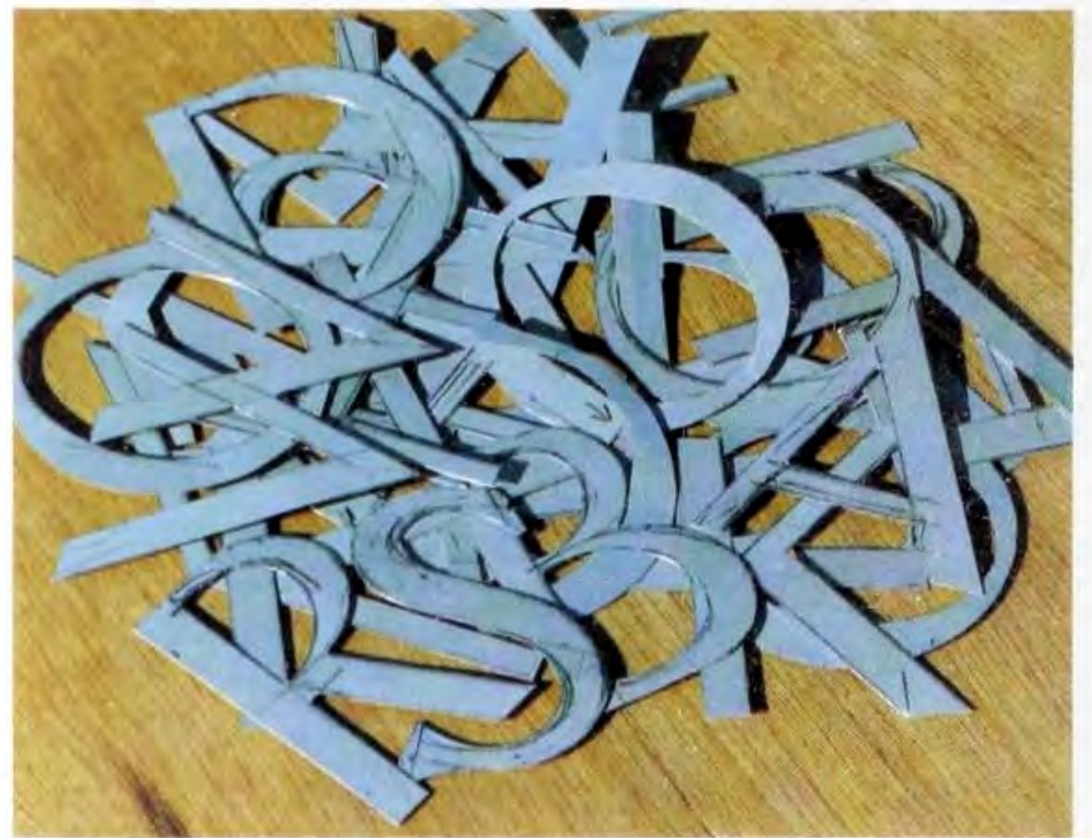
Fig 3.2 Letter templates in aluminum.
