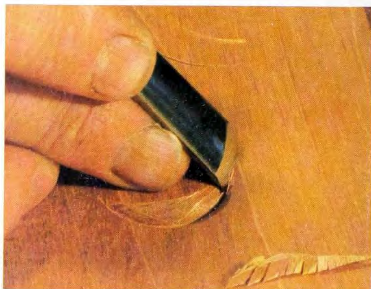
Fig 5.88 Cutting the inner wall of the crescent. Slicing begins with the corner of the gouge following the root, and exiting at the other corner.
