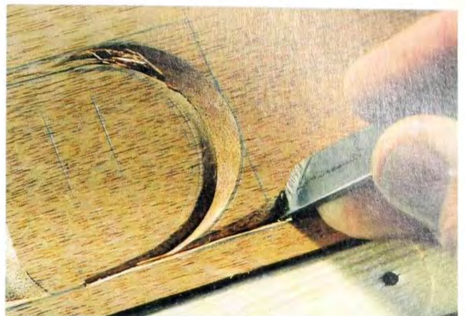
Fig 10.29 The end wall of the foot may need the sharper angle of a regular skew chisel to finish off, as here.
