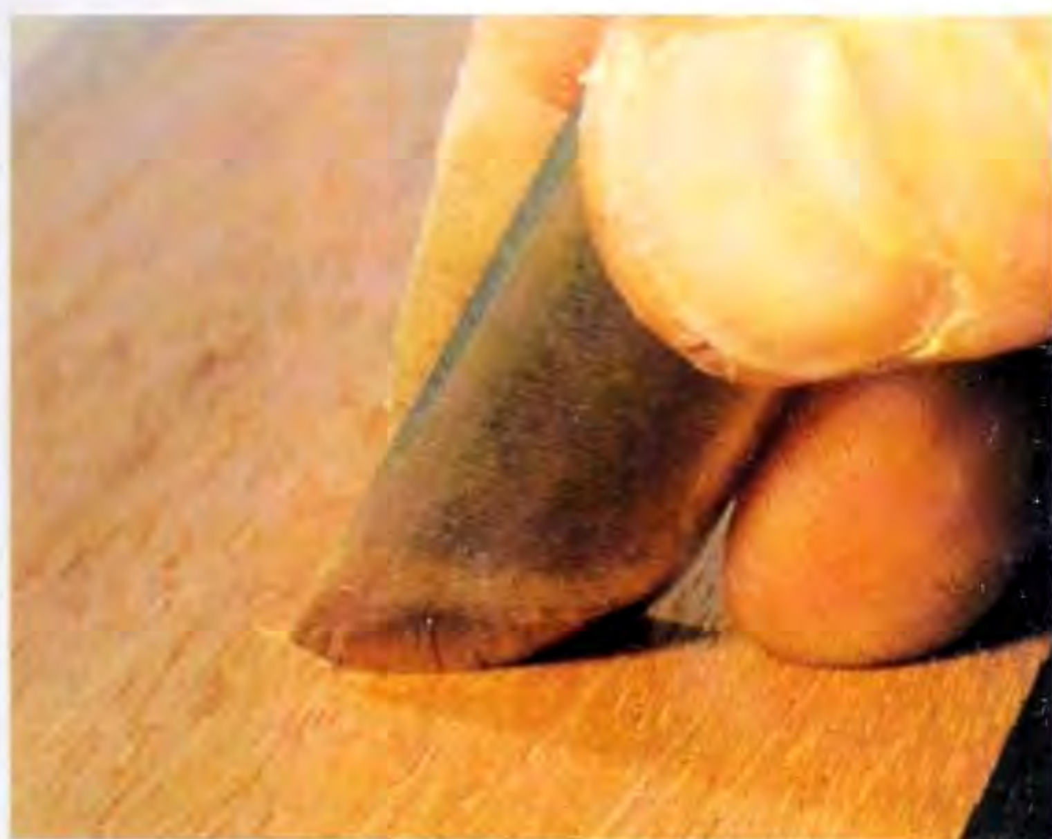
Fig 5.87 The position of the fingers for angled cuts from the opposite direction.
