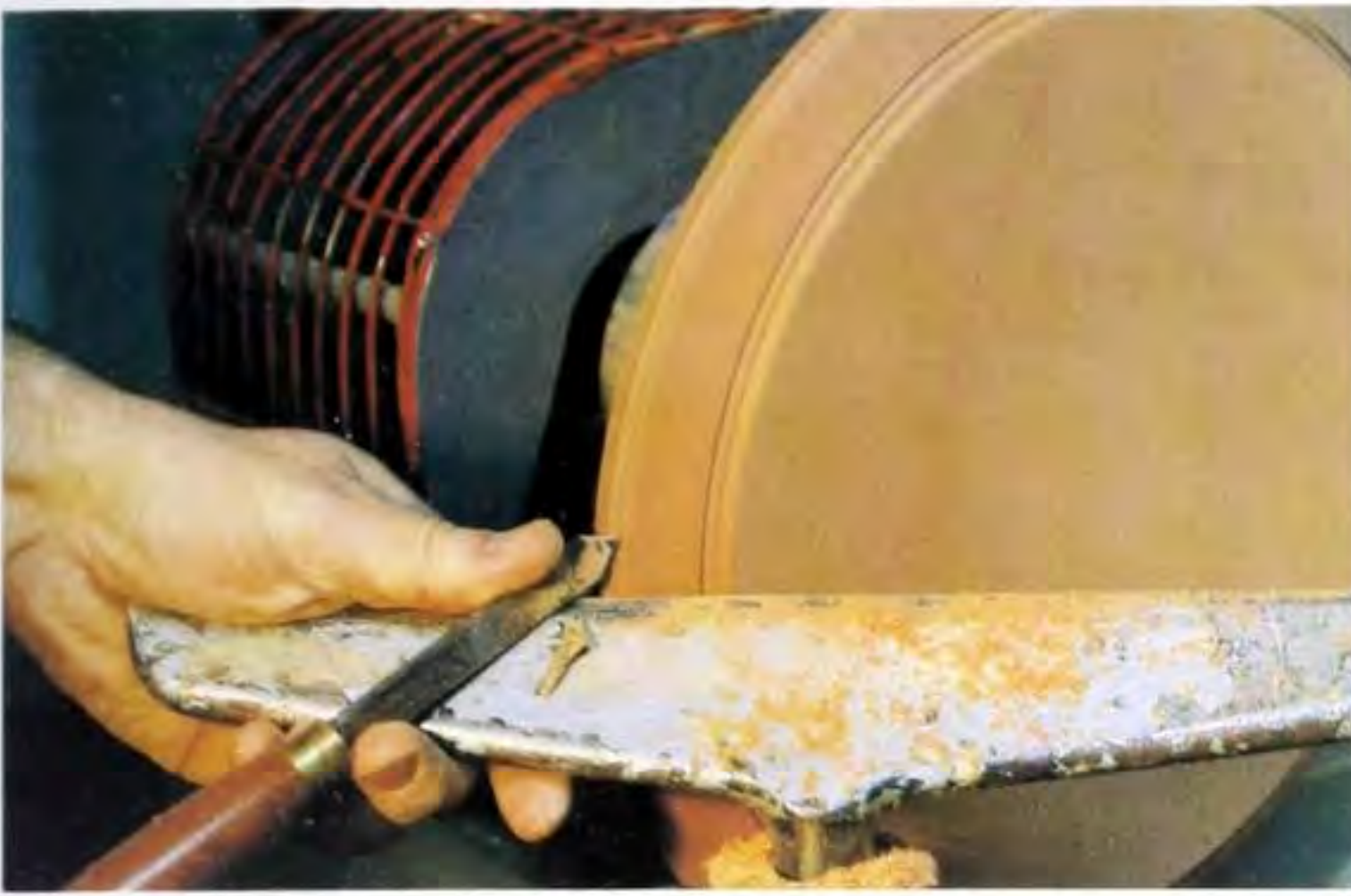
Fig 12.10 Turning the board allowed me to set the depth of the ground above and below the letters.
