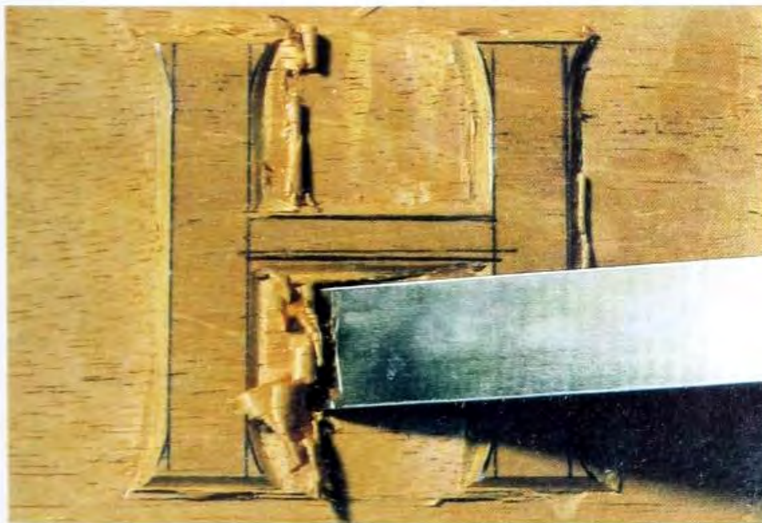
Fig 8.53 Levelling with the flat gouge.
