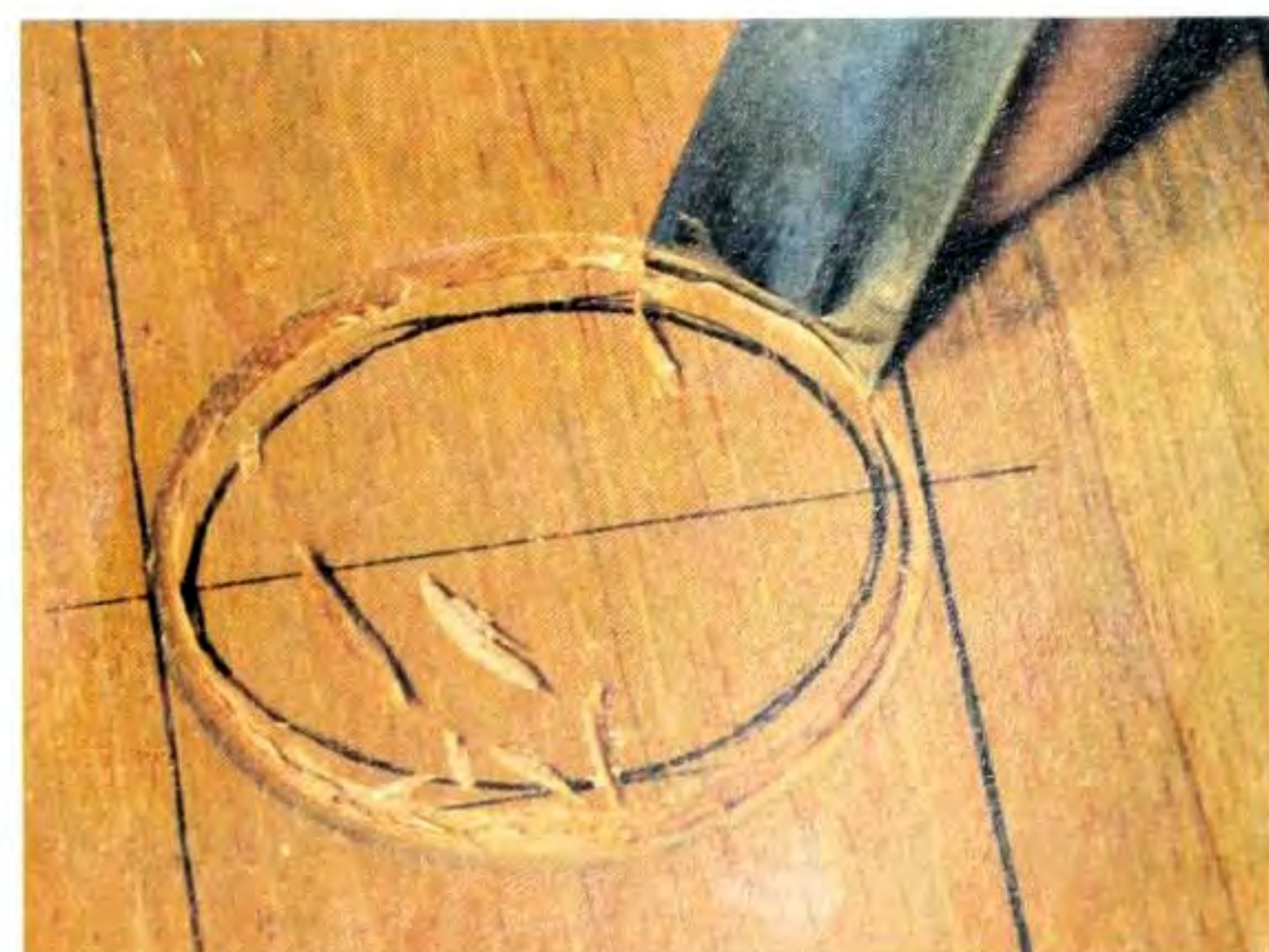
Fig 5.92 Make angled cuts to the outside.
