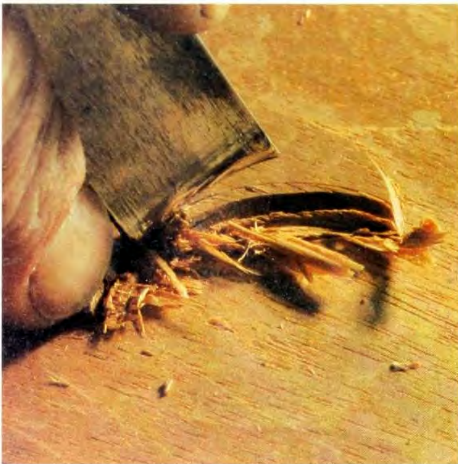
Fig 8.35 Slicing around the crescent with the corner of the gouge. Note the supporting finger.
