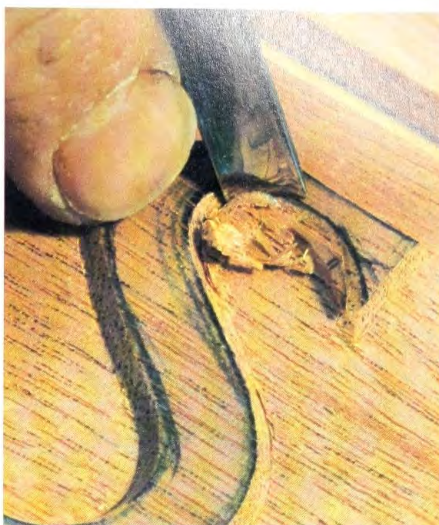
Fig 8.80 A narrow gouge is needed for setting-in the tight curves.
