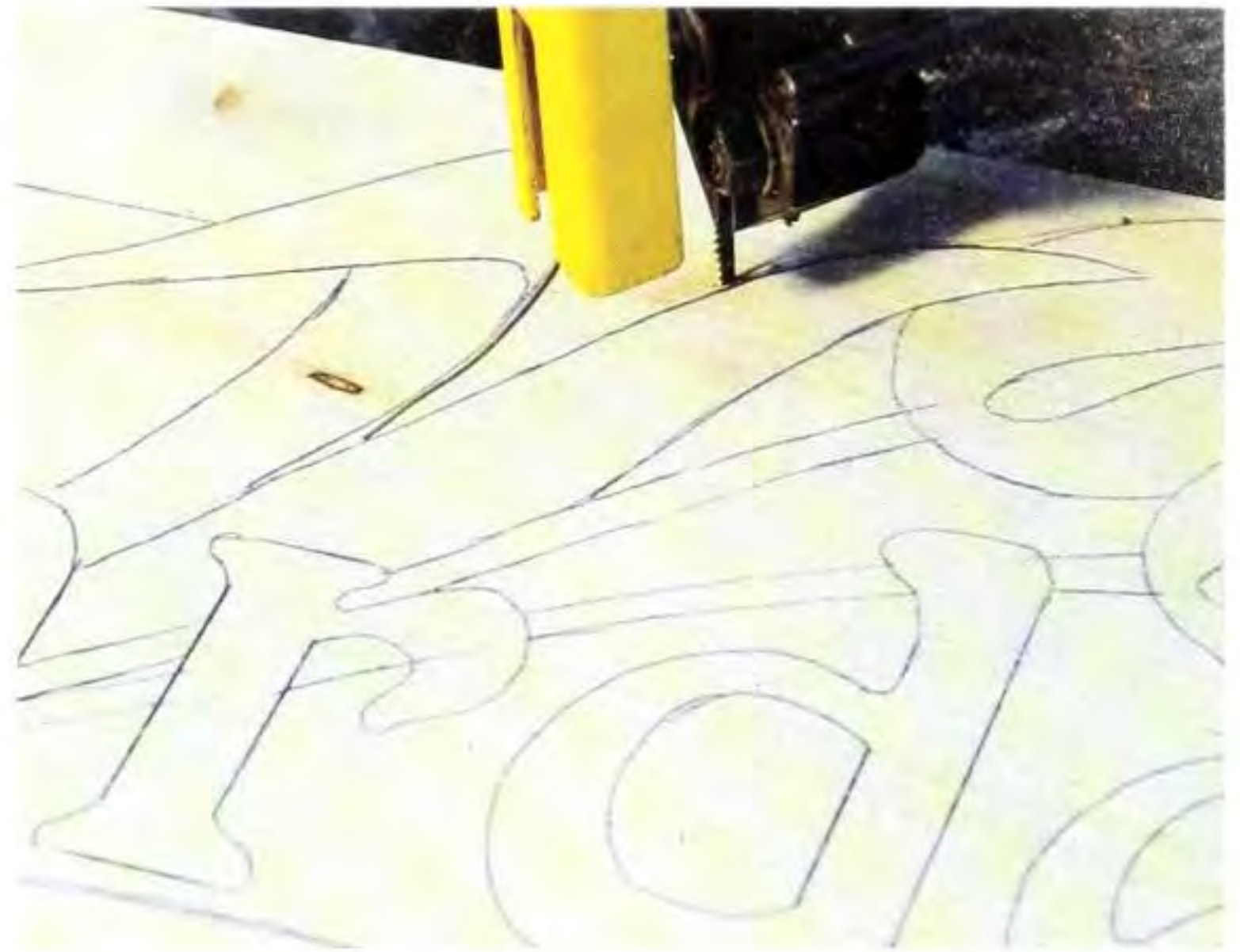
Fig 12.30 Bandsawing the profile of the board.
