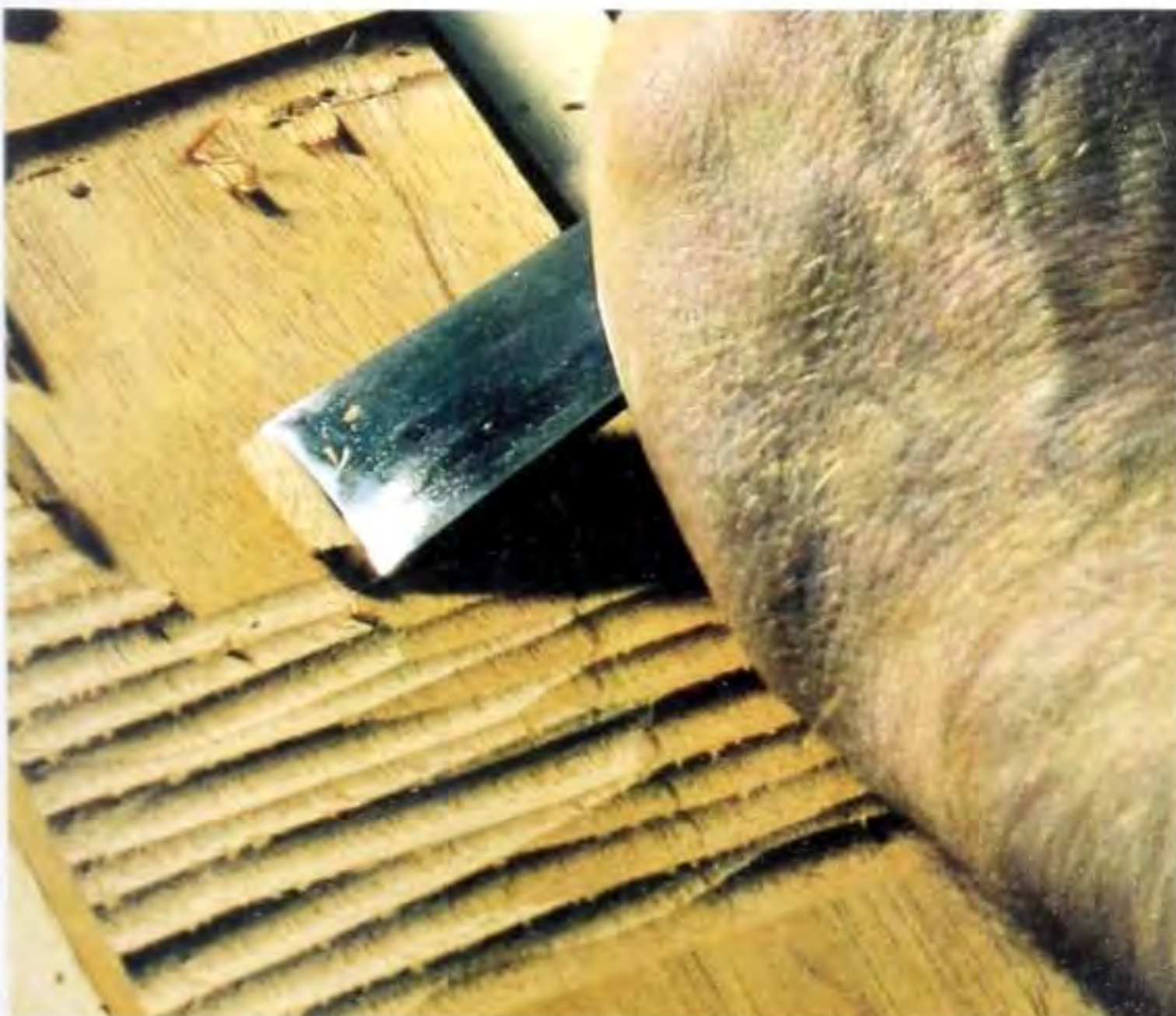
Fig 8.15 Levelling the lowered surface.
