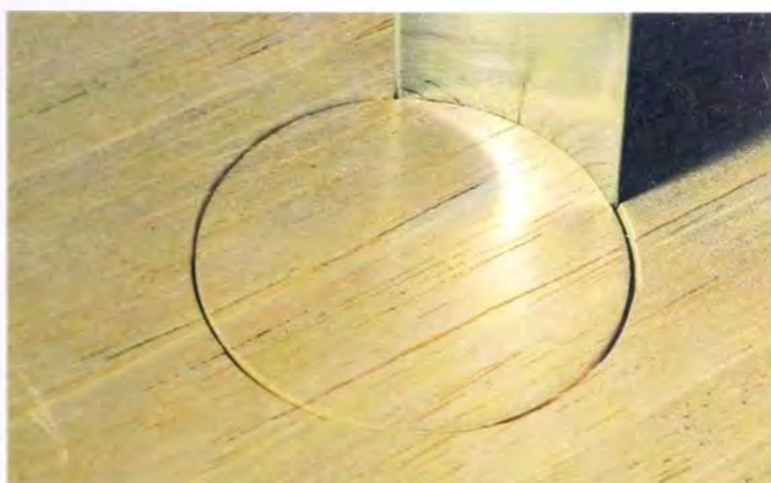
Fig 5.78 Eventually, the gouge will have cut a complete circle.
