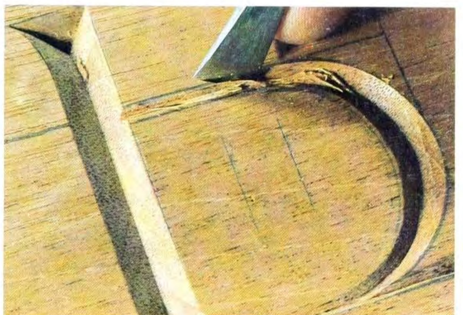
Fig 10.30 After the flat horizontal section has been removed in the normal way, merge in the lobes with the fishtail skew, or a flat gouge.
