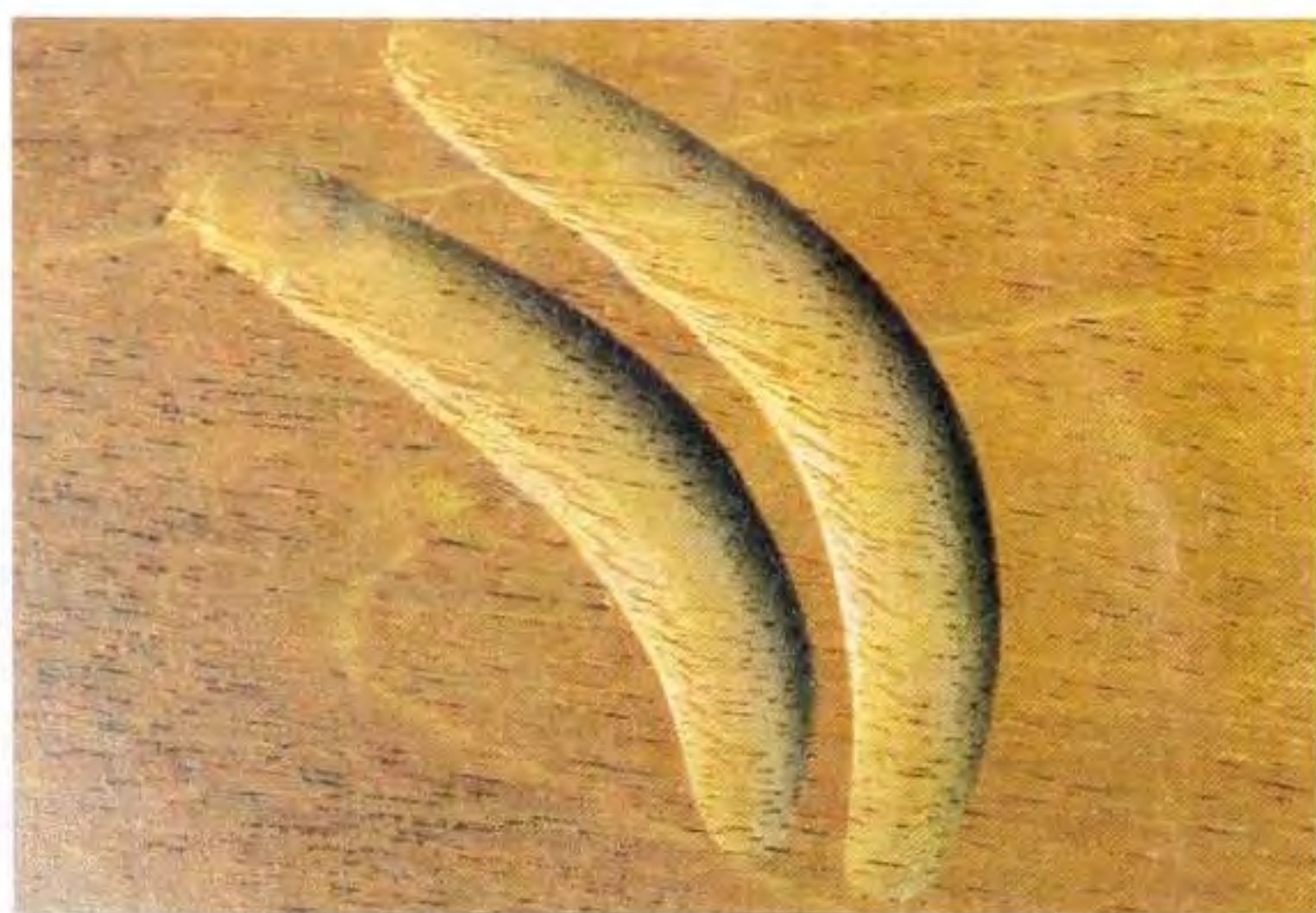
Fig 8.7 The left sides of these channels run against the grain, and have torn it. Always place this side in the waste wood.
