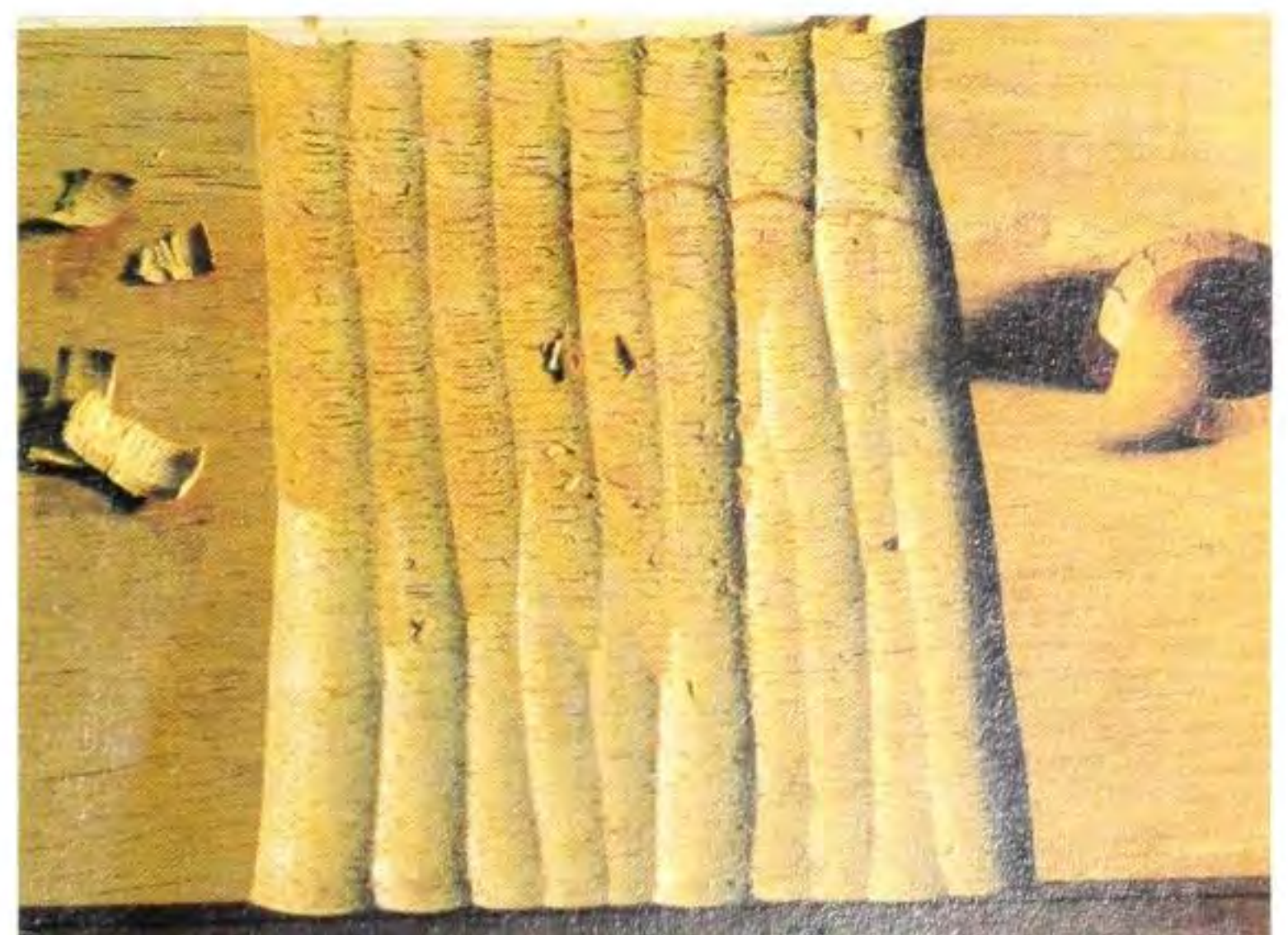
Fig 8.14 Starting from the edge, lay down a series of channels, stopping short of the far side. Then turn the wood around and finish off (there is no need to join the channels). The result looks a bit like a ploughed field.
