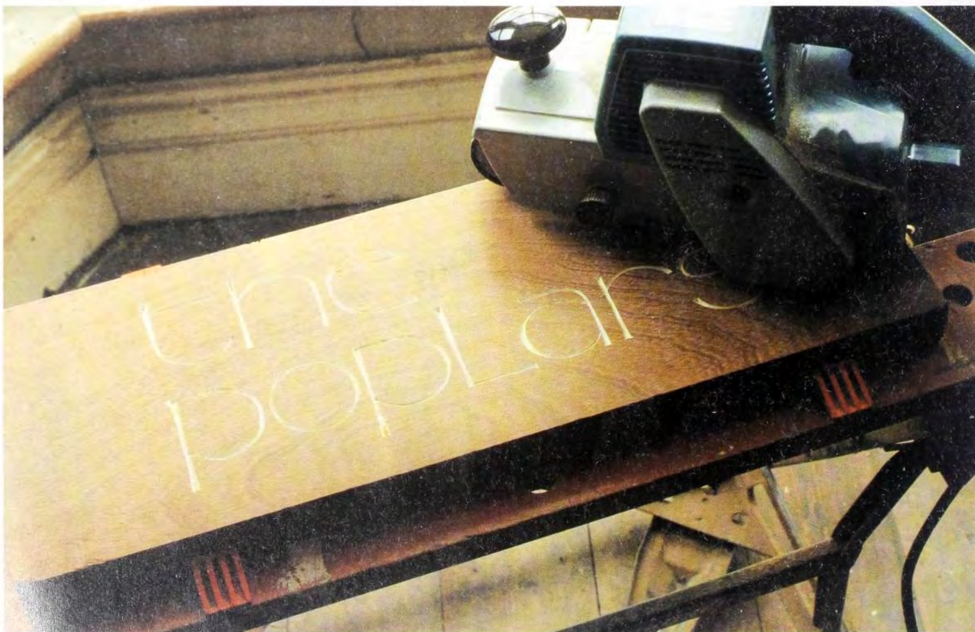
Fig 11.36 After painting, a very fine grit on the belt sander cleaned off the excess paint down to the bare wood. The sign was then finished with Danish oil.
