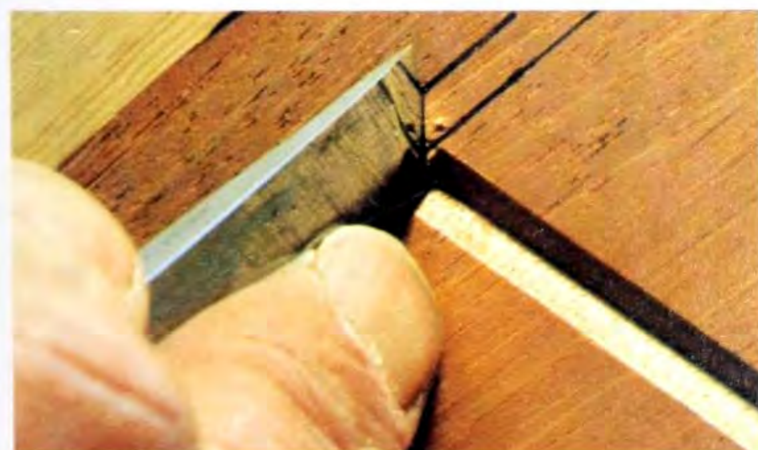
Fig 5.44 Cutting angled serifs. Begin with the stop cuts.
