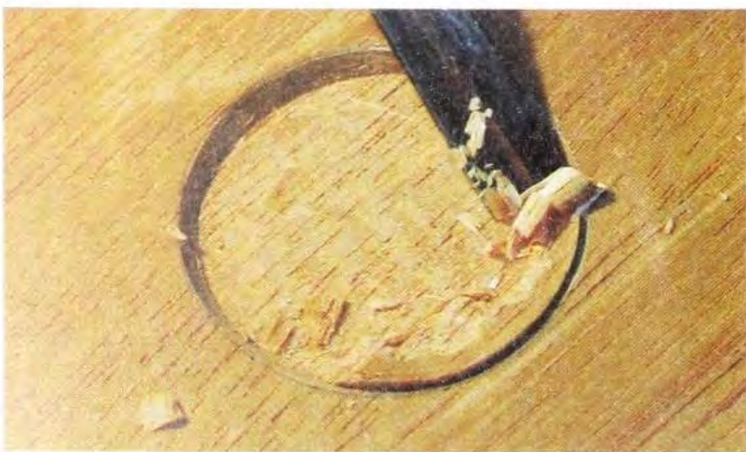
Fig 8.38 Levelling with a small flat gouge. Take care not to run the corner into the wall.
