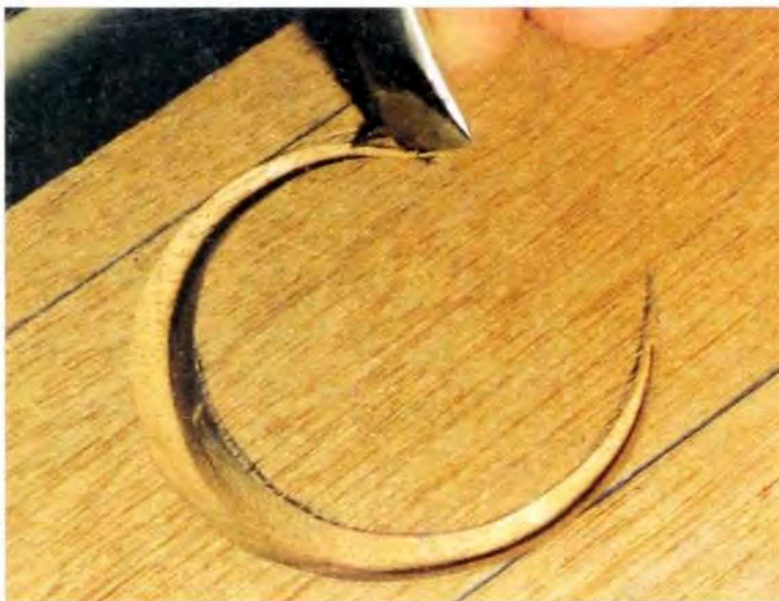
Fig 5.98 Make the end wall cut.
