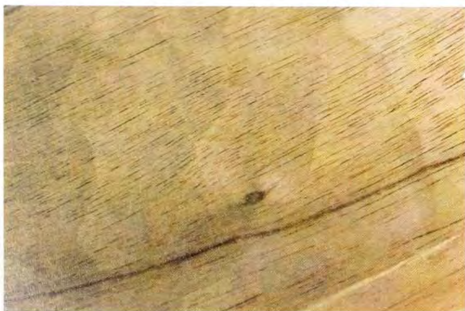
Fig 8.18 This is the sort of flat surface you should aim for, having a 'sense' of flatness, but with a light texture that shows it has been carved by hand.
