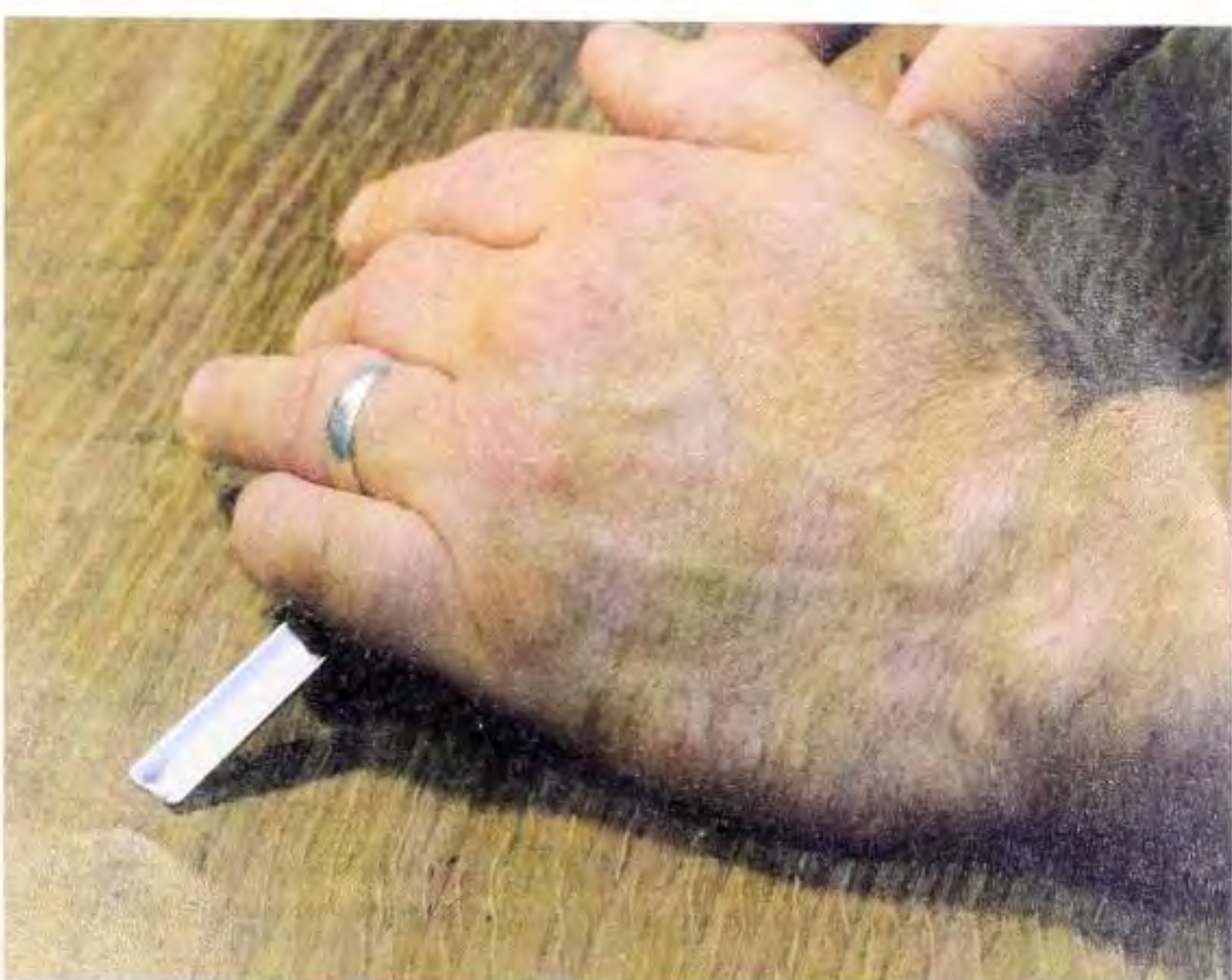
Fig 2.5 Two poor tool grips: the 'backcrank' and the 'snooker cue'.
