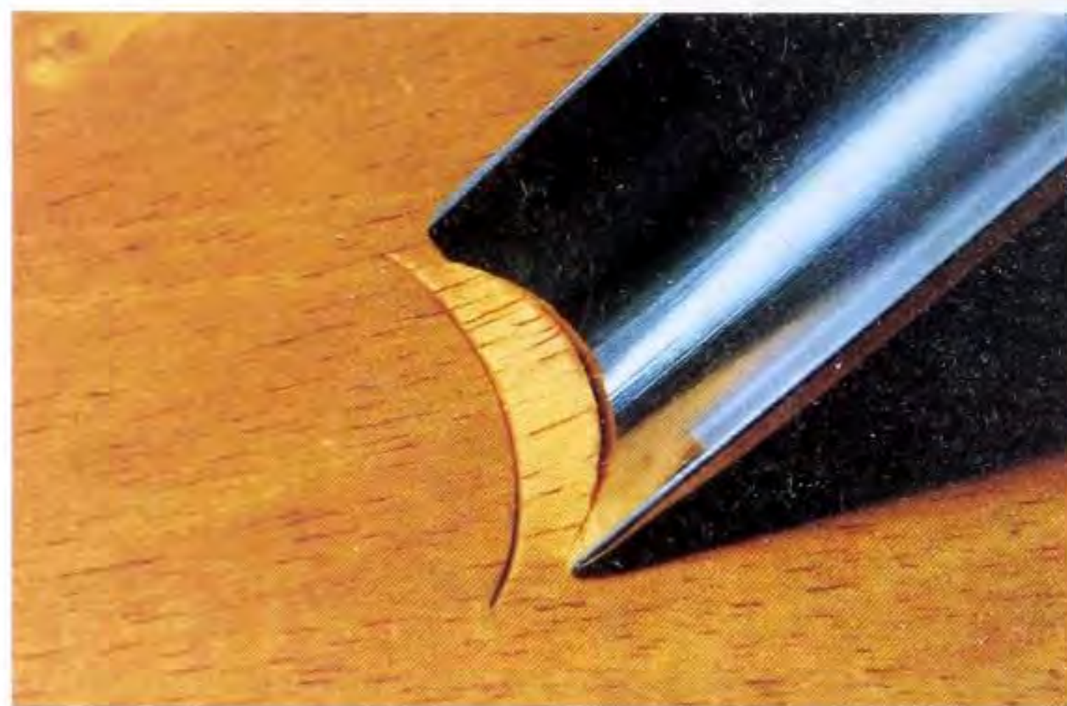
Fig 5.82 The angled cut following the vertical stab cut produces a crescent, clearly shown here.
