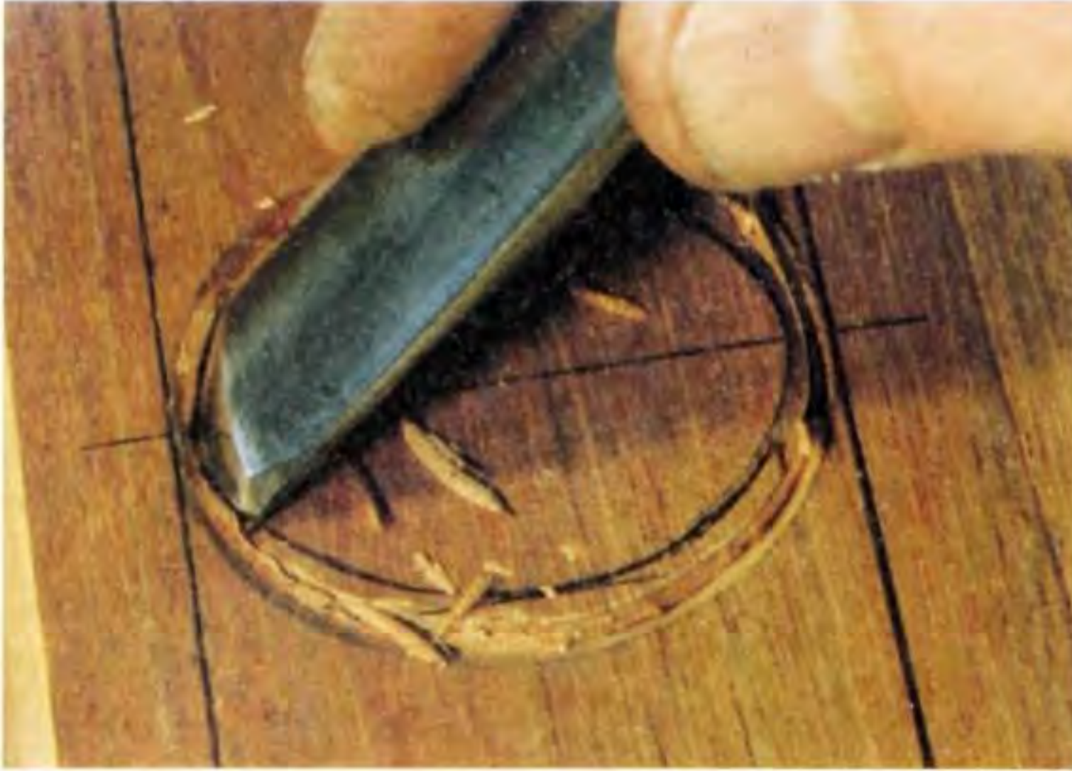
Fig 5.93 Use the same gouge for the top and bottom inside angle cuts.
