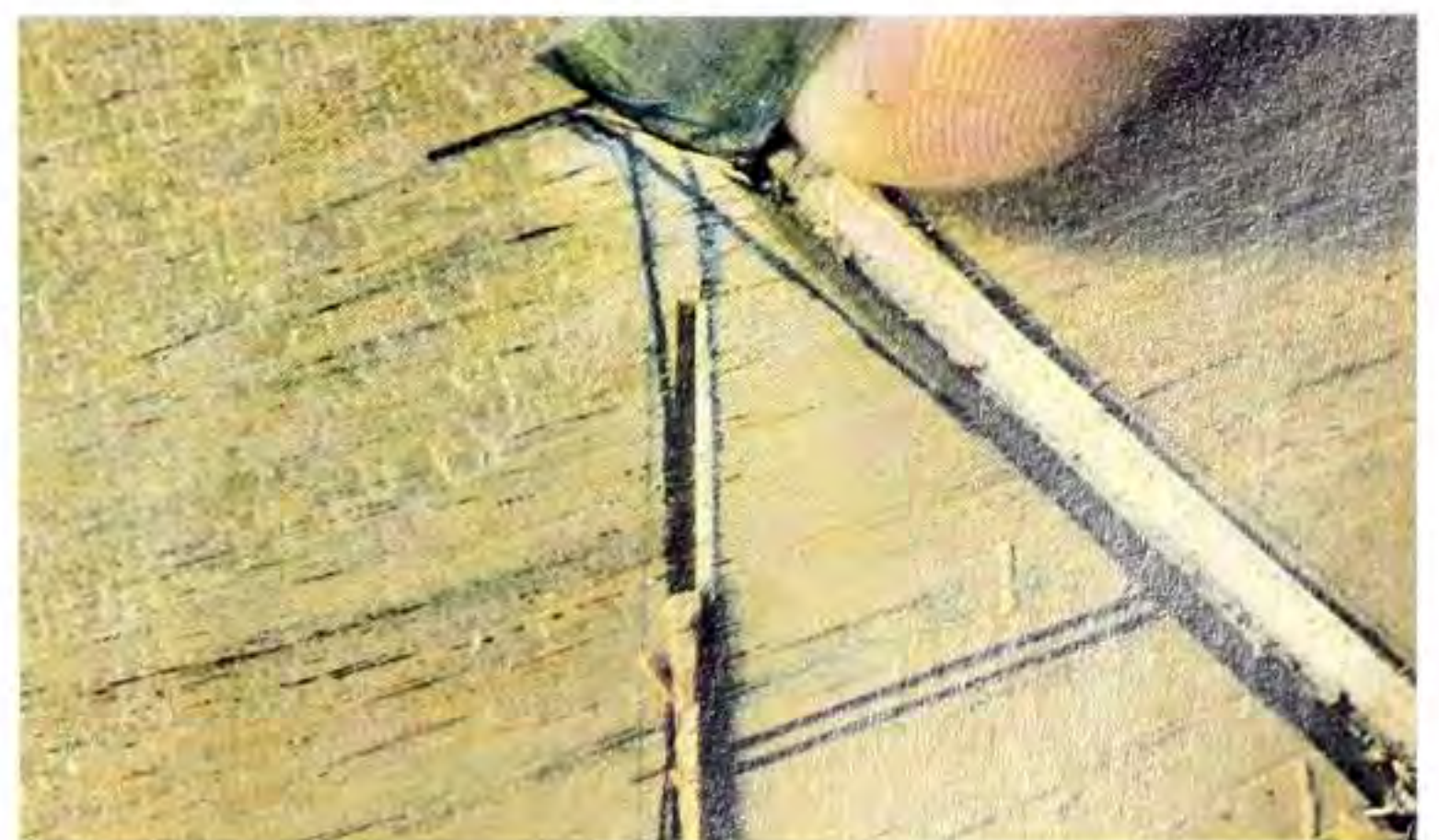
Fig 10.13 Using the skewed fishtail chisel to make stop cuts for the serifs.
