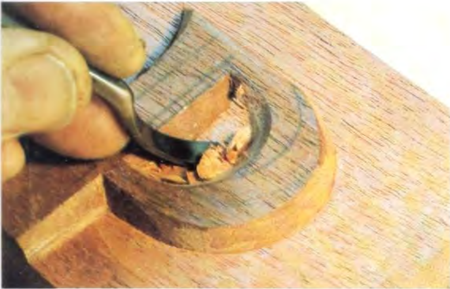
Fig 7.10 Here you can see how the tight bend of the gouge allows it to get into otherwise inaccessible areas. When buying these tools, the tighter the bend the better for this kind of work.
