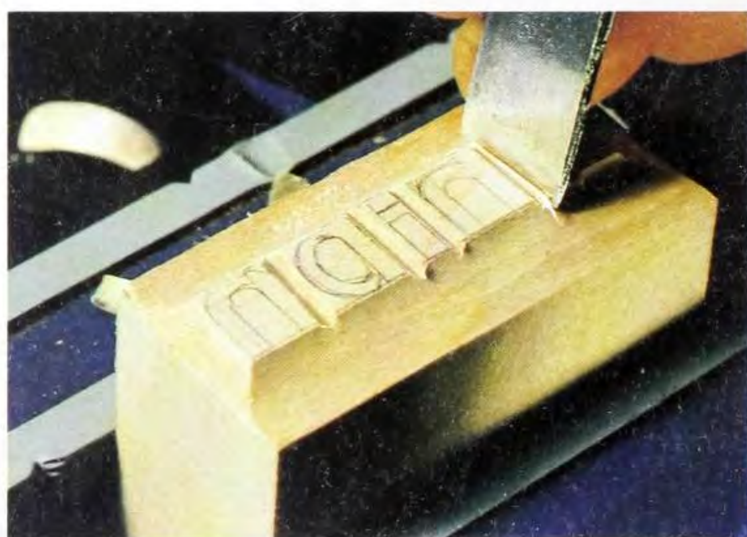
Fig 12.24 Separating the letters with a chisel. A V tool could be used for this job, but a chisel guarantees a straight line.
