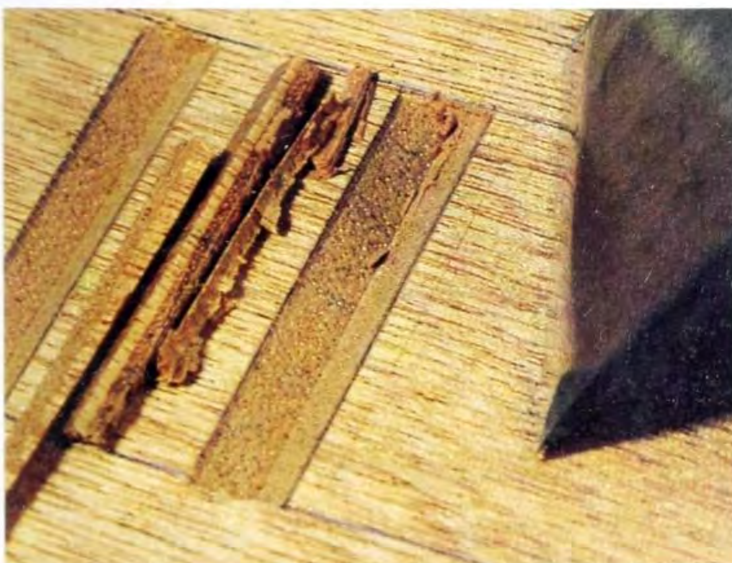
Fig 5.13 Making the centre stop cut, following by the two angle cuts which release the chip and shape the trench. This simple technique is a crucial one, and must be mastered.
