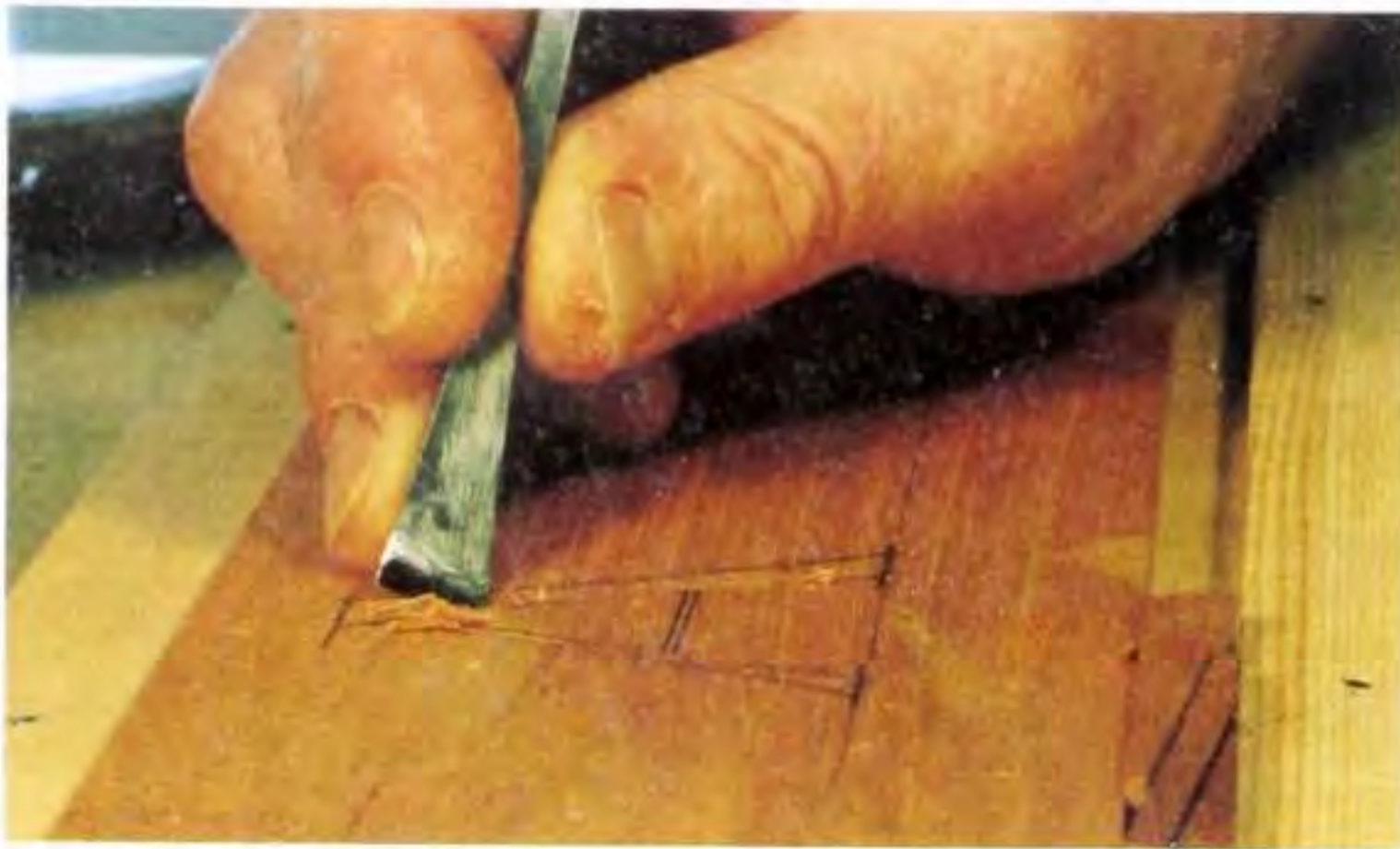
Fig 10.14 Running up the side at the right angle using the pen and dagger grip. For this slicing cut the thumb is the major mover and pivot.
