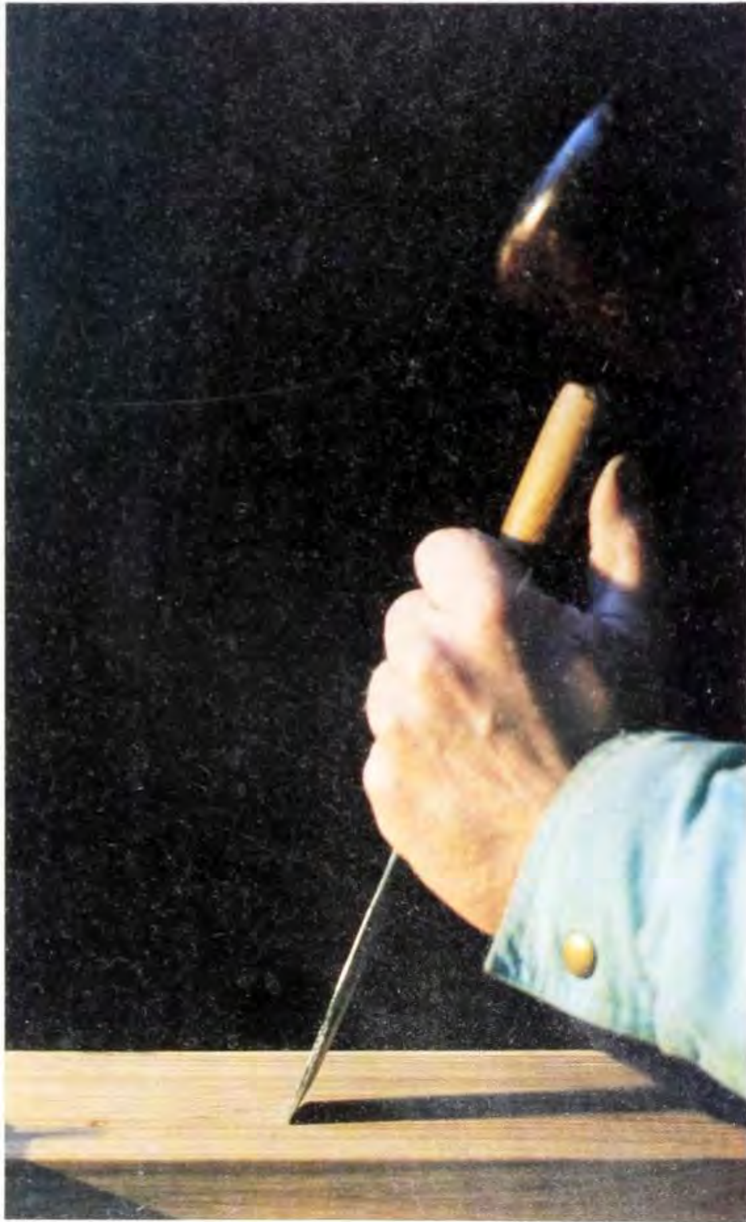
Fig 2.7 Striking with the mallet. Note the grip on the tool, especially the thumb on the handle which aids control.
