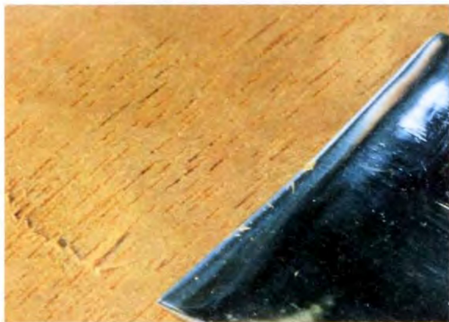
Fig 8.17 It is very easy to tear wood fibres with such a flat gouge. Clean up such tears as you go along.
