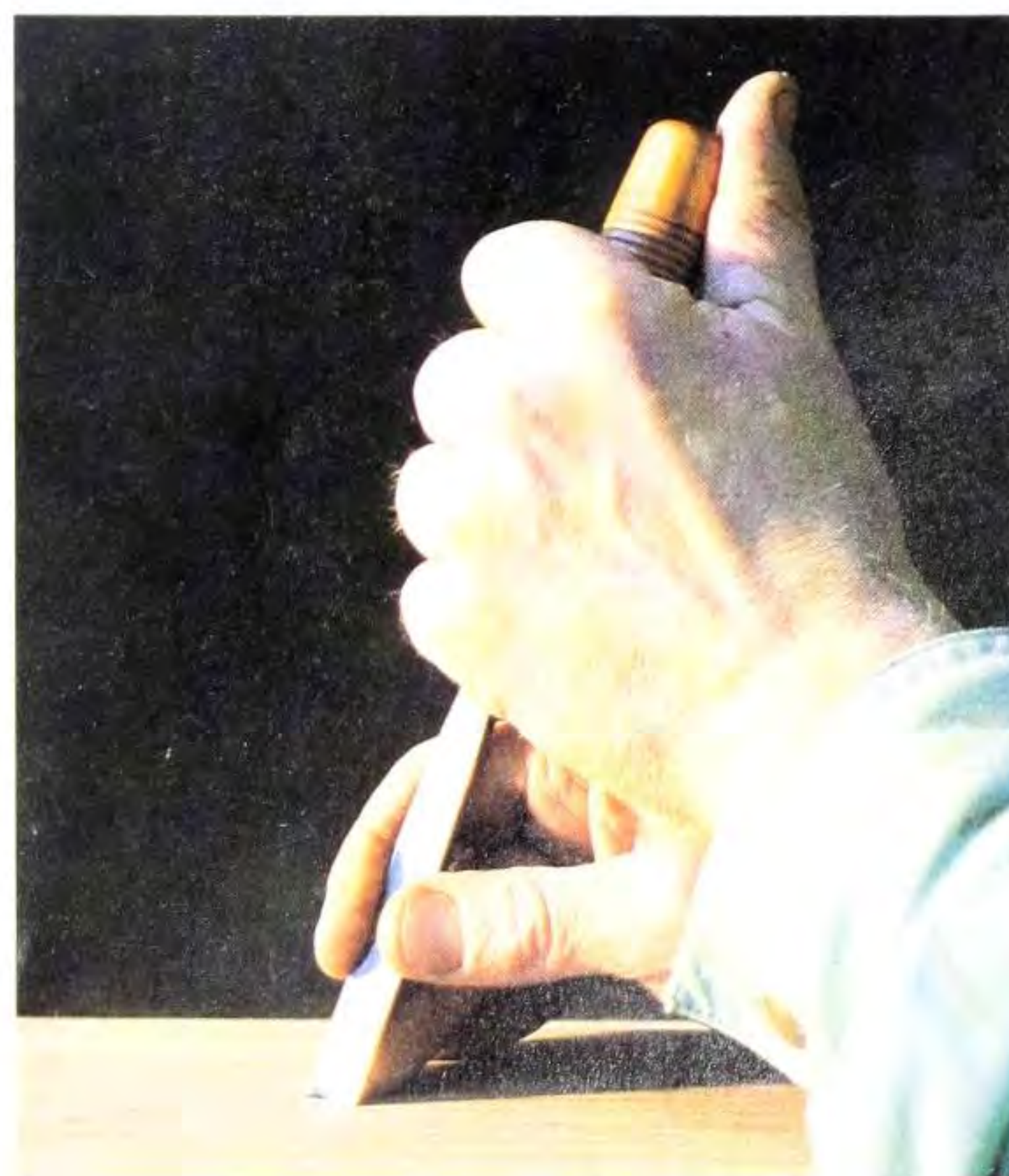
Fig 2.3 The 'pen and dagger' grip, showing how the blade of the tool is held rather like a pen, and the handle rather like a dagger. The starting position is shown above and the complete grip below.
