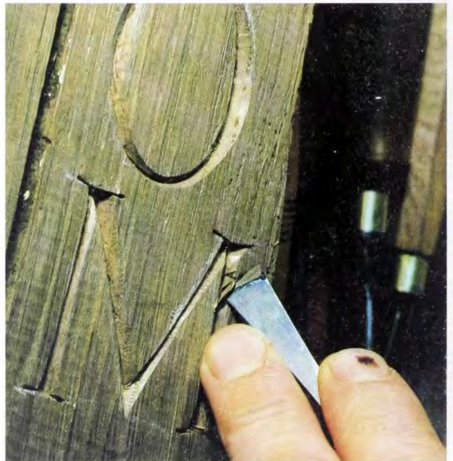
Fig 11.4 Shaping the versal waisting with a skewed fishtail chisel. Remember that when carving into vertical grain, stop cuts are required in the upright ends instead of the horizontal ends.
