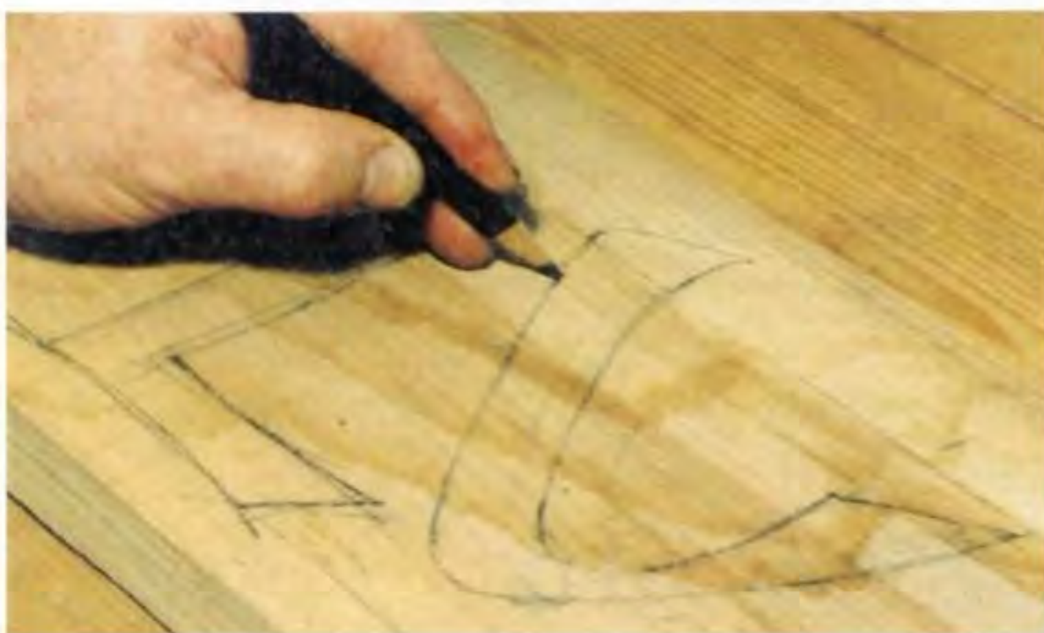
Fig 12.2 Drawing out the letters freehand.
