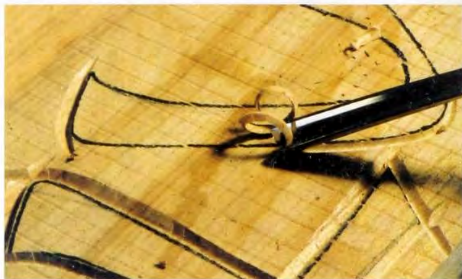
Fig 12.4 Close-up of the V-tool work. The tool is tilted away to give the correct wall angle, and always passes with the clean cutting side to the letter.
