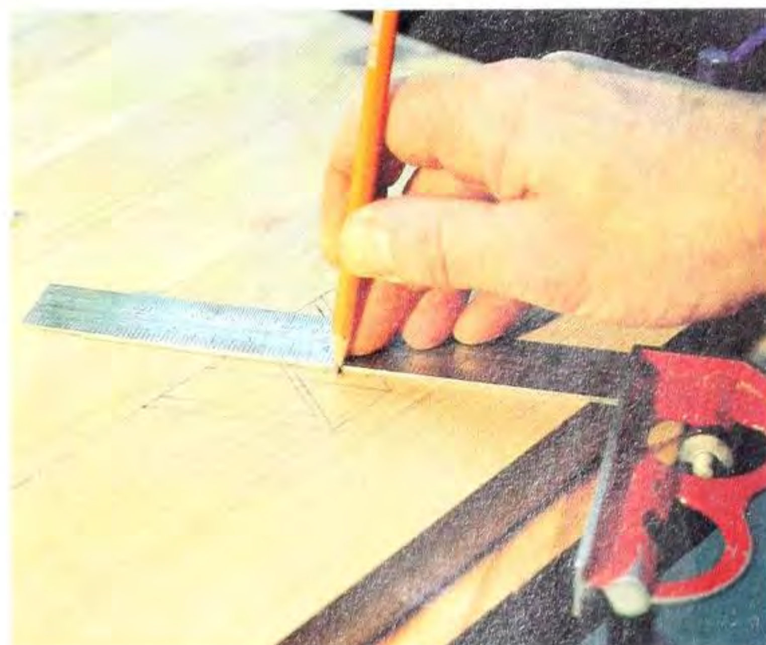
Fig 3.8 Filling in the horizontals, obliques and curves.
