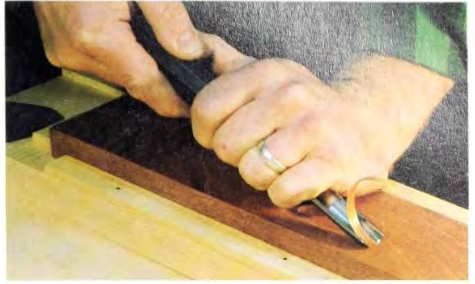
Fig 8.3 Both hands in the low-level (or low-angle) grip must work together. The thumb extended along the handle extends the effective width of the front hand and increases its control. The heel of the front hand always rests on the wood.
