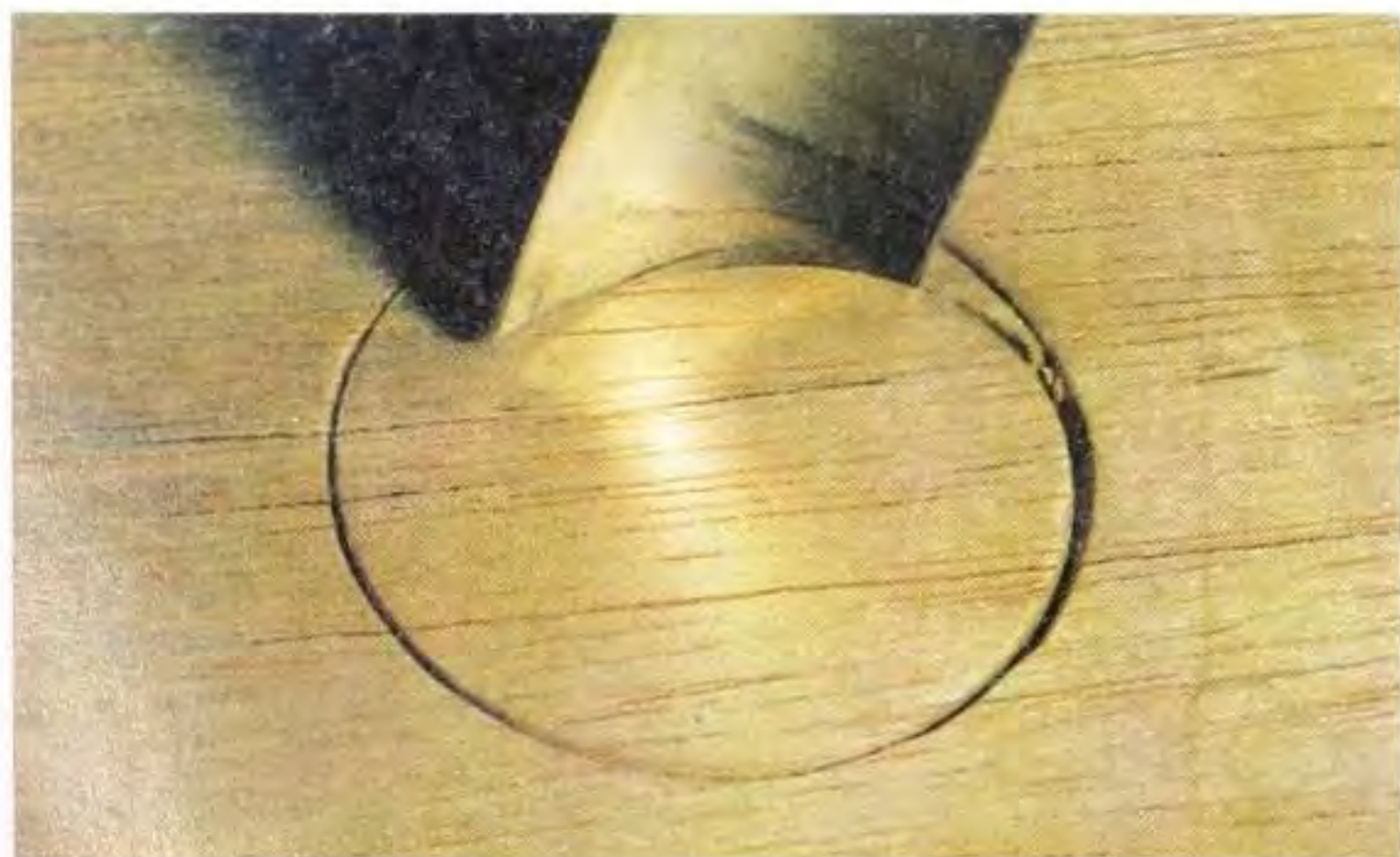
Fig 5.79 Start winding in the cut rather than following the circle.
