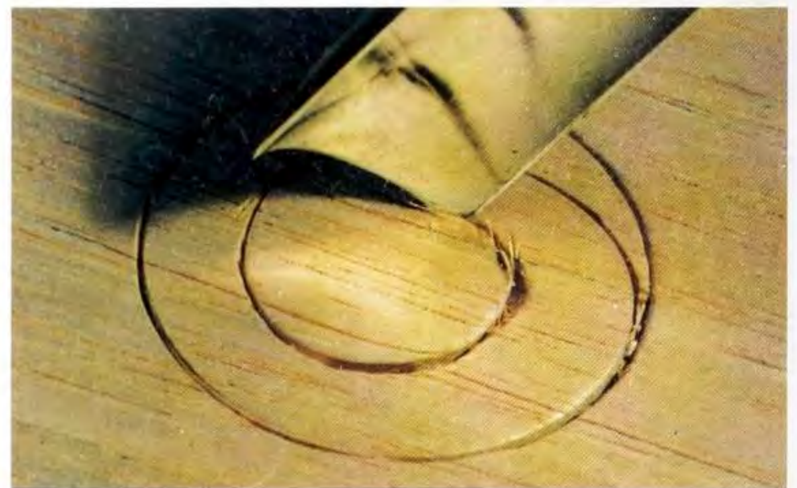
Fig 5.80 By pulling back the handle, and skating more on the trailing corner, you can easily cut a spiral into the centre of the original circle.
