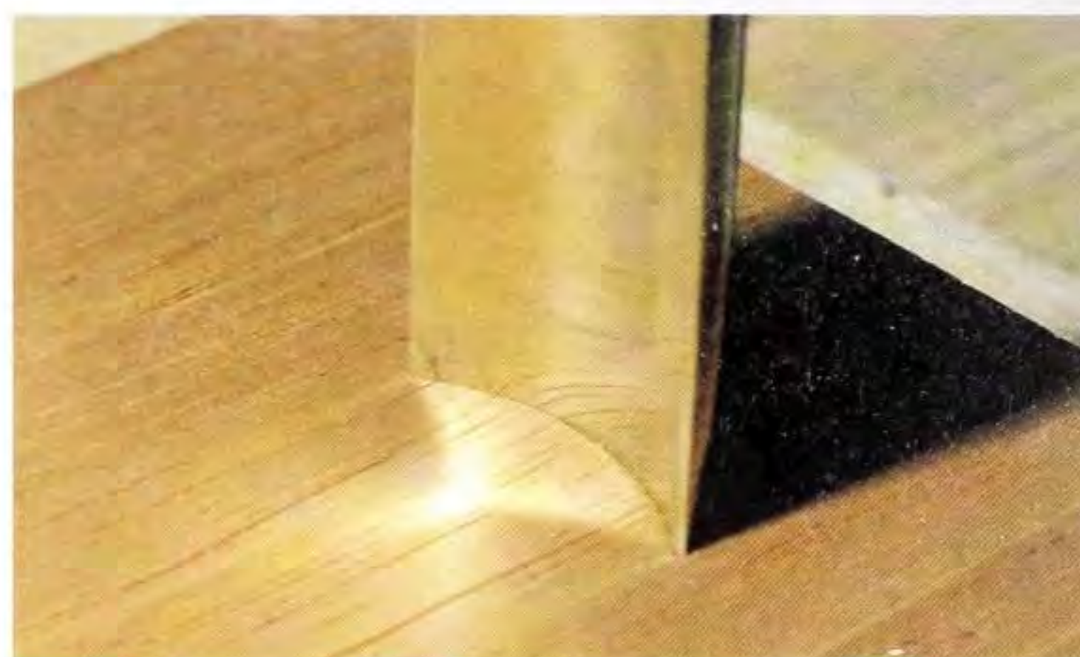
Fig 5.74 Start with a vertical stab cut.
