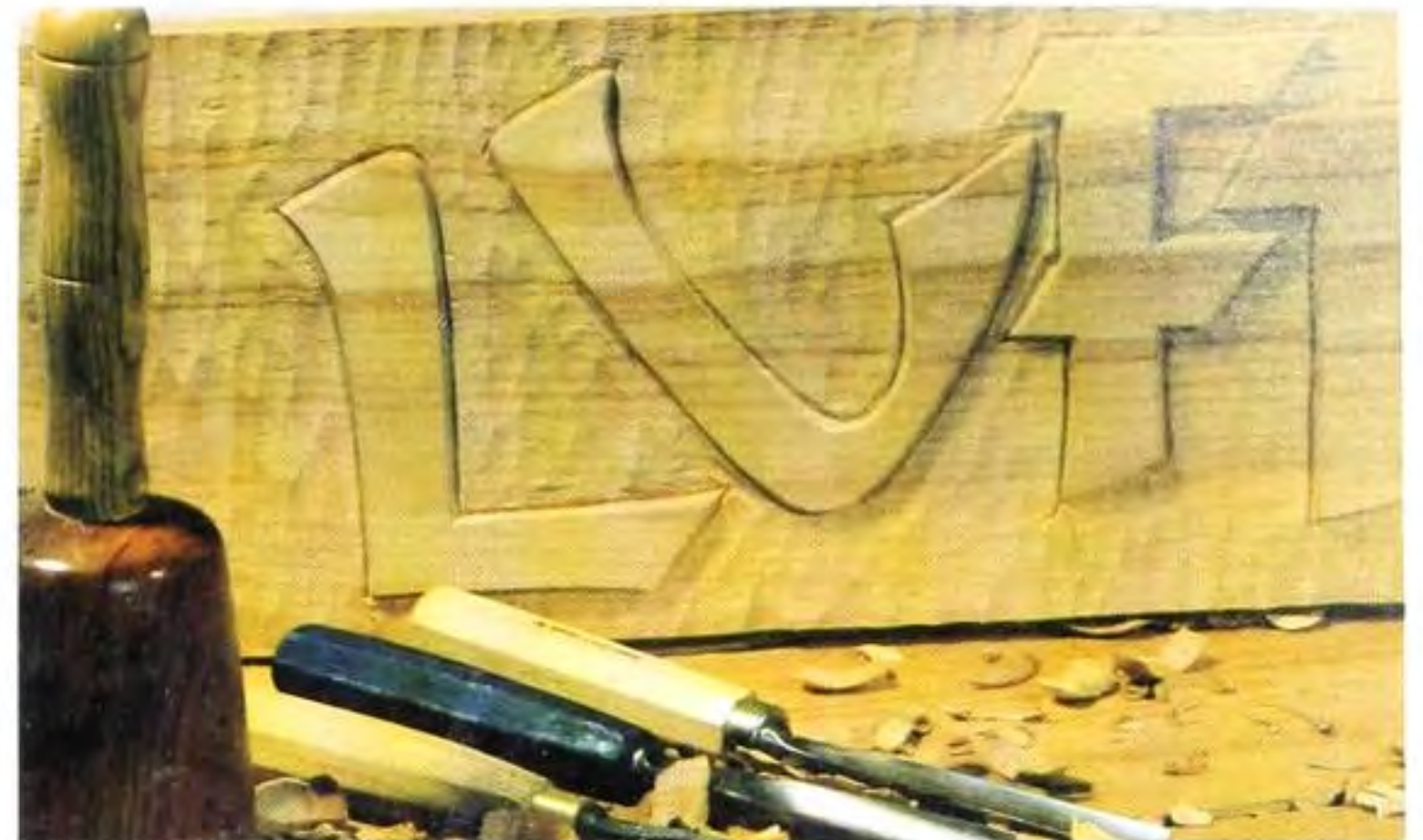
Fig 12.7 Some of the letters, and the tools used to carve them. A groove around the perimeters of the letters made with the V tool helped them to stand out even more against the tooled background.
