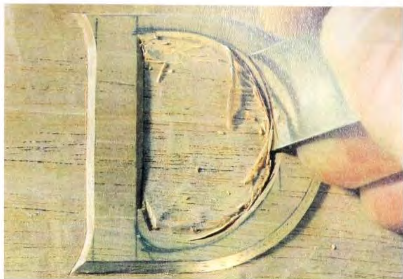
Fig 8.67 Setting the inner curve using the same gouge.
