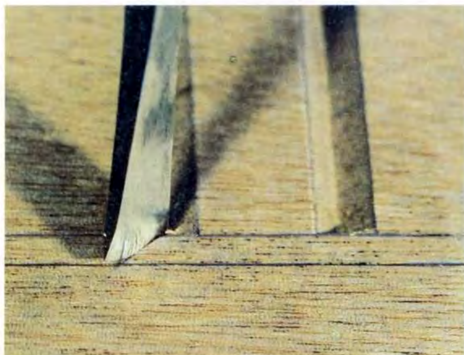
Fig 5.19 Stab the first stop cut with the corner of the fishtail chisel.
