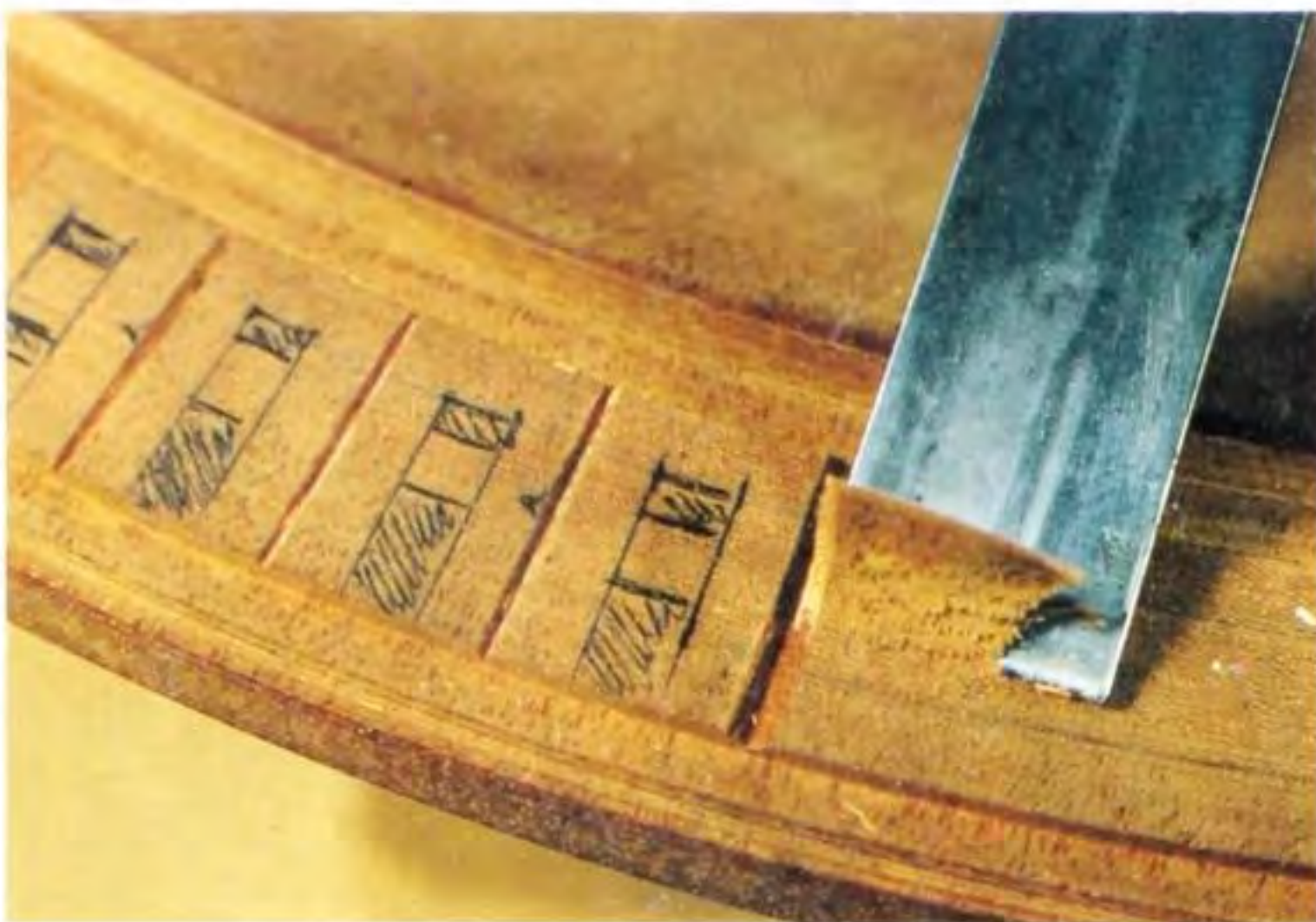
Fig 12.15 Levelling the ground between the words with a flat gouge.
