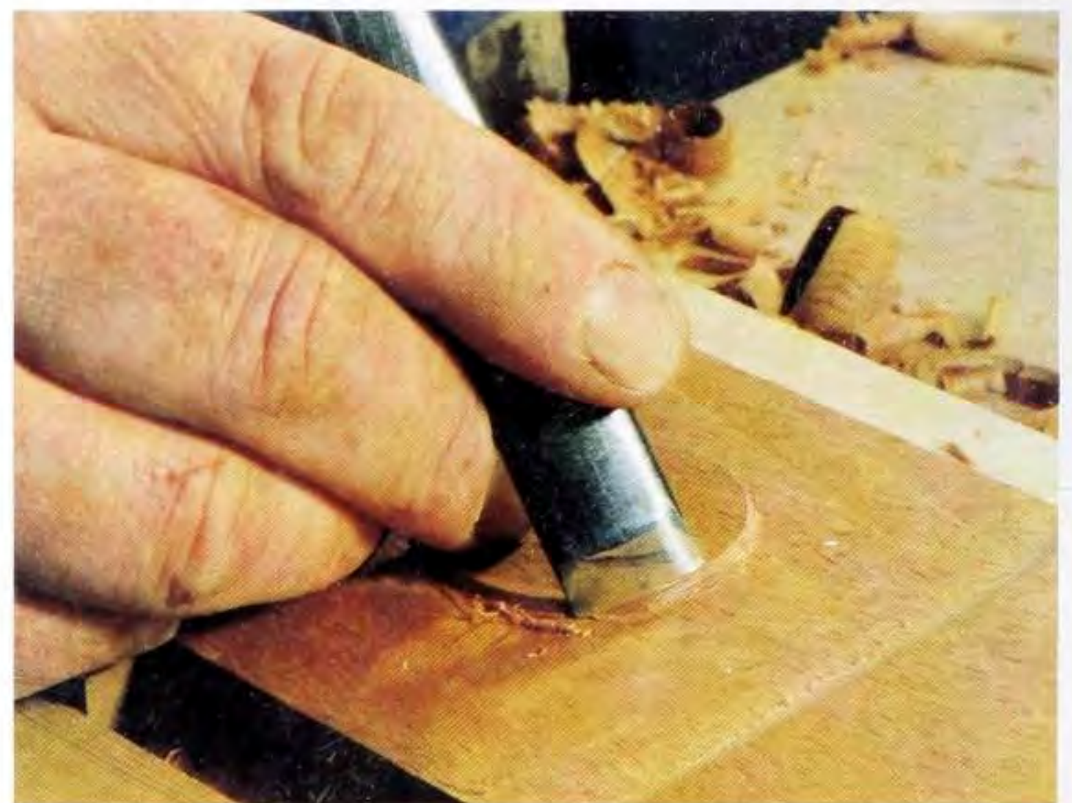
Fig 8.29 Using the corner of the gouge to slice around the circle. You need to pay attention to both the surface edge and the ground junction.
