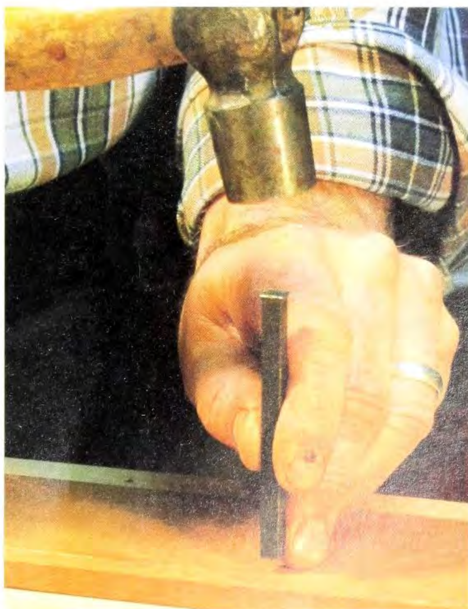
Fig 8.84 The froster poised above the wood surface. Note the supporting finger setting the height.
