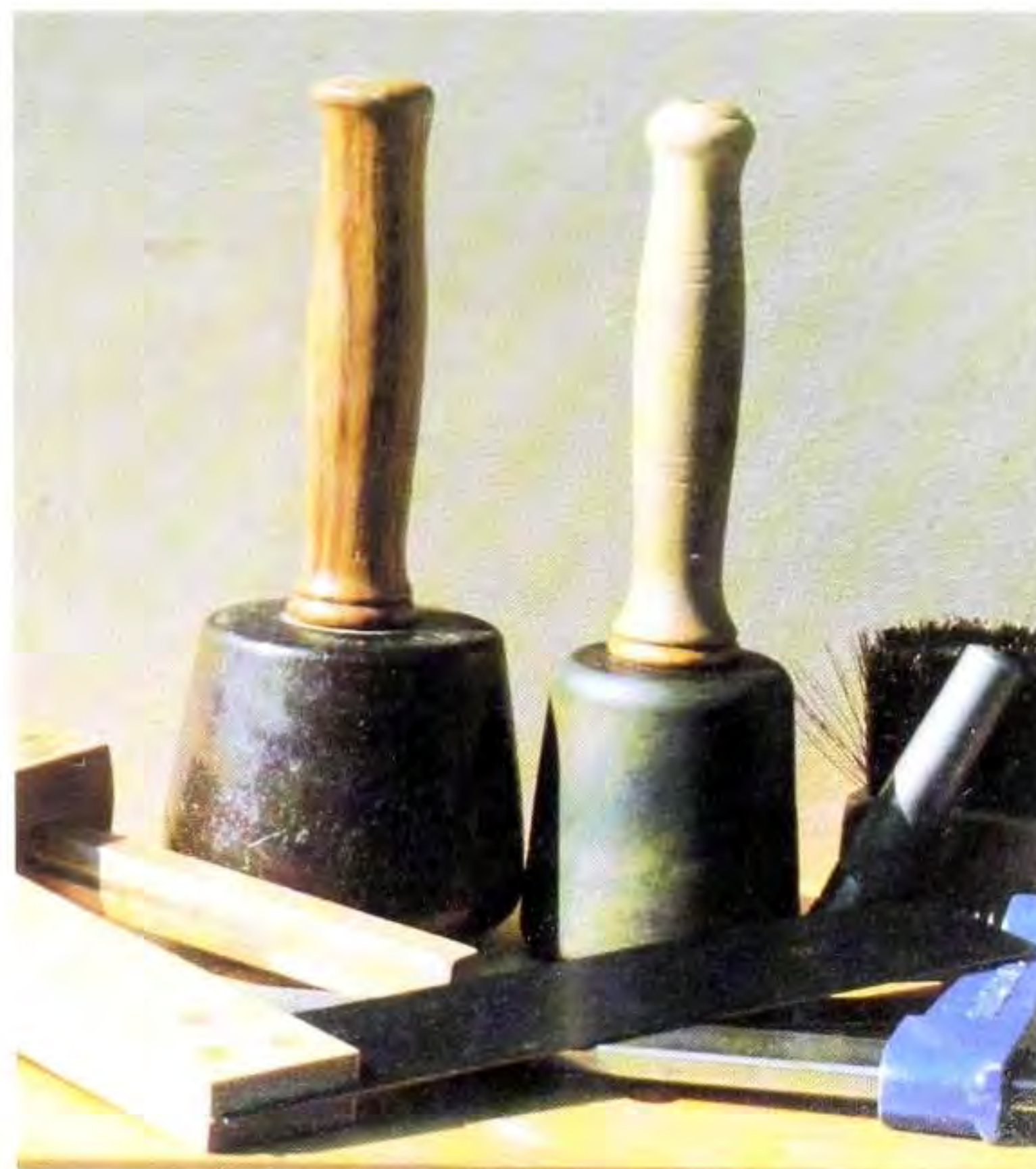
Fig 2.6 General equipment needed for lettercarving: mallets, clamps, a marking gauge and set square, and a stiff brush to keep the carving clean. The mallets shown here are made from lignum vitae. The larger weighs about 1kg (2.2lb), and the smaller 0.5kg (1.1lb).
