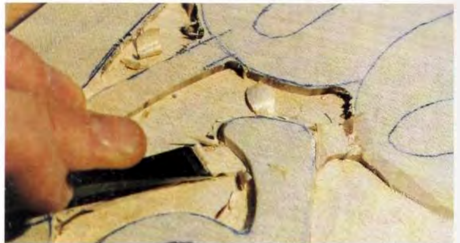
Fig 12.34 Taking down the stalks to the required depth before shaping.
