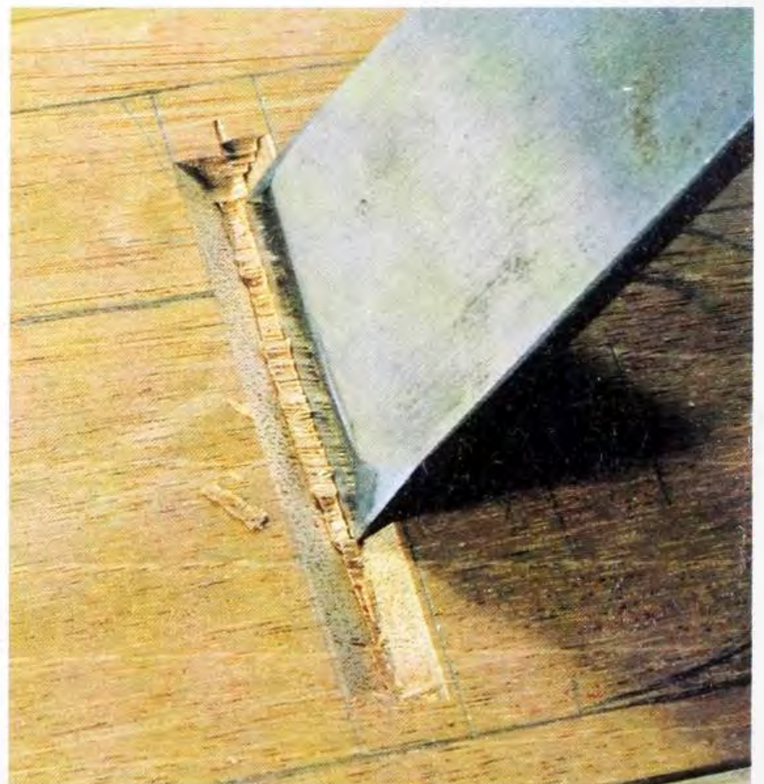
Fig 10.25 Incising the upright trench.
