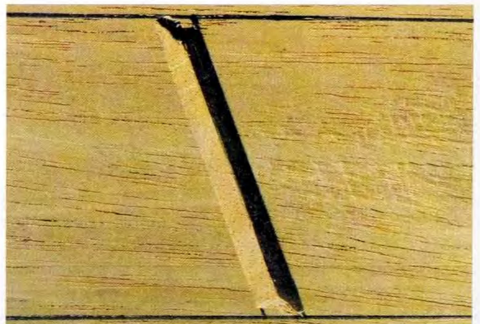
Fig 5.43 An angled trench, ready for serifs.
