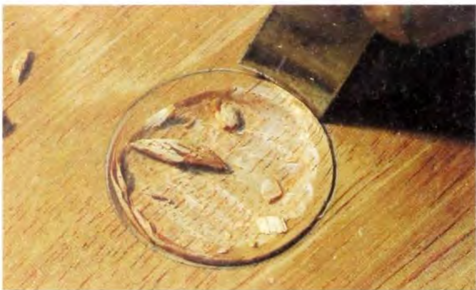
Fig 8.37 Setting in with a slicing cut which winds around the circle at the appropriate angle. You will find that, having removed material in the centre, the remaining waste wood easily pushes over and crumbles.
