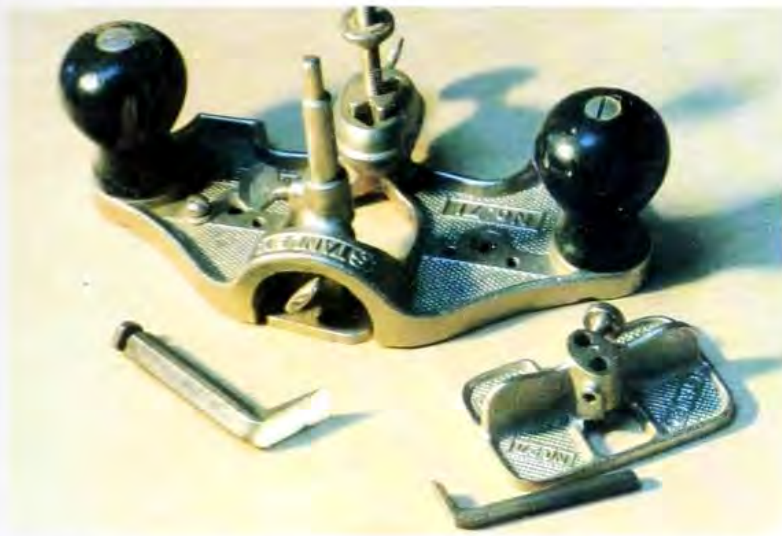
Fig 7.20 Two types of hand router, designed for housing and other woodworking joints.
