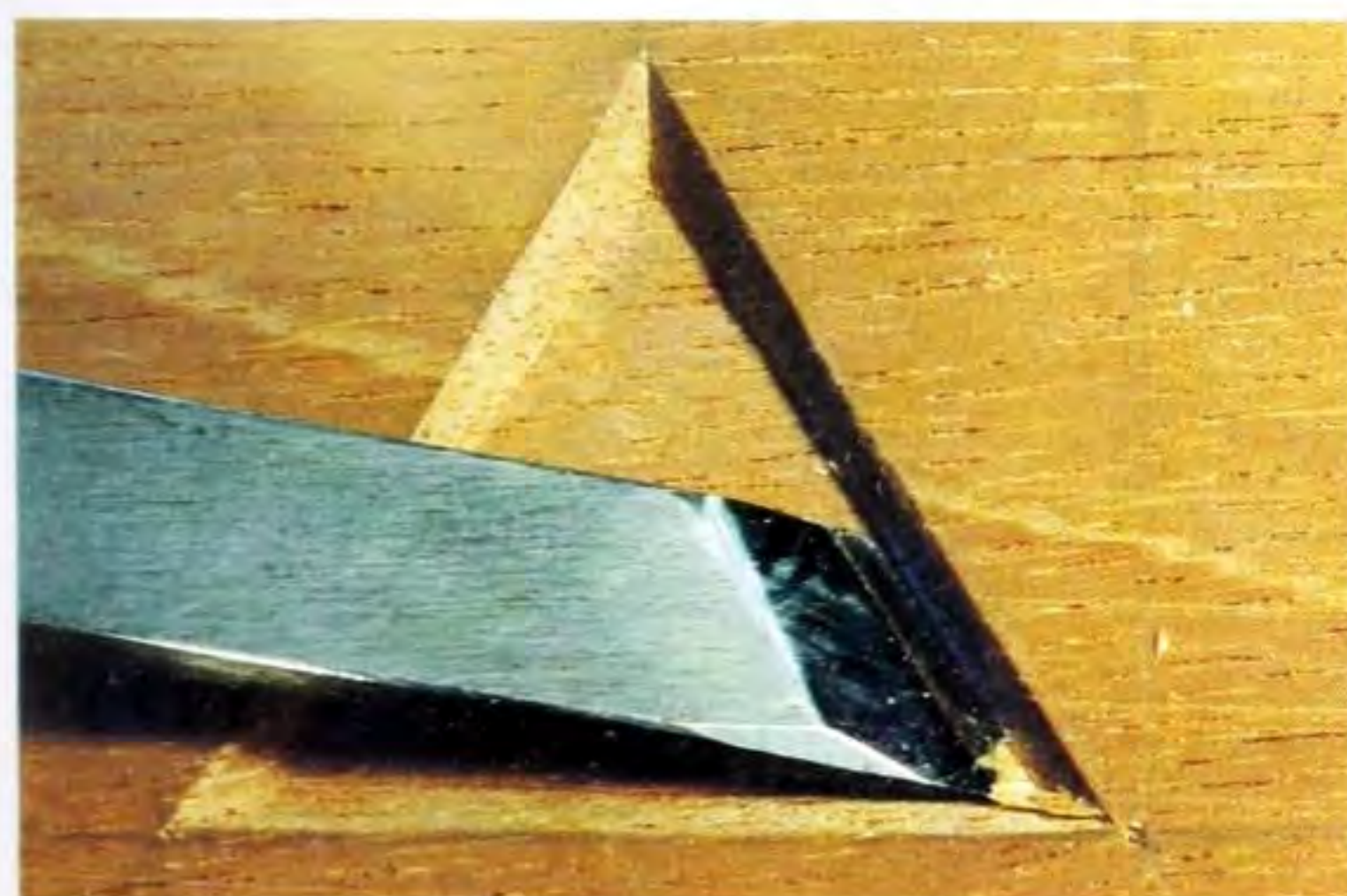
Fig 8.42 This is where a skew chisel comes into its own.
