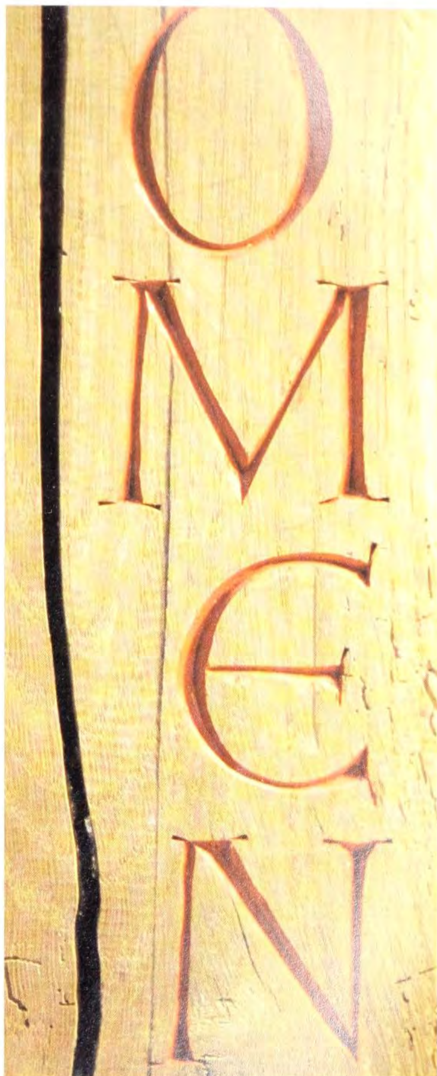
Fig 11.6 The incised lettering after painting but before oiling.
