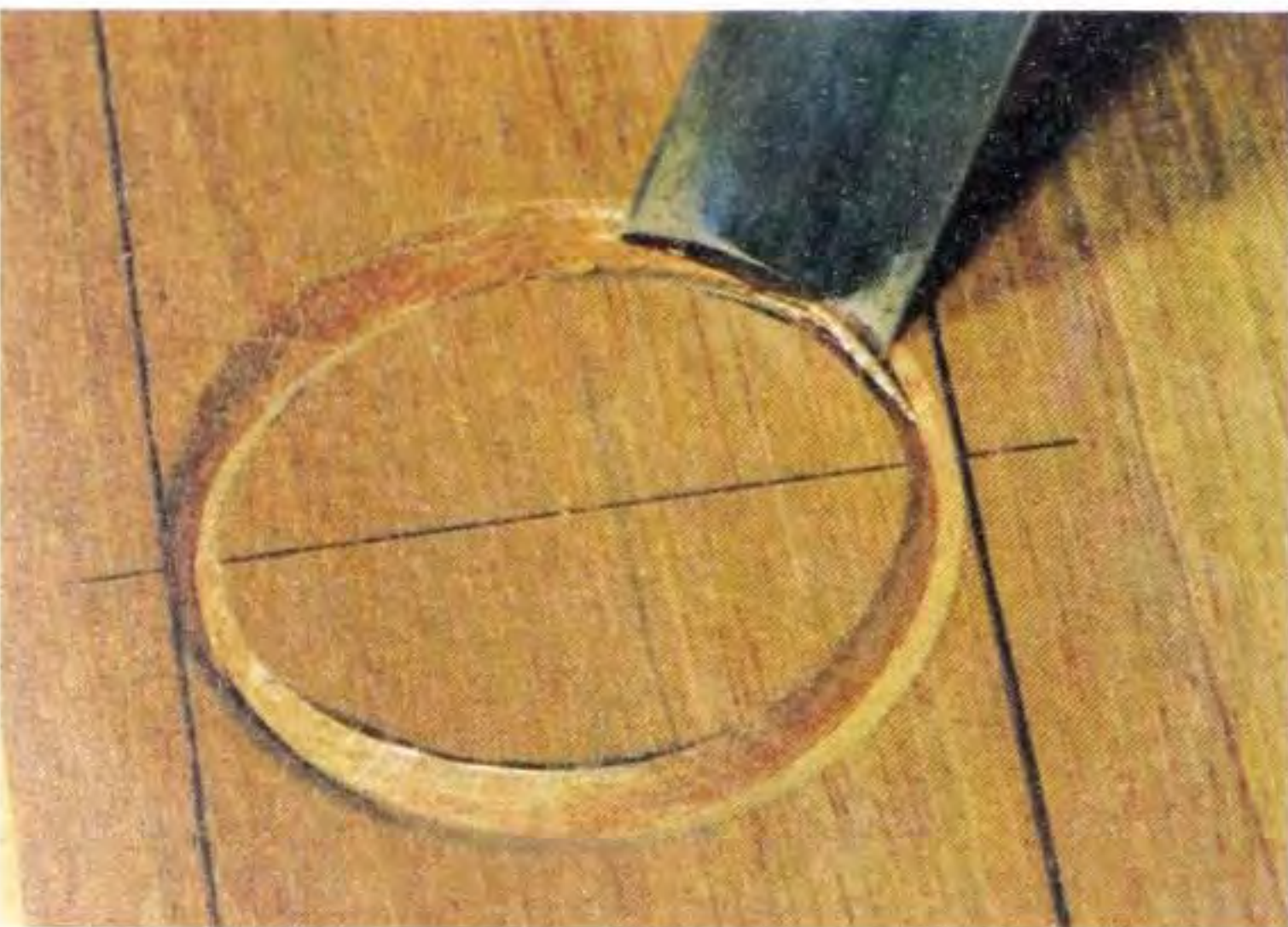
Fig 5.95 Clean up the outside wall down to the root. You may have to work on the inner walls as well at this stage.
