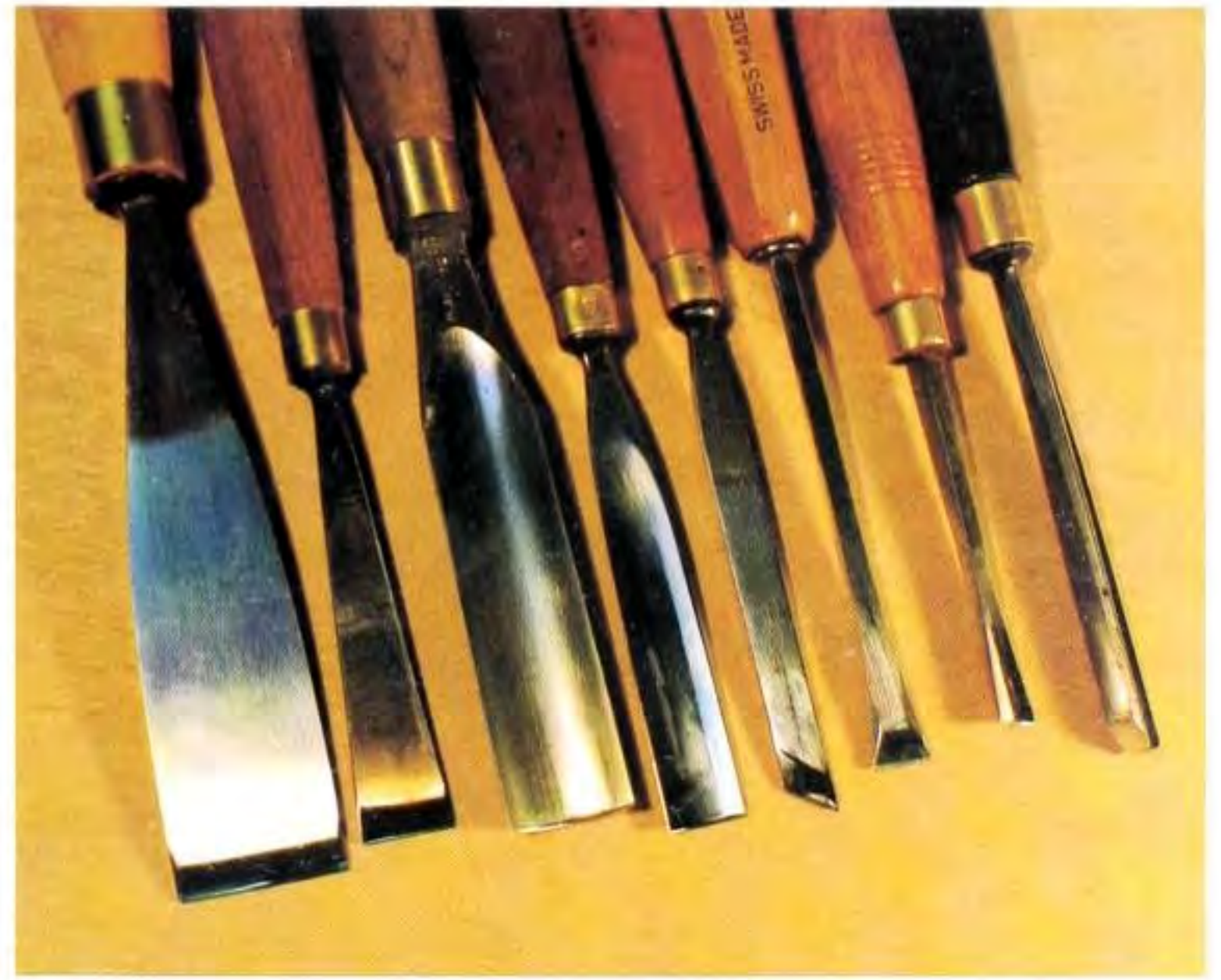
Fig 2.1 A simple range of carving tools used for lettercarving. From left: regular chisel; alongee chisel; deep gouge; flatter gouge; skew chisel; fishtail chisel; fishtail gouge; V tool.
