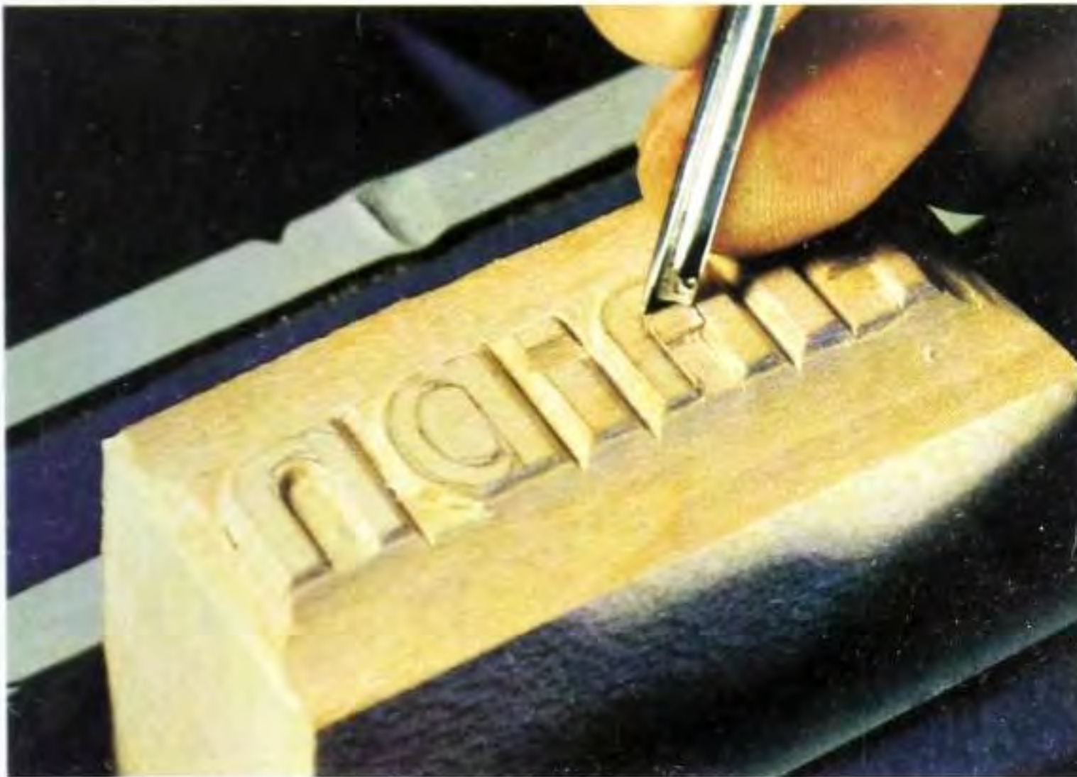
Fig 12.26 Finishing off the rounded counters using a small gouge.
