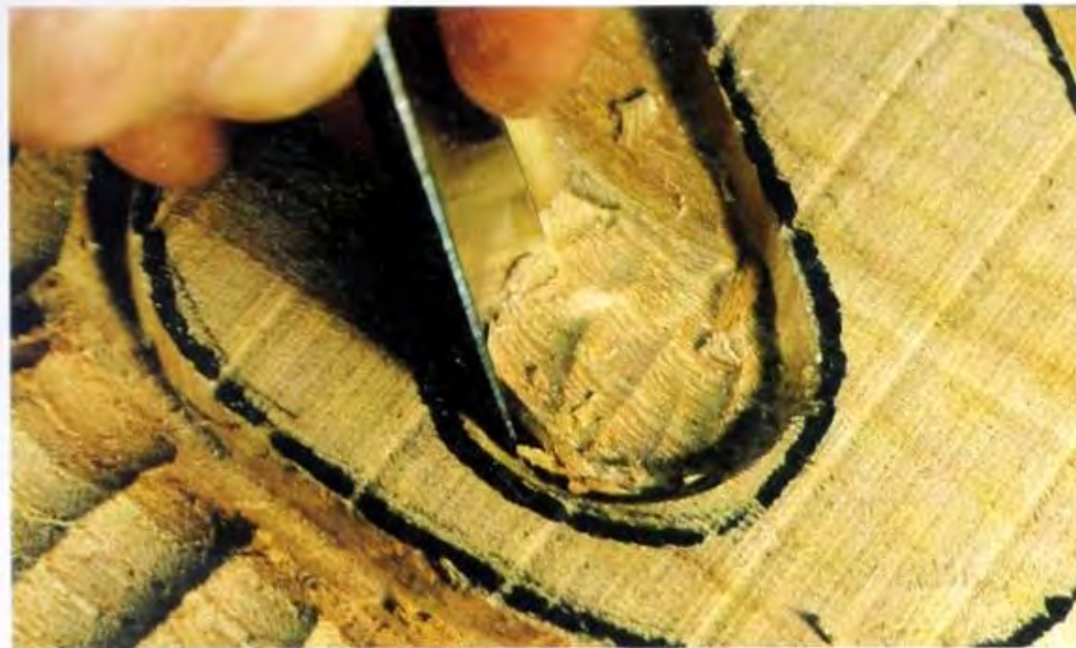
Fig 12.6 Setting in the more tightly-curved walls (those which caused the V tool to snatch) with a slightly shallower gouge than that used to lower the ground.
