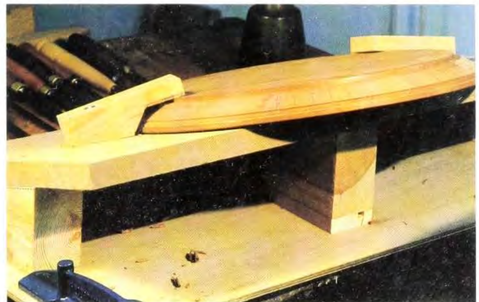
Fig 12.13 The method I devised to hold the board. The nibs can be quickly loosened with a screwdriver to re-position the workpiece.
