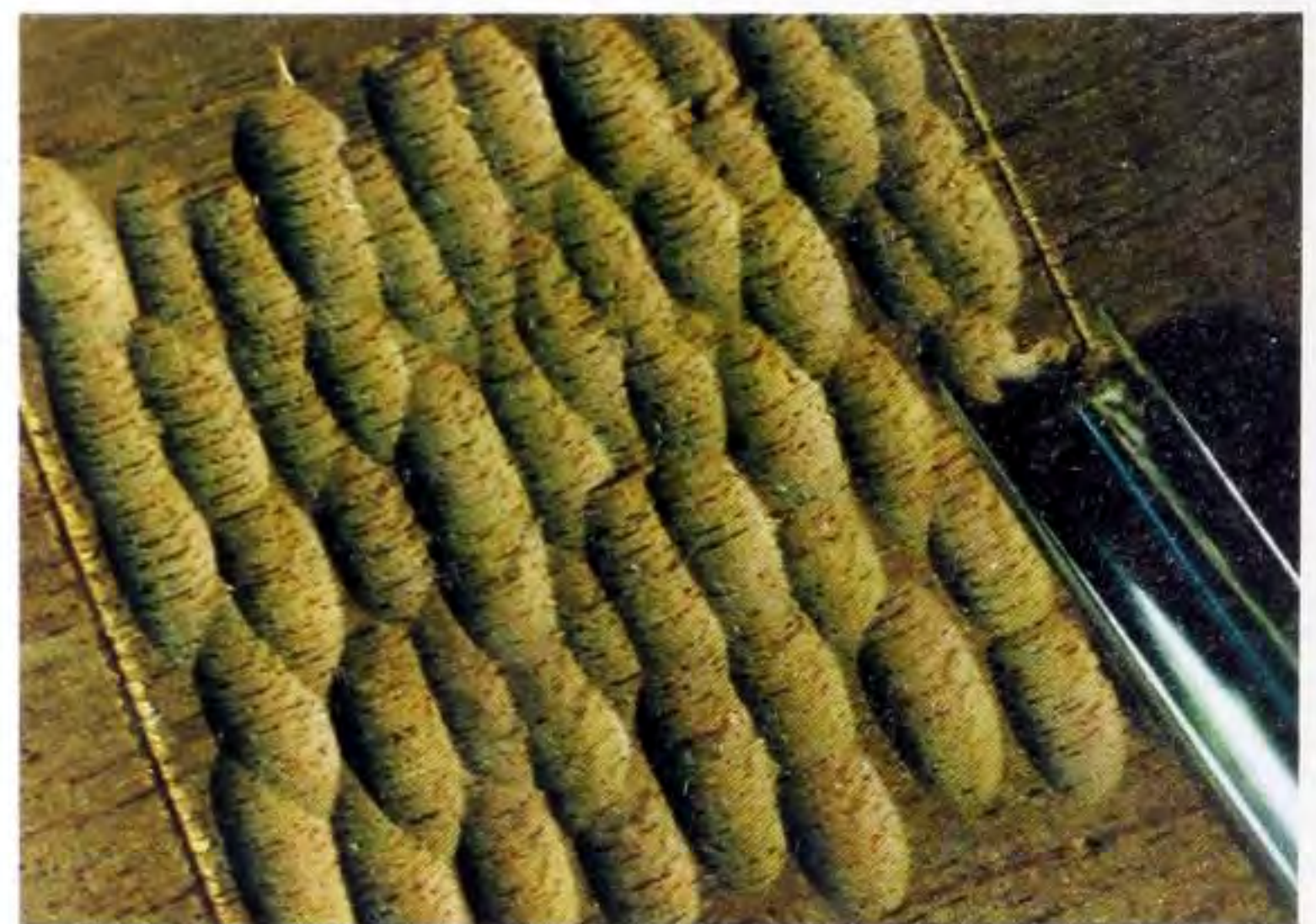
Fig 8.82 Texturing the ground using a deep gouge. The facets are best placed irregularly, or like scales, rather than in rigid lines. Depending on the wood, the crests between cuts can tend to crumble, so care is needed here.
