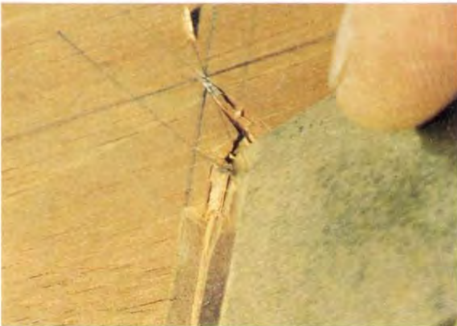
Fig 5.55 The third angled cut slices down to the root of the left oblique, again beyond the weak area, safely isolating it.
