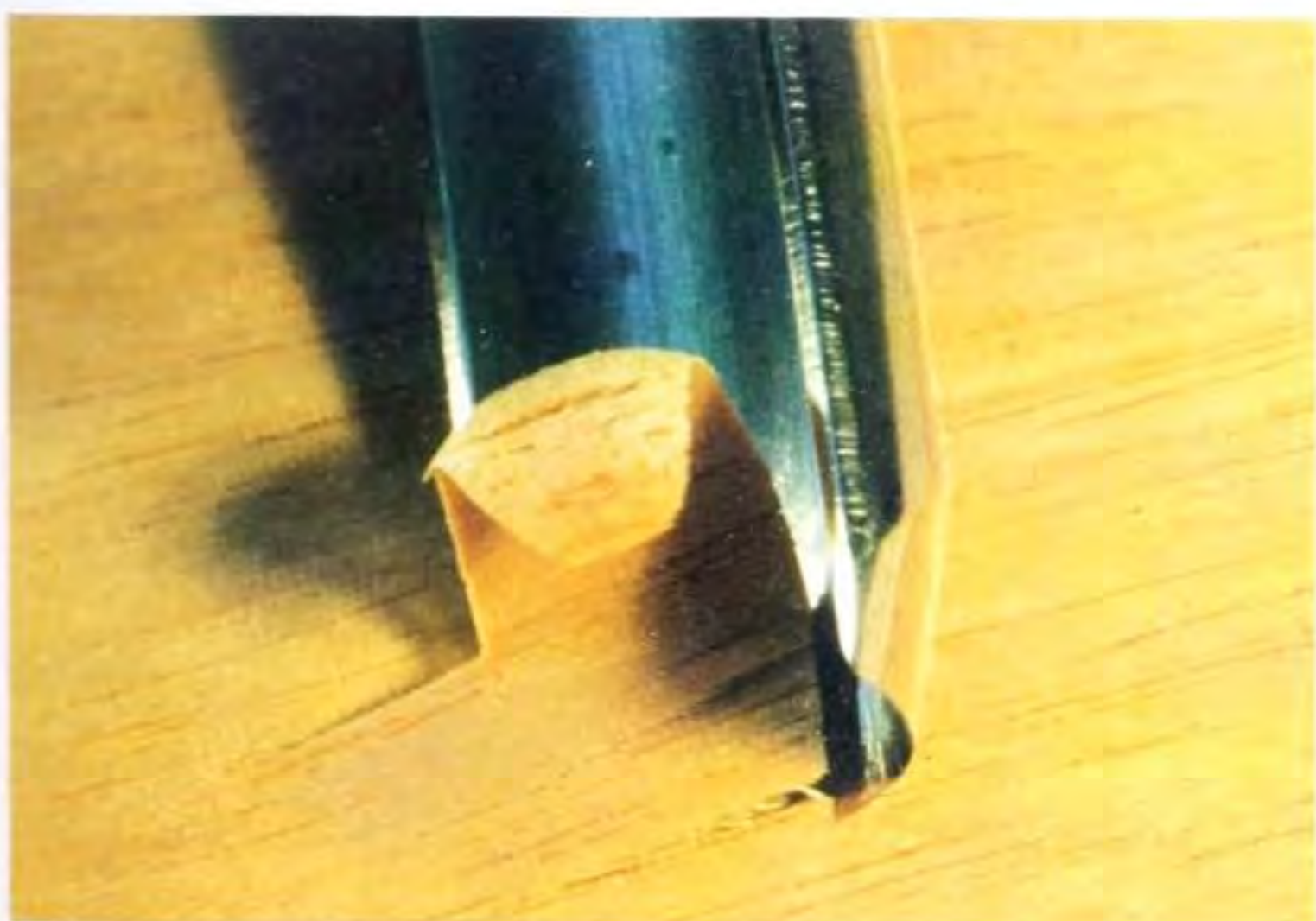
Fig 8.9 If you allow the corner of the gouge to go below the surface of the wood, it will tear the fibres.
