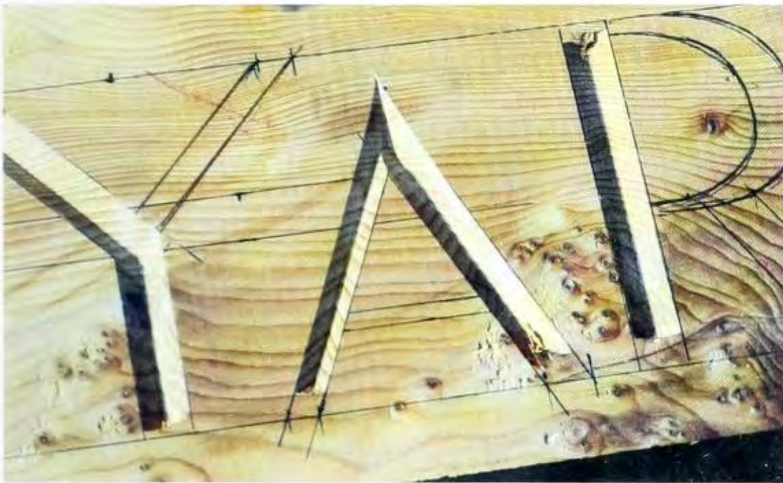
Fig 11.10 I used the techniques described in Chapter 5 to carve the letters. The straight elements were cut first, using the same chisel for as long as possible. Because of the size of the letters, I needed to cut the uprights in carefully merged sections.
