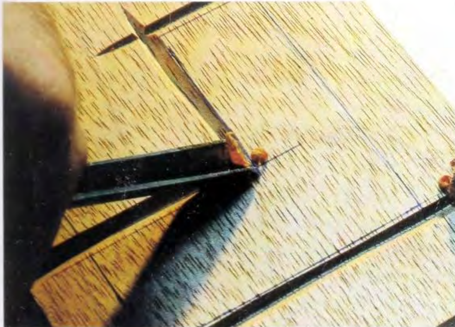
Fig 8.31 Lining in the fat L shape, running into the angle.
