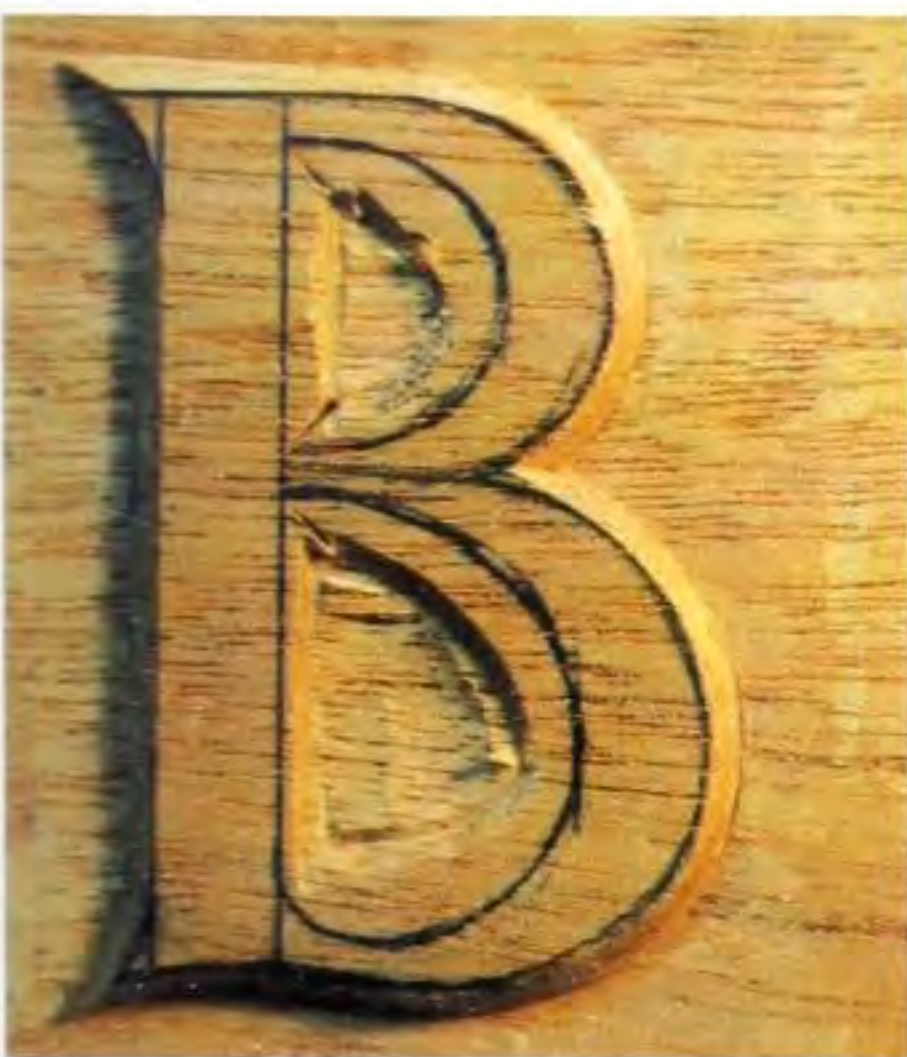
Fig 8.73 After levelling and setting in the outer curves, a stop cut is needed at the junction of the lobes, and you can see this clearly here.
