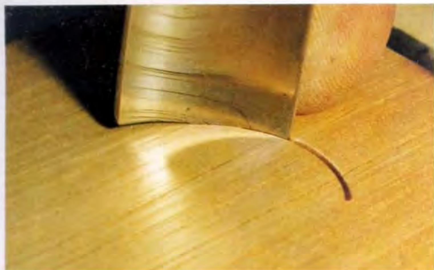
Fig 5.76 Push the gouge along, allowing the initial stab cut to guide the travel of the blade.
