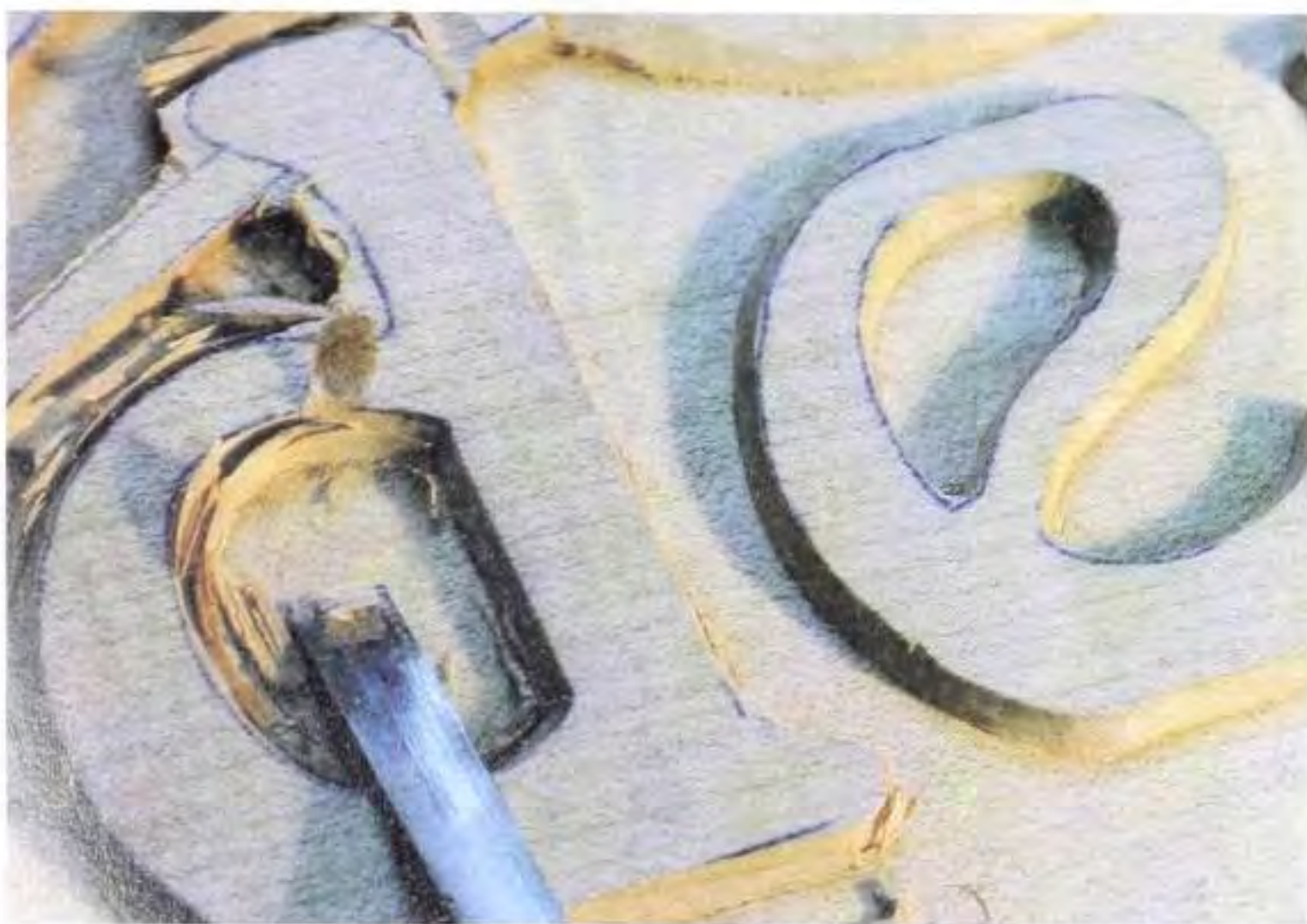
Fig 12.33 Levelling the closed counters. Cutting clean profiles is very important, even if you are not cutting exactly to the pencil line.
