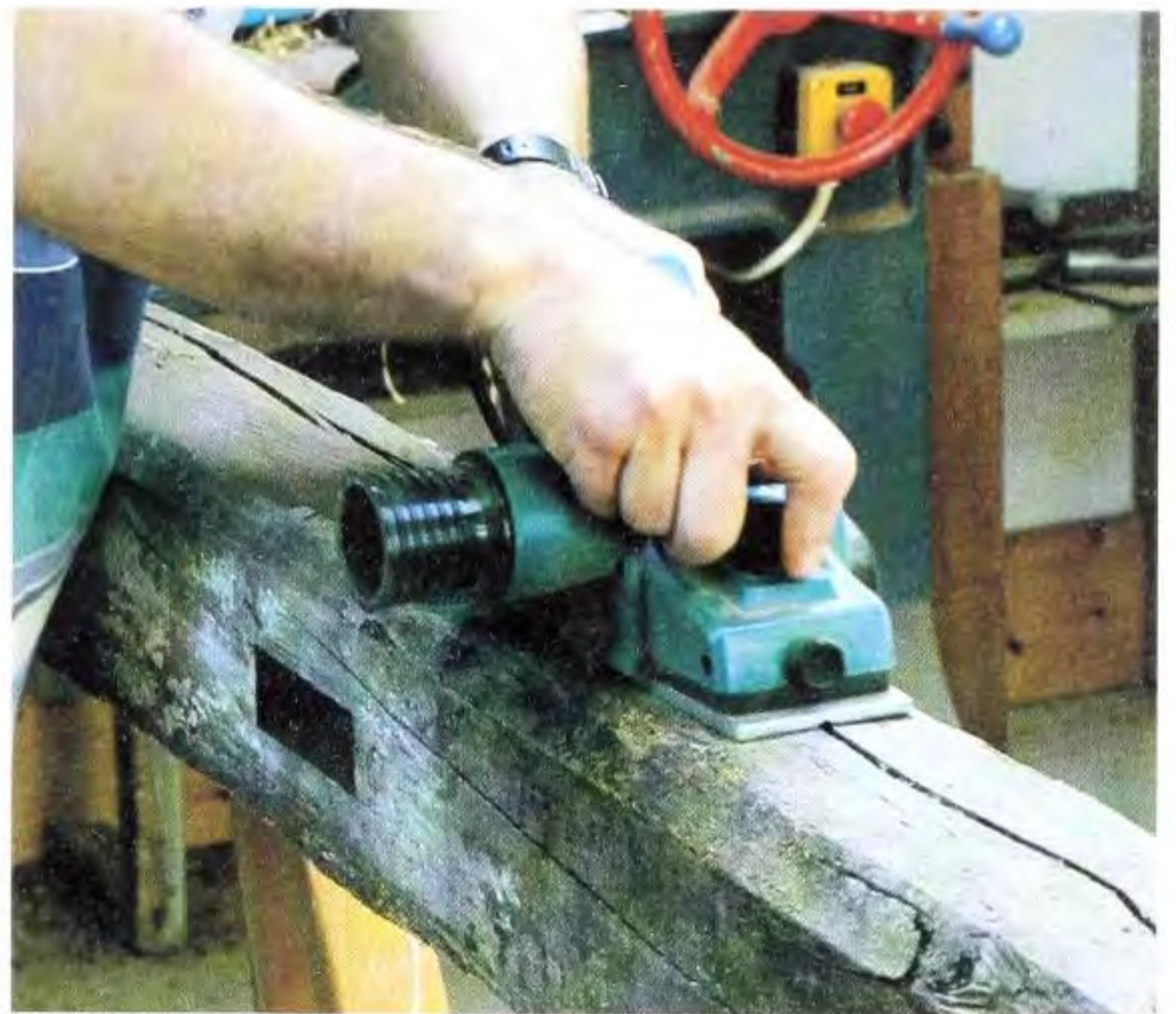
Fig 11.2 Cleaning up the wood to protect the carving tools and find out what surfaces are available to work with.
