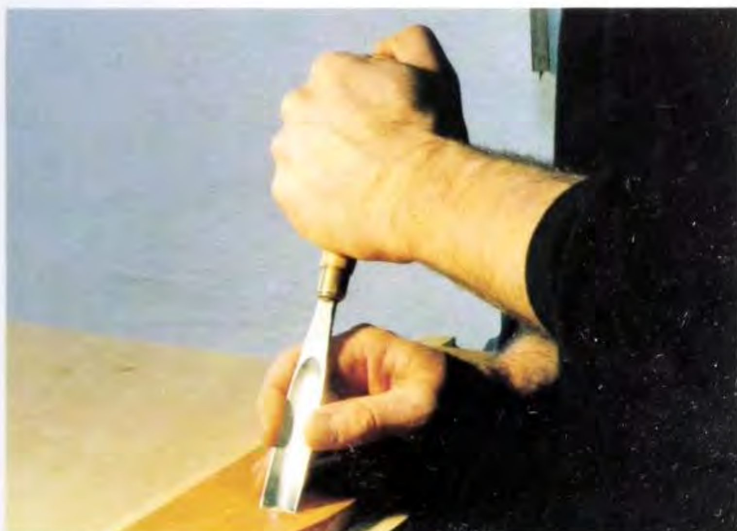
Fig 5.83 The angled cut cannot meet both the centre root of the crescent and the corners at the same time, so waste is left in the middle, which will have to be cleaned up by hand.
