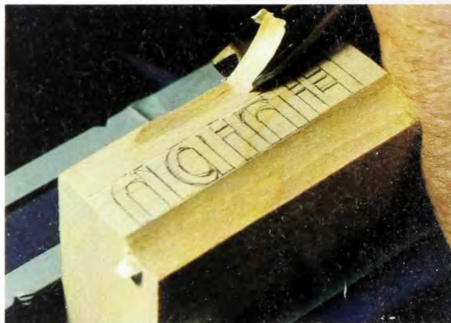
Fig 12.23 Lowering the ground around the word as a whole.
