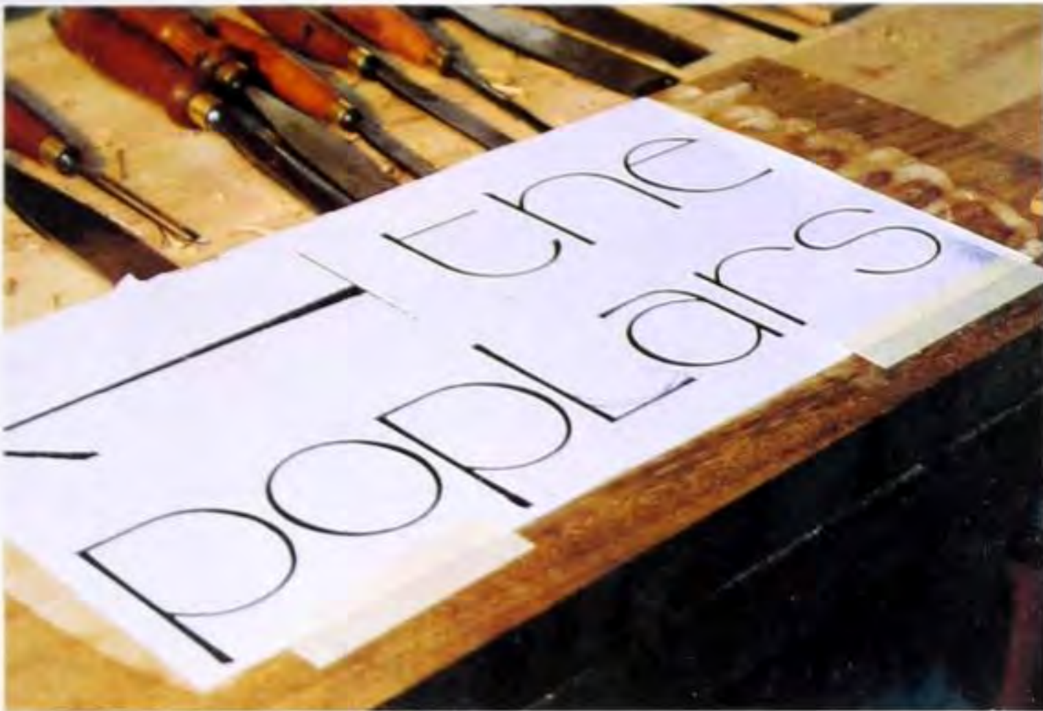
Fig 11.31 The paper layout of the transfer letters, glued to the wood with thinned PVA wood glue.
