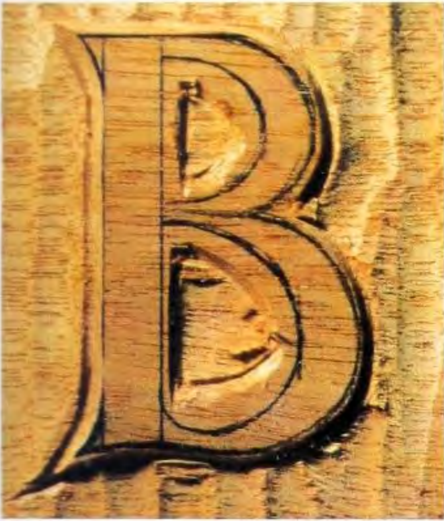
Fig 8.72 The ground lowered around the letter and inner counter.
