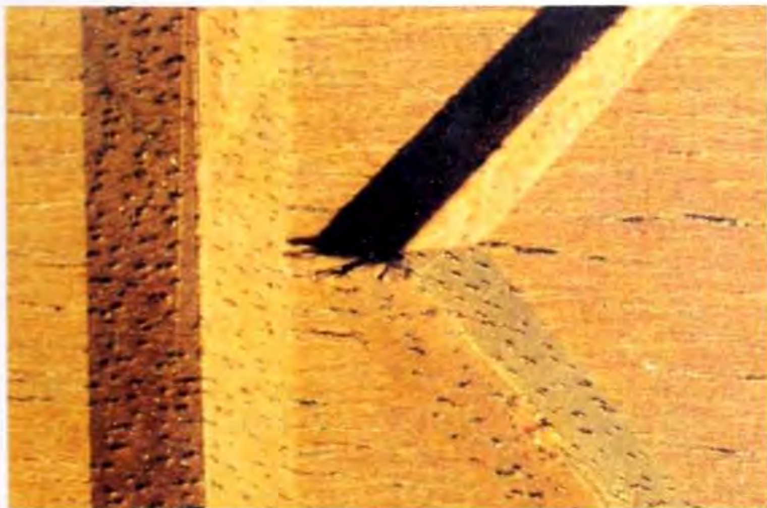
Fig 5.67 Close-up of the junction of K. It is vital that the apex does not invade the upright by breaking through the short grain.
