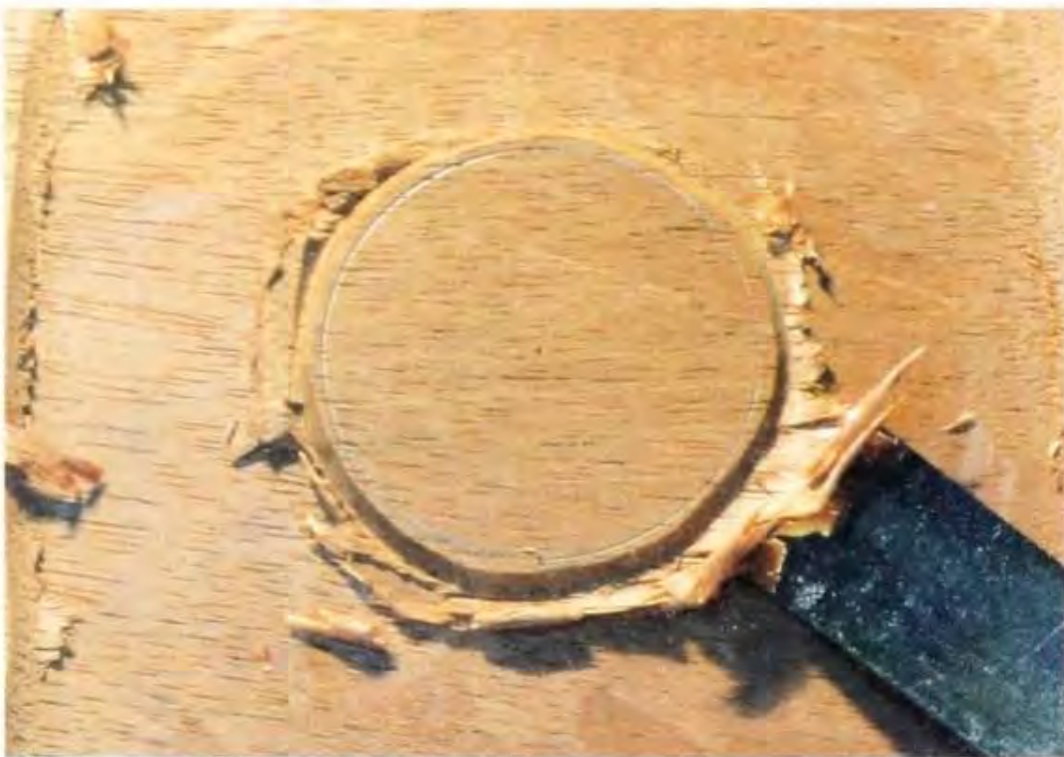
Fig 8.25 Levelling up to the circle. In this case a second light cut with the V tool to firm up the line and the junction is now required.
