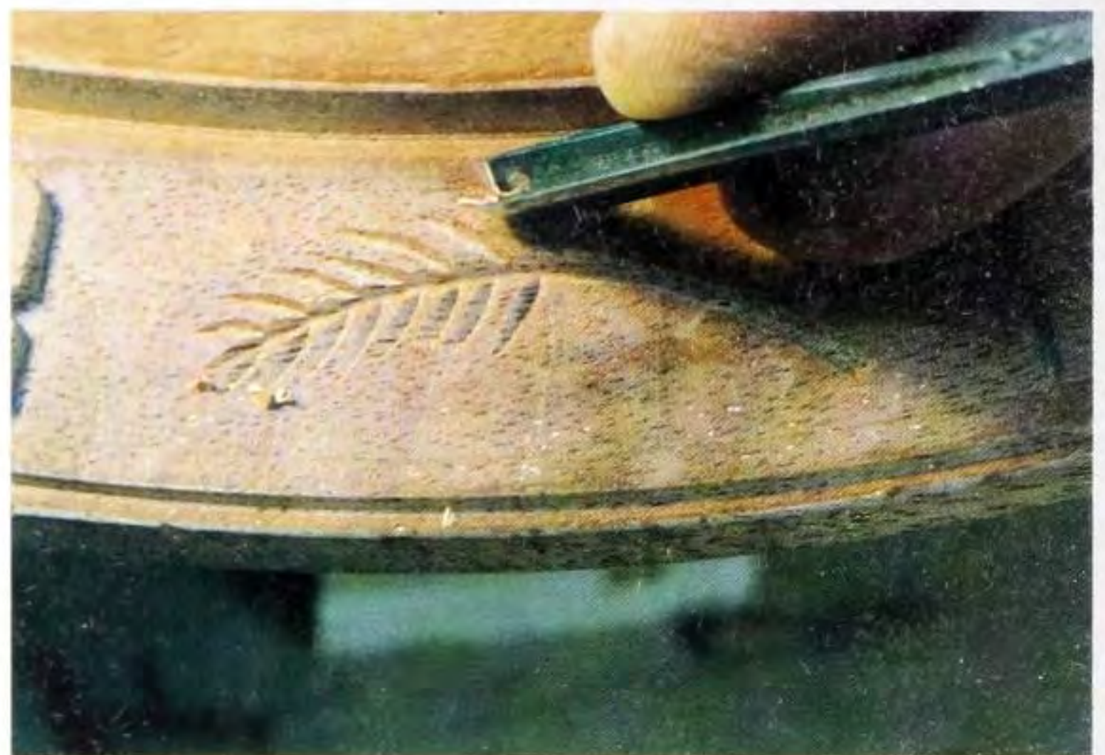
Fig 12.18 Carving the wheat-ear pattern between the words using a V tool.
