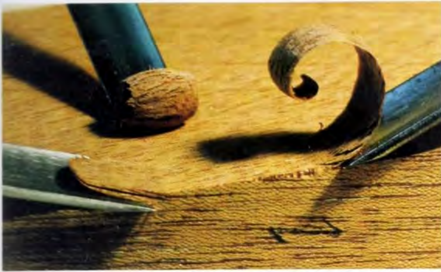
Fig 8.2 Working with the grain. On the left you can see how the grain tears as the edge cuts against it; on the right you can see a shaving rising smoothly as a result of cutting with the grain. Working across the grain (centre), is the most straightforward option for roughing out or lowering the background.
