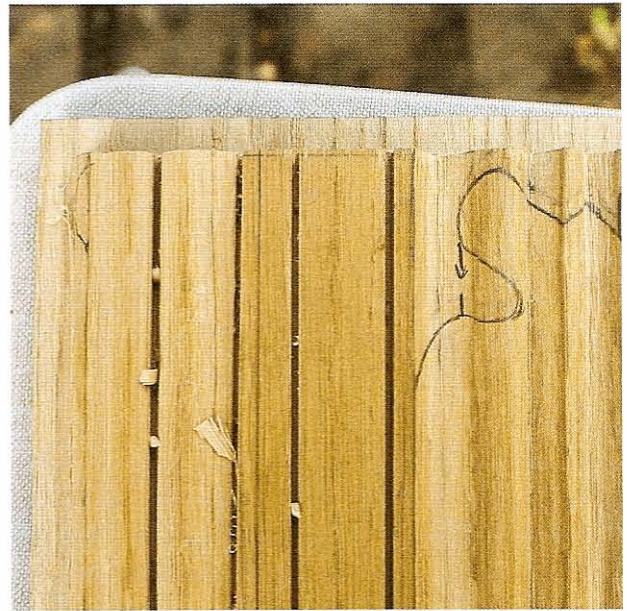
FIG 7.9 The pattern of the end drawn on to one side of a panel. It is a waste of time to draw it on the left side which still needs to be planed.
