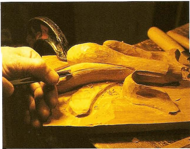
FIG 8.13 Marking a groove with a V chisel.
