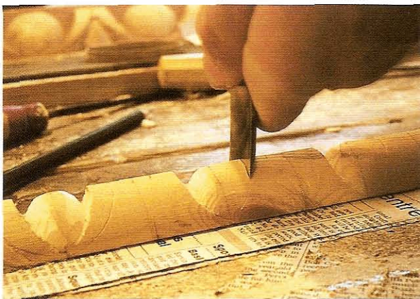
FIG 4.8 The first cut on egg and dart. The gouge cuts vertically on to the outline from the back edge.
