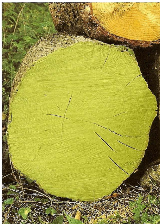
FIG 2.14 A piece of ash painted immediately after felling. Note the star shake around the pith and the other radial shakes that the sealing of the end could not prevent.
