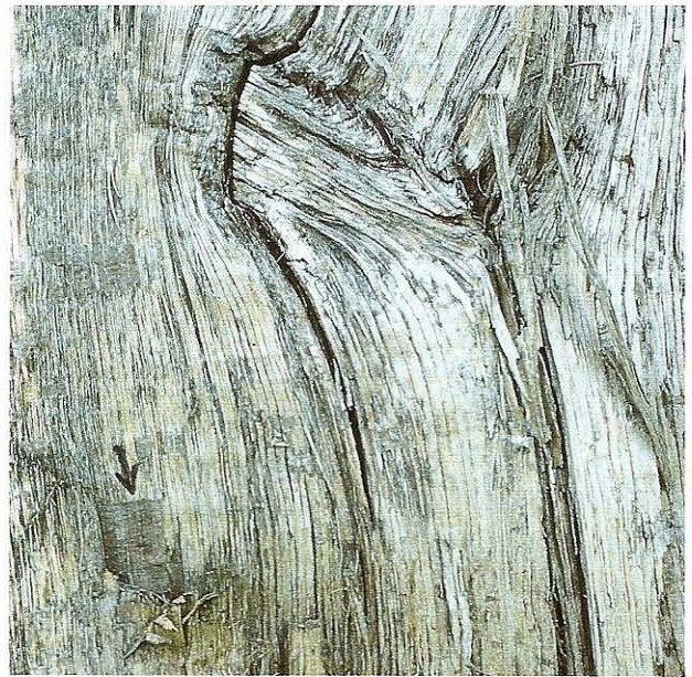
FIG 2.6 A riven section of an oak tree. The pith is the dark fissure running down the right side. The grain around the knot is typically disturbed. This branch was cut off some years before the tree was felled and the wood has grown around it. The outside of the log shows no sign of the dead knot within. The arrow (lower left) indicates a ray.
