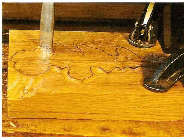
FIG 5.4 Stabbing down just outside the outline with a gouge which approximates to the shape. Be careful to prevent splits running from the corner of the chisel into the design.
