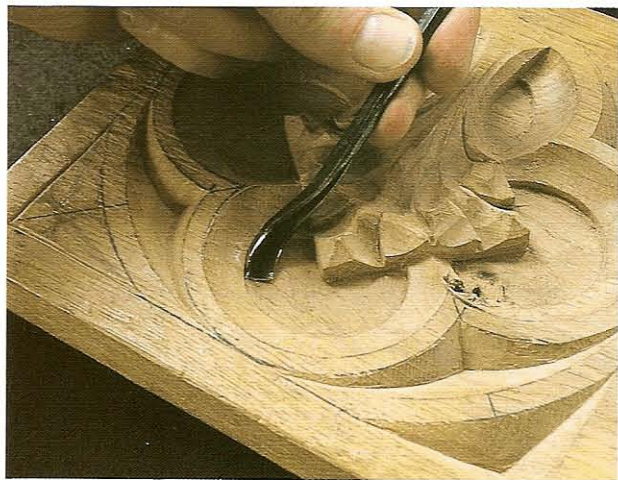
FIG 1.14 Bent V chisel used to clean out the join between side and ground on an inside curve.
