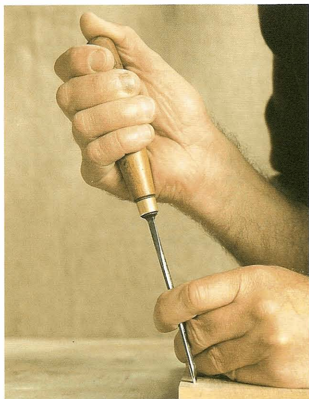
FIG 3.2 The first, stabbing, cut showing the angle of the blade, with the flute facing slightly downwards, and the positions of the hands.
