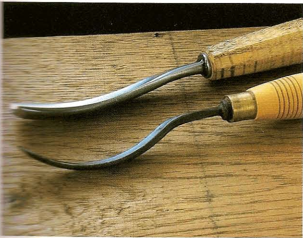
FIG 1.15 Two long bent gouges. The nearer one is heavily shaped and flexes at the neck, and is difficult to use.
