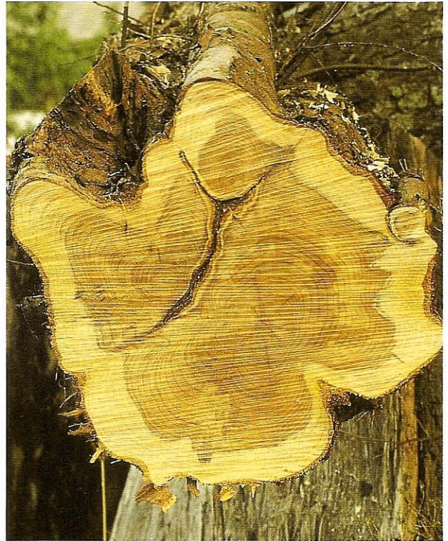
FIG 2.12 The cut end of a small yew tree. The dark area is heartwood; the light band is sapwood. The Y-shaped fissure is where the buttresses have begun to separate into three stems and is lined with bark. Had the tree continued growing for many years this fault would have been unpredictable from the outside of the tree.
