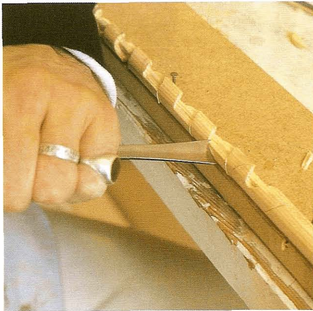
FIG 4.16 The edge of the ribbon at the near side of the interval has been stabbed in down to the ground. The side of the stick has been stabbed down. Now the No. 7 gouge picks up the line on top of the ribbon at the far side of the interval and is stabbed in towards the side of the stick. The chisel should slope downwards when making this cut. It is slid around to stop against the back of the next twist of the ribbon.
