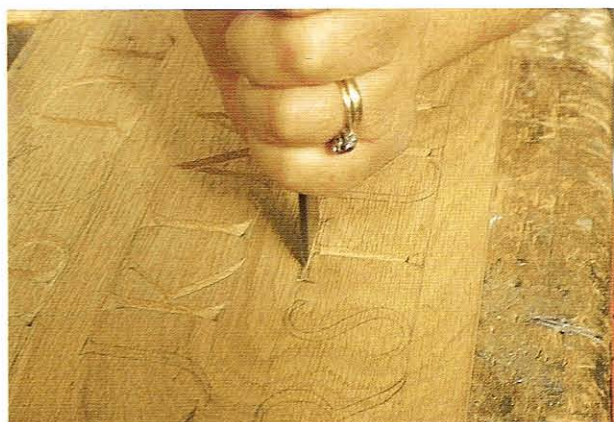
FIG 15.24 Stabbing the centre line of the arm of a T.
