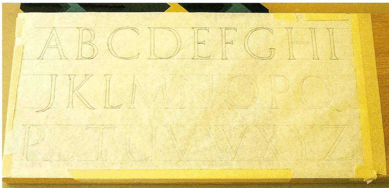
FIG 15.7 Alphabet drawn by Janet Monks being transferred to an oak board with the aid of carbon paper.
