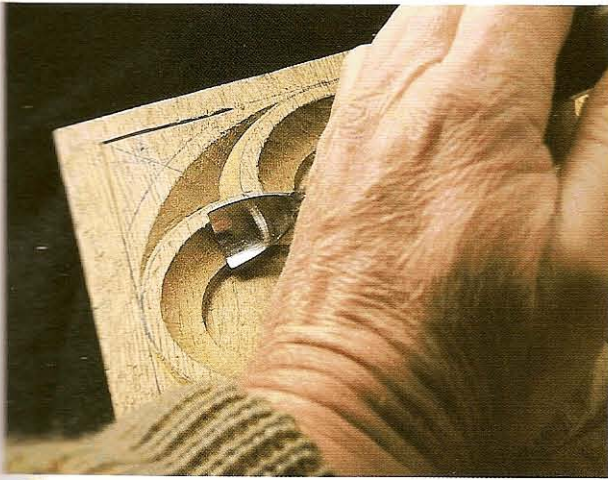
FIG 1.13 Large spoon bit used to shape a concave inside curve.
