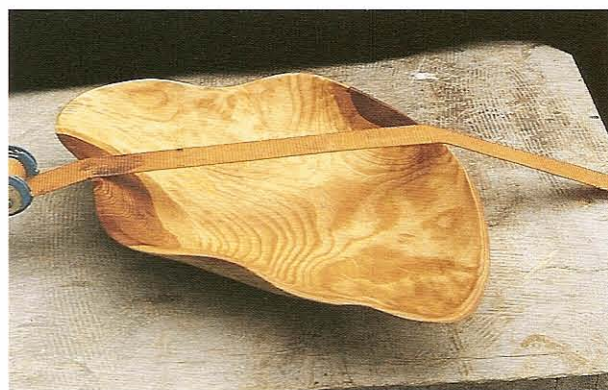
FIG 10.13 Bowl in Scots pine held by a webbing clamp (Dick Onians). The shape was dictated by the odd shape of the piece.
