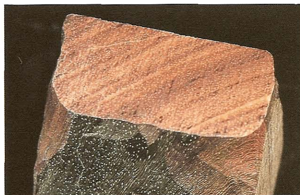
FIG 2.23 Padauk freshly cut across the end grain, but with varying degrees of brown where it has been exposed for different periods.
