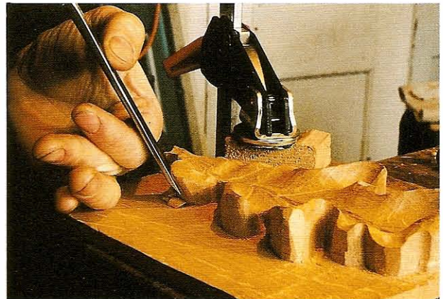
FIG 5.12 Beginning the undercutting. Note the angle of the gouge and how it fits the curve of the edge of the leaf.
