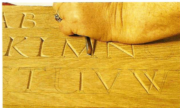
FIG 15.16 The first cut into the serif on an M.
