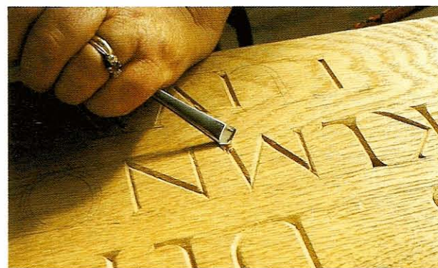
FIG 15.20 The end of the chip cut with the edge of the gouge rocked into the opposite corner.
