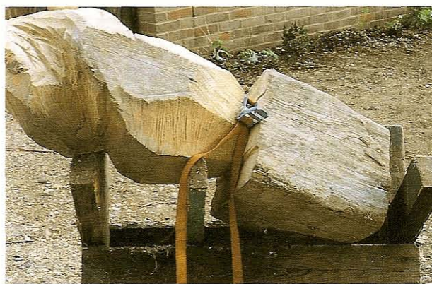
FIG 1.27 A webbing clamp holding an awkward piece on a saw horse.
