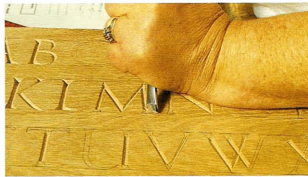
FIG 15.18 The fishtail cutting the right foot serif.
