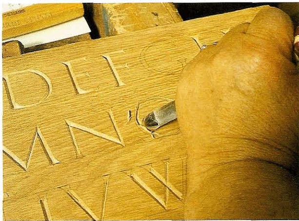
FIG 15.14 A round-ended No. 3 gouge stabbing in the outward facing curve of the counter of an O.
