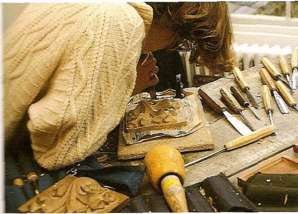
FIG 1.20 A student standing at a carving bench with the elbow level with the top. The body is leaning to exert weight on the chisel. The carving is held on scrap wood by a paper join and the block is clamped on the bench.
