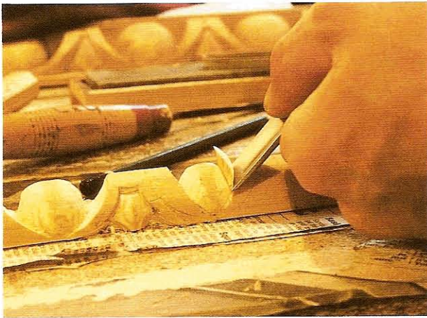
FIG 4.10 Cutting the cup. The gouge enters the wood vertically and the handle is dropped as the chisel goes down. This scooping cut gives a concave cup.
