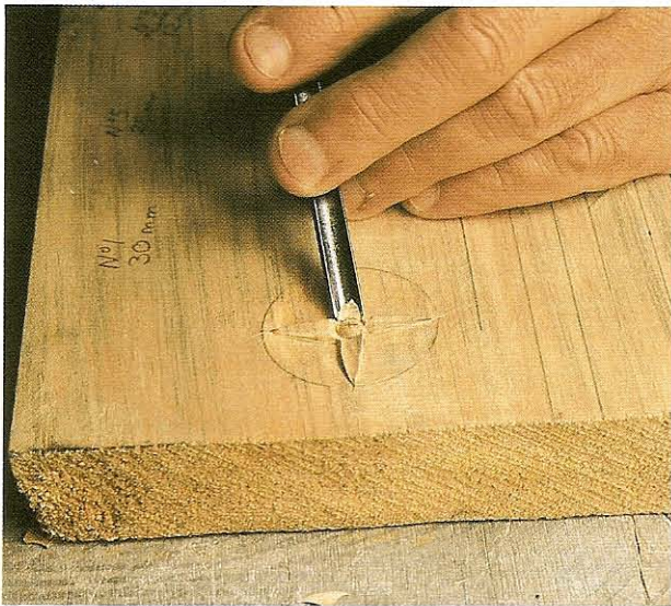
FIG 3.16 The boss has been domed and grooves are cut along the petals. The tool dips more steeply as it approaches the boss to give a good effect. Cutting the grooves like this across the grain can cause problems. The grooves could be made before the petals are stabbed in.
