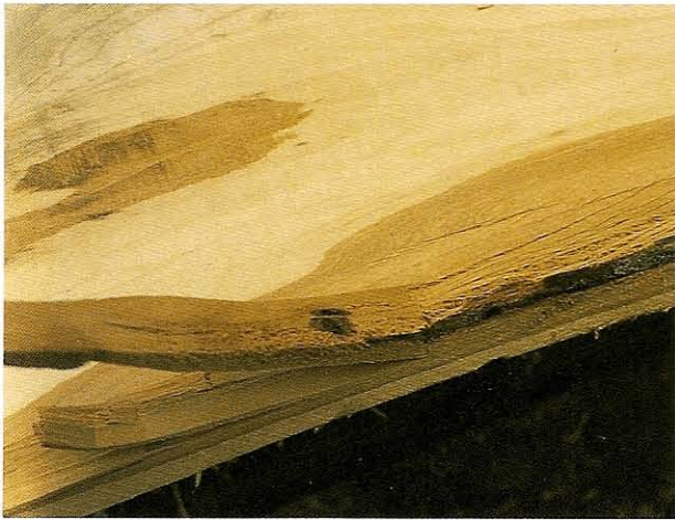
FIG 2.2 A piece of lime wood showing, from the front, the dark outer layer or bark, the pale-brown bast or phloem and the cream-coloured wood or xylem.
