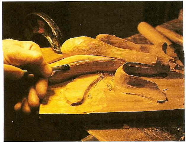
FIG 8.14 Rounding the surface of the banana down to the bottom of the groove with an inverted gouge.
