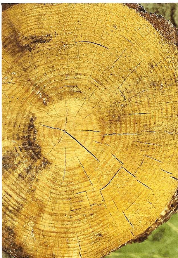
FIG 2.15 The end section of an untreated piece of pine showing end shakes, including some ring shakes. The white spots are fungus mycelia.
