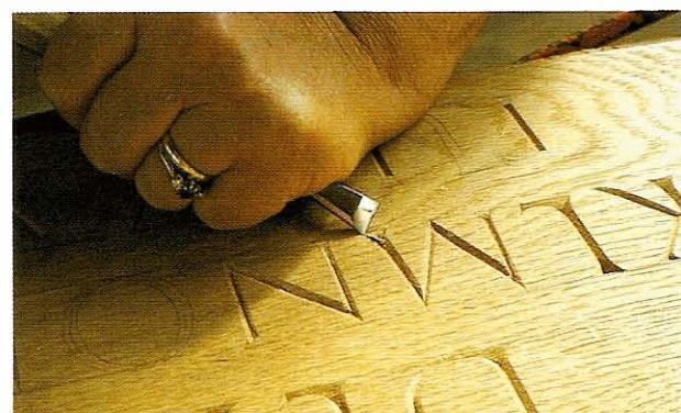
FIG 15.19 The fishtail being used flute-down to start the end of the serif with a chip cut. This should produce a concave end to the serif.
