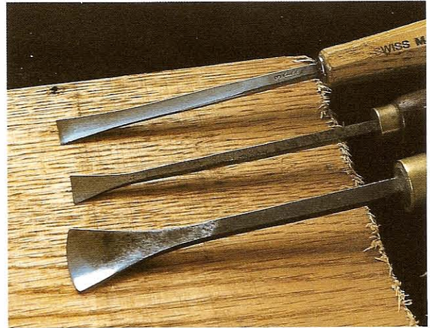
FIG 1.7 Fishtails – from top: Swiss No. 3, English No. 3 and No. 5. Note the greater splay on the English tools and the rounded end of the No. 5 which reduces the tool's usefulness.
