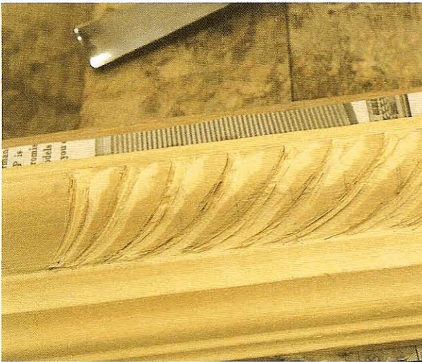
FIG 4.25 The ribs having been established, they can be cleaned up later; the shaping of the gadroons is damaging them. The No. 5 gouge was used flute-up for the inside curves of the tails.
