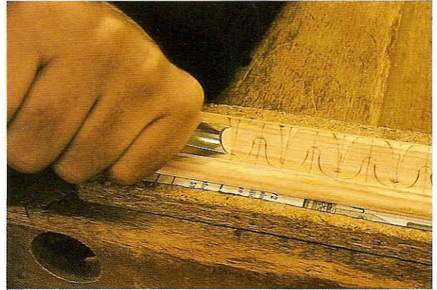
FIG 4.19 Cutting in from the side of the leaf to the edge of the rib with a No. 7 gouge, preferably with a bull nose.
