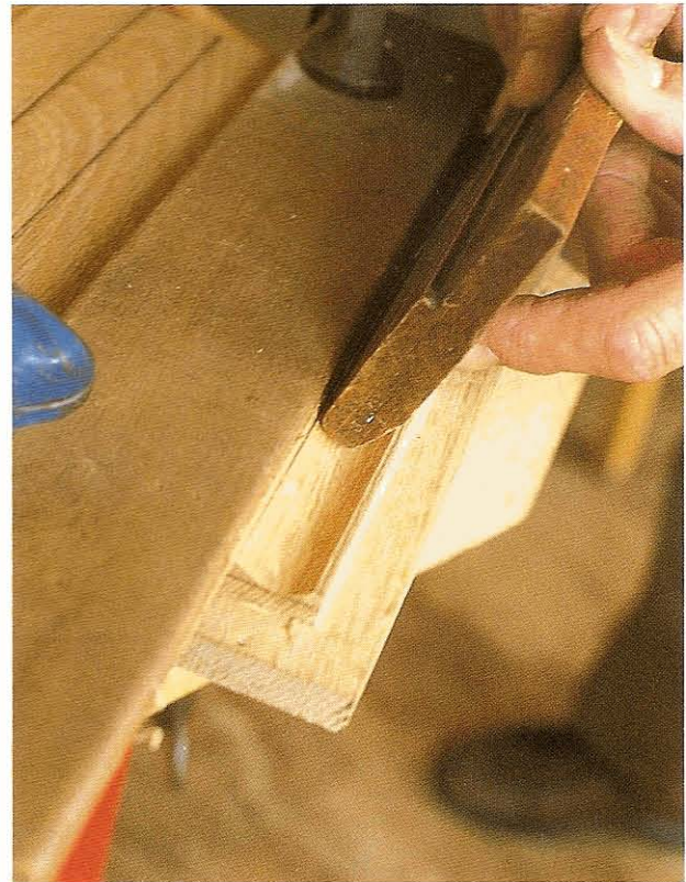
FIG 7.6 A moulding plane used against a fence clamped on the wood to cut a hollow.
