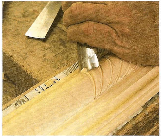
FIG 4.24 The ribs have been roughed out and the large No. 5 is rounding the side of the first gadroon.
