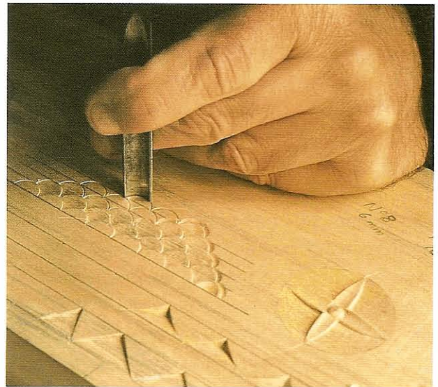
FIG 3.17 A scale being stabbed in with a No. 8 gouge, which is rotated to make a bigger scale. The bottom ones have been chipped out already.
