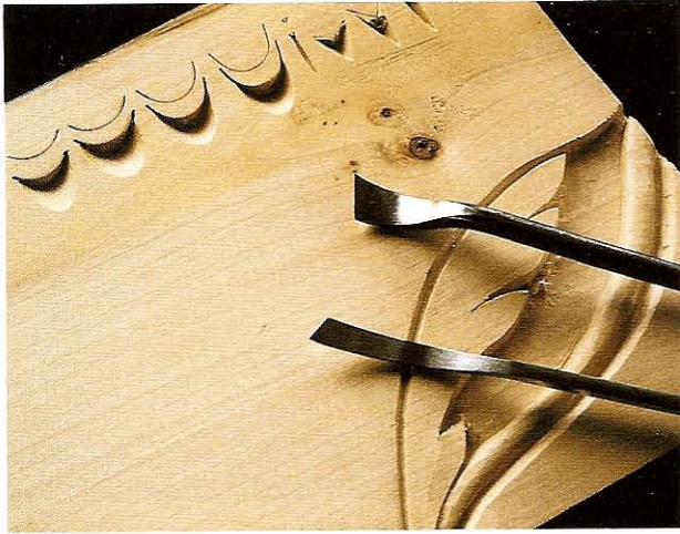
FIG 1.4 Left- and right-hand skew front bent chisels, Nos 22 and 23. Square-ended ones can be modified to produce the same shapes.
