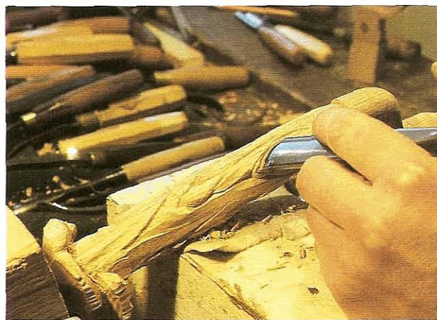
FIG 9.21 Using a chip carving technique to deepen grooves and define shapes.
