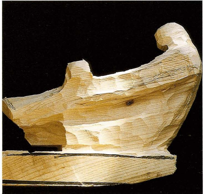
FIG 13.16 The main outline is already there after roughing out with the angle grinder. Note the dark dead knot below the arms.
