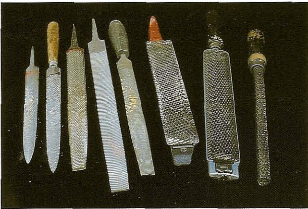
FIG 1.33 Various rasps: from left, two hand-cut rasps, typically pointed; standard half-round coarse bastard rasp; flat and half-round dreadnoughts; three Surform rasps (flat, half-round and roundfile).
