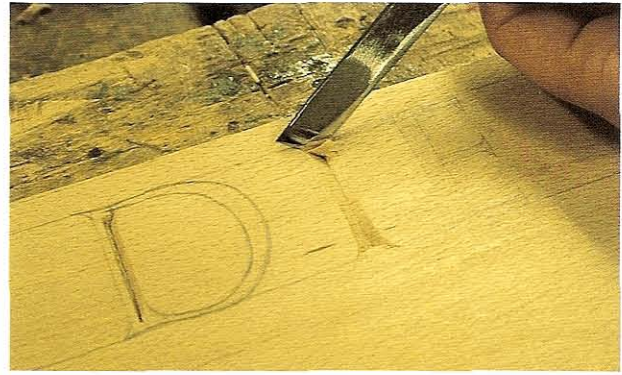
FIG 15.22 The shape of the letter shown. The skew has to have a fairly blunt angle at its tip to reach into the corner of the serif. If it were more acute it would dig in and make a mess.
