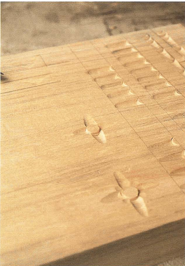
FIG 3.7 Tapered cuts made towards a stabbed circle to form flowers. Note the smaller cuts in the angles of the bottom example.
