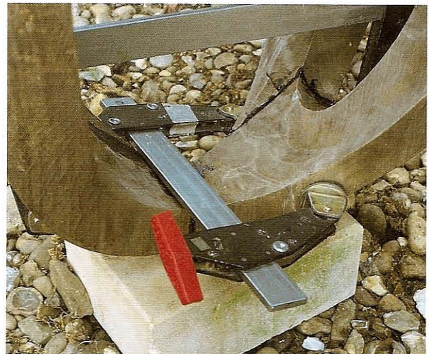
FIG 1.31 A Jet clamp, showing the head fitting well on an angled surface.
