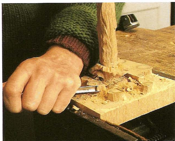
FIG 9.26 Roughing out the bubbles with a No. 11 gouge.
