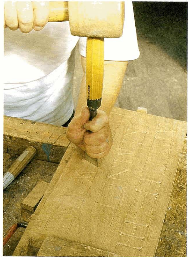
FIG 15.8 Stabbing the centre line of a straight letter with a No. 1 chisel which reaches from the inside point of the serif to level with the inner point of the V.
