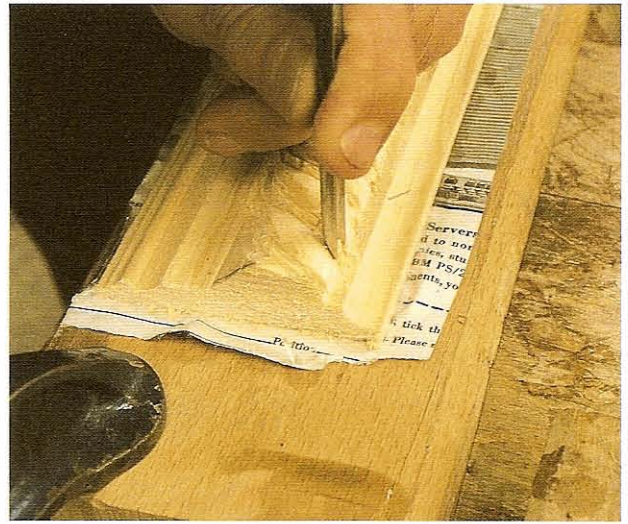
FIG 4.26 Cutting between the noses of the broad ridges with a deep gouge.
