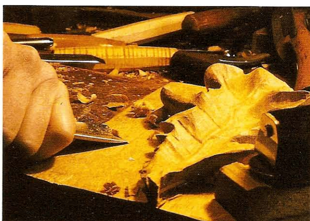
FIG 5.14 The final cuts are made along the ground, with the grain, to get the cleanest finish and to remove dirt.
