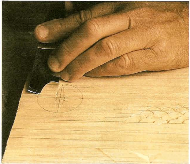
FIG 3.15 The saucer-shaped depression for the flower to sit in is carved by making triangular pockets with the No. 5 gouge. To get a convex outer edge the gouge is used flute-up.
