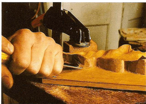
FIG 5.13 The ground cut in to meet the undercut using the same No. 3 gouge.
