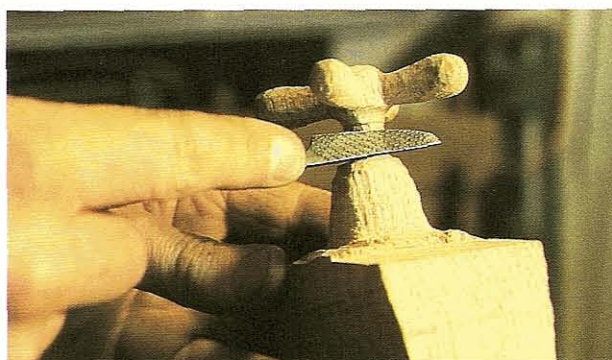
FIG 9.19 Using a riffler to shape the stem of the tap.
