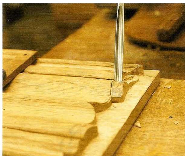
FIG 7.12 The top of the second layer is started by cutting in from the corner of the fold with a deep gouge.
