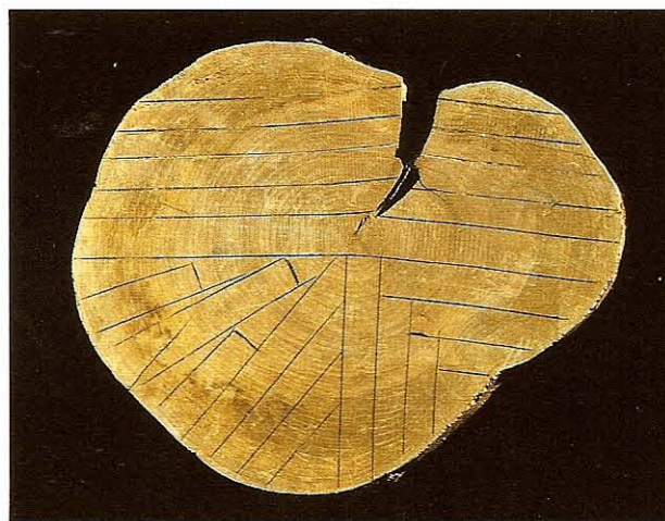
FIG 2.17 Cross-section of a cherry branch. The typical ways of converting the wood into planks were drawn on before the wood began to dry. The top half represents the way boards would be plain sawn. Note the cupping of the boards on the sides away from the heart. The bottom-left quarter shows why true radial sawing is wasteful. The bottom-right quarter and the next part of the bottom left show more economical ways of quarter sawing.
