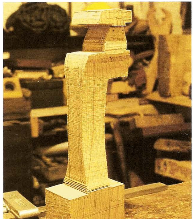
FIG 9.17 The shape bandsawn to yield large offcuts.
