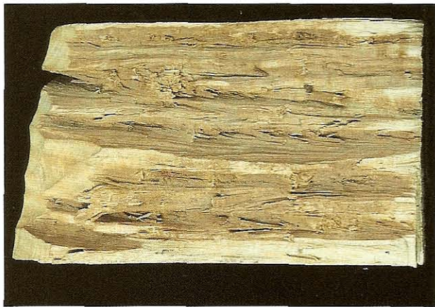
FIG 2.9 Satinwood when planed and sanded smooth has an attractive lustre in its cell walls. The different angles of the grain visible where it has been riven make carving along the grain virtually impossible.
