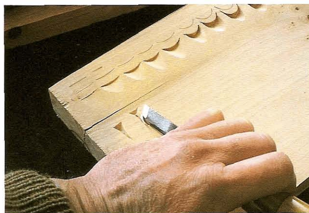
FIG 1.11 Skew chisel chasing the side of a groove, as in letter cutting.
