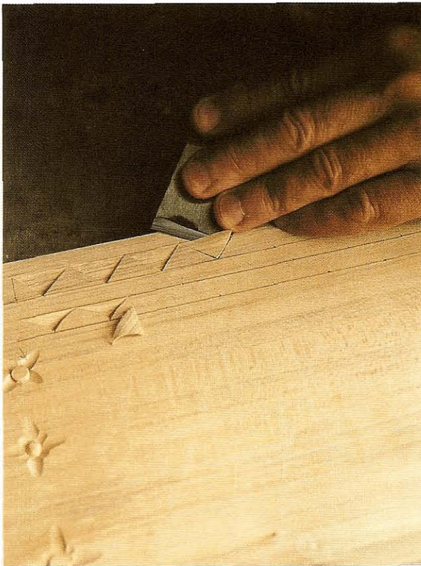
FIG 3.10 Triangular pockets. After the V is stabbed, the chisel is sloped down into the centre of the cut, starting with its corner entering the wood at one of the shallow corners and following that side of the V line until the edge meets the other line. The back line should occur naturally.
