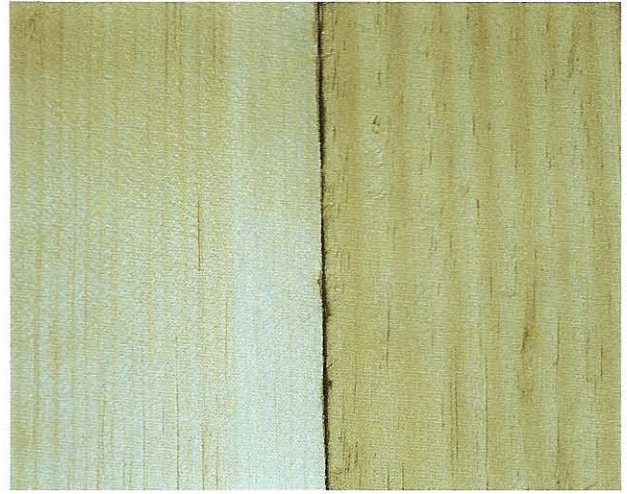
FIG 2.5 Slow-grown Quebec yellow pine (left) compared with the coarser texture of fast-grown southern yellow pine (right). The dark lines are resin ducts.
