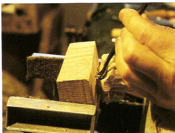
FIG 9.23 Shaping grooves under the splash with a deep spoon bit gouge.
