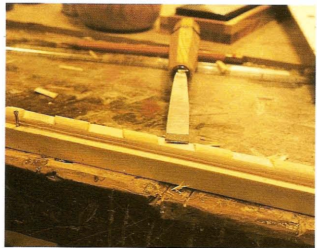
FIG 4.14 The first stage in cutting ribbon and stick, showing the straight edge used. Note that it is narrower than the interval it has flattened.
