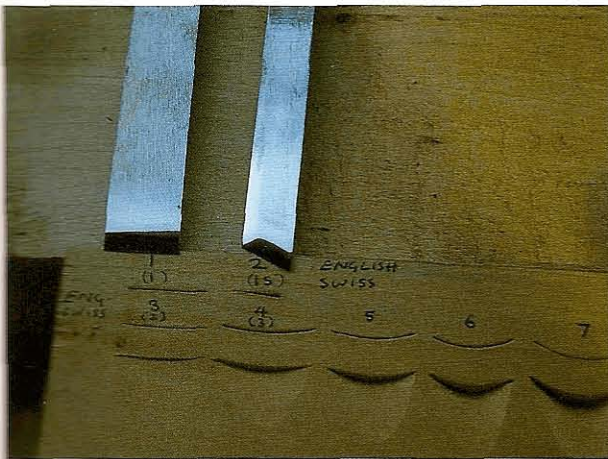
FIG 1.2 No. 1 straight-edge and No. 2 skew chisel. Note that the metal has been ground back on the side running from the obtuse angle to make it less likely to pinch in a groove.
