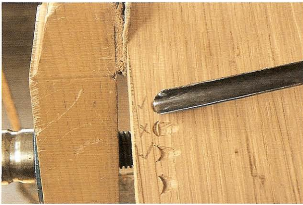
FIG 3.5 From the bottom: two correct chip cuts; the classic mistake where the chisel has been reversed; and how this cut can be made successfully with a special shape to the gouge edge.
