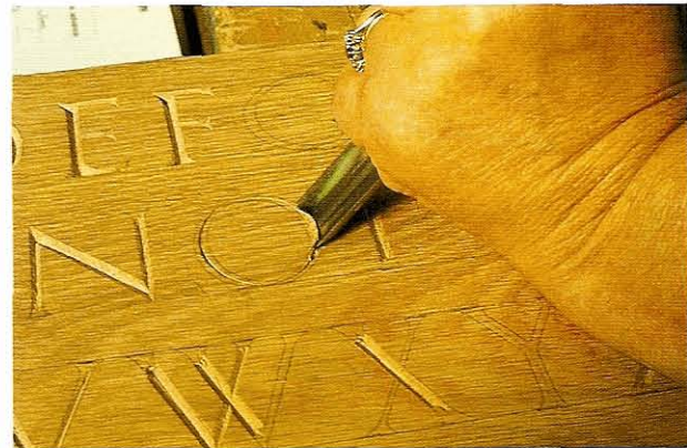
FIG 15.13 A large gouge stabbing in the inward-facing curve of an O.
