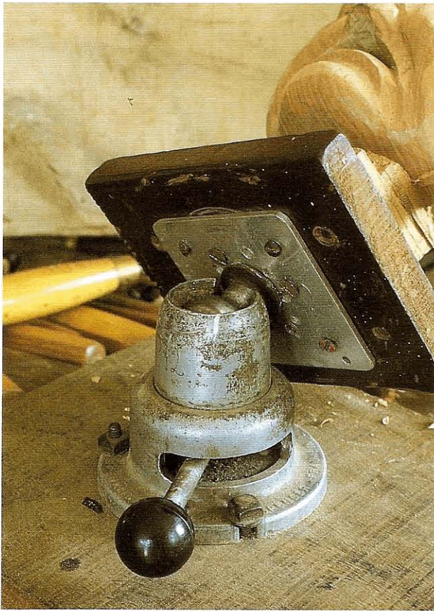
FIG 1.28 A universal vice of the ball-and-socket type with a homemade face plate. The work is screwed on from underneath.
