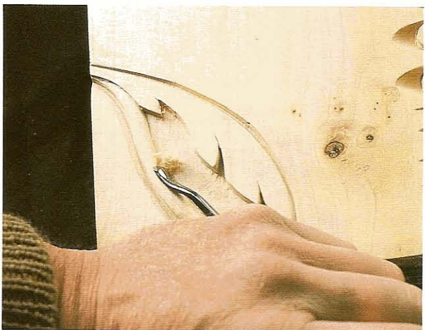
FIG 1.16 Backbent gouge rounding a stem on an inside curve.
