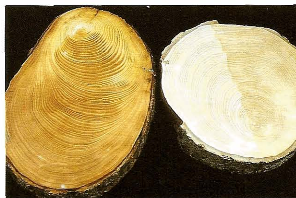
FIG 2.19 Reaction wood. Compression wood of Cedar of Lebanon (left) and tension wood of ash (right). Note the off-centre pith and the irregular colouring. The right-hand side of the ash has been cut with a chisel to show the advantage over the dull sanded finish on the left.
