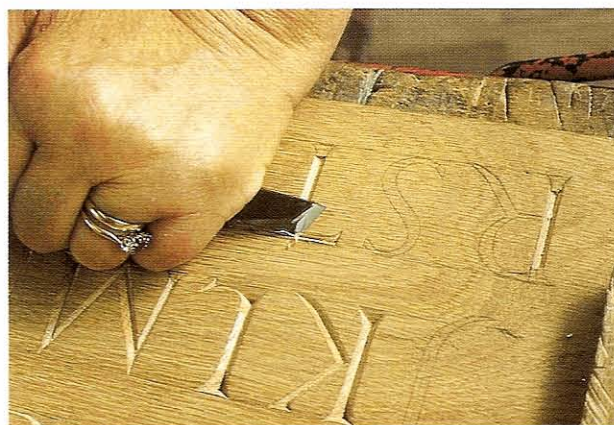
FIG 15.25 Chasing the side of the arm of the T with a skew chisel.
