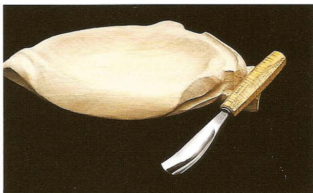
FIG 10.6 Beech bowl nearly finished, showing a No. 8 long-bend gouge resting against the holding lug which is still retained.
