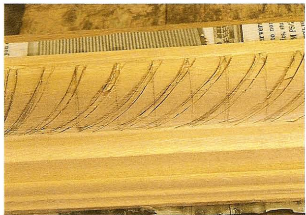
FIG 4.22 Gadrooning drawn up and the small ridges stabbed in. It does not matter that the wood has split as it will be carved later.
