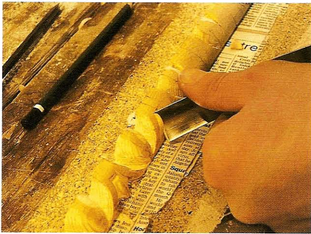
FIG 4.12 After the rim of the cup has been stabbed in, a chip cut facilitates the shaping of the dart.
