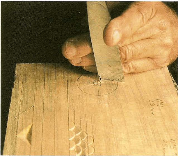
FIG 3.14 Starting a more complex flower. The centre ring has been stabbed and a circle marked outside it less far away than the No. 5 will reach. Note the pencil marks around the inner circle. The diameters should continue beyond the outer circle. The edge of a petal is stabbed here.
