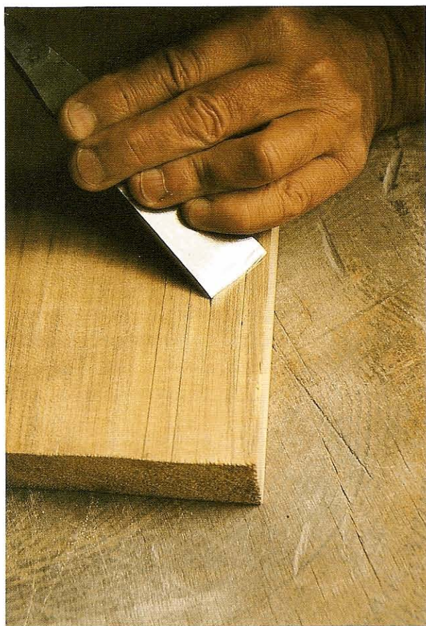
FIG 3.11 Making the stab cut at too shallow an angle. The wood splits and the corner of the V will look rough. Here the chisel has wrongly bitten into the wood beyond the back line.
