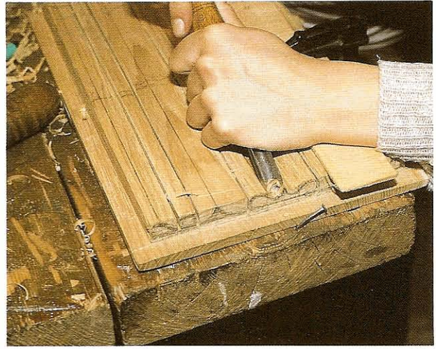
FIG 7.5 A deep gouge carving a deep fold. The saw cuts do not always follow every line drawn along the surface.
