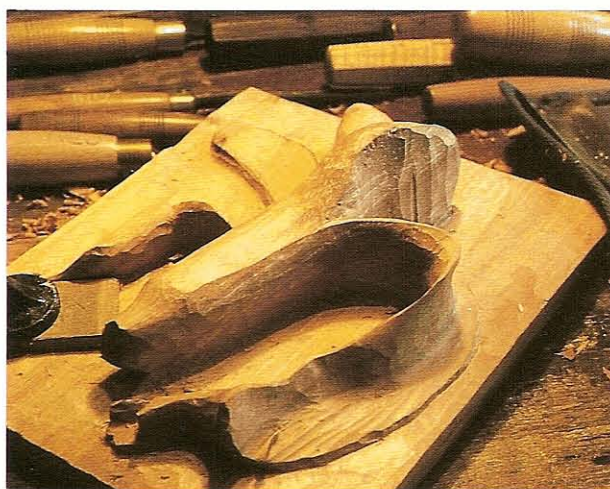
FIG 8.10 The undercutting of the overhanging piece of skin is not attempted until the flesh part has been shaped.
