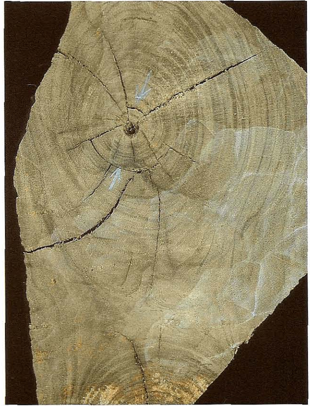
FIG 2.21 Transverse section of a fork in walnut. Note the light-coloured diseased areas and the arrowed ring shakes. The many shakes around the typically large pith were almost certainly present in the growing tree.
