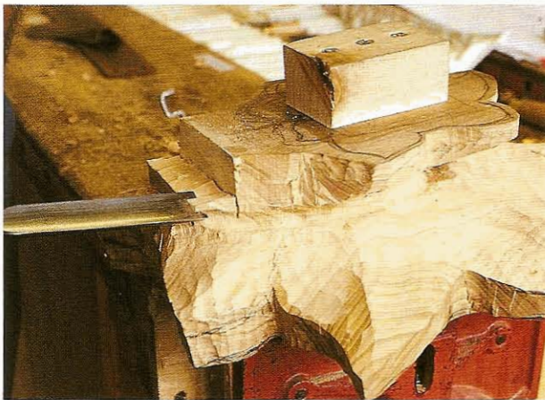
FIG 10.18 Cherry-wood bowl held in vice by block screwed into top surface of the bowl blank. Note the chisel being used to split off wood to the saw cut.
