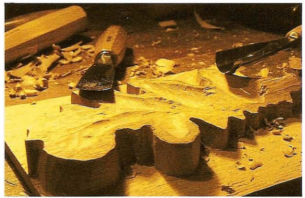
FIG 5.8 The two gouges used for tilting the edges of the leaf and beginning to model the hollows. Note the sharp join between the ground and the vertical sides.
