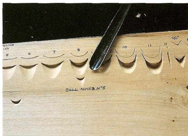
FIG 1.18 A bull-nosed No. 8 gouge with its chip cuts. Note the deep marks left in the corners by the conventional No. 8 in the cut above.
