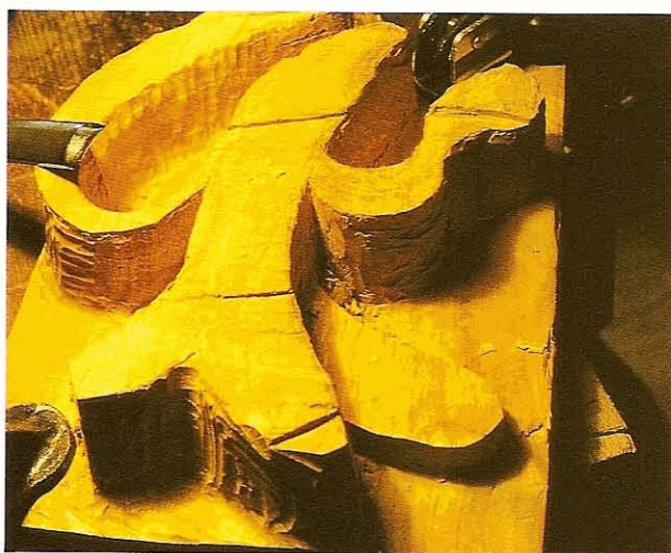
FIG 8.6 The outline has been set down and the lowest levels established.
