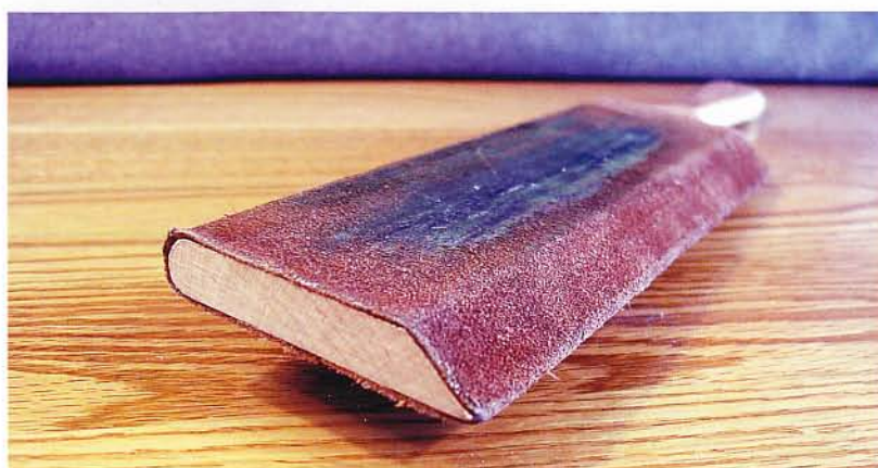
Butz strop. The curved and angled sides sharpen gouges and V-tools. Use the flat surface to sharpen knives.
