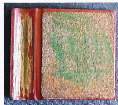
Slip strop. The strop's two sides include a variety of surfaces for stropping gouges, V-tools, and knives.
