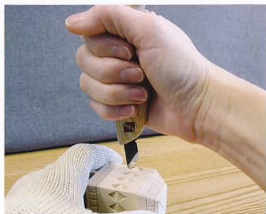
Overhand grip with the skew knife. Hold the skew knife just as you would hold a dagger.
