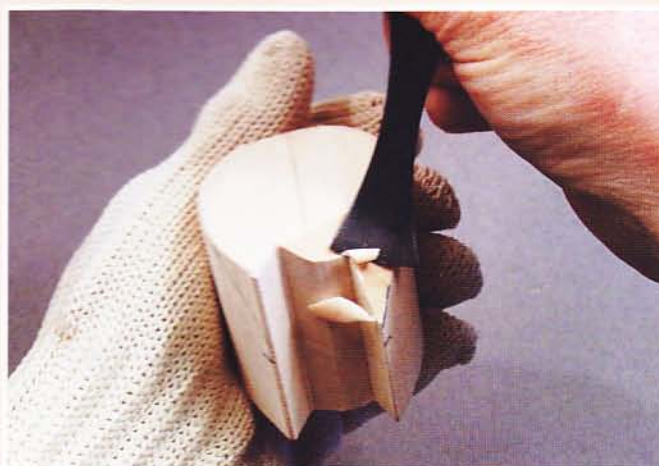
30 With the #3 \frac{7}{8} " or #3 \frac{5}{8} " gouge, carefully round the backs of the ears.
