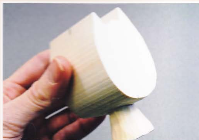
28 Use the #3 \frac{1}{8} " or #3 \frac{1}{4} " gouge to round the neck. The diameter of the cat's neck at the base is 1" and near the head, \frac{3}{4} ".
