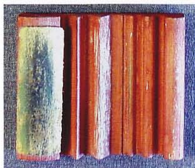
Slip strop. The strop's two sides include a variety of surfaces for stropping gouges, V-tools, and knives.
