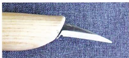
Detail knife. Delicate details are carved with the thin, sharp-tipped blade of a detail knife.
