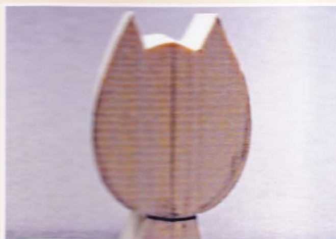
26 Band saw the pattern for the cat's head.
