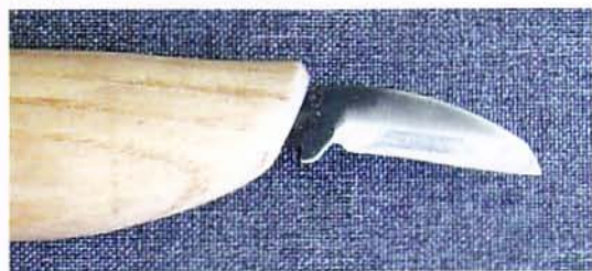
Bench knife. The bench knife has a sturdy blade and is used for scoring, rounding, and shaping.
