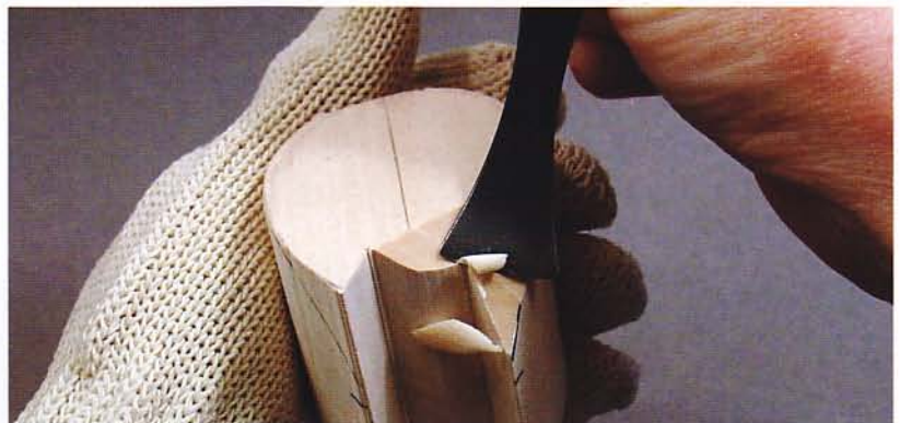
Gouge cut. Bring the gouge toward you, keeping your opposite hand out of the path of the gouge.
