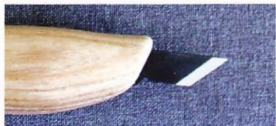
Skew knife. The 45-degree angle of this knife blade creates the geometric shapes associated with chip carving.
