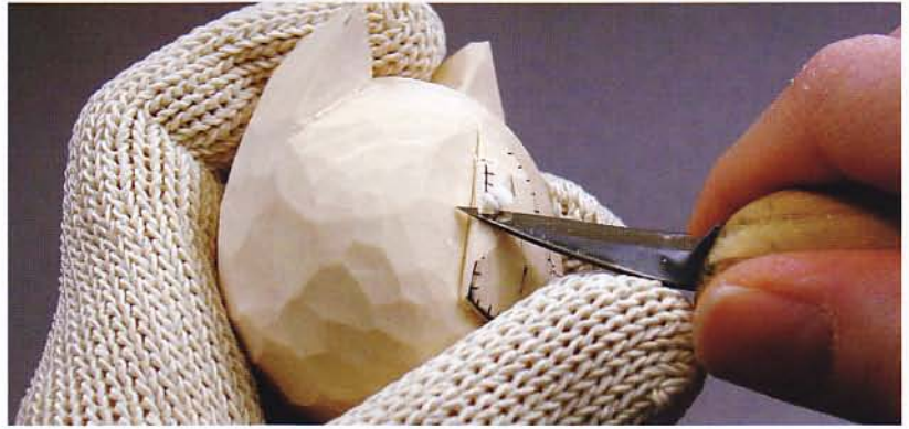
Push cut. Use the thumb of your opposite hand to push the blade of the knife away from you.
