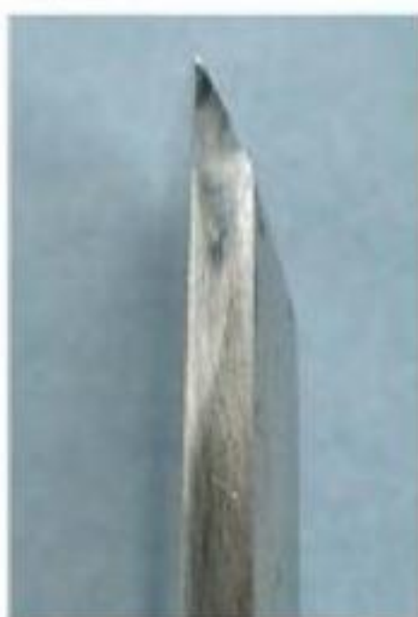
Figure 3-2. This bench chisel has an angle of approximately 35 degrees.
