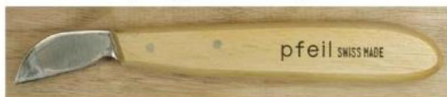
Figure 2-4. Notice the downward angle of the blade as it comes from the handle of the main cutting knife. This blade angle was a huge innovation that helps in maintaining the consistency and proper angle for carving.
