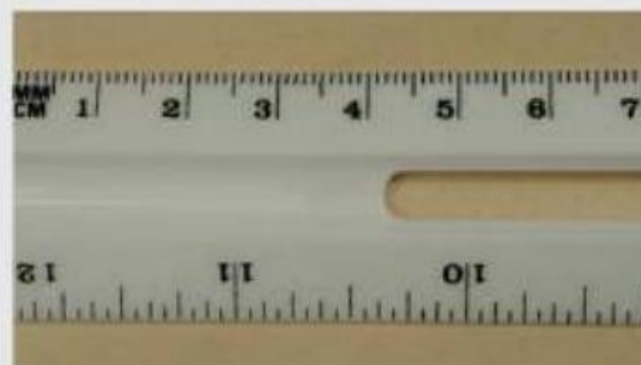
Figure 5-16. Many rulers and T-squares have both English or Imperial and metric measurements. This one has been enlarged to show detail.
