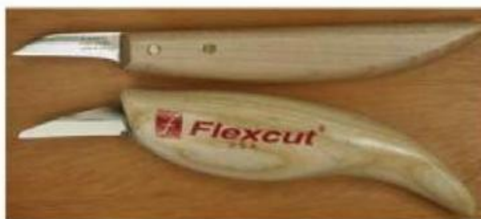
Figure 2-1. Conventional carving knives are not suitable for chip carving because the blade comes straight out from the handle without a downward angle.
