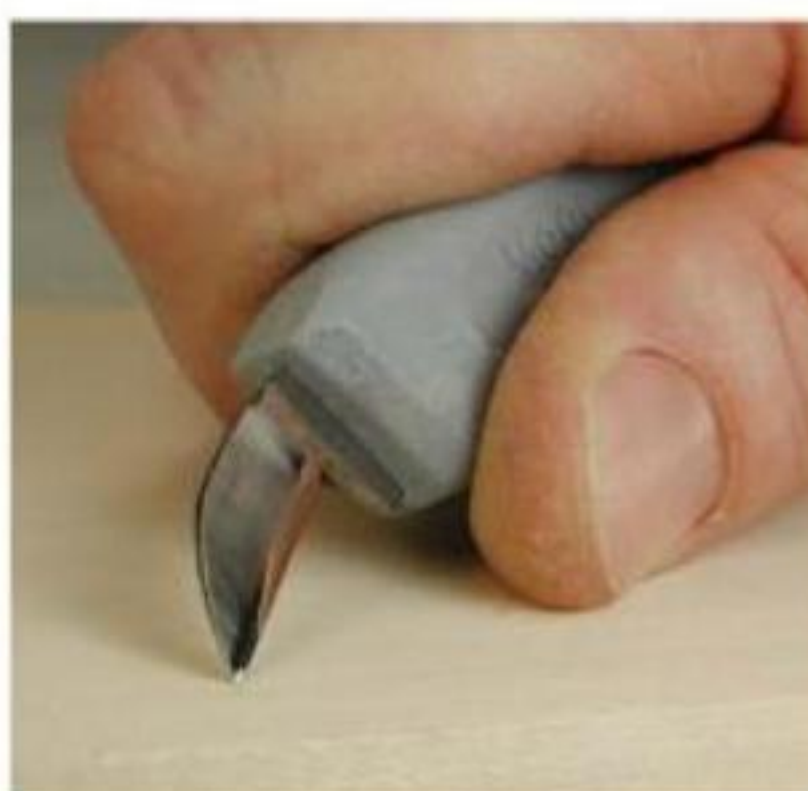
Figure 4-12. Hold the small knife at a 65-degree angle just as you would the large knife.
