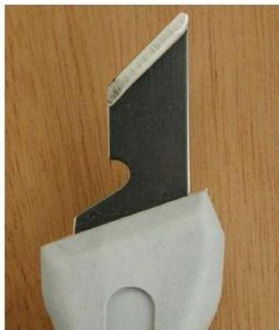
Figure 3-15. The tip of the stab knife is ground to an angle rather than to a point.
