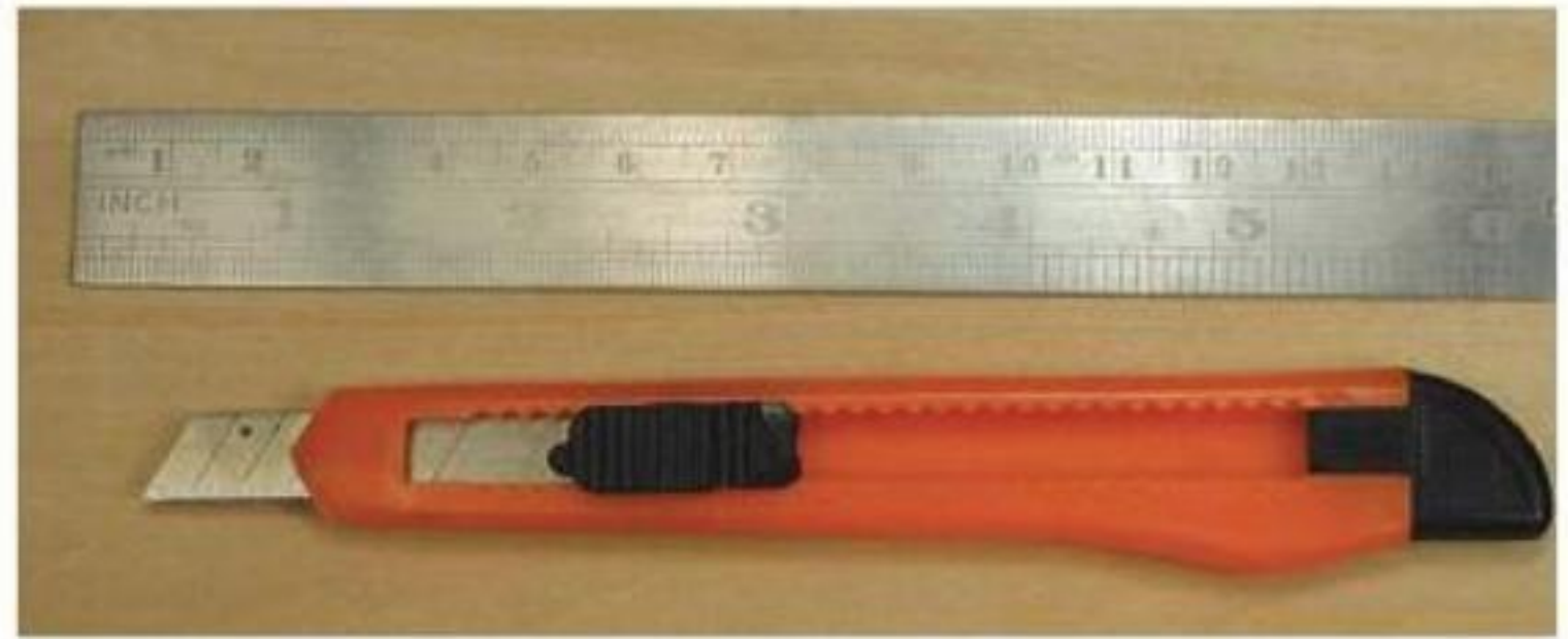
Figure 5-21. A steel ruler and a razor blade for cutting long straight-line chips.
