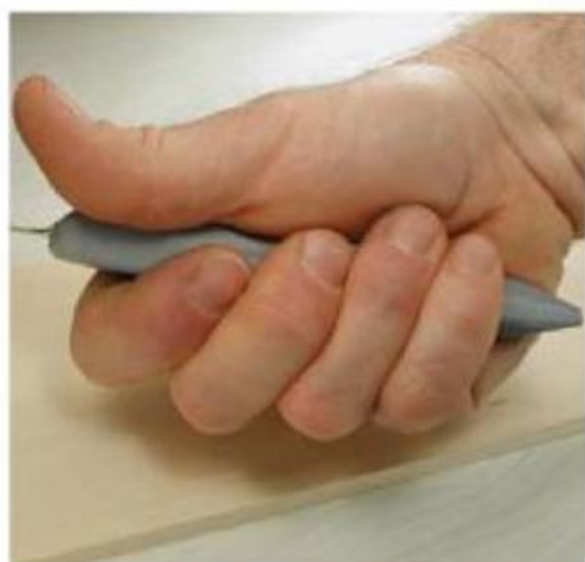
Figure 4-11. The handle of the small knife is long enough to protrude past your grip.
