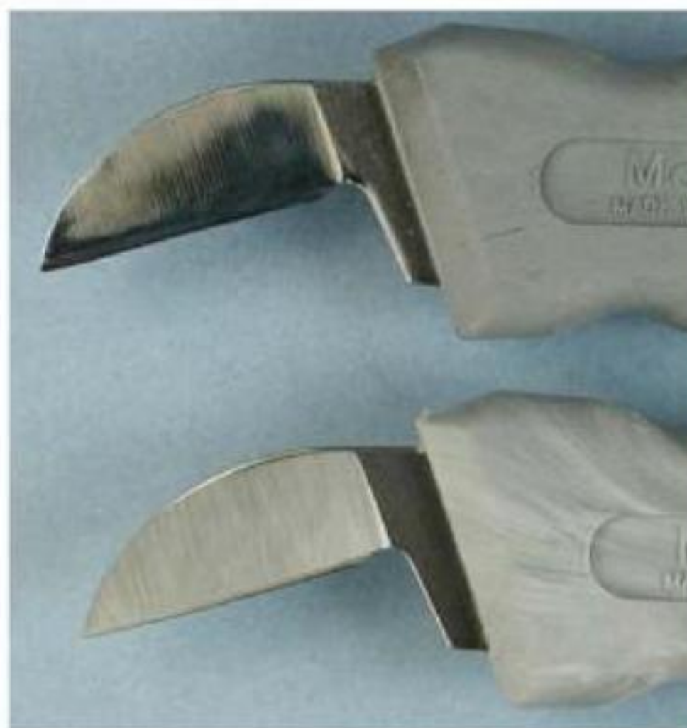
Figure 3-13. Compare the polished edge of the top blade to the unpolished bottom blade.
