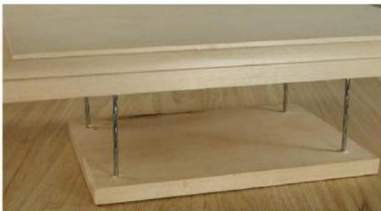
Figure 1-11. The homemade support suspends your wood and allows air to flow on all sides.
