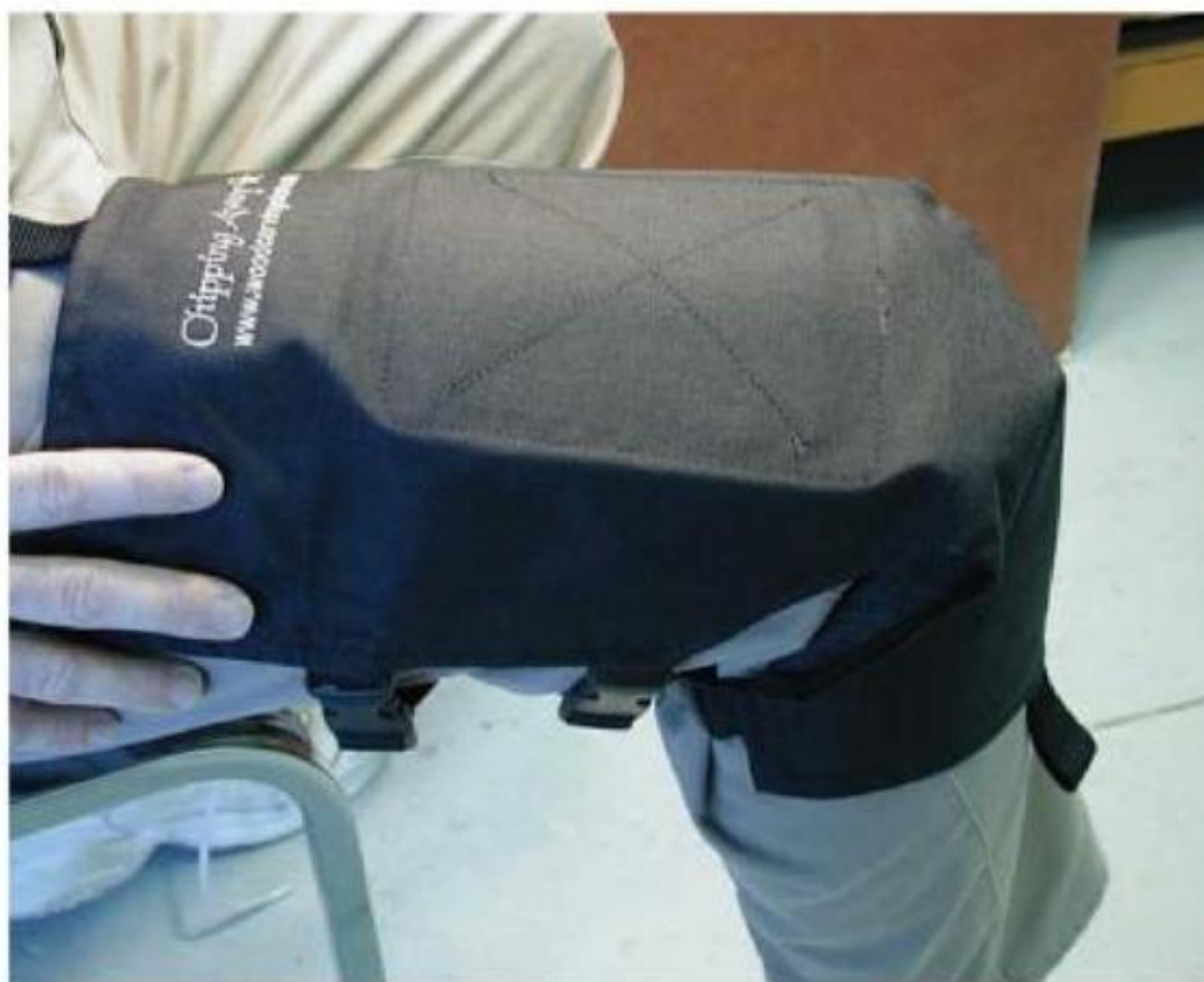
Figure 2-14. Notice how the apron's work surface is reinforced with a heavy synthetic pad, protecting my leg or clothes from any stray cuts.
