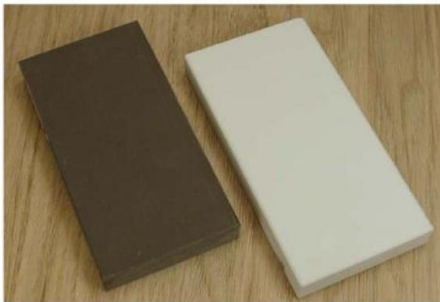
Figure 3-11. The dark ceramic stone (left) is approximately 800-grit. The white ceramic stone (right) is approximately 8000-grit
