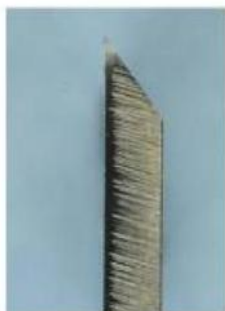
Figure 3-1. This joiner blade has an angle of approximately 45 degrees.
