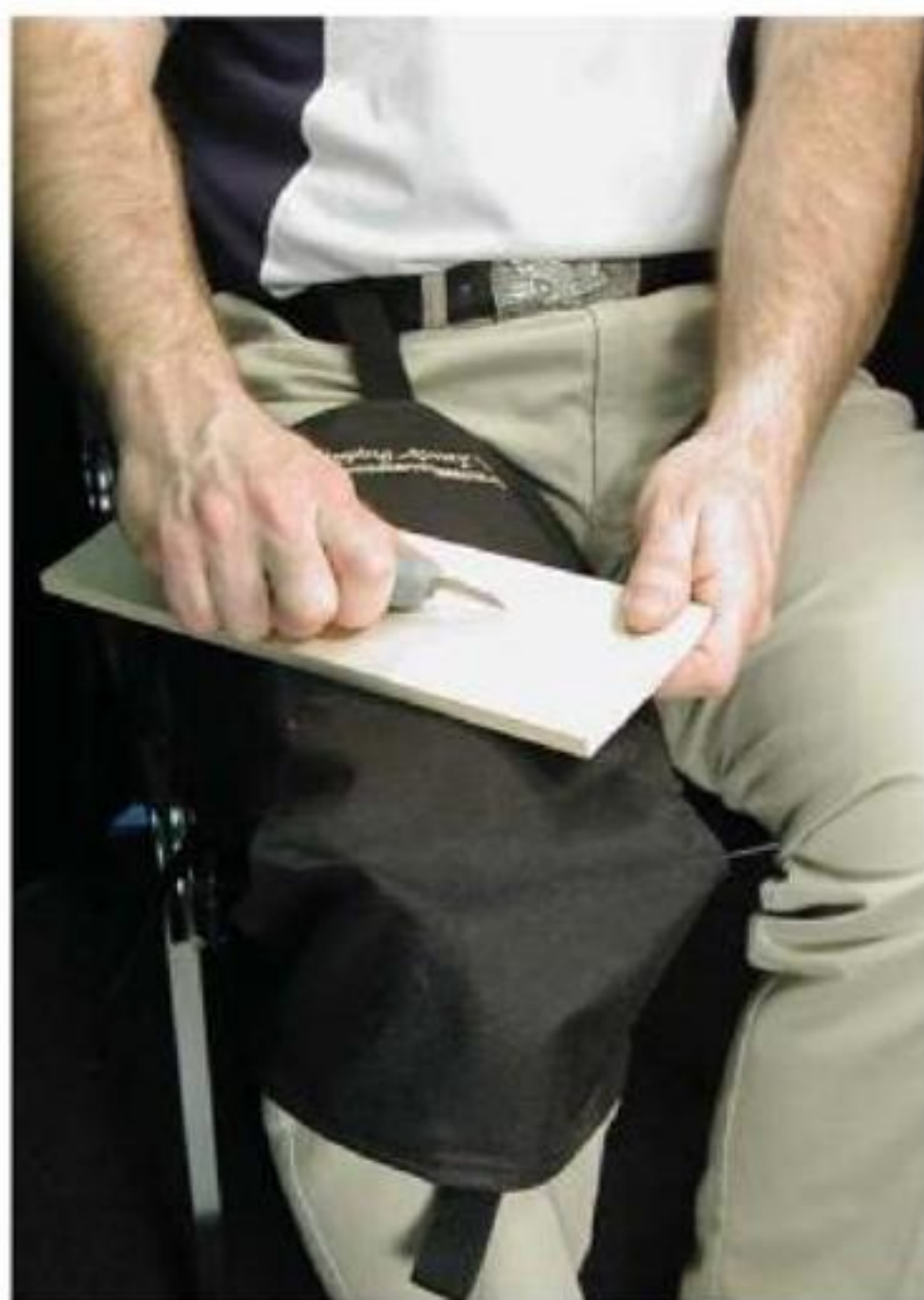
Figure 2-13. Because chip carvers often carve on their laps, they need to wear protective gear. Here, I am using a leg apron.
