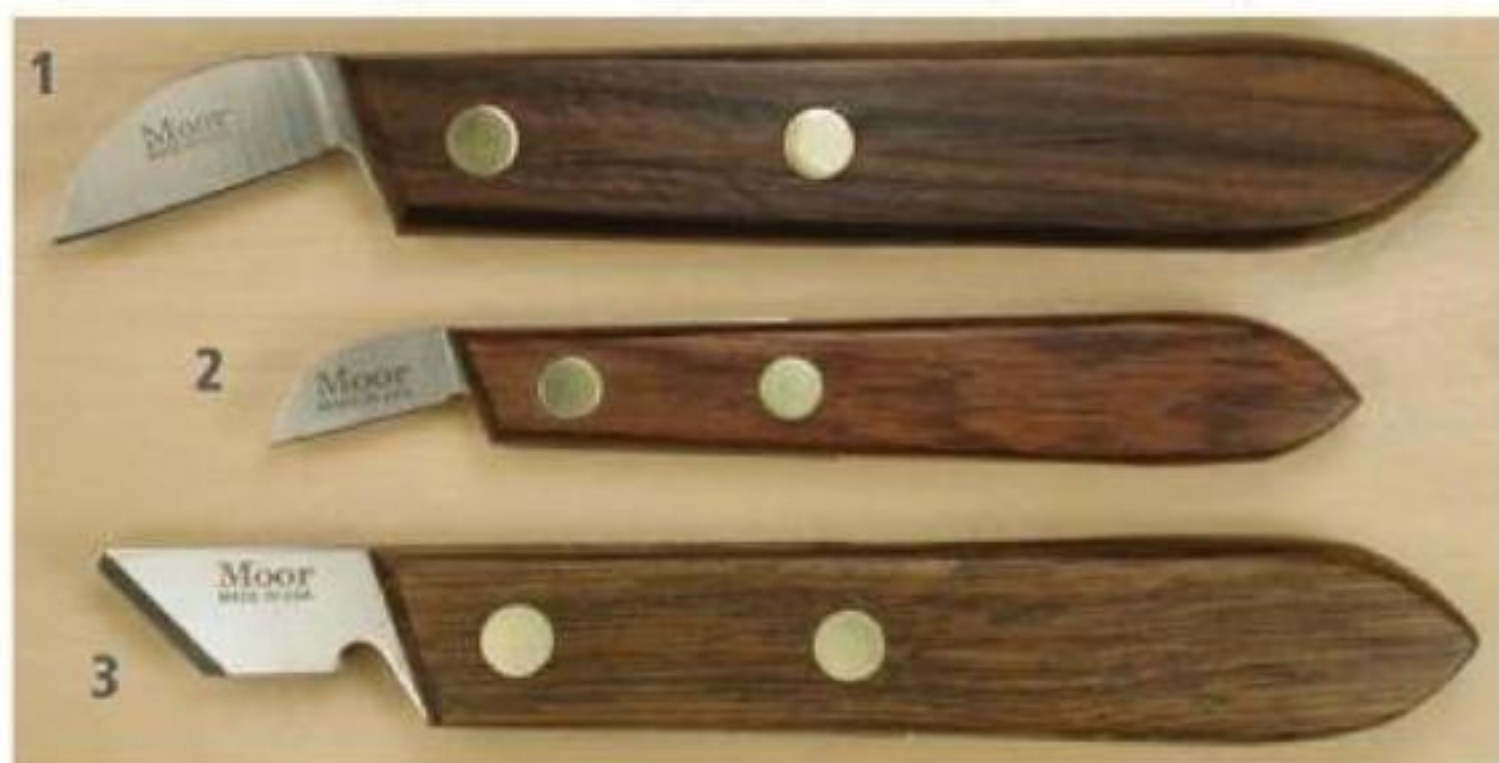
Figure 2-5. A set of three tools, introduced in the early 1990s, that was designed to produce maximum results with either the traditional or the more contemporary styles of chip carving.
