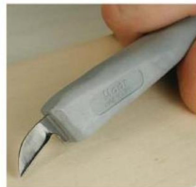
Figure 4-10. Notice how the handle flares out for added grip.
