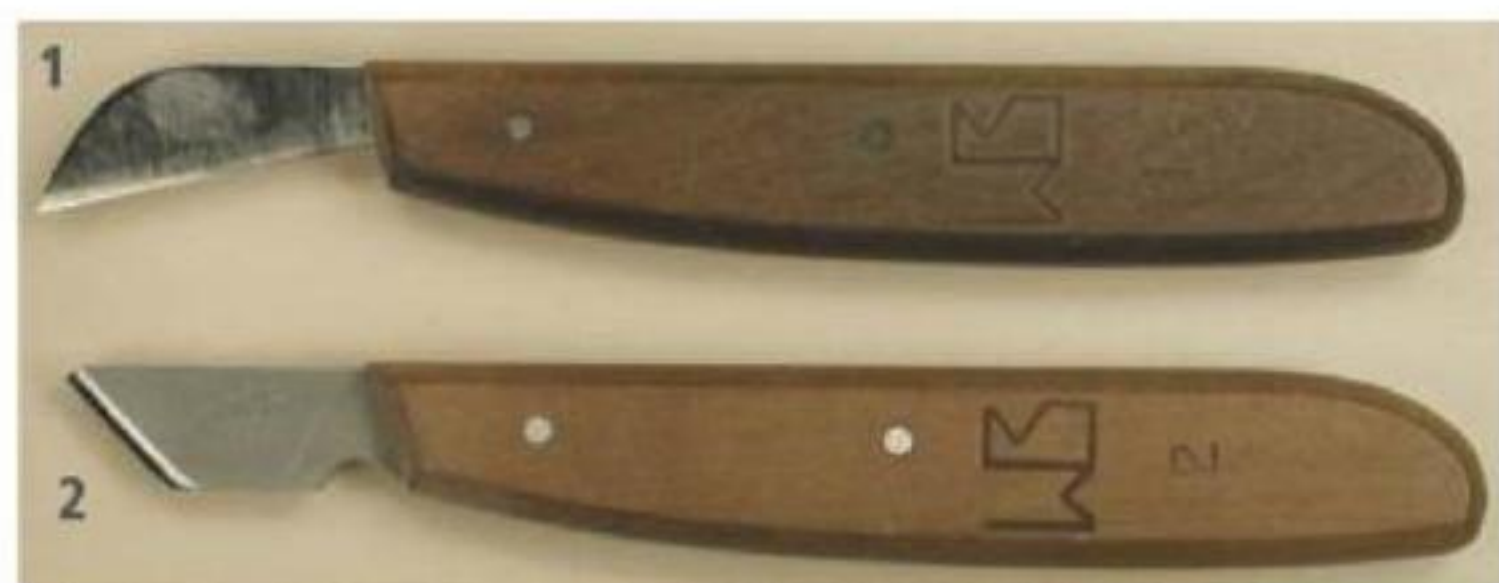
Figure 2-3. The Swiss eventually refined their approach to include only two basic tools—the cutting knife (1) and the stab knife (2).
