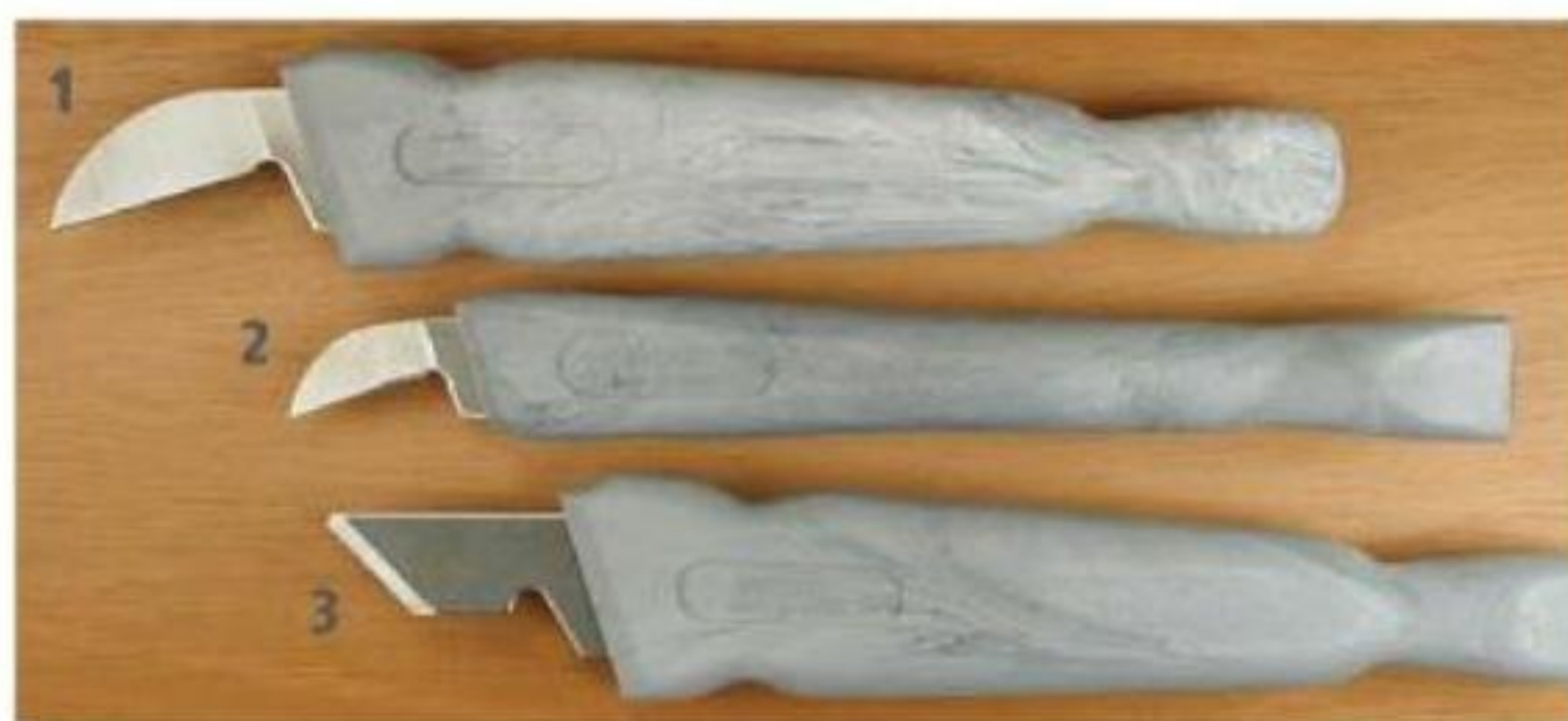
Figure 2-6. Improvements to the Moor chip carving knives included a longer handle for knife 2 as well as more ergonomically shaped handles for knives 1 and 3.
