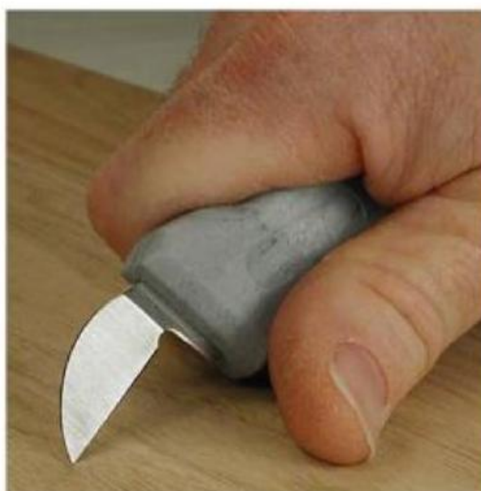
Figure 2-7. Notice how the ergonomic handle is designed for the proper grip.
