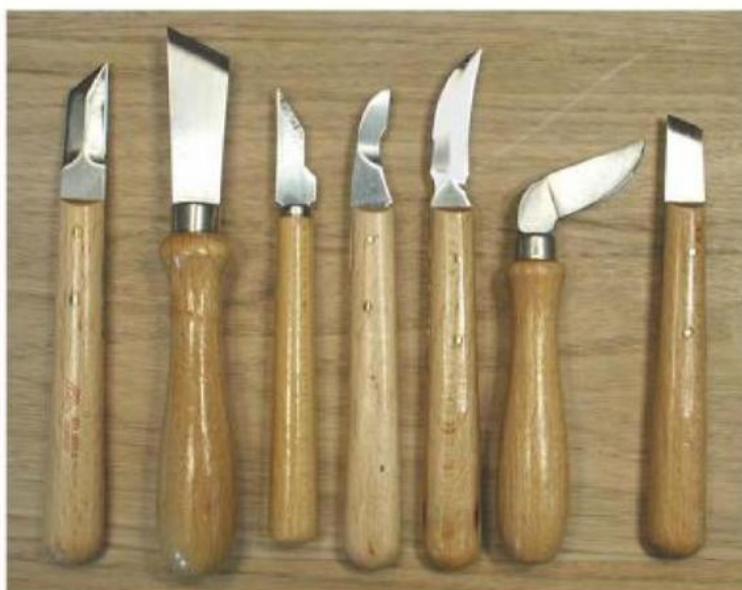
Figure 2-2. Seven of ten tools, specifically designed for chip carving, offered by a German company.
