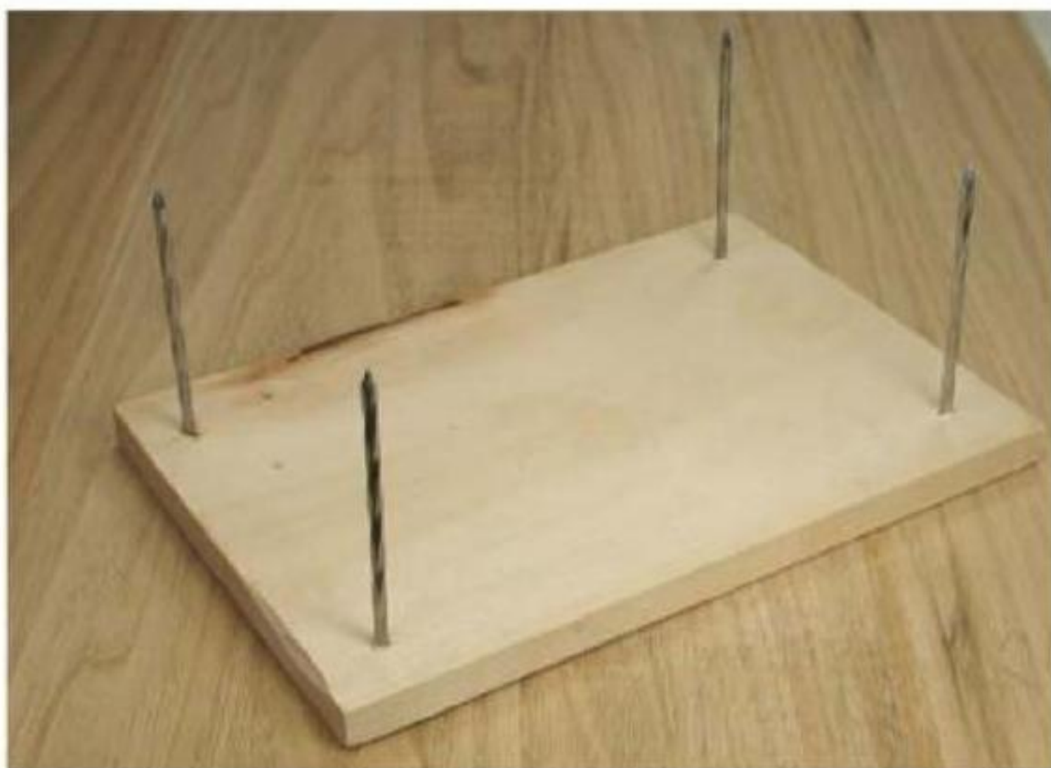
Figure 1-10. Create a simple support by driving finishing nails through a thin piece of plywood.
