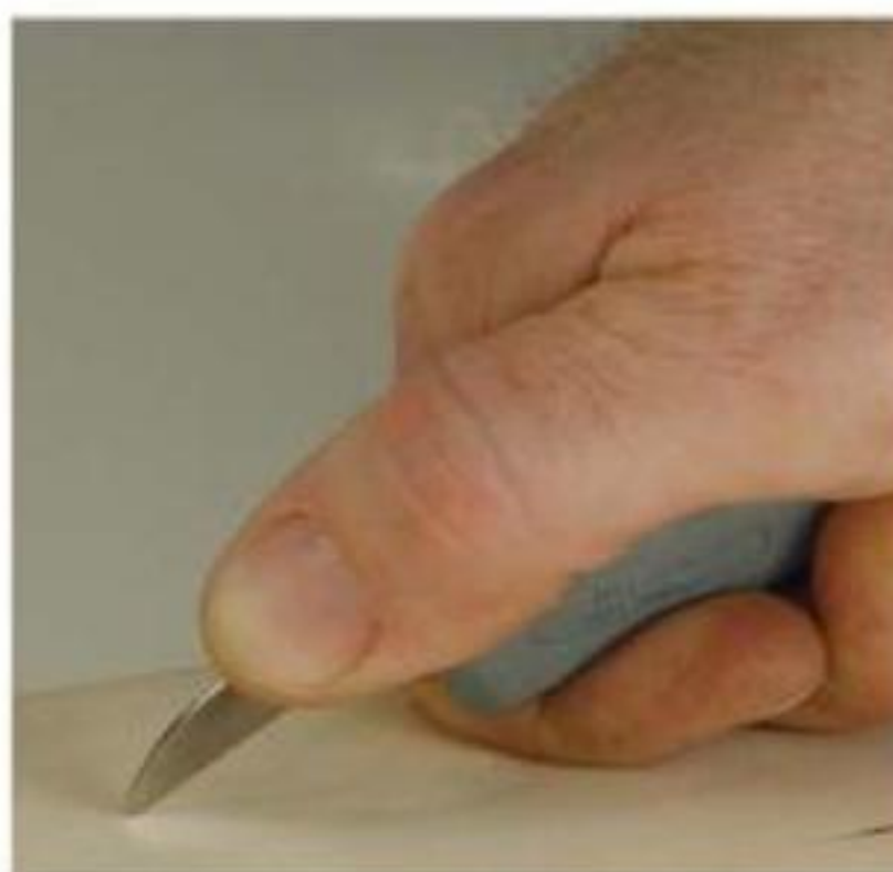
Figure 4-9. Notice how the thumb is placed on the back edge of the knife and on the handle. Keep your fingers in contact with the wood at all times.
