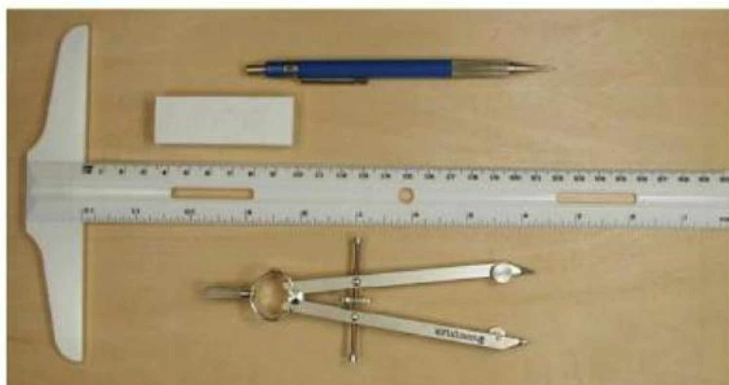
Figure 2-8. Basic drawing tools: 0.5mm mechanical pencil with B lead, white polymer eraser, 12" T-square, and 6" bow compass.
