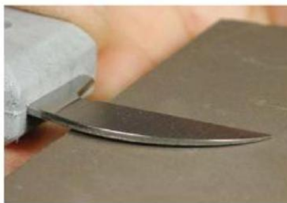
Figure 3-5. Ten degrees is about the thickness of the back edge of your knife.
