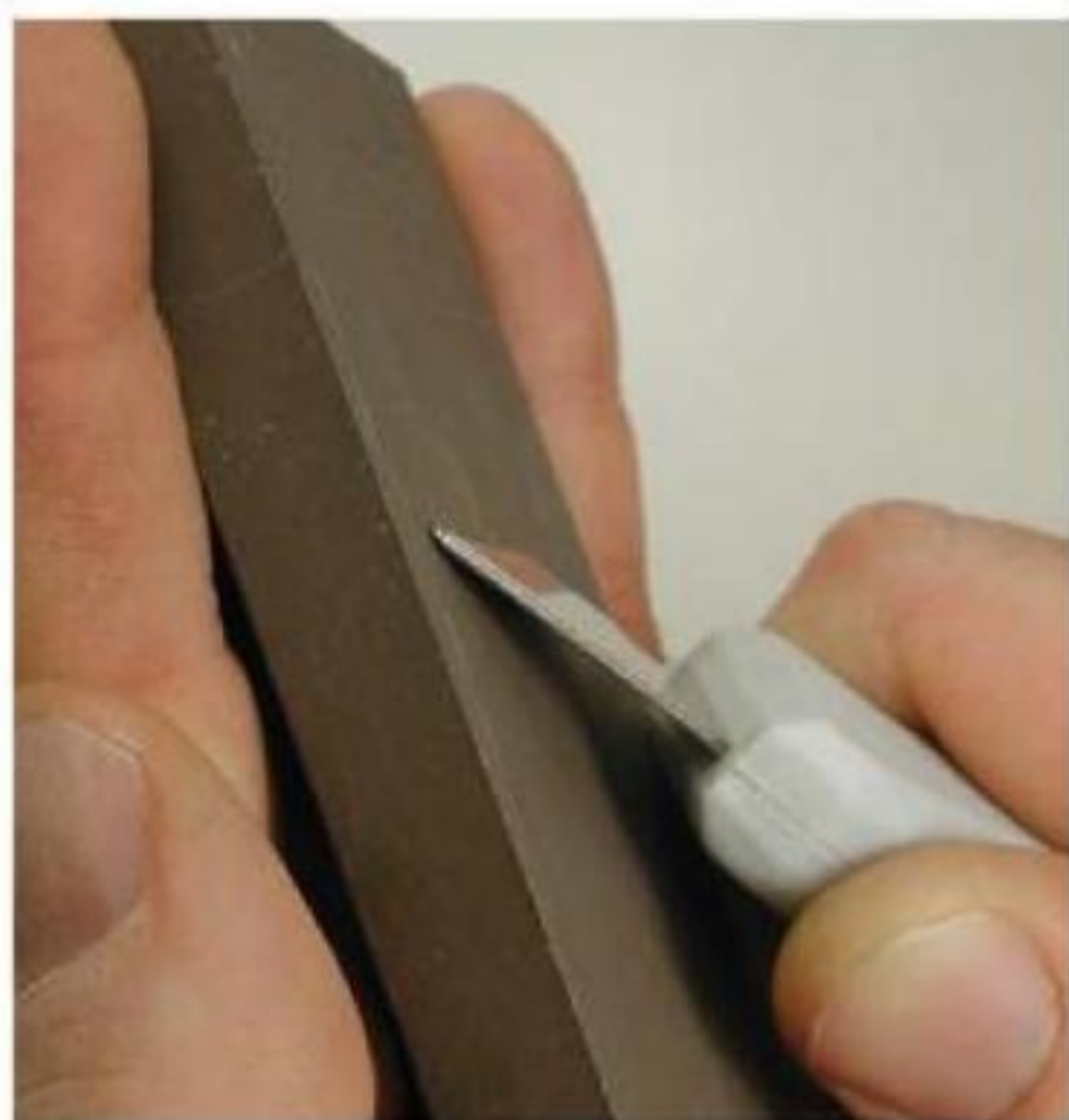
Figure 3-16. The stab knife, sharpened to a 25-degree angle. This stab knife comes in a pre-ground state and requires only minimal sharpening.
