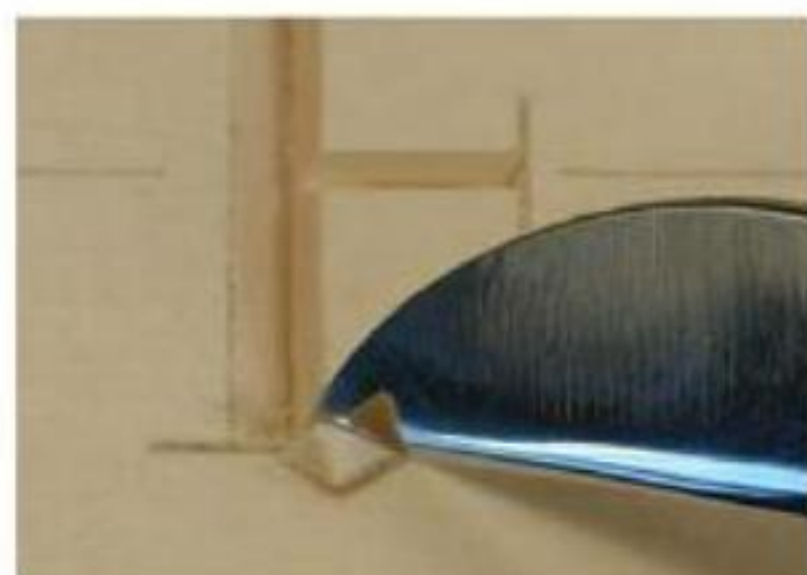
Figure 13-18. Now that the letter is carved, it's time to go back and chip out the serifs. Use both position one and position two, just like the flip-flops.
