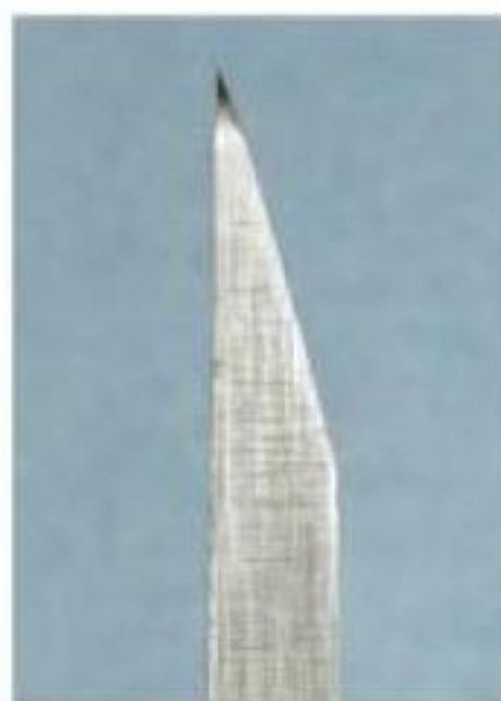
Figure 3-3. This mortise chisel has an angle of approximately 25 degrees.
