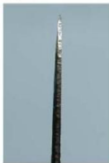
Figure 3-4. The angle for a chip carving knife, as seen when looking at the back edge of the blade.
