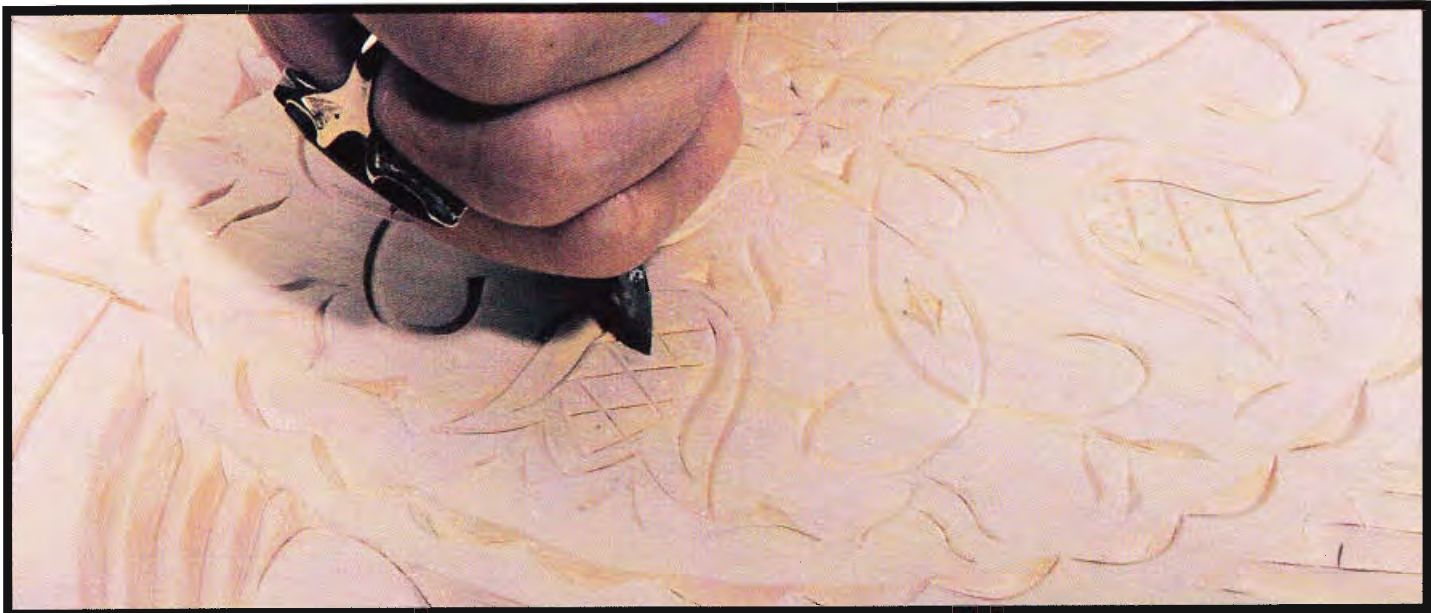
A final touch to the top is to put dots in the diamonds of the tulips with a nailset.
