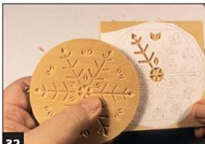
32 Complete the carving and finish. All major cuts have been made on the piece on the right. The board on the left shows the finished carving. I use my band saw and a 1" belt sander to finish the edge. Then, I remove the paper, sand, and seal the wood.
