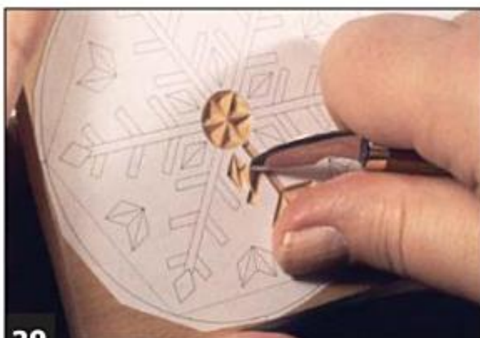
29 Remove the chip. The final chip of the diamond is released.
