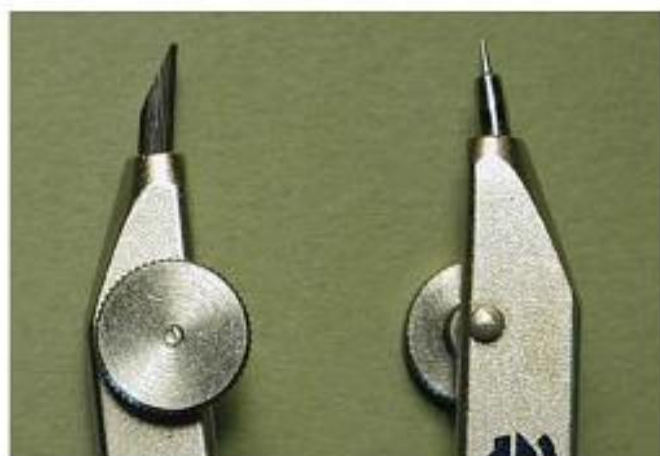
Figure 14-1. Notice that the lead in a compass is sharpened to one side.
