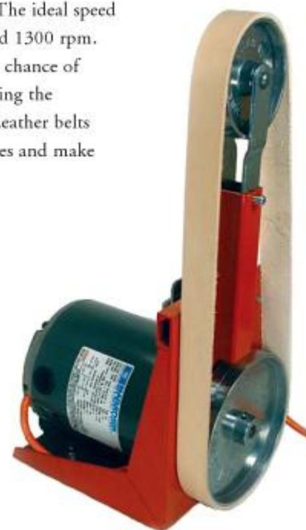
Figure 3-17. I have never found a better power sharpener than a simple 1" belt sander that has been converted, such as this one.
