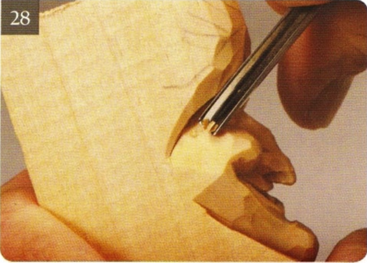
28 Carve the crow's feet. Use a \frac{1}{8} " V-tool to add a few wrinkles and crow's feet to the corners of the eyes.
