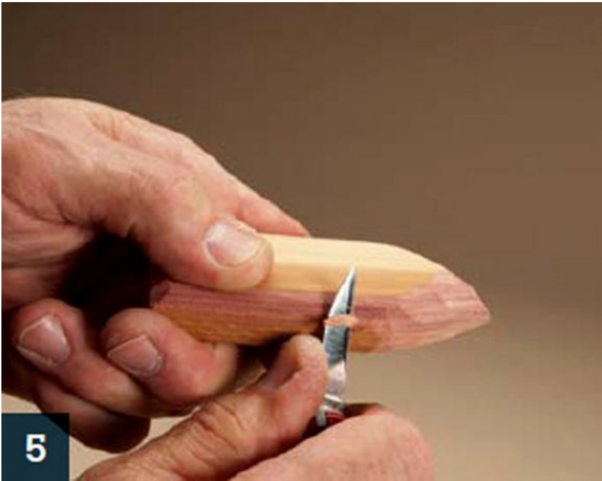
Shape the bottom of the hull the whole way around the boat.
