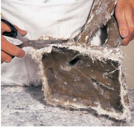
9 Trim off the excess matting where necessary.
