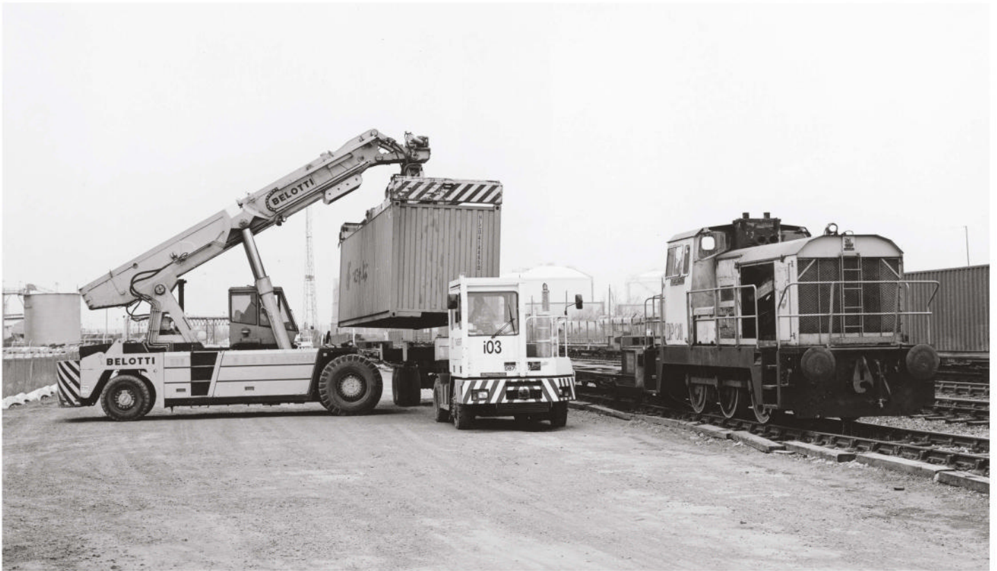
Freightliner provided an interim terminal for the newly developing Thamesport in July 1991, using sidings belonging to the BP Isle of Grain refinery. The restricted loading gauge in North Kent meant that containers had to be conveyed on low-deck FLA wagons between Grain and Stratford, where they were transhipped to and from standard wagons for the trunk journey. Thomas Hill 0-6-0 diesel-hydraulic Kentish Maid waits while loading takes place at Grain on February 19th, 1992.
