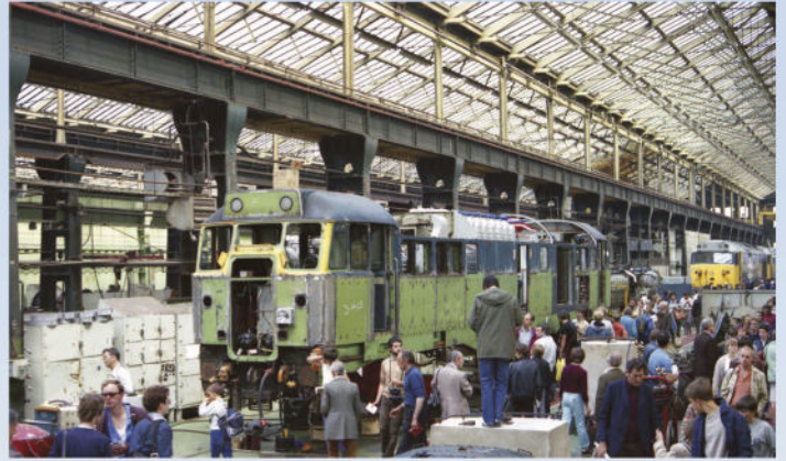
31412 is undergoing heavy overhaul in the Erecting Shop at Doncaster Plant during the Open Day on July 28th, 1984, along with an unidentified Class 50. A sealed headlight has been fitted to the Class 31 as part of the work, and a refreshed EE 12SVT powerplant is in situ. I appear to have followed the example of the chap in front of me by climbing onto some suitable object to get a better shot. The 31 was cut up in 2006.
