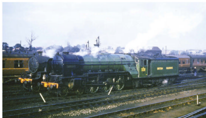
The Peppercorn A2s reverted to 'common practice' by having the cylinders placed between the bogie wheels to give a more pleasing design that also caused fewer maintenance issues, as some failings of the Thompson product could be designed out. Here we see 531 at York in Apple Green with British Railways lettering in 1949. E Sanderson/Colour-Rail.com
