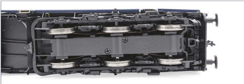
Power is supplied to all six axles.
