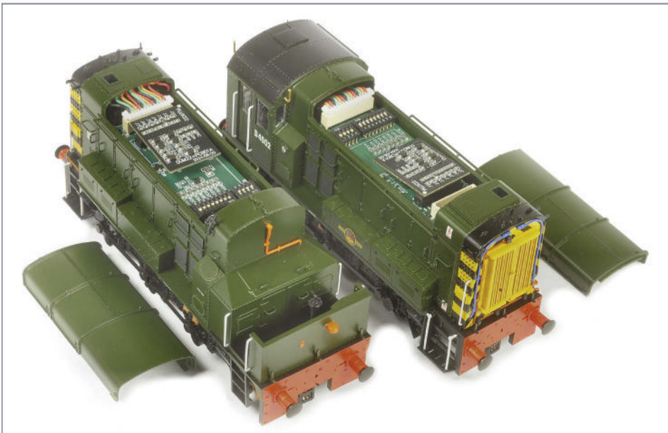
Roof panels removed to reveal the DCC sockets and microswitches for independent control of the lights in DC mode.
