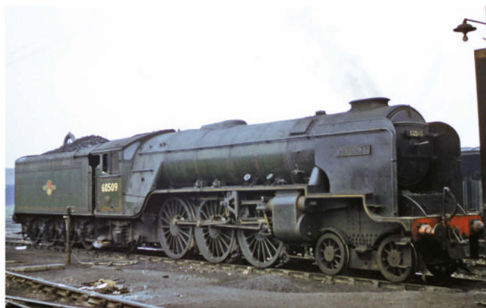
Before launching the new design of A2 (later A2/3), Thompson built two batches of prototypes. The first six were rebuilt from the Gresley P2 2-8-2s, while the second batch were new builds but based on the popular V2 2-6-2. However, both designs featured what many considered to be an ugly front-end design, with the outside cylinders behind the bogie as seen on 60509 at Haymarket shed in May 1959.
