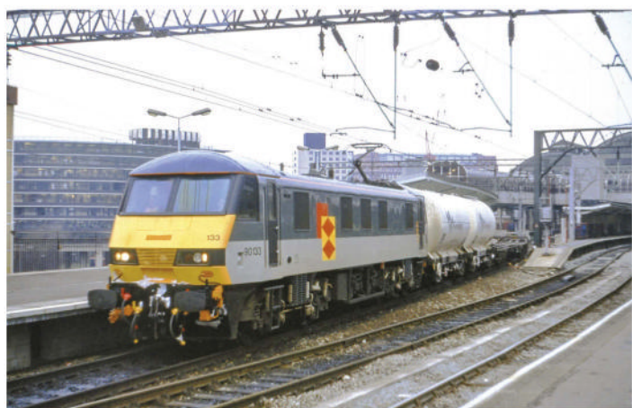
14 Class 90s received Railfreight Distribution livery, including 90033, which, after being restricted to 75mph and having its train heating isolated in 1991, was renumbered 90133. Here, the dedicated freight locomotive is seen gliding past platform 13 at Manchester Piccadilly on February 22nd, 1994, with the 13:03 SX Trafford Park West Sidings to Allerton via Crewe Basford Hall. Immediately behind the 90 is a pair of two-axle PCA powder wagons hired by Cerestar, which were carrying starch from their factory in the Trafford Park industrial estate to the paper mills at Sittingbourne, while the rest of the formation comprised a lengthy rake of empty Freightliner flats heading to Allerton for maintenance. DAVID RATCLIFFE
