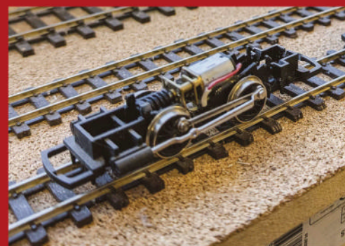
This is clever. A Hornby 0-4-0 chassis remotored with a cheap N20 geared power unit, so super-slow running.
