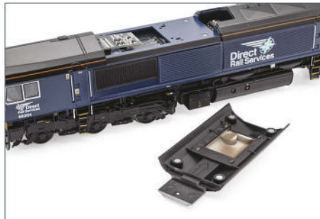
The magnetic access to the DCC area is well executed.
