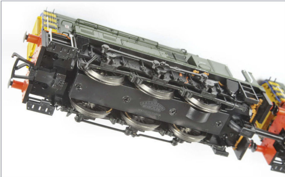
The underside of the slave unit shows one of the two fully functioning chassis on the loco.
