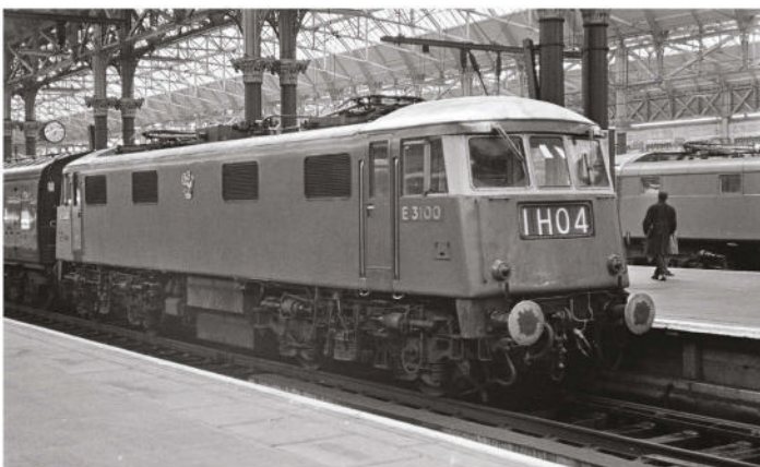
Although the final AL3 Bo-Bo electric had been intended to be E3305, it was chosen instead as a test bed for stepless voltage control and numbered E3100. Other than having ventilation louvres on the internal walkway side, rather than windows, E3100 looked much like the other AL3s built by English Electric and was photographed after arriving at Manchester Piccadilly with the 06:55 from London Euston on August 28th, 1962. D. Ratcliffe Collection
