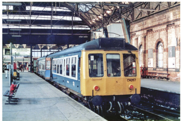
By the late-1980s, many of the local services from Manchester Piccadilly to New Mills and Rose Hill were operated by Class 108 Derby two-car DMUs. Chester-allocated set CH267, formed of Driving Motor Brake Second 51920 and Driving Trailer Composite 54276, had just arrived from New Mills Central when recorded in platform 2 on February 8th, 1989. DAVID RATCLIFFE
