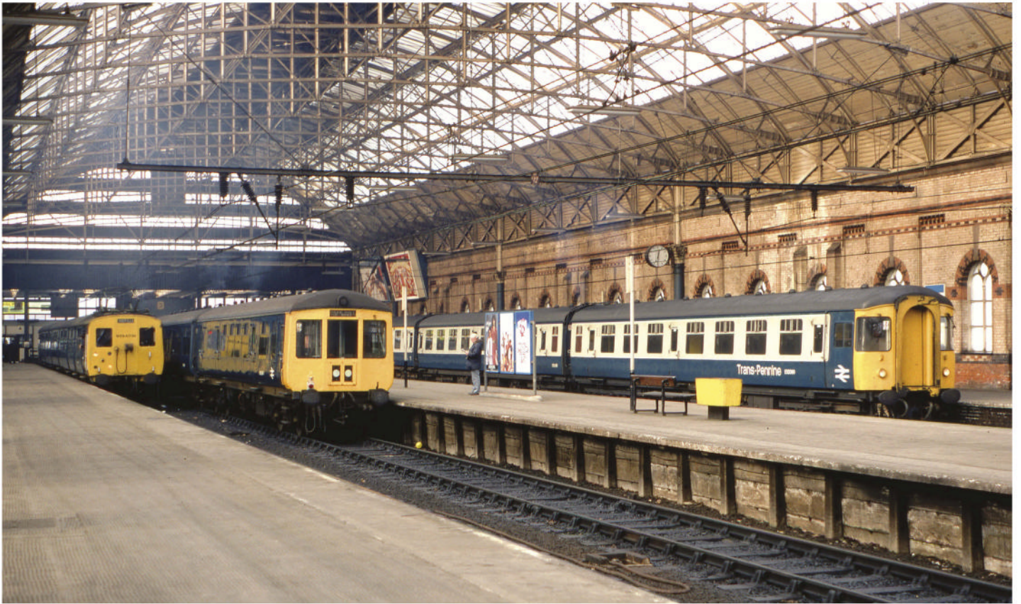
This January 1983 view of what had been the Eastern Region side at Manchester Piccadilly sees a reconfigured four-car Class 123/124 Trans-Pennine unit waiting to leave platform 1 as the 12:45 to Cleethorpes via Sheffield. Platform 3 is occupied by a Gloucester Railway Carriage & Wagon Co. Class 100 two-car 'Lightweight' DMU set. This was due to form a service for Rose Hill via Bredbury while in platform 4, one of the eight LNER-designed three-car 1500v DC Class 506 EMU sets, which were introduced in 1954, has recently arrived from Glossop.
