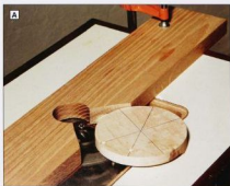
To rout the base and lid coves, fit your router with a V-block fence to help keep your fingers safely away from the rotating router bit.
