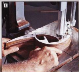
Make the final cut to free the lid as a smooth continuation of the curve that comes down the top of the tail.
