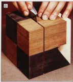
Carefully slice through the last \frac{1}{8} " by cutting down the center of the saw kerf with a utility knife.
