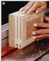
B Separate the box lid by raising your saw blade \frac{1}{2} " and cutting evenly around the box perimeter as shown.
