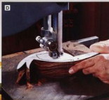
A \frac{1}{8} " bandsaw blade will help you saw the sharp inside corners in the box.
