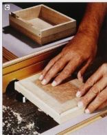
C Rout the mortises for the 114" jewelry-box hinges. Test-fit the hinges in the openings to check the depth and width.
