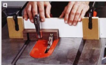
Install an extended miter-gauge fence to saw the deep dados in the body.
