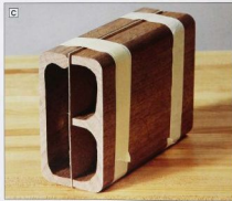
Insert a \frac{1}{8} " spacer between the lid and bottom before fitting the ends.
