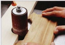
When forming the legs, use a fence with a drum or spindle sander to sand a straight edge and smooth radius.
