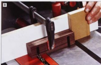
The body dados help when setting stopblocks for sawing hinge dados in the lid.
