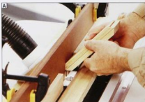
Position the front/back parts against the fence and right stopblock, and lower them onto the running bit.
