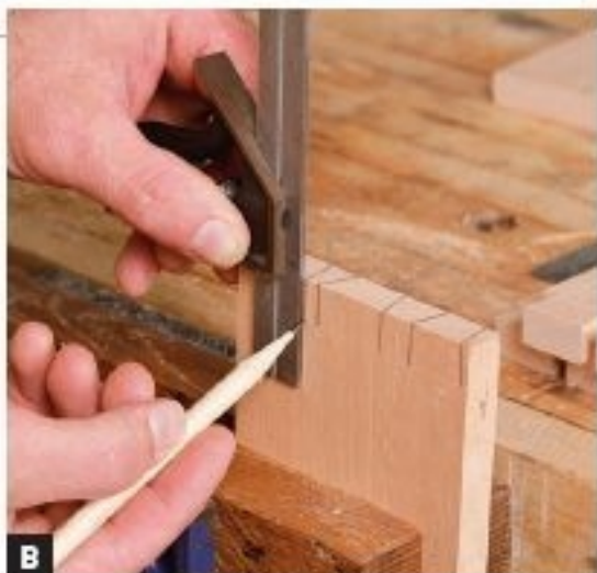
B USING A SQUARE, MARK THE FACES of the pins down to the baseline.
