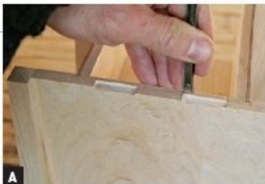
ARE THE HINGE-MORTISE walls straight with a chisel. You're cutting with the grain.
