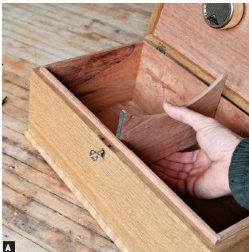
THE GLUED FELT ON THE ENDS of the dividers should make a snug, but not tight, fit.
