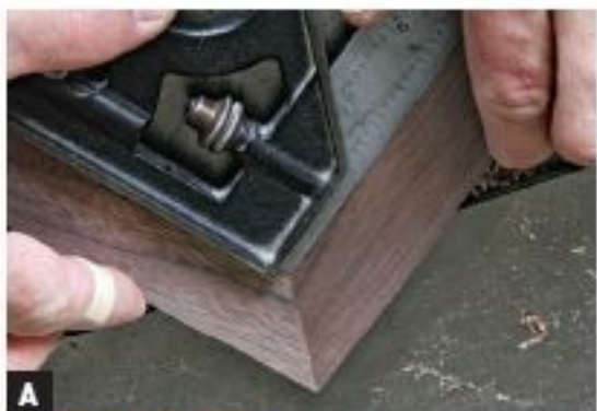
CHECK THE TEST MITER CUTS for the top trim pieces carefully. They'll be very visible in the finished box.
