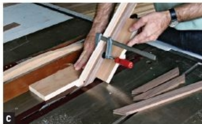
USE A SIMPLE JIG to support the trim pieces while you kerf the ends.
