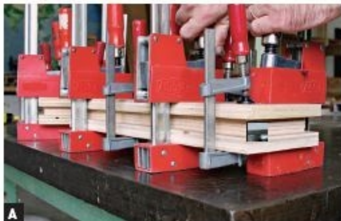
USE FLAT PLYWOOD CAULS and strong clamps when you glue up two pieces of \frac{3}{4} -in. plywood for the box sides.
