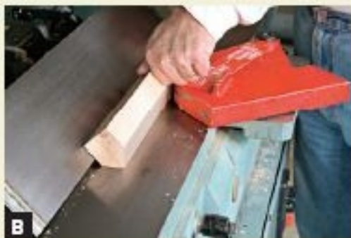
B JOINT NEW FACES on the edges of the boards at 45 degrees.
