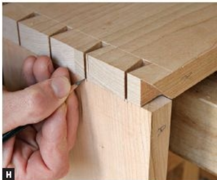
H TRANSFER THE FRONT of the pin locations to the face of the pin board. You can't reach inside with a pencil.
