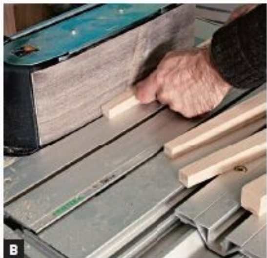
SAND THE BANDSAWN FACES of each post smooth and flat on a stationary belt sander. This tool helps keep the sanded surfaces straight, flat, and square.
