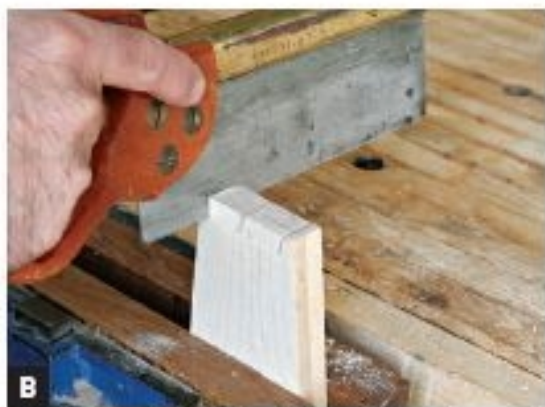
B CUT THE EDGES of the tails on both front joints at the same time. This will save you a little time and is more accurate.
