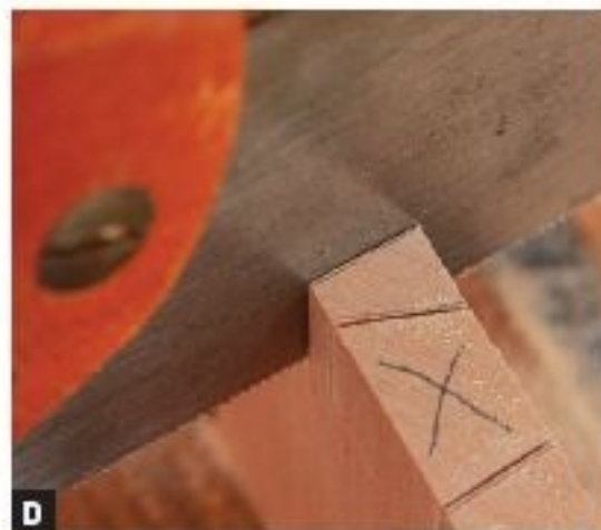
D SAW JUST TO THE SIDE OF YOUR PENCIL LINE, leaving both the line and a little bit of wood. This ensures your pins won't be too loose.
