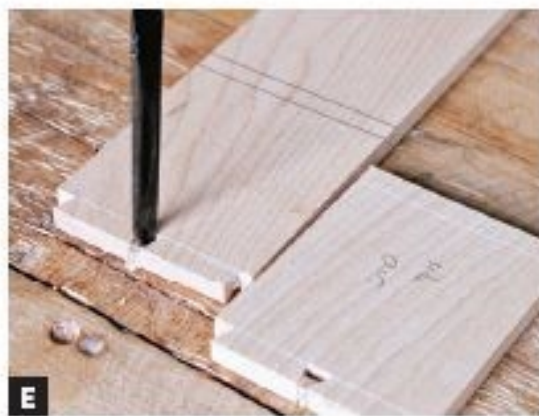
E CHOP OUT THE TAILS on the fronts of the two side pieces of the drawer with a small chisel.
