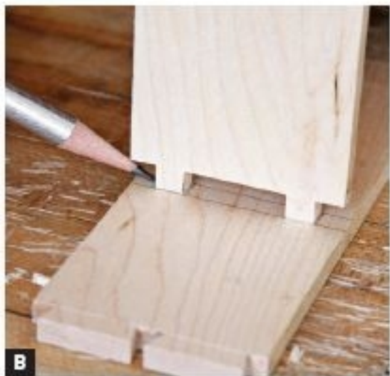
LAYOUT THE MORTISE HOLES using the tenons you've just cut.
