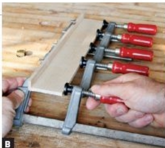
B GLUE AND CLAMP the tray side to the bottom. Check that the joint is even at each clamp and that the bottom isn't bowed.
