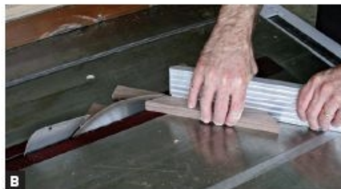
CUT THE TOP PARTS two at a time so they're exactly the same length. They're small enough to stack against the miter fence without being unwieldy.
