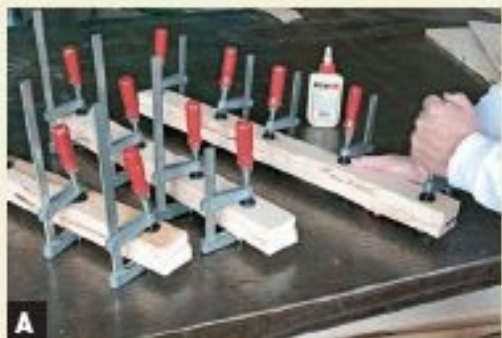
A CLAMP 2-IN.-WIDE BOARDS together face to face to create thicker stock.
