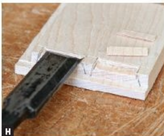
H REMOVE THE CHIPS from the end with cuts parallel to the face. Use the bench hook to keep the workpiece steady.
