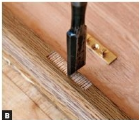
B CHOP OUT THE UPPER PLATE MORTISE to an even depth. The depth and alignment of the plate determine how well the box closes, so cut carefully.
