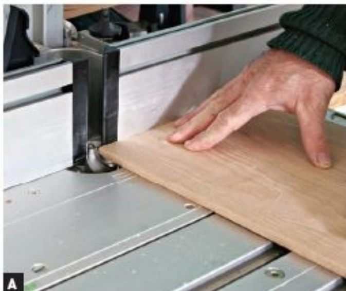
A ROUND THE EDGES OF THE BOTTOM board on a router table. Cut the ends of the board first, then the sides for best results.
