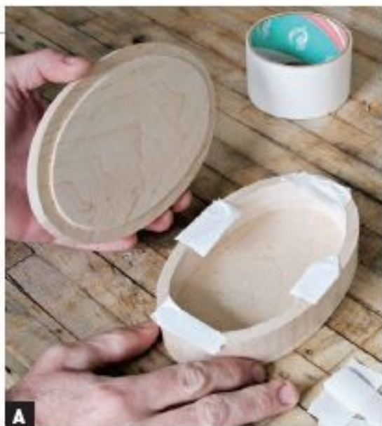
A WITH DOUBLE-SIDED TAPE , secure the lid to the box before routing or sanding the exterior.
