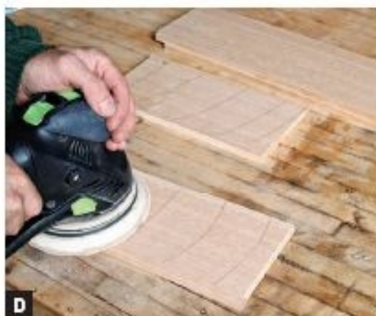
CAREFULLY SAND THE EDGING FLUSH with the faces of the sides. Try to angle the sander very slightly away from the face to avoid sanding the veneer. Use pencil marks on the face to guard against this.
