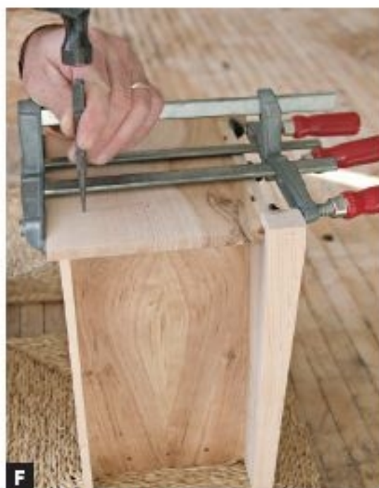
F WITH THE BOTTOM GLUED and clamped to the back, set the nails that hold the bottom to the sides.
