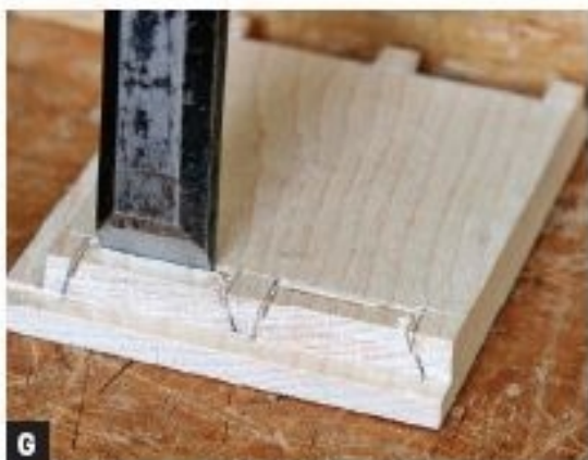
G CHOP CLOSE TO THE BASELINE with a chisel to begin removing the waste between the pins. Don't try to break out chips from this angle.
