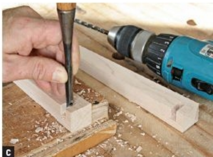
CHOP OUT THE MORTISE WASTE with a small chisel, taking small cuts each time.
