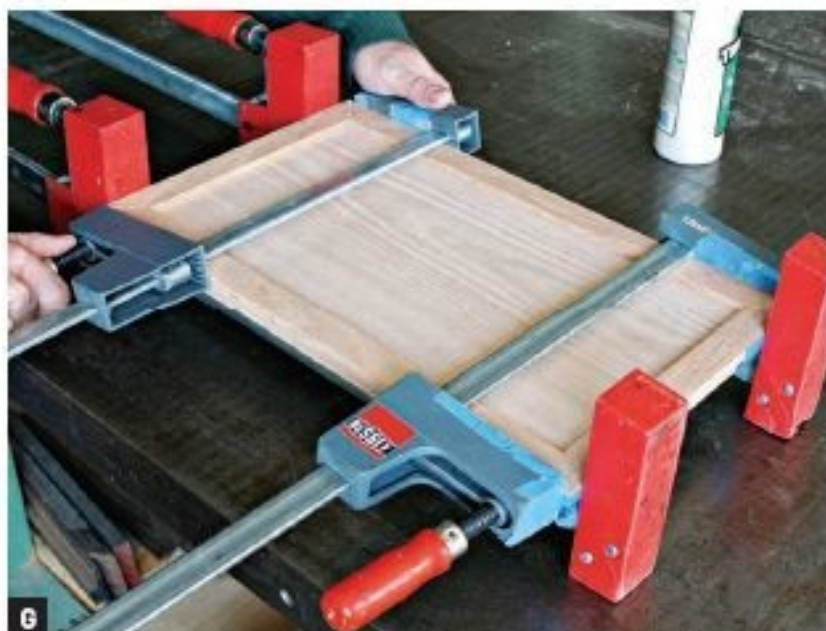
CLAMP THE TOP MOLDINGS around the plywood panel and lining. Check the corner joints for alignment and fit, both on the top and below.
