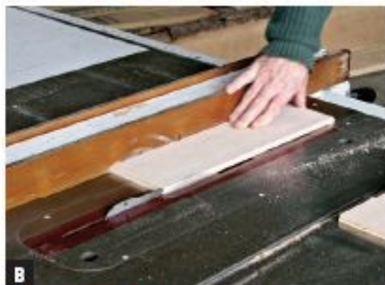
RIP BOTH EDGES OF THE PLYWOOD SIDES on the table saw. First, rip one edge over finished width, then rip the opposite edge to final width.
