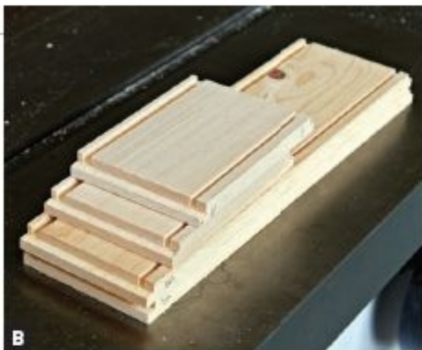
THE RABBETS AND GROOVES should be the same depth.
