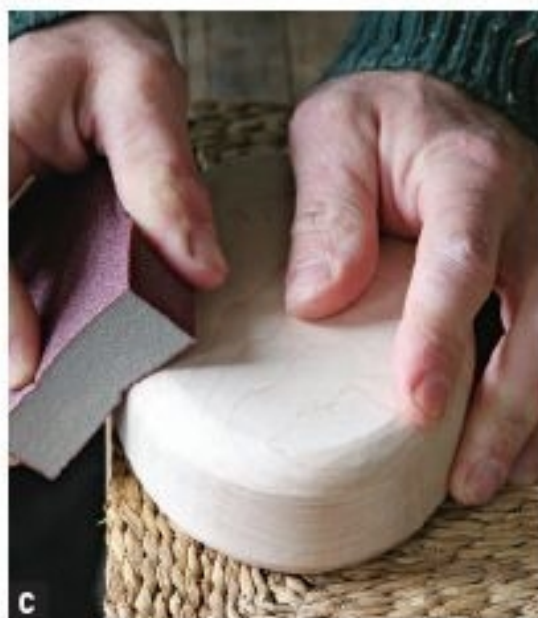
C FINISH SANDING THE EXTERIOR of the box with sanding sponges that conform to its curves.
