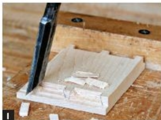
I TO REMOVE THE WASTE in the corners of the pins, angle the chisel and pare from the sides.
