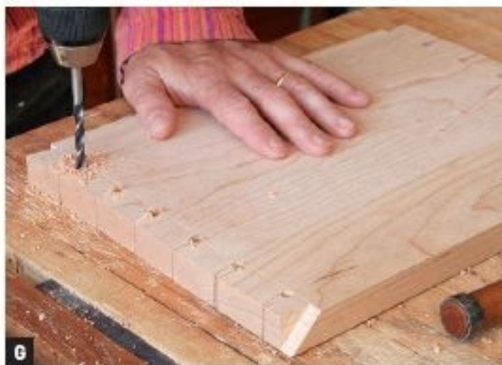
G DRILL OUT THE WASTE between tails, either with a cordless drill or on a drill press. It's faster than chopping.
