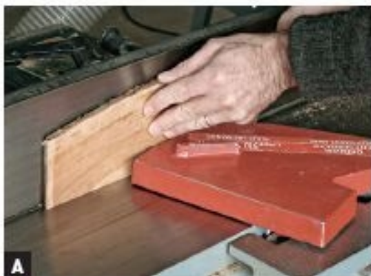
JOINT THE INSIDE EDGES of your veneer straight and square. A
