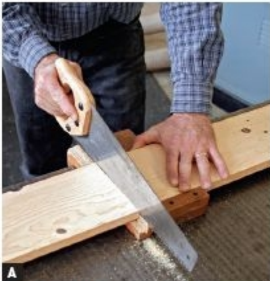
A USE A CROSSCUT SAW AND BENCH HOOK to cut your lumber to oversize lengths.
