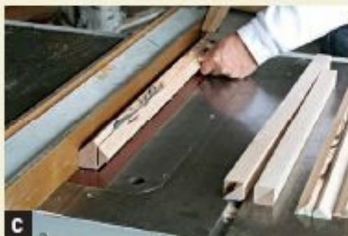
C RIP THE BLANKS SQUARE and to width on the table saw.
