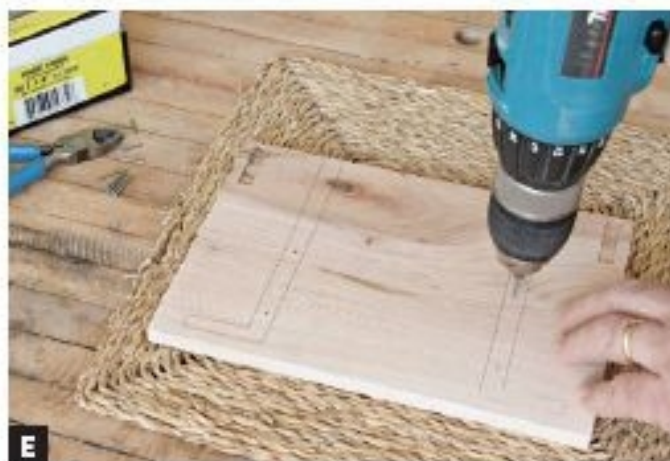
E DRILL THREE PILOT HOLES on either side in the bottom inside the layout lines that show where the interior sides will intersect. Use a 3d nail with its head cut off as a bit.
