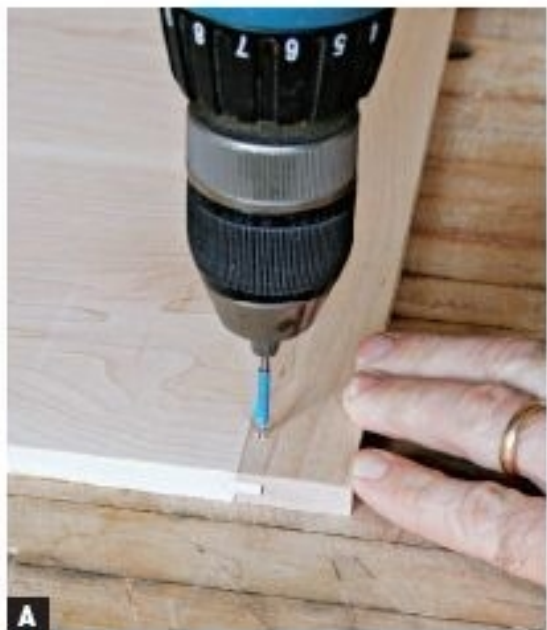
A DRILL \frac{3}{32} -IN. PEG HOLES about 1 in. from the edge of the panel, centered on the tongue and groove. To avoid drilling through, use blue tape on the drill bit as a depth guide.
