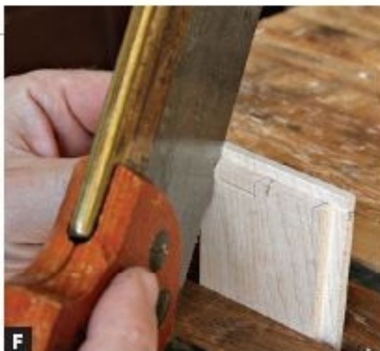
F SAW THE SIDES OF THE PINS , keeping the saw angled so that the edges of the drawer front aren't marred.
