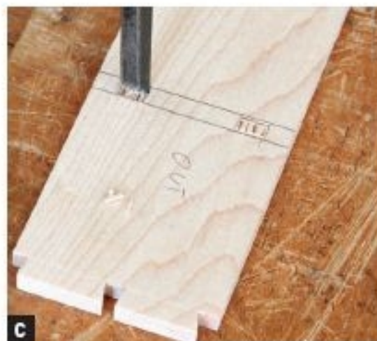
CHOP OUT THE MORTISES slowly, taking small chips at a time. Chop too vigorously and it's possible to split the board.
