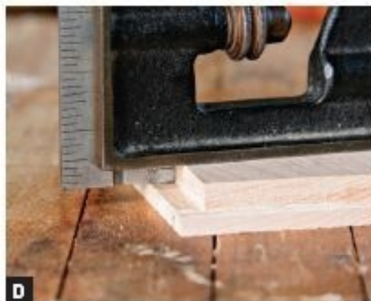
D CHECK THE ACCURACY of the rabbet with a square. Pare with a chisel to make corrections.
