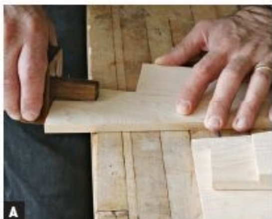
A SCRIBE THE BASELINE for the dovetails on the faces and edges of each board.
