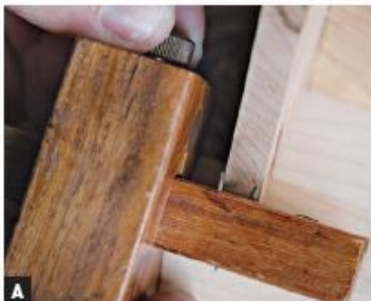
SET YOUR MARKING GAUGE to the thickness of the bottom with the fence \frac{3}{8} in. from the inside pin.
