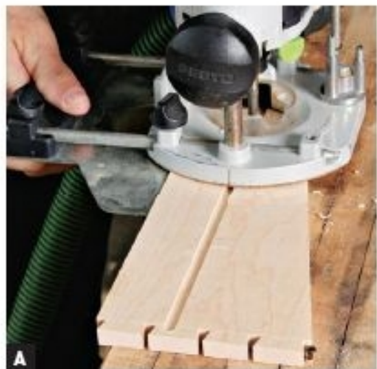
A CUT A GROOVE for the interior tray with a plunge router and straight bit. Keep the workpiece from moving by setting screws in the corners of your workbench.
