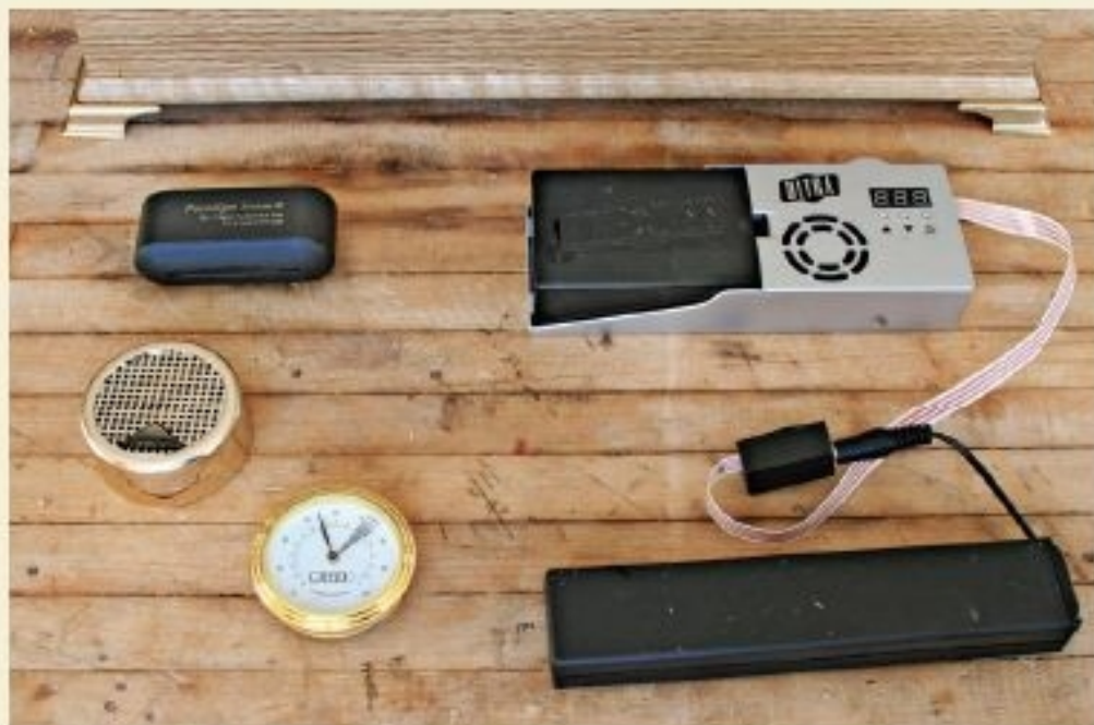
CLOCKWISE FROM TOP RIGHT: An electronic humidifier with integrated hygrometer and attached battery pack is bulky but convenient; an analog hygrometer with full humidity range indicated; two different styles of foam humidifiers in gold and black.
