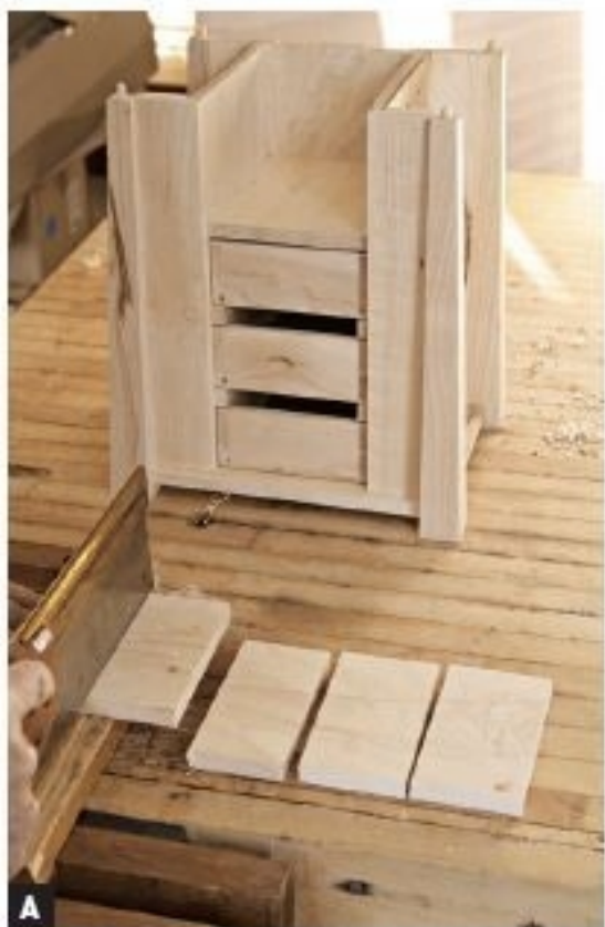
CUT A SHALLOW KERF in the false front to make it look like two drawers.
