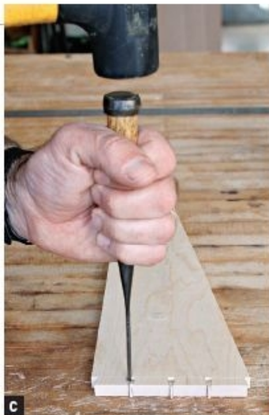
C CHOP OUT THE WASTE between tails with a chisel that fits.
