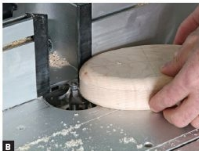
B ROUND OVER THE TOP AND BOTTOM EDGES on a router table. Be careful to push the workpiece through the cut, against the direction of the bit.
