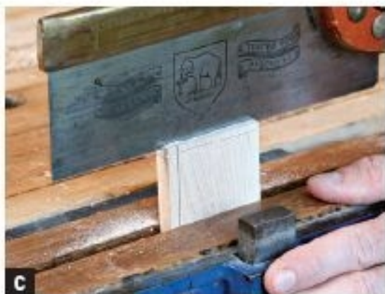
C SAW THE EDGES of the rabbets with the drawer front in a bench vise.
