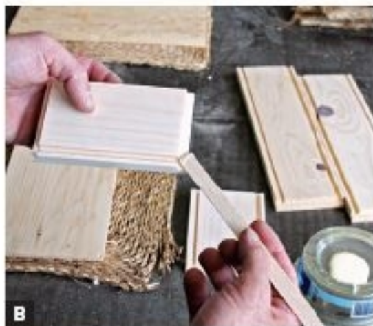
USE A STICK OR BRUSH TO DAB GLUE along the two faces of each rabbet. Be careful not to get glue in the grooves.
