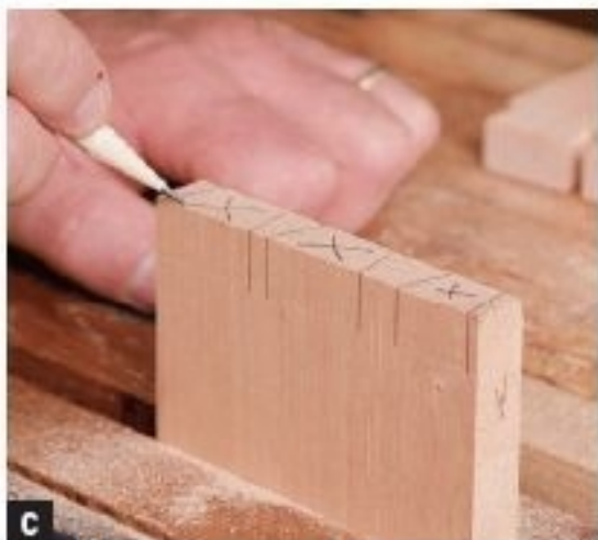
C MARK THE WASTE ON THE PIN BOARDS so you don't get confused when sawing.
