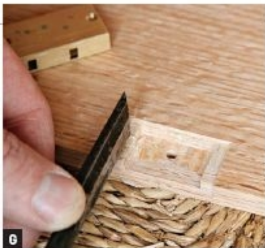
G PARE THE SHALLOW MORTISES for the lip and plate with a sharp chisel.
