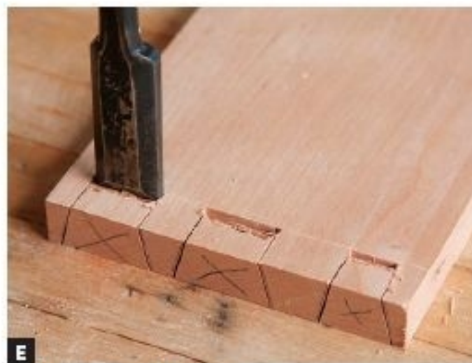
E CHOP THE WASTE BETWEEN THE PINS. You can use a smaller chisel for most of the work (they cut deeper faster). But use a wide chisel when you cut to the baseline for straight results.
