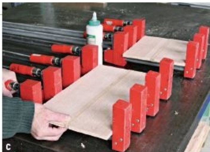
MAKE SURE YOU ALIGN the solid oak edging perfectly with the box sides. Clamp two at once, with the edging inward, to ensure even pressure along the length.
