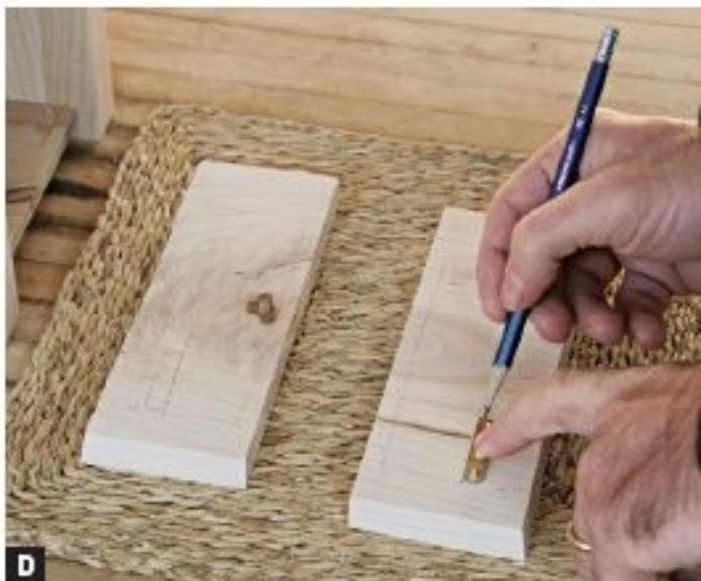
D LAY OUT THE KNIFE-HINGE mortises in the top side pieces.
