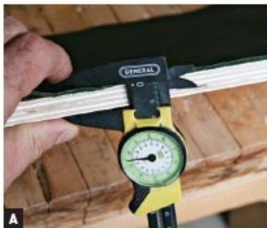
MEASURE THE TOTAL THICKNESS of the box bottom and the leather lining. Use this measurement for cutting the grooves in the box sides.
