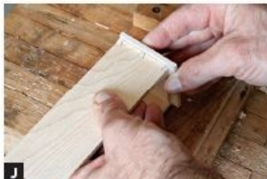
J TEST FIT THE JOINT after you've removed the waste. You should be able to push the joint together with hand pressure alone.
