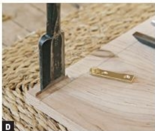
D PAVE THE KNIFE-HINGE MORTISE sides straight with a sharp chisel. Leave the layout lines intact for a tight fit.
