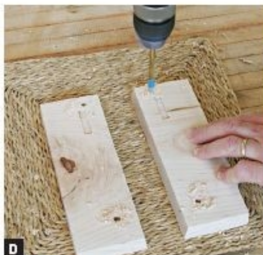
D DRILL THE OPPOSITE dowel holes in the top sides about \frac{3}{8} in. to \frac{1}{2} in. deep.
