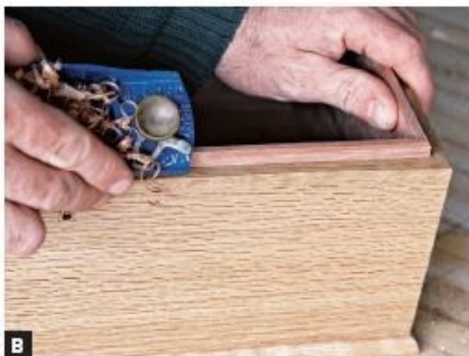
B CHAMFER THE OUTSIDE EDGES of the cedar lining. This helps the top close with ease.
