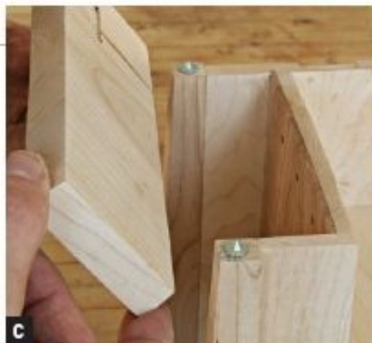
C WITH DOWEL CENTERS IN PLACE, align the top sides on the box as best you can by your layout marks.
