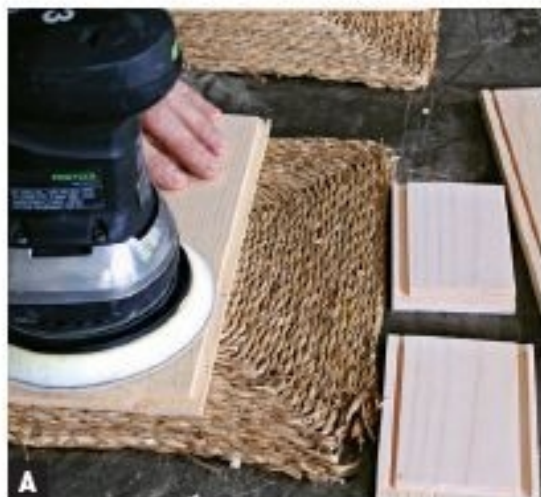
SAND THE INSIDE SURFACES OF THE BOX up to 220 grit before assembly. Use a pad to protect the soft pine from the work surface.
