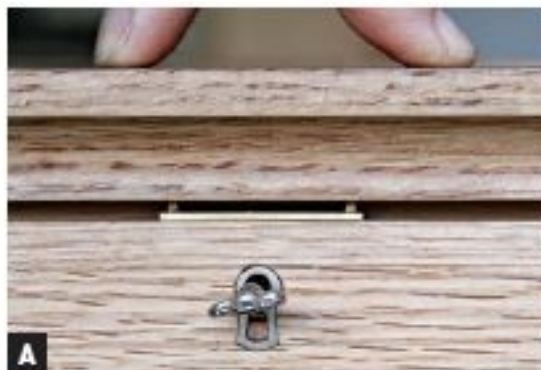
A PRESS THE LID DOWN on the upper plate (fitted in the lock). The fingers on the plate will dent the underside of the top and mark the location where you should mortise for the plate.
