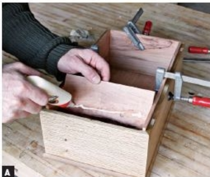
A A BEAD OF GLUE CENTERED on the back of the lining will keep it in place but let it expand and contract at the edges.
