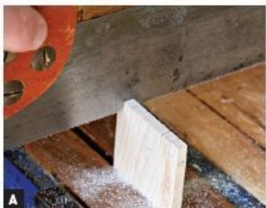
SAW THE TENON SIDES as you would a dovetail pin, but at 90 degrees to the face of the board.
