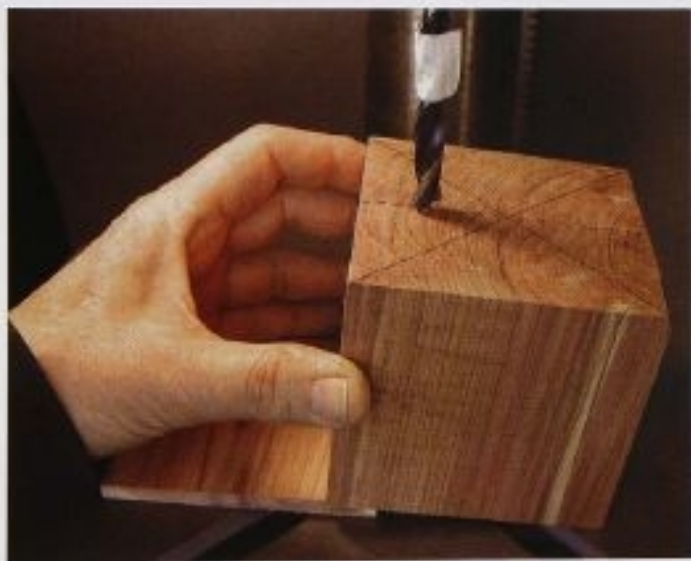
FIG. 4 Place the block on the spacer just as the template was, and the angle will be correct. Hold the block firmly, and drill the hole, using a piece of masking tape on the bit as a depth stop.
