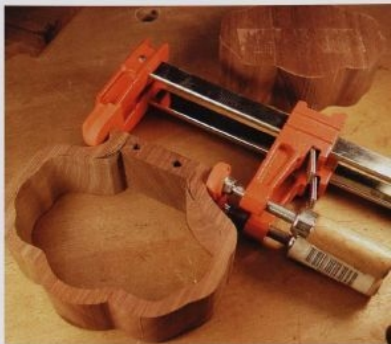
FIG. 12 With the lid carving complete, the lid and base can be cut off. Then the interior can be cut out of the body, and it can be glued together. Clamping is easy on this box.
