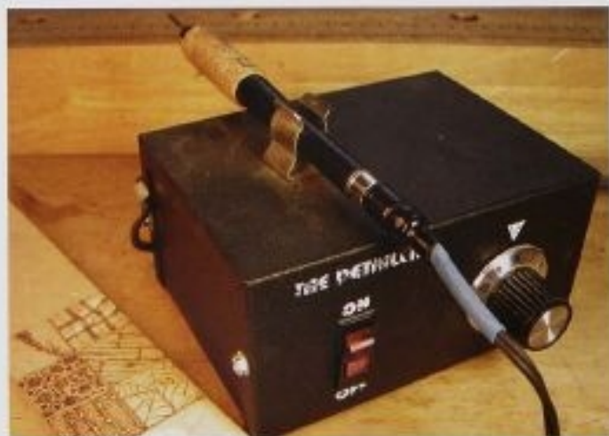
FIG. 6 A wood burner with a temperature control will make your job a lot easier and will make the project look better. If all you have is an inexpensive, stick-type burner, however, it probably will handle most of the projects in this book that call for wood-burning.
