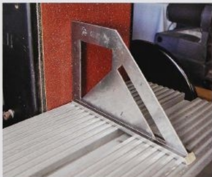
FIG. 43 This square is not expensive, so I don't mind using it to check the square of the belt sander table to the rough surface of the sandpaper. It is also a good tool to carry around in an apron pocket because it is small and expendable.
