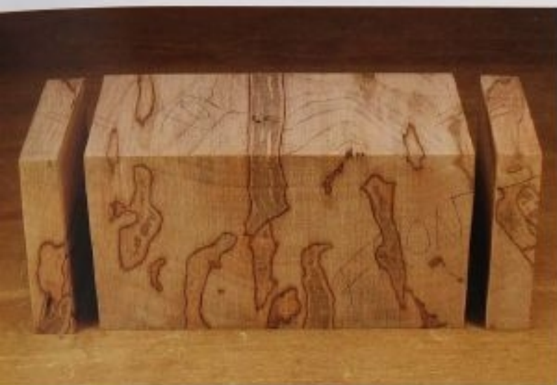
FIG. 1 To make a 7"-long box with a 6"-capacity band saw, cut wood off of each end to leave a 6" box body block.
