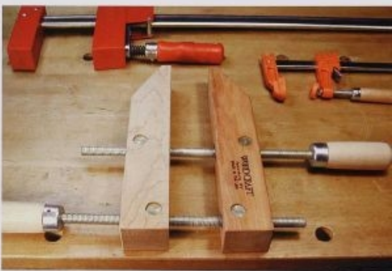
FIG. 45 Bar clamps (top) and hand-screw clamps (bottom) are very powerful and can crush small boxes if not used with great care. They also can bend a piece of wood into alignment during glue-up if that is what you need.
