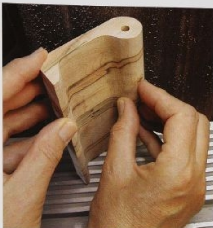
FIG. 5 If there is some deviation in the hinge, you will need to sand it to be as symmetrical as possible. Don't worry about the outside shape too much yet; just keep the hinge holes centered as best you can.
