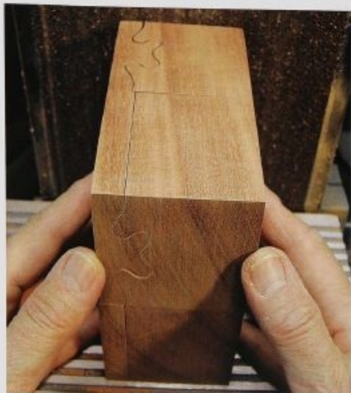
FIG. 7 Hold the boxes together while you sand with the grain on the sides. Don't let your fingertips stray into the sanding belt.
