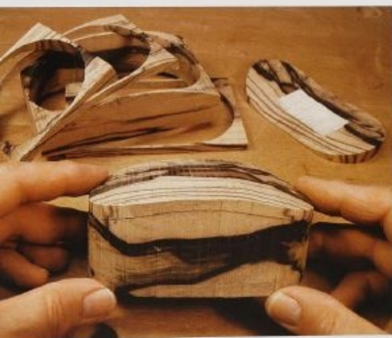
FIG. 3 After reassembling the pieces and cutting out the top view, you have a good idea of what the final box will look like.
