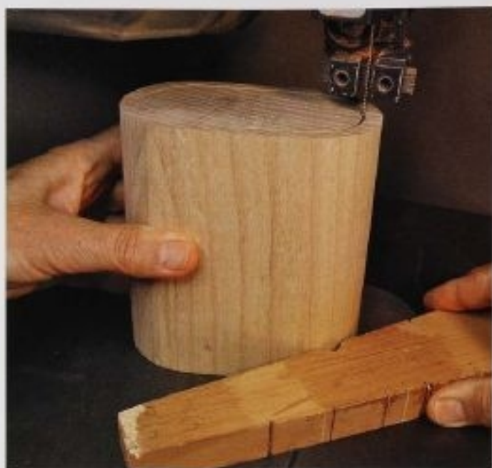
FIG. 11 On very deep cuts the blade is hidden until it emerges from the block. Keep your hands out of the danger zone, and use your push stick whenever possible.
