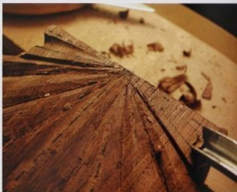
FIG. 10 To make the round-bottomed groove at the hinge end of the box, you will need a carving gouge. Here, I'm using a \frac{1}{16} " #11 gouge.
