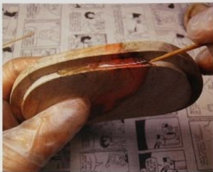
FIG. 53 For a poor fit on a curved lid, you can add epoxy around the lip. When set up, you can sand and shape it. The box will have to be finished with a surface finish.
