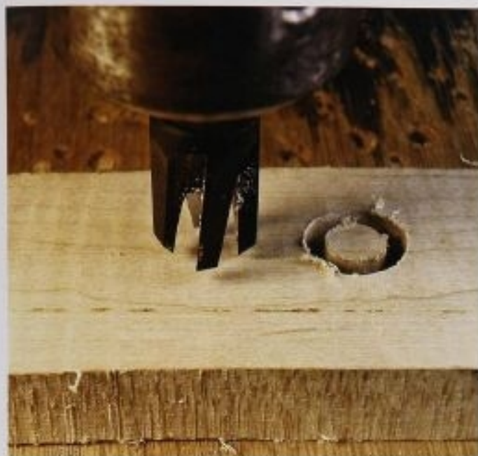
FIG. 5 A plug cutter is used with a drill press on the face of the wood to cut out the required diameter inlay plugs.
