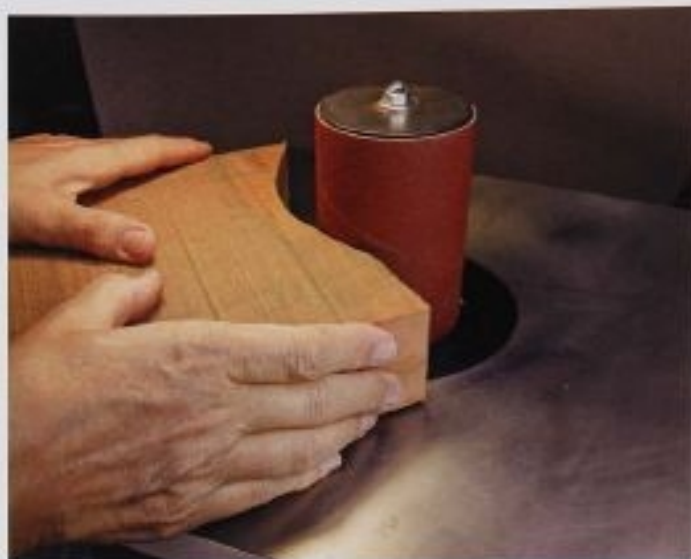
FIG. 35 An oscillating spindle sander is the best tool for sanding interior curves. Because the sanding drum moves up and down vertically, it does not make the horizontal scratches generated by a drum sander chucked in a drill press.
