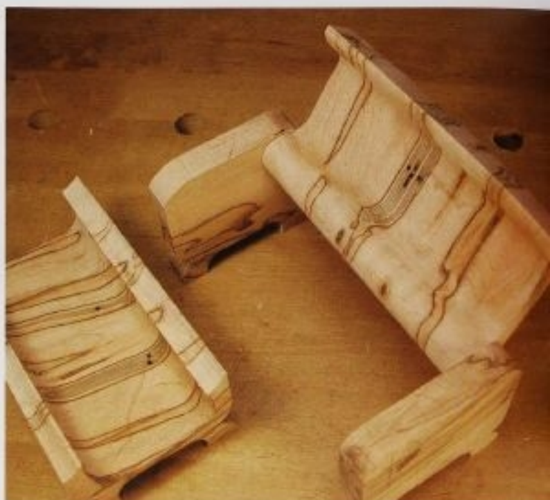
FIG. 6 The lid pivots on the hinge pins in the end pieces. When the sides are attached to the body, the lid will fall into place.
