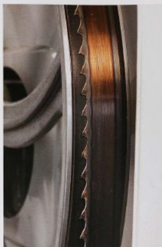
FIG. 19 This is how the blade should look when it is correctly centered on the wheel. Make sure it is centered on both wheels before turning on the machine.
