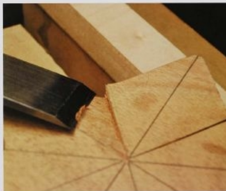
FIG. 18 First, make stop cuts straight into the wood at the inner corners of the star. Then make slicing cuts up to those stop cuts. Work from the top of the star points down to the low points between them.
