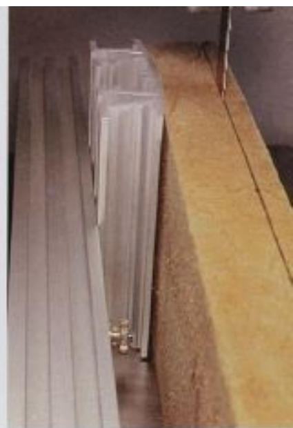
FIG. 27 Resawing and ripping with a resaw guide is one way of overcoming drift. The fence alone can also be adjusted to some extent to account for drift.
