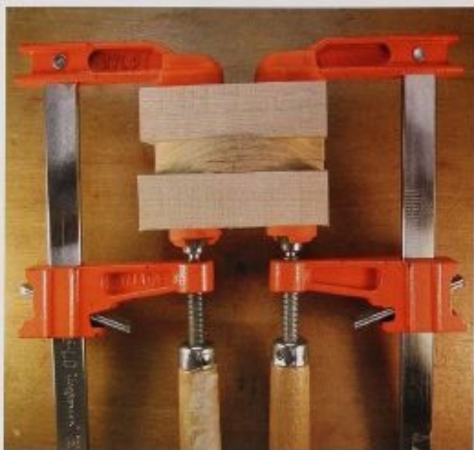
FIG. 41 If you don’t have enough clamps, a few will do. Use pieces of scrap wood to distribute their pressure evenly on your project.
