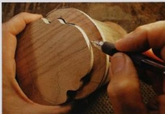
FIG. 11 Once one end of the lid is fitted to the box body, you can use the profile of the end piece to mark where the wood needs to be removed. Be careful to keep the same orientation throughout the process. Because the ends probably are not identical, don't make the mistake of turning the lid around and tracing the wrong profile.
