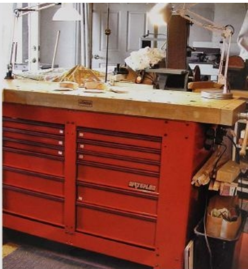
FIG. 42 My workbench is one of the most used tools in my shop. I can store small tools in the shallow drawers, and the well-lighted surface is used for all layout and glue-up. Sanding and finishing are done on other benches.
