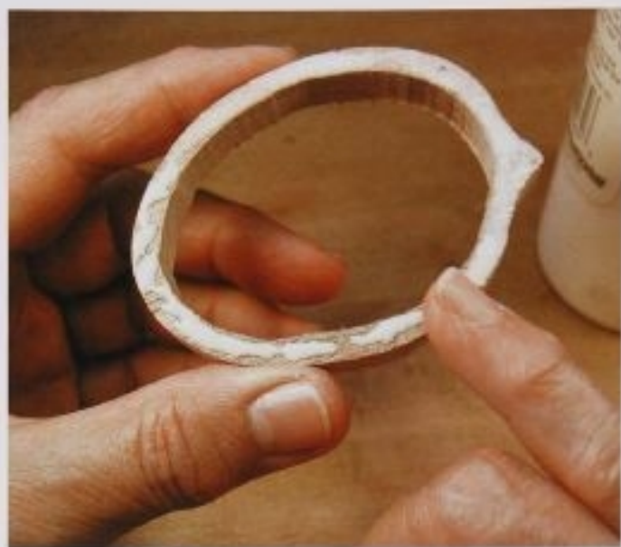
FIG. 40 Using your little finger to spread wood glue is not very high-tech, but it works well. You can precisely place the glue, as here, to keep squeeze-out toward the exterior edge of a box.
