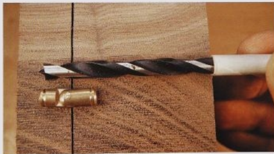
FIG. 3 By laying the hinge in place on the box, you can double-check that the drilling depth will be sufficient. Mark the depth with a piece of tape on the drill bit to easily see where to stop.
