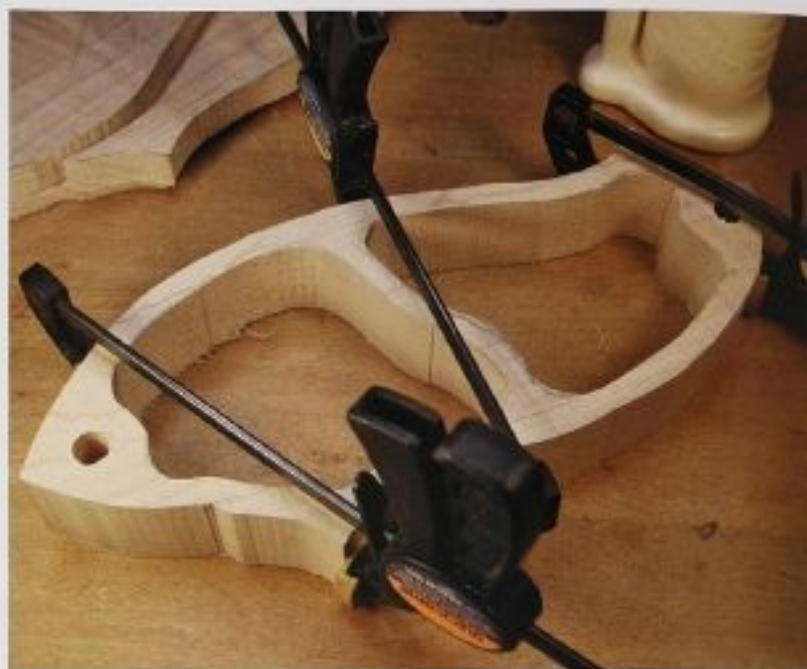
FIG. 2 Clamp at each of the glue joints, making sure that the edges are even and have not slipped out of place.
