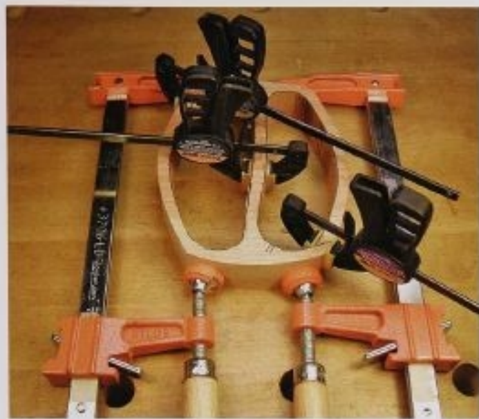
FIG. 39 Doing a dry run will keep you from putting glued surfaces together and then realizing that the clamps are too short and the ones you need are located at the other end of the shop.
