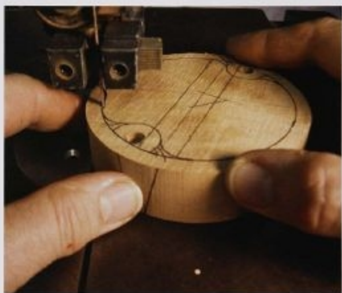
FIG. 8 Cut out the interior of the body, being careful to leave enough wood around the holes. Remember, the boxes are mirror images of one another so one interior pattern will be the reverse of the other.
