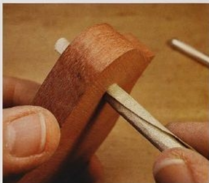
FIG. 8 Roll a section of sandpaper into a rod shape that can be used to make the holes in the lid and body a little larger, if necessary. You want the fit to be firm, but loose enough to allow the lid to pivot in the body, and to allow the pin to be epoxied into the lid.
