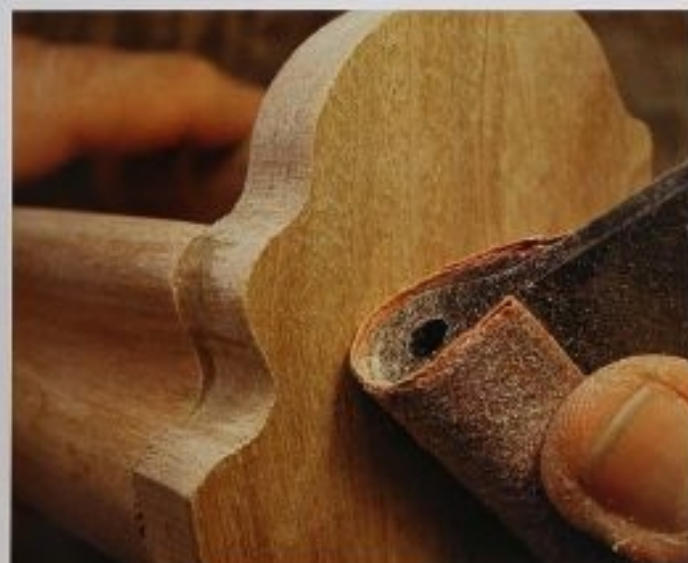
FIG. 10 Using rubbery profile sanders saves your fingertips and results in a nicely rounded, smooth finish in the coved areas.
