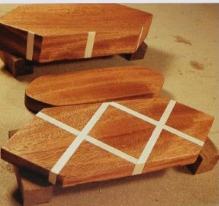
FIG. 9 The parts drying again after being finished with tung oil. It is easier to go through the entire finishing process without the hinges getting in the way. Reinstall the hinges after the finish is applied.
