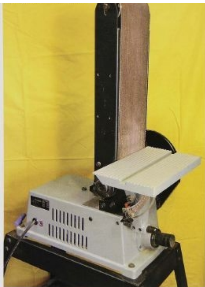
FIG. 29 This 6" belt sander ("Big Bertha"), seen from the left, gets more use than any other tool in my shop except the band saw. It has a 1-HP motor that is unstoppable, so watch your fingers!
