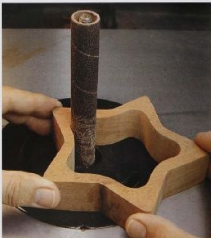
FIG. 15 An oscillating spindle sander makes light work of sanding the interior. This job also can be accomplished with a drum sander, or by hand. Always sand the interior before assembly.
