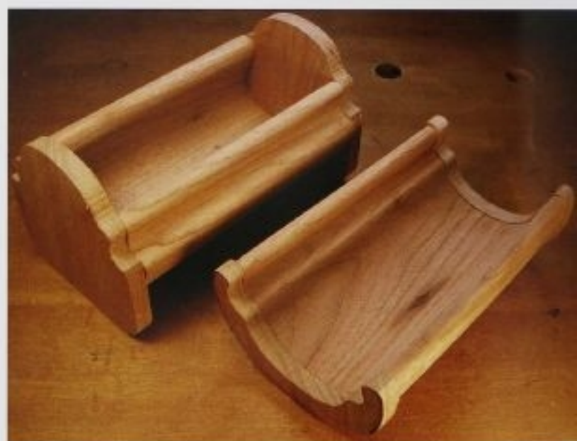
FIG. 7 The box looks almost done after the clamps are removed, but there is still a lot of work to be done. First, the sliding mechanism needs to function smoothly, and then the box can be sanded to a beautiful finish.
