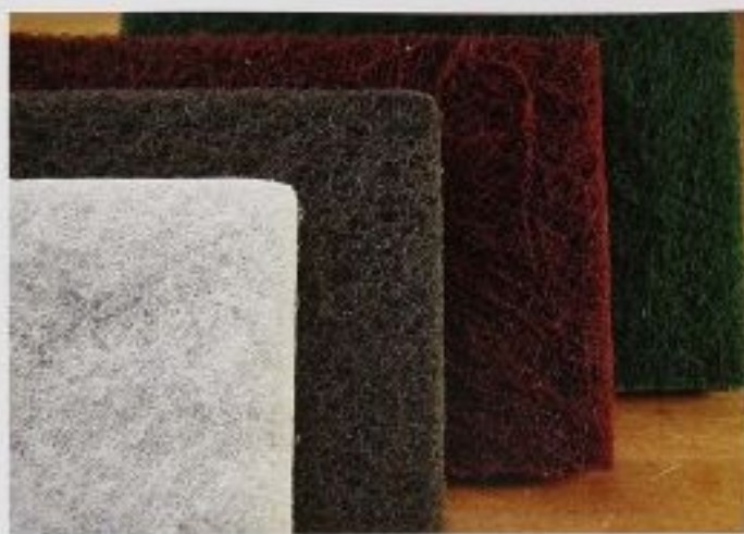
FIG. 38 Abrasive pads (scrubbies) range from very fine, the white pad, to very coarse, the green pad. Use them instead of sandpaper between coats of finish.
