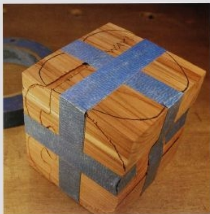
FIG. 8 After cutting the first outline, again reassemble the cut-off pieces and tape all back together again. Match up the cut ends of the old masking tape as a guide for the correct location for the new tape. Then make the second outline cut.
