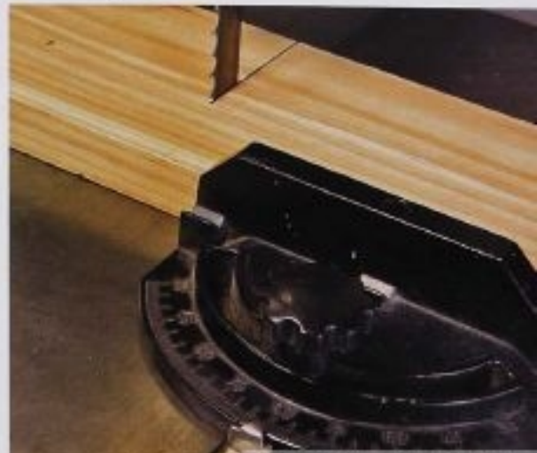
FIG. 14 The miter gauge keeps the wood perpendicular to the blade for crosscuts (cuts across the grain). Band saws do not make the best crosscuts because of the tendency of the flexible blades to twist with the movement of the wood and wander off course (drift).
