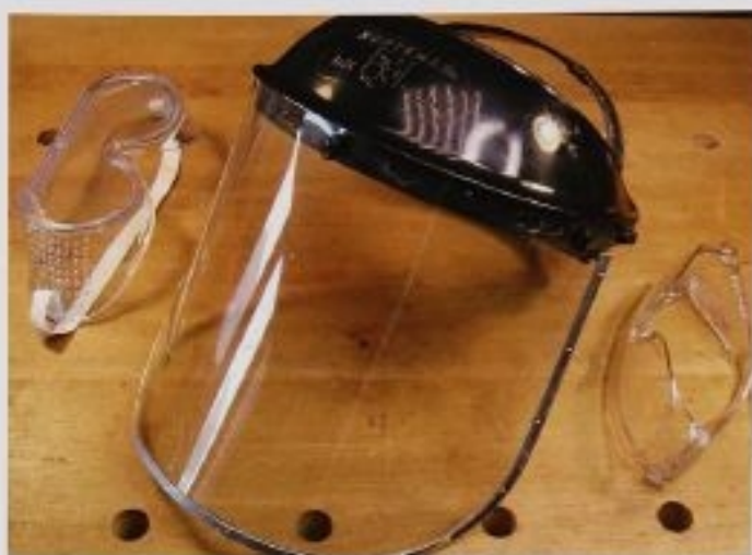
FIG. 4 Three different types of eye protection. On the left are inexpensive goggles that will do the job, but are not very comfortable. In the middle, a full-face mask that will protect your facial bones as well as your eyes. On the right, safety glasses that are comfortable to wear; some even fit over your glasses.
