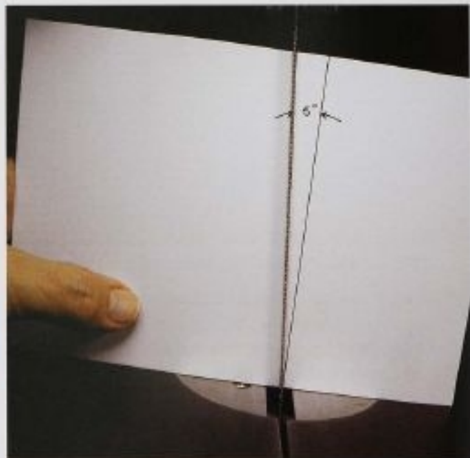
FIG. 12 Use the same template you made earlier to adjust the band saw table for a 5° cut.
