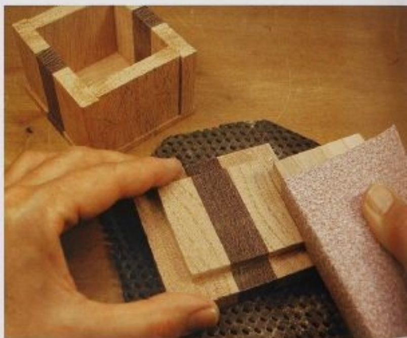
FIG. 6 The sides moved during glue-up, and the lid liner no longer fit. Sand the lid liner with sandpaper wrapped around a block of sharp-edged wood to keep the edges flat and square. Work to keep the stripes in alignment as you remove wood.
