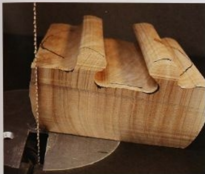
FIG. 13 Double-check that you are starting the cut on the correct side of the body. Put the body on the downside of the blade.
