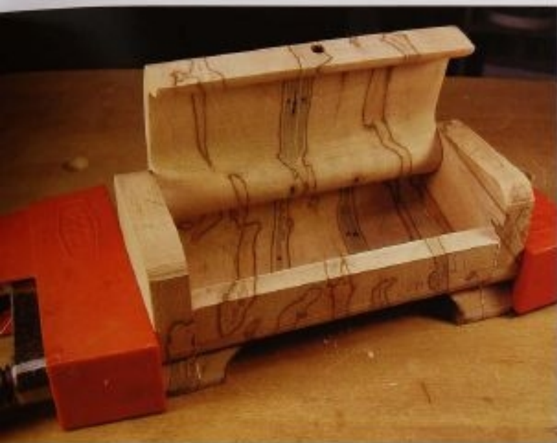
FIG. 8 The big-boy clamps come out for this glue-up. This large parallel clamp makes an easy job of applying even pressure, but you could use three regular clamps instead.
