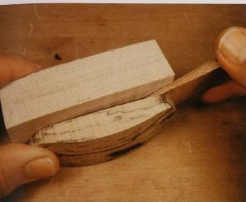
FIG. 5 Use a wedge-shaped piece of wood to carefully pry smaller pieces of wood from the stabilizing block.
