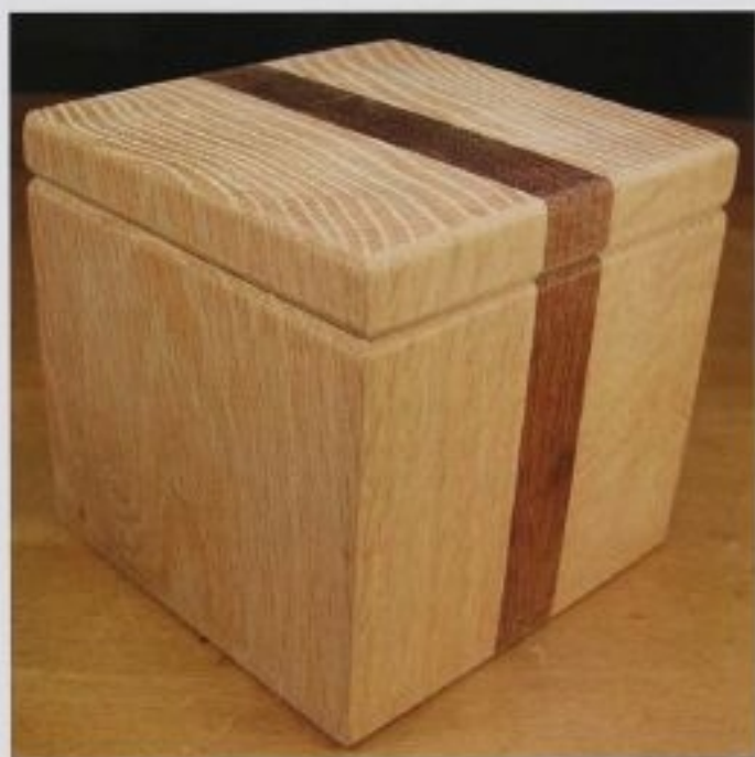
FIG. 9 Chamfers at the meeting of lid and body effectively disguise the alignment error. Chamfers make the box easy to open and look good.
