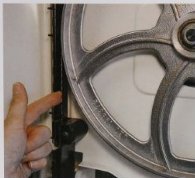
FIG. 20 Pluck the blade between the wheels on the support-arm side of the machine to determine optimum tensioning by tone. Listen for the “twang.”
