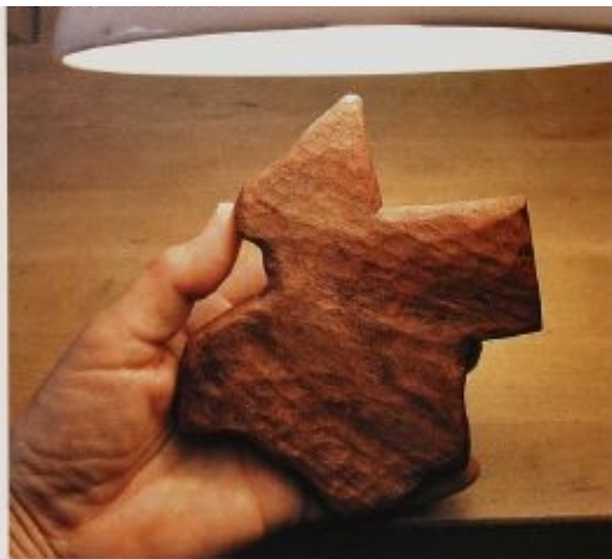
FIG. 1 Looking at your project under straking light, that is, light coming at an acute angle to the wood, will show any defects.
