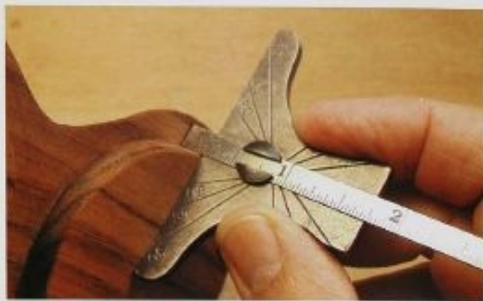
FIG. 46 This inexpensive depth gauge is useful when making band saw boxes. Here I'm using it to measure the thickness of the lid liner of a box.
