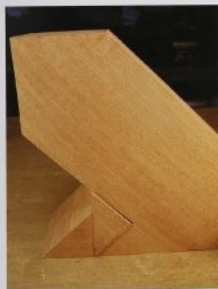
FIG. 1 To support the box block at the required 45° angle, use the scraps that you generated when you cut the ends off, or cut another piece of scrap to a 45° angle.
