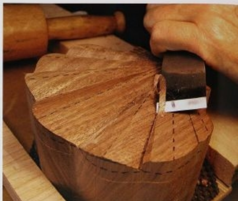
FIG. 8 Keep your chisel sharp enough to slice through the wood cleanly with just hand pressure. You'll get a better finish that will require less sanding. Notice how the edge of the blade is cutting with the grain. If the chisel digs into the grain, you're going in the wrong direction.
