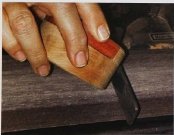
FIG. 11 The edges also can be rounded freehand on the belt sander if you have good eye/hand coordination and you check your progress frequently.
