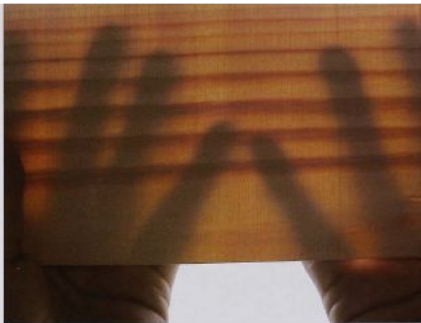
FIG. 12 Thin stock can be cut smoothly and evenly with a \frac{1}{8} " 4-TPI (tooth-per-inch) blade on a 14" band saw with a good fence, slow feed rate, and a steady hand.
