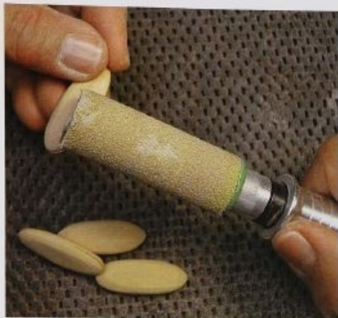
FIG. 8 If you keep the two petal layers taped together while you sand them to form, they will be easier to handle. Watch your fingers when you power-sand such small pieces.
