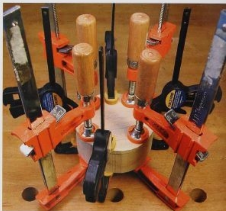
FIG. 42 You can use one-handed quick-type clamps to align your pieces to be glued and then add screw-type clamps for more pressure, if necessary.
