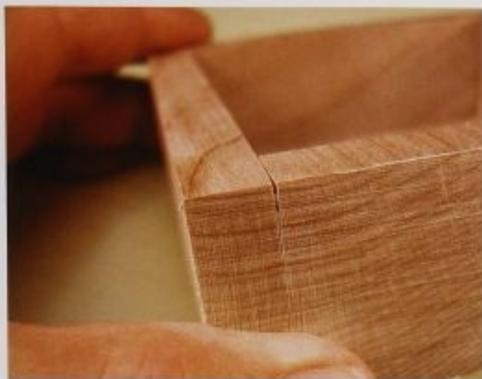
FIG. 43 Oops! My edge-sanding must have been crooked, and now the corners don't meet squarely. When filled with a wood glue and sanding dust mixture and then sanded flat, the repair will be invisible.
