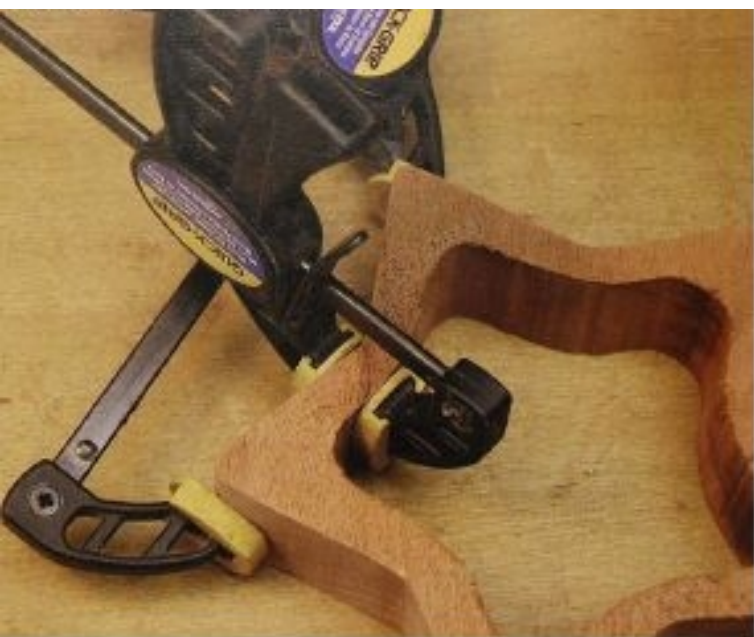
FIG. 13 Use two clamps to hold the body joint together: one to hold the sides in alignment and one to close up the kerf. Light-duty clamps are best for these jobs, where too much pressure could break the wood.
