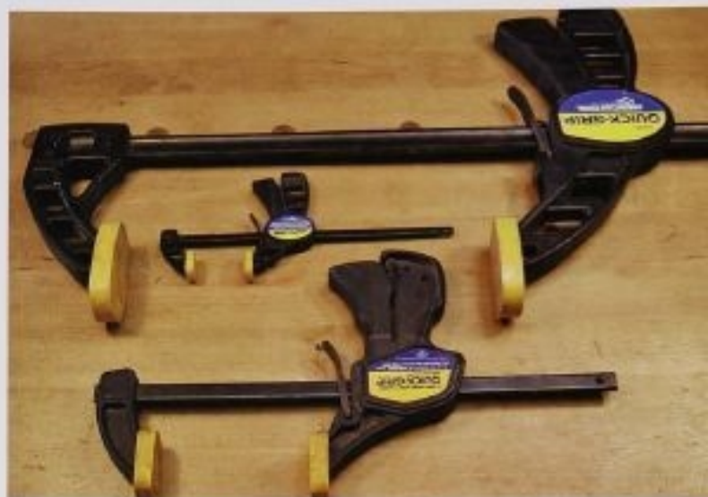
FIG. 44 One-handed clamps are quick and easy to use and they can apply enough pressure for most box-making purposes.
