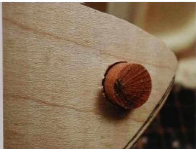
FIG. 4 The fit of this hinge pin was not good enough to secure with just glue. I mixed some fine sanding dust with glue to make a paste to put into the hole and around the dowel. Use a square to keep the dowel perpendicular to the lid as the glue sets up.
