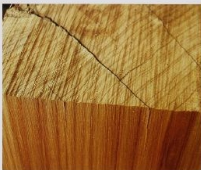
FIG. 1 The depth of surface cracks in found wood determines whether the wood is good enough for making boxes. Notice the difference in color between the top (exposed) surface and the newly cut vertical grain.
