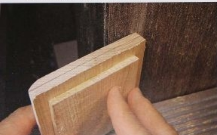
FIG. 10 Hold the wood so it meets the belt evenly, and keep it on the table as you move it smoothly from pencil line to pencil line until you have generated a pleasing curve. Sand just to the center of the pencil line so the remaining half line can continue to act as a guide as you change to finer grits.
