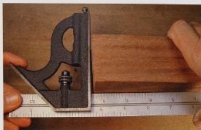
FIG. 16 While squaring up a block, use your combination square to determine which of the two sides of the block is closest to square with the top. In this case, this is not it; there is a large gap between the combination square and the side of the wood.
