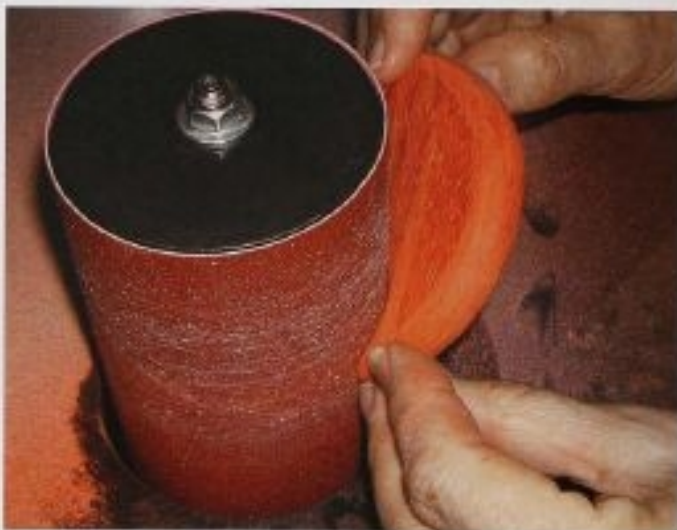
FIG. 12 Sanding the top of the lids' meeting edges is made easier with an oscillating spindle sander, but it can also be done with a drum sander in a drill or with a power rotary tool. Do not round over more than halfway through the thickness of the lids.
