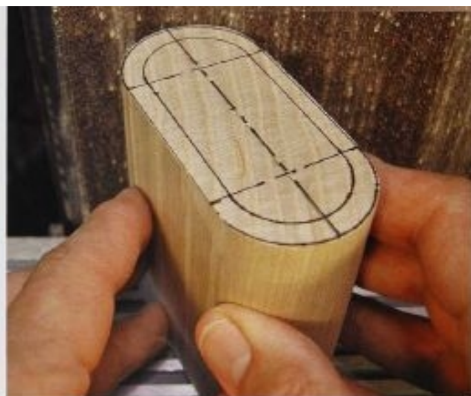
FIG. 3 Use a coarse grit sanding belt to sand to the line. Keep your fingers away from the moving belt. It gives a rough manicure.
