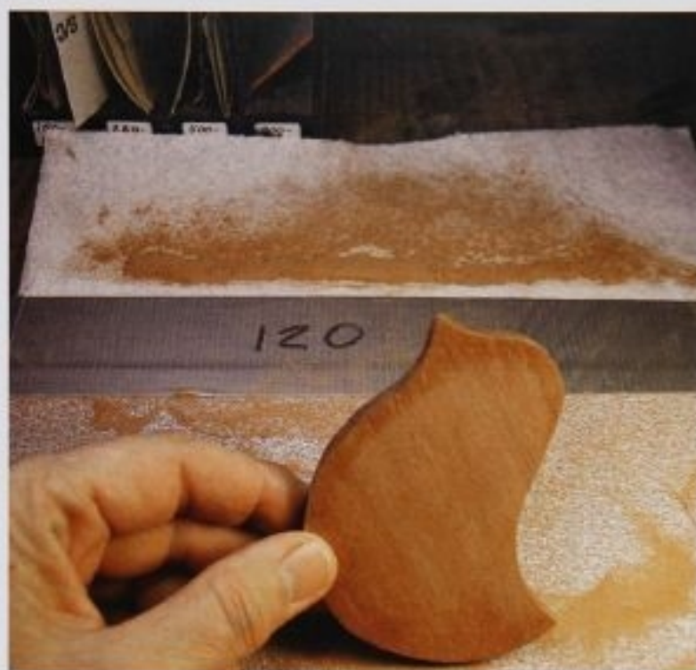
FIG. 5 A small problem with the sanding belt resulted in a big hand-sanding job using sanding boards. The pile of sanding dust on the paper towel will be saved for use in filling gaps in other boxes made of koa.
