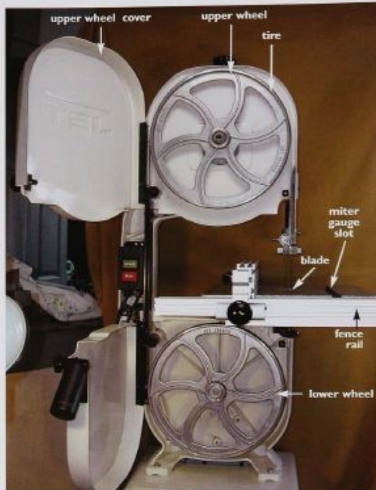
FIG. 2 Opening the wheel covers exposes the wheels, on which rubber tires are mounted. The blade rotates on the tires.
