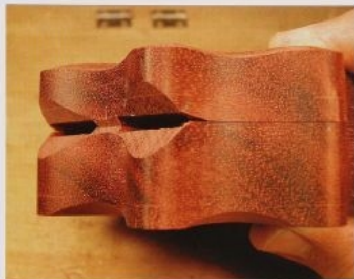
FIG. 3 The hinge mortises need to be deep enough to accommodate the hinges. Put the lid on the body, and check that the holes are even and that they line up. This photo also shows the material removed at the rear at a 45° angle to enable the box to open.
