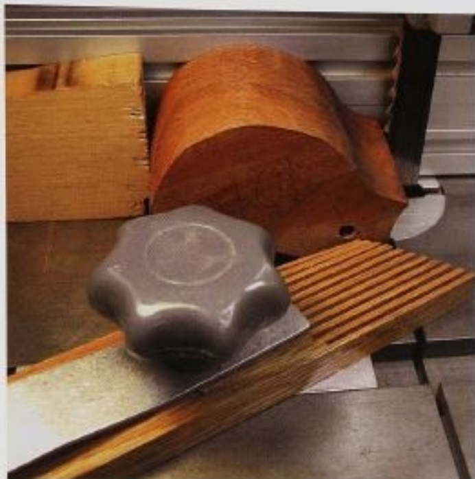
FIG. 1 Use a feather board and push stick to be safe. Keeping the head and tail on the table creates a fairly stable arrangement, but keep some pressure on the piece to hold it to the table as it is being cut.
