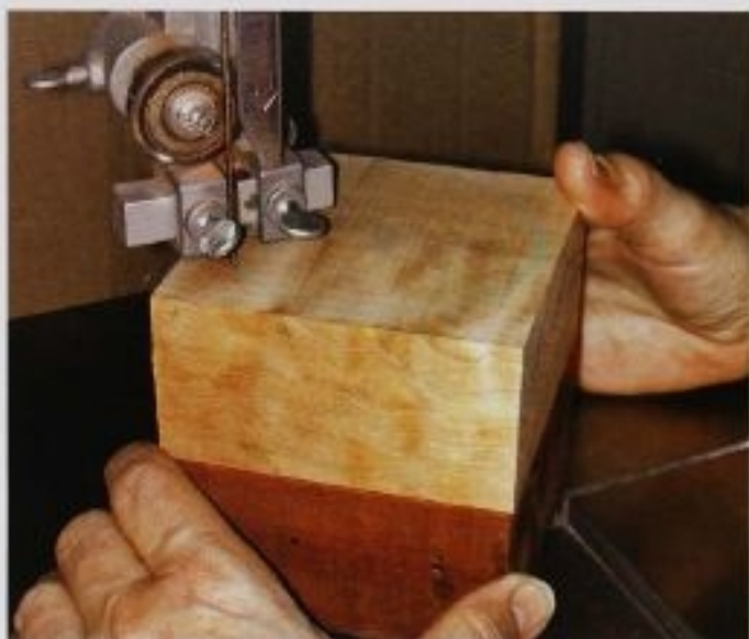
FIG. 1 Cutting through 4" of hard wood is difficult for a \frac{1}{8} " blade, so go slowly. For such a large circle, a \frac{1}{4} " blade could be used, but then you would have to change blades for the interior cuts.
