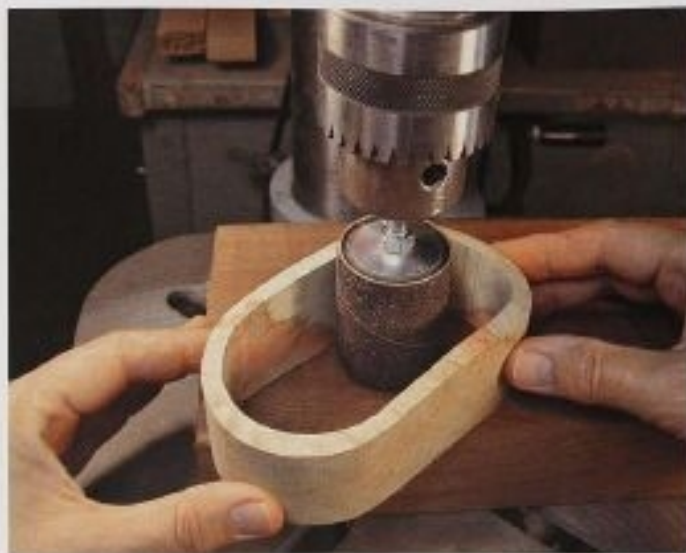
FIG. 33 Drum sanders, such as this 1 1/2" diameter one chucked in the drill press, will work for sanding interior contours.
