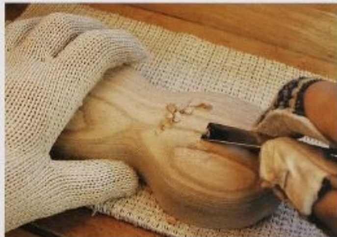
FIG. 2 Overlapping shallow slicing cuts produce a pleasing overall texture on this Peanut Box.
