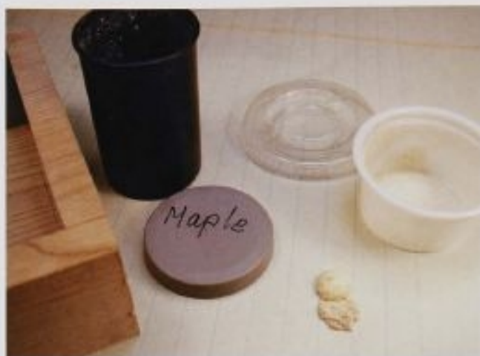
FIG. 44 I keep some extra sanding dust in small containers like this condiment cup and film canister. That way I have a supply ready to use for a quick fill. Add the wood dust to the drop of glue until you have the consistency of toothpaste. Use it quickly, before it dries.
