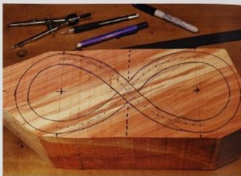
FIG. 2 Size the plans to fit the block of wood available. There is no need to keep to the size of the plans in this book. Just proportionally shrink, or enlarge, all of the drawings and dimensions. Dashed lines indicate relief cuts. Notice that this model was made with the opposite crossing to that of the plans. Oops!
