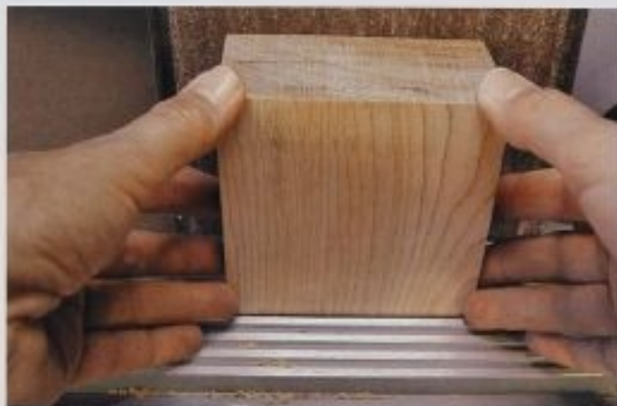
FIG. 32 When flattening a large surface, keep pressure evenly distributed across the block and watch your fingertips! Your touch needs to be firm, yet gentle. If you press too hard, you may take off more wood than you want.
