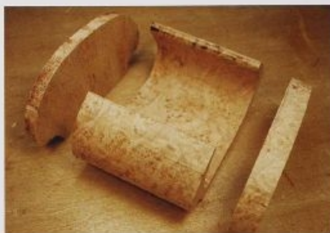
FIG. 3 Here the drawer pieces have been cut from the core. Notice that the band saw blade is beginning to burn the wood, a sign that the blade needs to be replaced. It broke while working on the next project.
