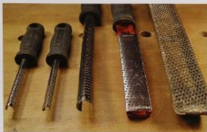
FIG. 39 Planing rasps leave a very smooth finish on the wood. From the left are small round, small square, large round, flat, and heavy duty planing rasps.
