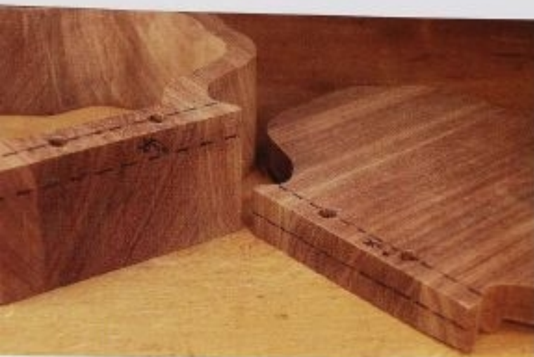
FIG. 13 Mark the lid and body for the centerline of the hinges. The hinge chamfer must end at the center of the holes.
