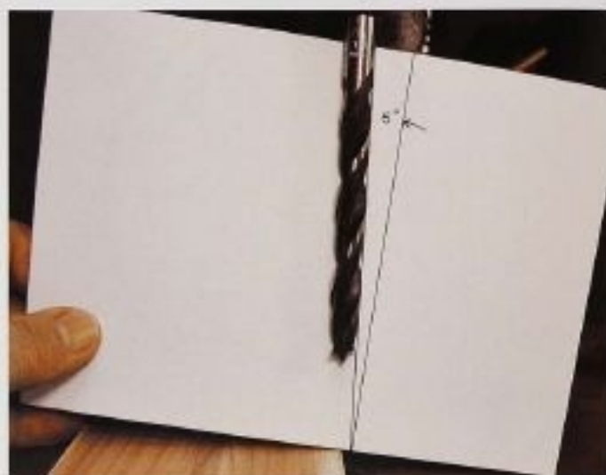
FIG. 3 By setting the angle template on the 1/4" spacer you can make adjustments with the spacer so the drill will make an accurate 5°-angled hole. Make sure the drill bit is aimed toward the center of the block.
