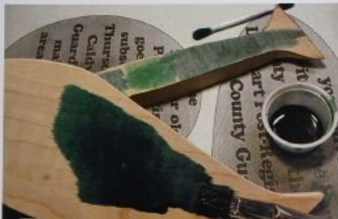
FIG. 6 Be generous when applying dye. If you try to paint it on, the result will be streaky and irregular. Try out the mixture on a piece of scrap figured maple to see how it will look before using it on the box lid. At first the color was too green; a couple more drops of blue made it just right.
