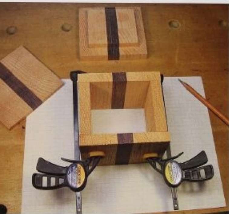
FIG. 4 During your dry-fit test, draw lines on the sheet of paper inside the pieces to make it easier to realign the sides when doing the actual gluing. Draw lines on the inside of the body sides to indicate where the corners overlap to help you to keep the pieces square during clamping. Note: Make your notations lightly with pencil.
