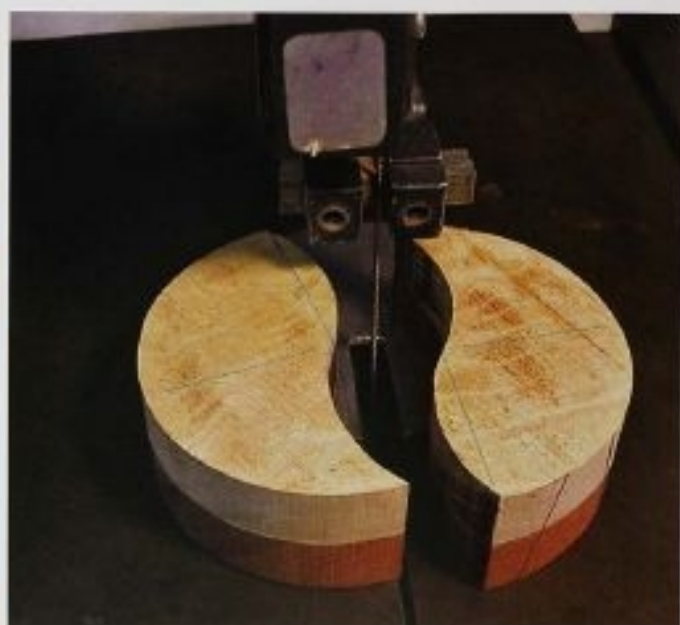
FIG. 4 Cut through both lids at the same time, and they are guaranteed to match.
