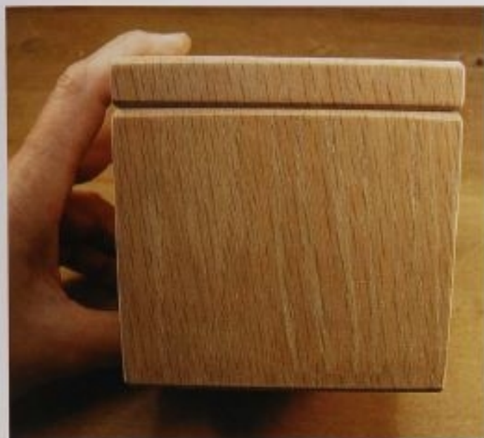
FIG. 7 With a wood as coarse-grained as red oak, the glue-line practically disappears with a good joint. This is a side with three joints, but they are almost invisible.
