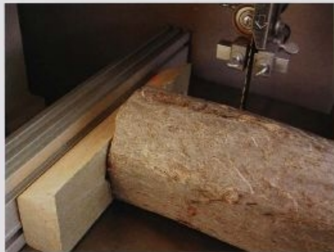
FIG. 15 The stabilizer can rest on the fence to allow you to get a straight cut, or you can use your miter gauge to keep the wood square to the blade. Make sure you do not cut into the nails. Band saw blades are not very useful after they try to cut steel.
