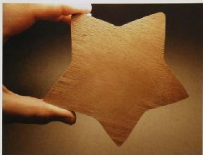
FIG. 36 With strong side-directional lighting, or straking light, you can see the slightest imperfections in your sanded surface. For this Star Box interior, I left the edges untouched so the bottom seam will be invisible.
