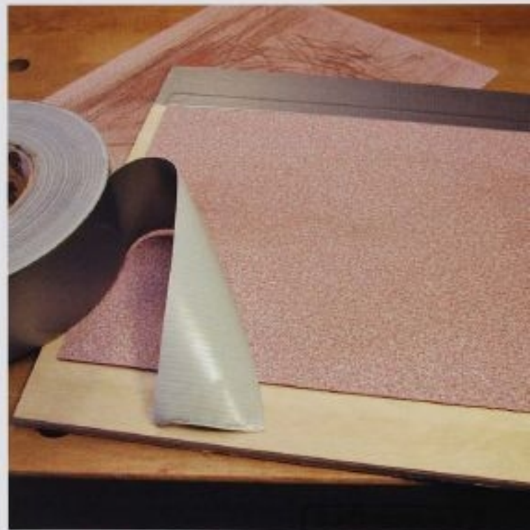
FIG. 36 Make a couple of these sanding boards for controlled sanding of flat surfaces. Here I've used 12x12" squares of \frac{3}{4} " plywood and some duct tape.
