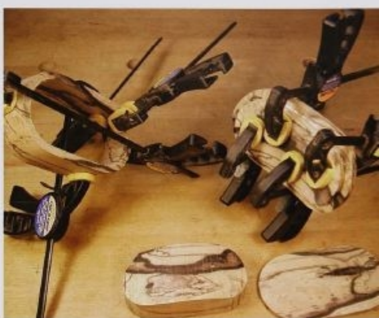
FIG. 6 The body is glued and clamped together, and the lid liner is glued to lid. While you're waiting for the glue to set up, you can make another box from the core.
