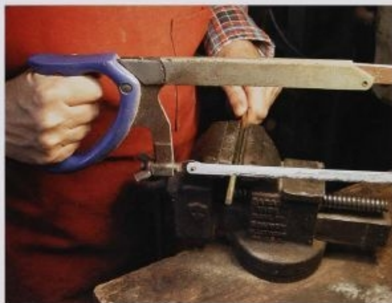
FIG. 6 A metal vise is useful to keep the brass rod steady for cutting with the hacksaw. Use slow, firm strokes and press down only on the push stroke for effective metal cutting.
