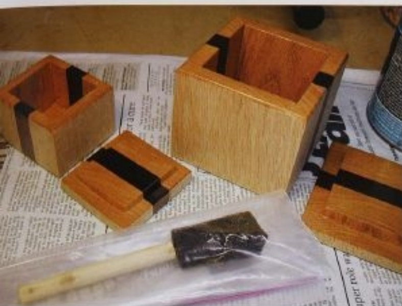
FIG. 13 When you have to put on many coats of surface finish, you can seal your brush or rag in a plastic bag so it doesn't dry out and you don't have to clean it every time.
