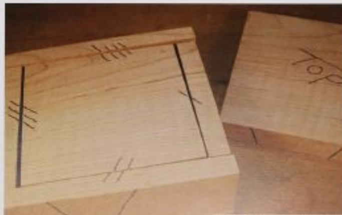
FIG. 2 This is how the body should look after the sides have been cut off. Notice how the registration marks help keep everything in order.
