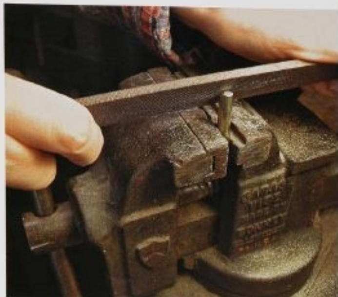
FIG. 7 Use a metal file to first flatten and then round the eye end of the brass rod. Use both hands for better control with the file. Work with slow, firm strokes, and apply pressure only on the push stroke.
