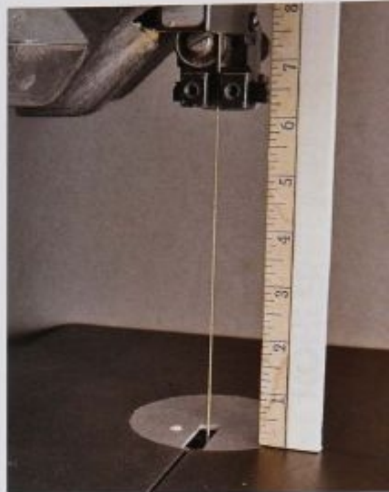
FIG. 7 The vertical cutting capability, the resaw capacity, of this 12" band saw is the same 6" as it is for a 14" machine.
