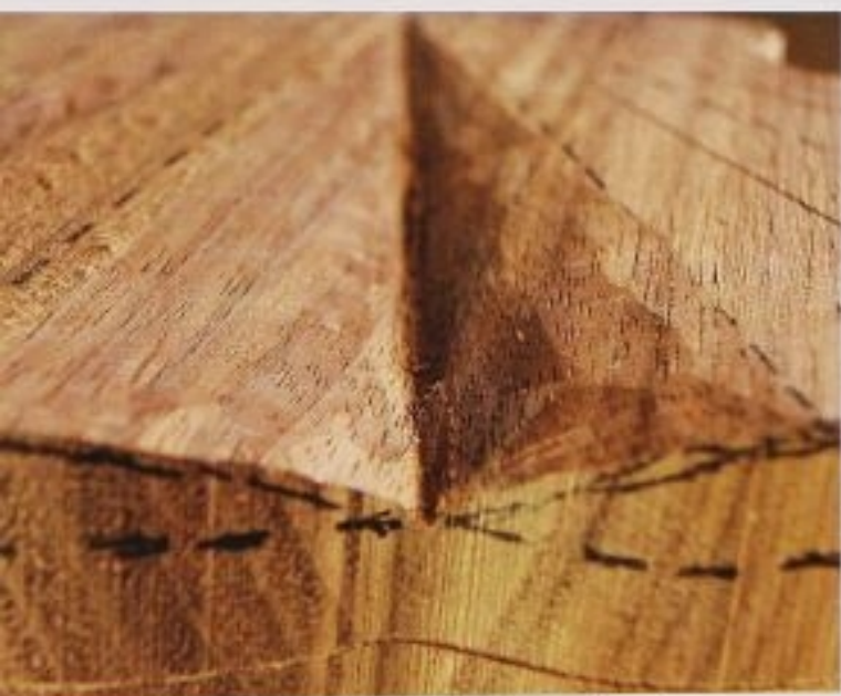
FIG. 9 Continue rounding the curves until you have a smooth, tapering arc at each division. You may want to draw an arc at the end of the division as an aid to keeping the curves consistent.
