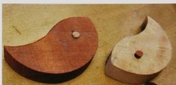
FIG. 7 Leave a little of the plugs sticking out from the lids. They will be sanded smooth when the lids are sanded.
