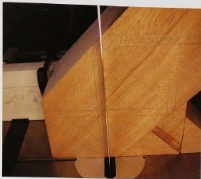
FIG. 2 Get around to the back of your band saw so you can see to line up the blade with your layout lines. Notice the small clamp to the left of the block. It is attached to the miter-gauge auxiliary fence and acts as the stop for that side of the inlay line.
