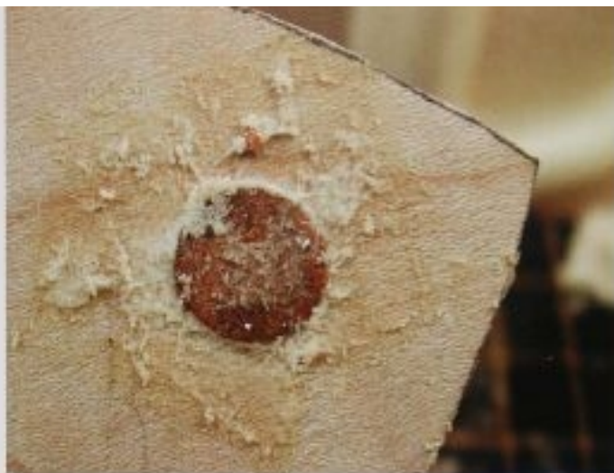
FIG. 5 The result of the dowel fix is messy, but power-sanding will fix the exterior quickly. The interior, where the dowel sticks out, will require some scraping before sanding by hand. All the glue must be removed or the dye will not be absorbed into the wood and the finish will be uneven.
