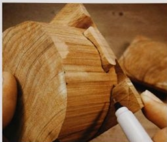
FIG. 14 After the body outline has been cut out, use it to mark the matching sides of the lid and base piece.
