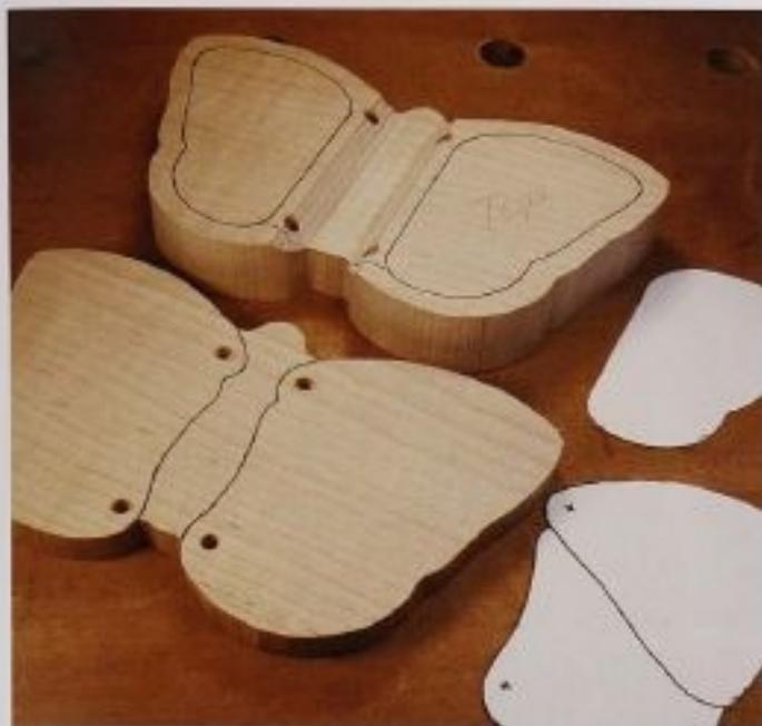
FIG. 5 Mark the topside of the body piece and the body side of the lid/wings. Be sure to leave at least \frac{1}{8} " of wood around each of the hinge holes, and then cut out the interior and wings.
