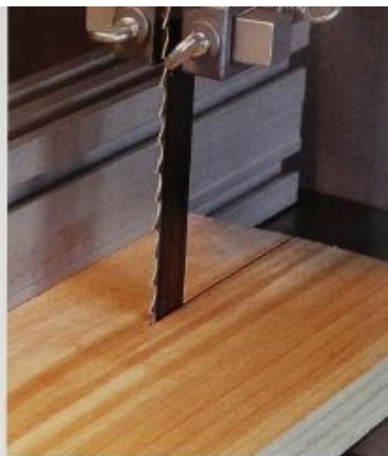
FIG. 10 This after-market fence is easy to adjust, and it helps keep the wood feeding straight into the blade for precise rip cuts (with the grain). The blade guard has been raised for demonstration only. Always keep the guard as close to the wood as possible.
