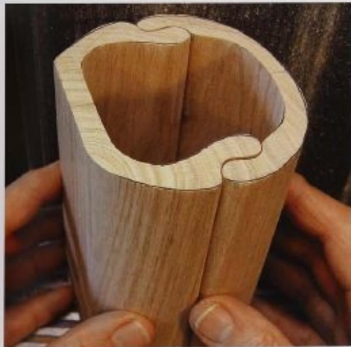
FIG. 4 It is safer and easier to sand the body and lid on the belt sander table while the two pieces are held together vertically. If you were to try to do this job with the piece held horizontally, the force of the belt could cause the wood to spin out of your hands.
