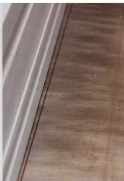
FIG. 26 Compare the edge of the fence to the drawn line to see the extent of drift with this blade on this piece of wood.
