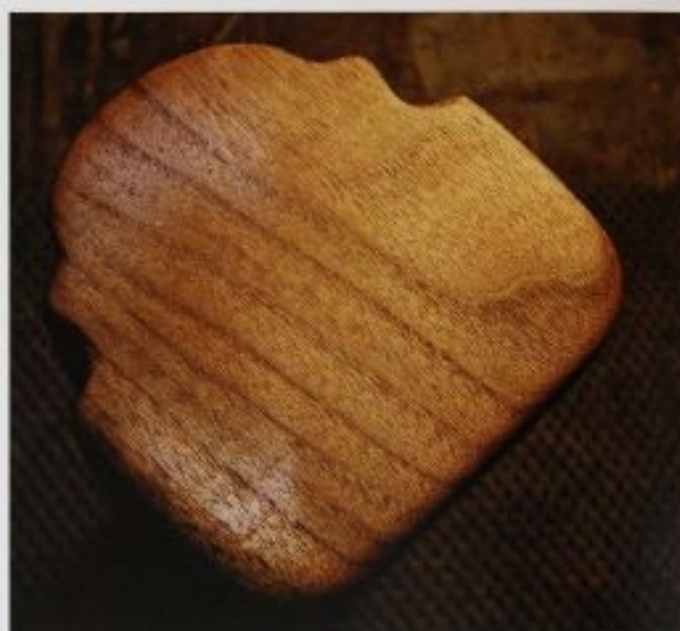
FIG. 13 After the sanding sealer has dried, and before putting on the final coat, you will need to rough up the gloss and smooth down the surface of the finish. The best tool for this job is a maroon nylon scrubby. The left half of this end has not been scrubbed; the right half has been.
