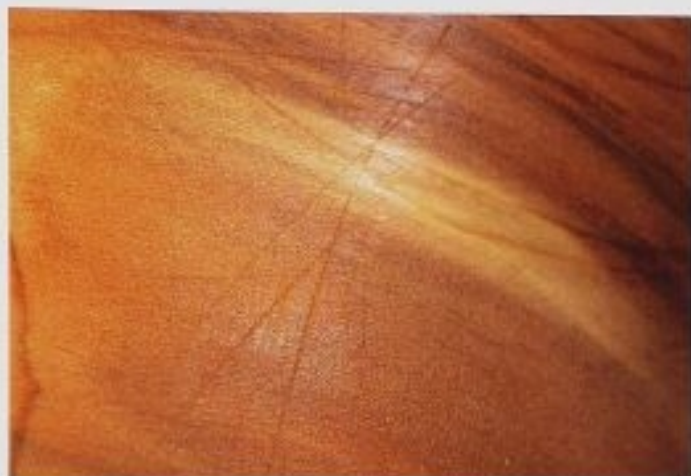
FIG. 7 Oh misery! After the first coat of lacquer, a mess of scratches became visible. I must have skipped a step in the sanding procedure. No help for it but to sand it down through the finish and back to the grit that created the scratches, and then work carefully back through the finer grits to 320-grit.
