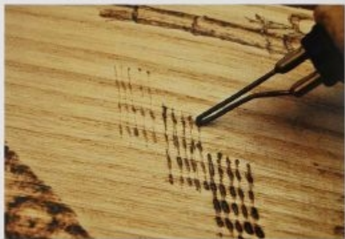
FIG. 8 Make a few practice burning strokes on the same type of wood as your boxes. The burn on the left is too light, the one on the right is too dark, and the middle one is just right to burn dark enough without creating smoke.
