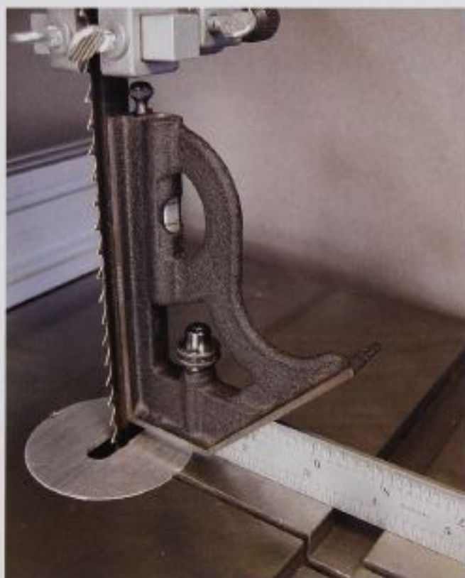
FIG. 28 Before cutting into your wood, check that the band saw table is adjusted square to the blade. Now you are ready to start making some sawdust.
