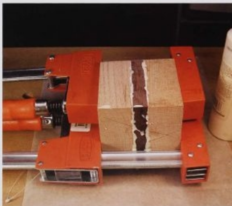
FIG. 3 Use sufficient glue and lots of pressure to assure a good lamination. Here I've used the big guns, screw-type clamps, for maximum power.
