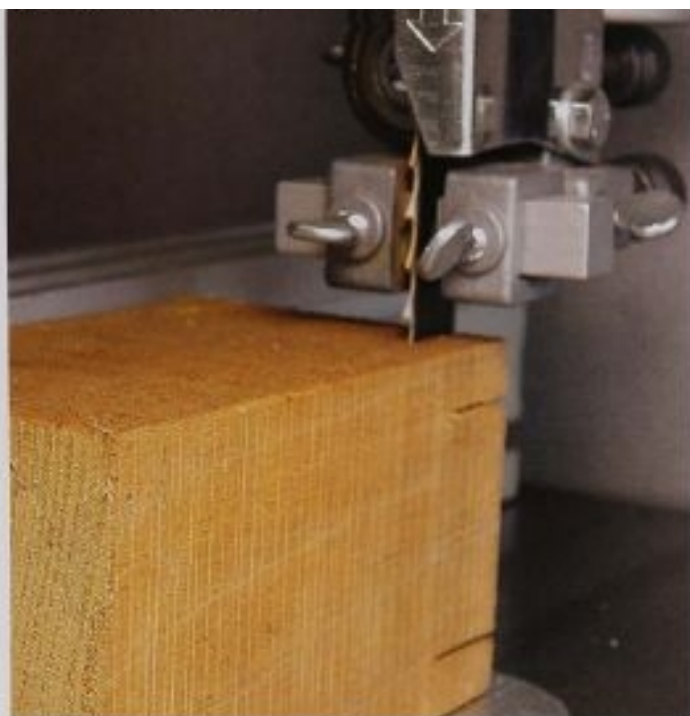
FIG. 8 Here the blade guard is positioned correctly, just above the wood. In some of the pictures in this book the blade guard has been raised to make it easier for you to see the setup; but the blade guard is always just above the wood when I am cutting with the band saw.
