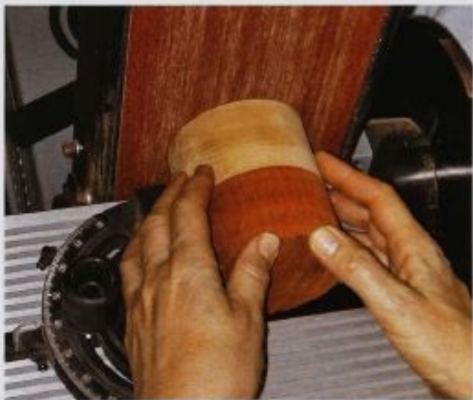
FIG. 2 Use the miter gauge and table when sanding the ends square. If you don't have this arrangement, use a square to check the ends; then mark irregularities with a pencil, and sand to the lines by eye.
