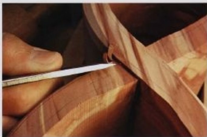
FIG. 6 To emphasize the twisting concept of the infinity or Möbius symbol, I carved a separation at the crossing. Use a simple gouge with stop cuts and slicing cuts to make about a \frac{1}{8} "-deep relief carving that tapers to the surface. This maneuver also effectively disguises the entrance cuts.
