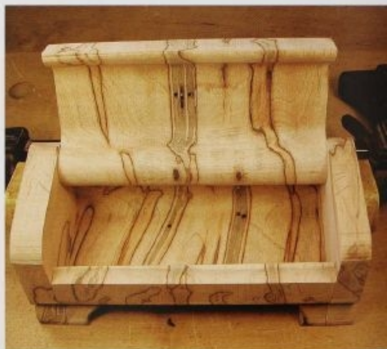
FIG. 7 Use a quick clamp for trial-fitting the pieces together. I usually have to assemble and disassemble the box a dozen times before I feel that the fit is as good as it can get.
