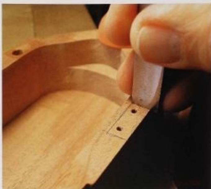
FIG. 8 Make clean stop cuts all around the hinge location for the mortises. Mark the depth to about \frac{1}{16} ", and chisel to the stop cuts.
