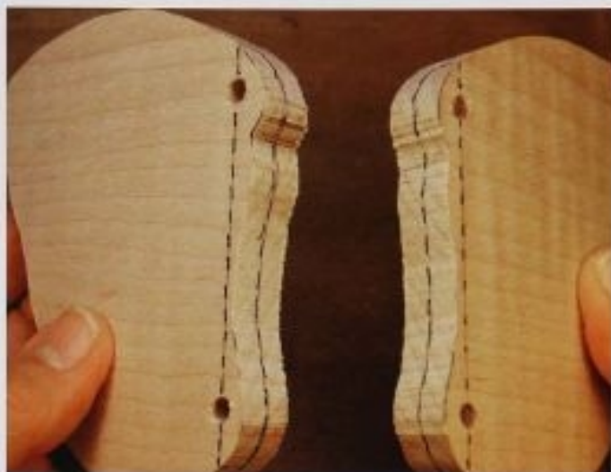
FIG. 6 Mark the underside of the wing pieces for sanding chamfers for the hinge clearance. Make sure the chamfer ends in the center of the holes.
