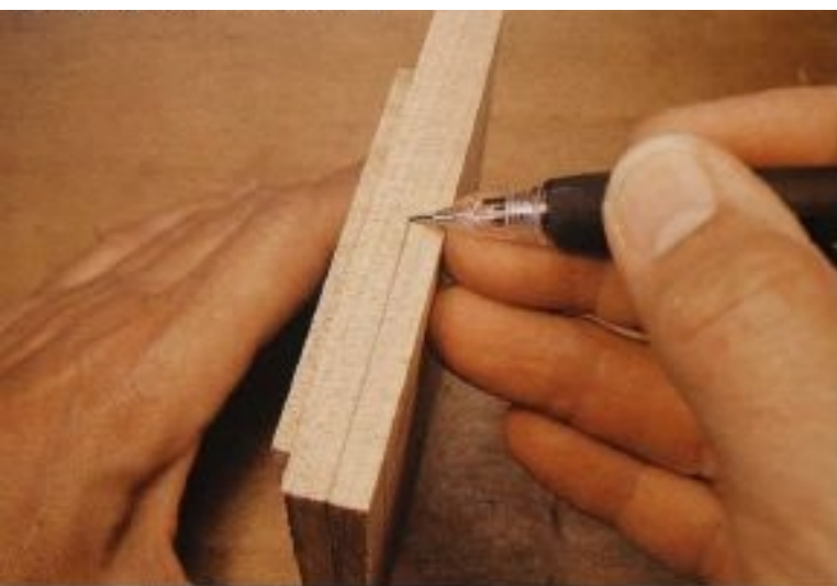
FIG. 8 It takes a little practice to use your fingers as a marking gauge. By spacing the pencil mark with your fingers against the piece of wood, you will save tedious measuring time. Use this technique especially when making measurements in from the edge of a complex, curvy shape.
