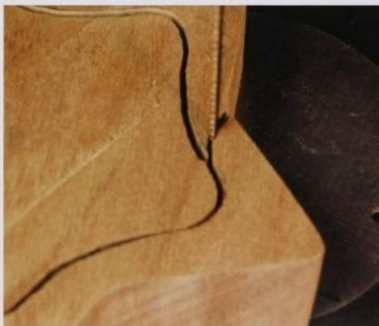
FIG. 12 After you have cut around the interior, turn off the band saw and back out through the entrance kerf. If you try to do this with the machine running, you'll likely cut into the box sides, making an invisible joint impossible.
