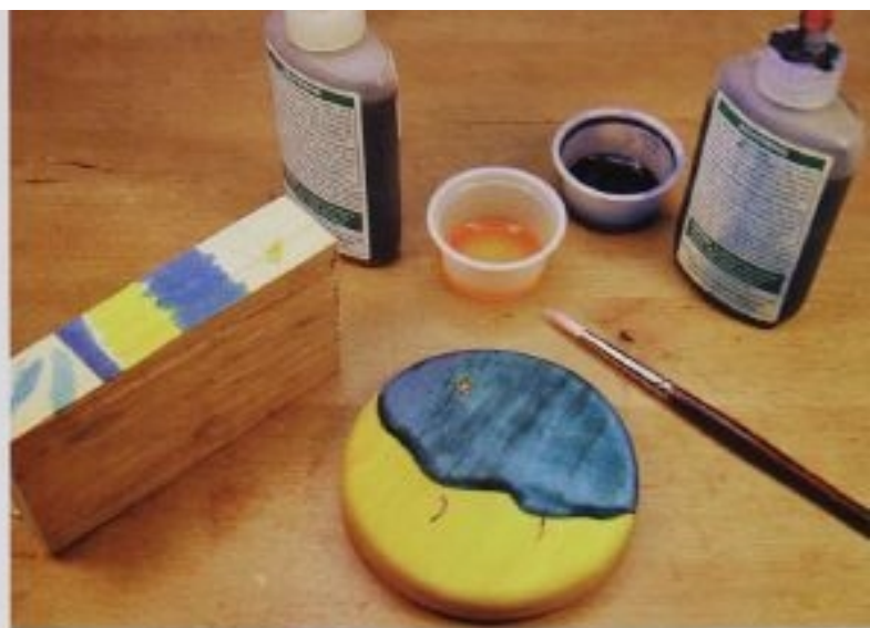
FIG. 8 Here is the setup for dying. On the left is a practice piece for testing dye concentrations. Use small containers of diluted dye, and test on the same type of wood as your project.
