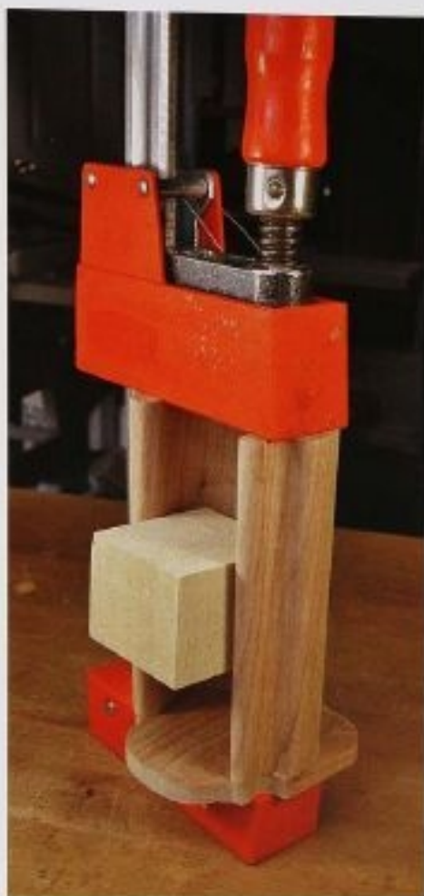
FIG. 5 The spacer between the sides of the body is a piece of tupelo made to force the sides out just \frac{1}{32} ". Use two spacers to keep the sides parallel. The large clamp guarantees a good glue joint, and the sides will stay a little apart, causing the lid to fit better.
