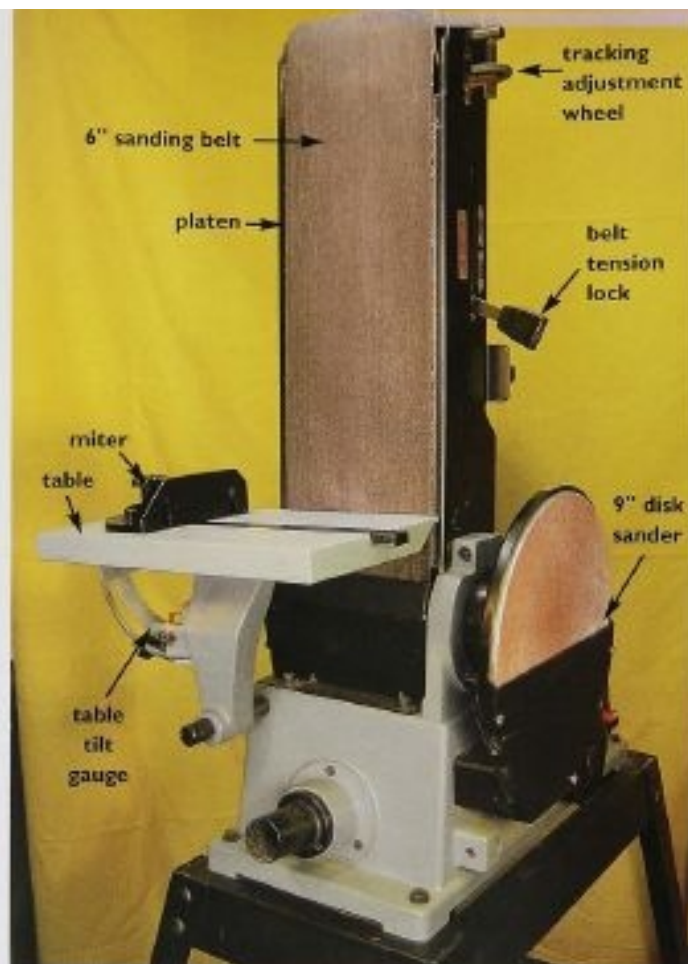
FIG. 30 Belt sander, right view. The tracking adjustment wheel on a belt sander controls the tendency of the belt to drift. The tensioning lever loosens and tightens the sanding belts. Make sure the belt is in position and tight before turning on the power.
