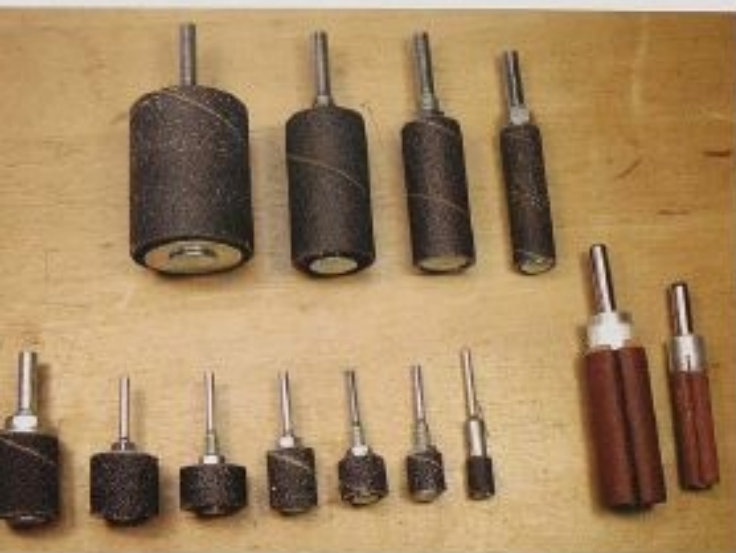
FIG. 32 Here is an assortment of sanding drums: The top row shows 4 diameters for 2" long drum sanders with 1/4" shafts. They can be used in drills, drill presses, and larger rotary power tools. The bottom row has 6 different diameters for shorter drum sanders that have 1/8" shafts, for use with smaller rotary power tools, like Dremel tools. The two larger sanders on the right bottom row are made of soft rubber and take small sheets of sandpaper instead of preformed drums. They work very well for sanding contours.
