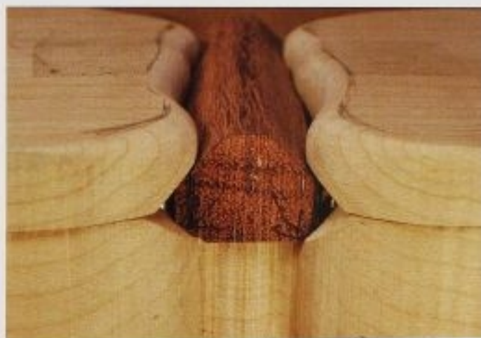
FIG. 10 The body must fit snugly between and under the wings. You don't want a hammer-force fit, but remember that after you shape and sand the body, the fit will be looser so keep it as tight as possible at this point.
