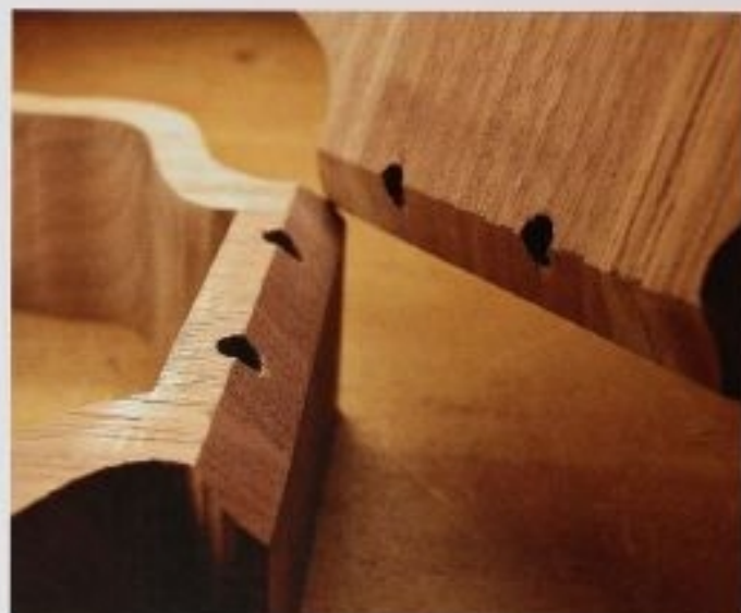
FIG. 14 As you chamfer the edges with the belt sander, check your progress frequently. Keep the pressure even, steady and light until you reach the center of the holes. Done correctly, the chamfers will be straight, flat, and will neatly bisect the holes.
