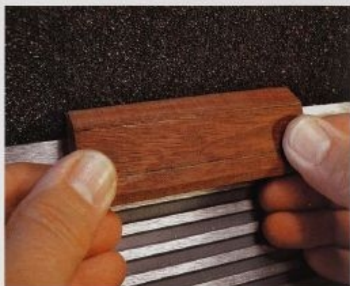
FIG. 9 Watch your fingers when sanding small and difficult-to-hold pieces of wood, such as the butterfly body shown here. It would be safer, easier, and result in a better job if you attached such small pieces to a block of scrap to give yourself more holding power.
