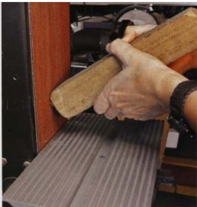
FIG. 34 Keeping your belts clean of sawdust will greatly extend their effectiveness and their lifespan. Sanding dust does not make a very good sander, and you may stress your sander motor unnecessarily trying to sand with a sawdust-filled belt. Use a rubber sanding cleaning stick regularly.
