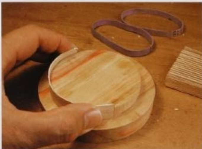
FIG. 51 It may take more than one strip to go around the lid liner. Glue one strip at a time and your job will be a lot easier. Trying to keep more than one piece of slippery wood in place while you apply the rubber bands is nearly impossible.
