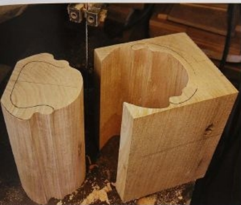
FIG. 2 The results of the first cut show there are still two well-supported pieces ready for their second cuts. Don't worry if you stray a little off the line while cutting. It is more important that the contour is smooth and even.
