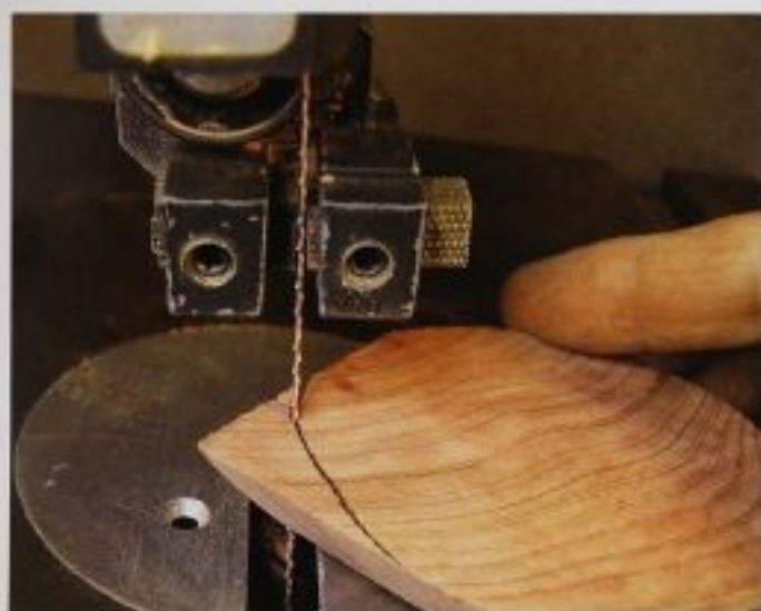
FIG. 15 When cutting the base, place it with the inside up and locate it downhill from the blade to insure that the angles will match those on the body. Repeat with the lid piece.
