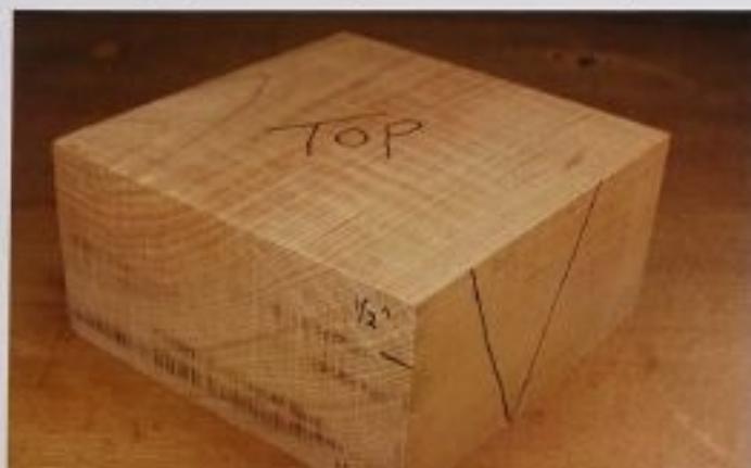
FIG. 1 Registration marks will help when you reassemble the pieces for gluing after cutting the block into the box parts.
