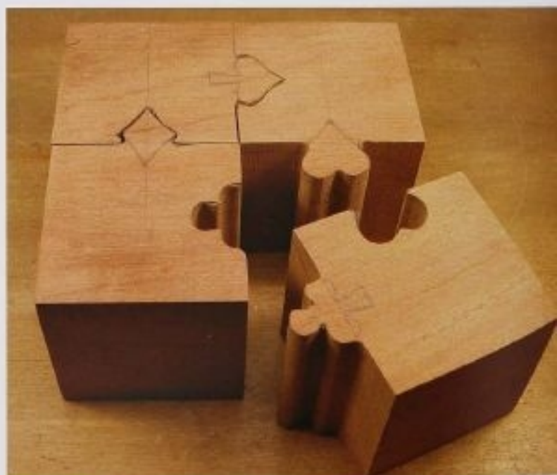
FIG. 3 At this point it looks like an overgrown jigsaw puzzle for the fumble-fingered. Each piece has a key and a void for the key in the adjoining block.
