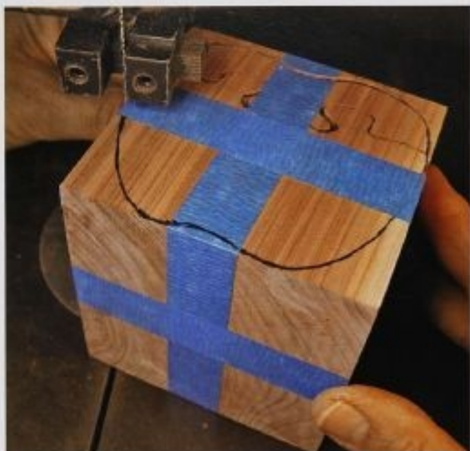
FIG. 7 After cutting out the keyway, reassemble the block and tape it together securely before cutting out the outline on the keyway side.
