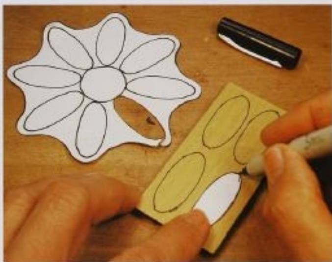
FIG. 7 Cut the pattern for the petals out of the same pattern that you used to mark the box perimeter. If you sandwich two layers of wood together, you only need to cut out four petal shapes. Note that this version of the pattern used a large center piece, but the final pattern has a smaller center.
