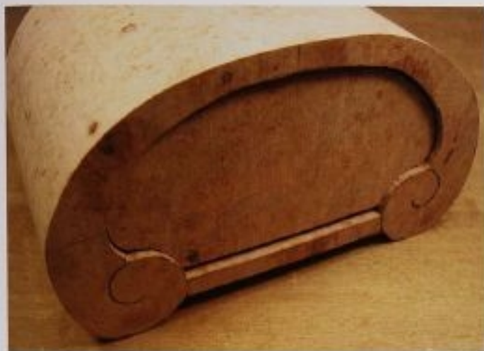
FIG. 4 The drawer will be shorter than the box interior because of the two kerfs created when cutting off the front and back. Put the box front, with the drawer in place, against a 60-grit sanding belt, and bring the box body to the same level as the drawer.
