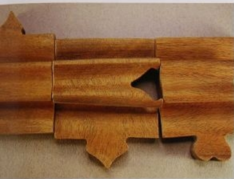
FIG. 4 The lid piece in the center is much wider at one end than the other. This is what happens if the block is not kept flat on the band saw table at all times. The result is a one-way keyway.
