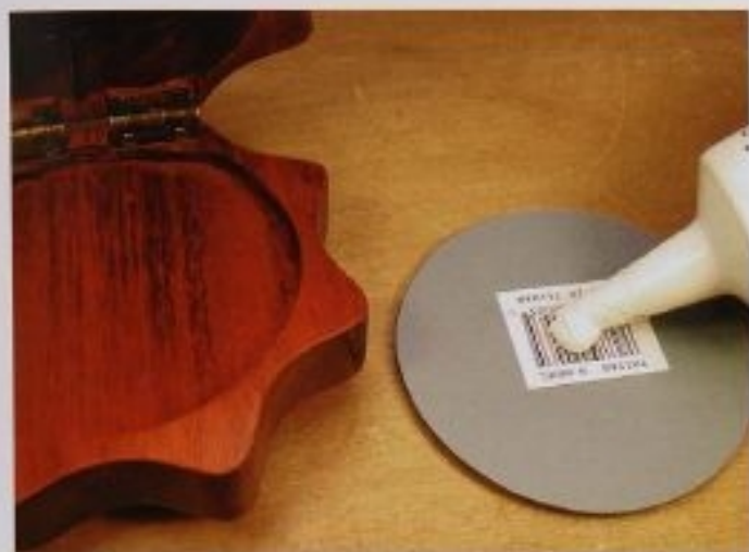
FIG. 11 The mirror had a label on the back, so I placed the adhesive caulk there. One good drop in the middle should hold it just fine.
