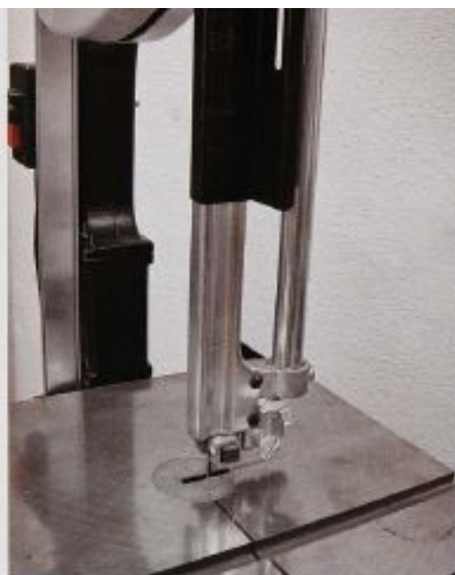
FIG. 9 With a riser block installed on this 14" band saw and so much blade potentially exposed, I am careful to keep the blade guard extension in the fully lowered position for safety.
