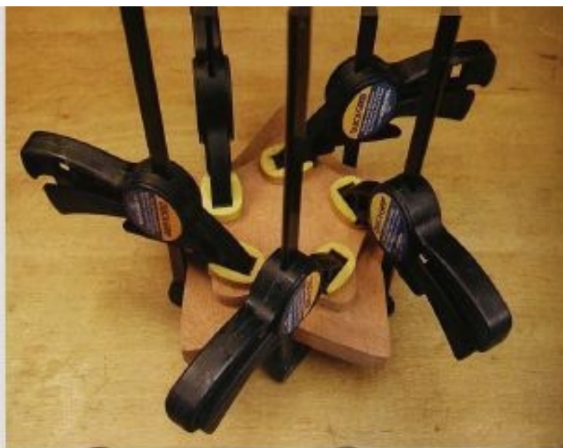
FIG. 14 Join the liner and lid firmly so there is no unsightly gap between them. Use as many clamps as necessary. Check the position of the lid liner before finally tightening the clamps.
