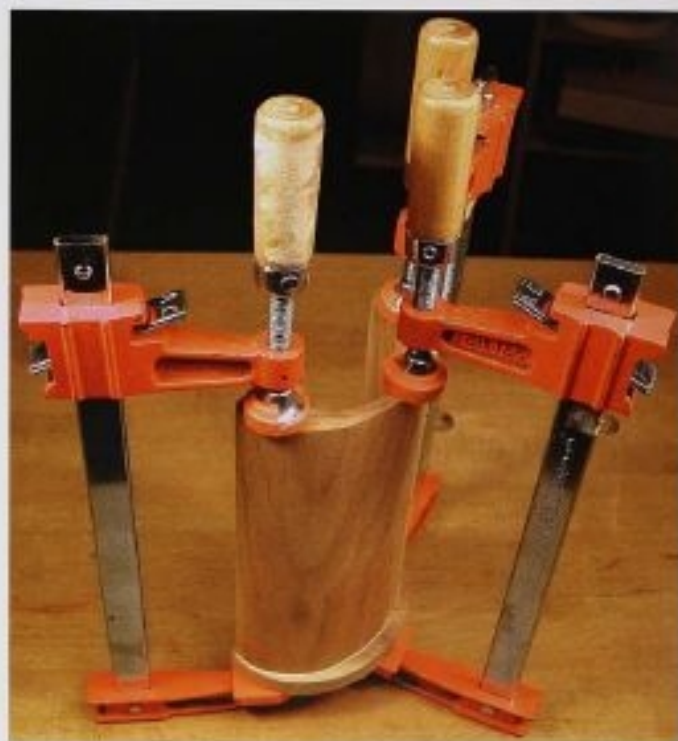
FIG. 6 Glue one end at a time when putting the lid together with its ends. Make sure the ends cover the edges of the lid. They always can be sanded back to ensure a good fit.
