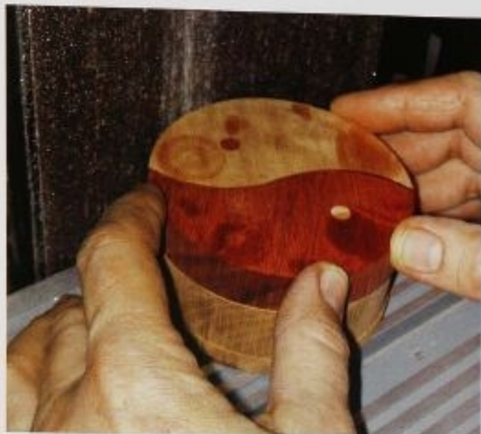
FIG. 9 It will take a lot of careful sanding to make the exterior of the box smooth and even. Take off only as much as is necessary so the sides of the box don't get too thin.
