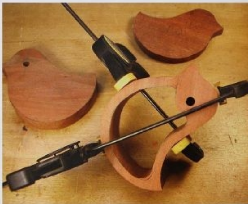
FIG. 3 Cross-clamping will hold the edges together while the glue dries, and it will keep the edges from sliding into the wrong position.
