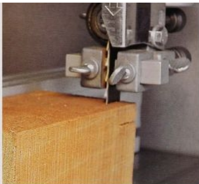
FIG. 24 This is a good setting for the blade guard, just 1/4" above the wood.
