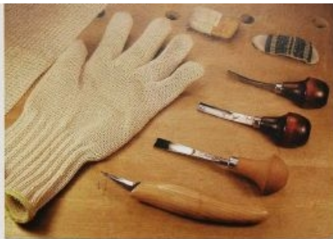
FIG. 1 Basic carving tools sufficient for many of the carving projects in this book. From the top left: nonslip rubber mat; Kevlar safety glove for hand-holding wood; finger and thumb protection for the hand-holding knife, and gouges. From the bottom: carving knife; #3 sweep, \frac{1}{2} " wide; #7 sweep, \frac{3}{8} " wide; #11 veiner, \frac{1}{8} " wide. Add a couple of chisels and you are set.
