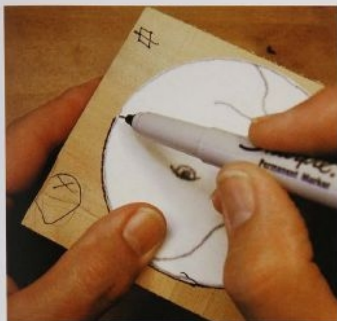
FIG. 1 By cutting out a copy of the plan, it is easy to shift the pattern around to avoid blemishes in the wood.
