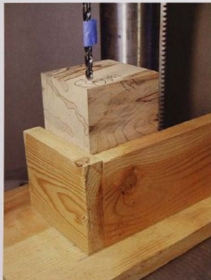
FIG. 3 A simple corner jig like this can help you to keep your tall block upright.
