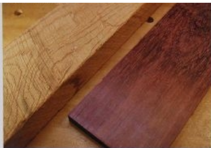
FIG. 1 Choose lumber with a straight grain and good contrast between the different pieces. Wood seldom comes from the mill in good enough shape to laminate, so you'll have to plane or sand it flat and smooth.
