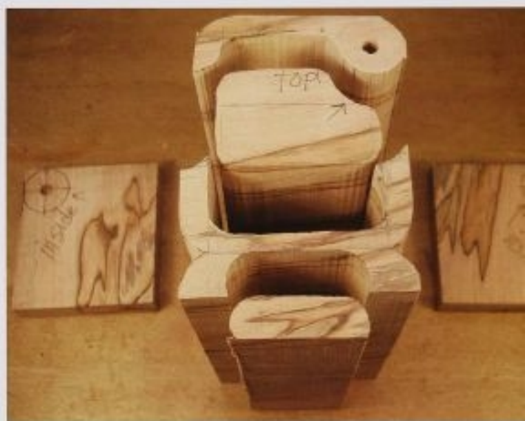
FIG. 4 These are the pieces cut from the block after the interior cuts have been made. It is very important that the band saw blade be as vertical as possible, so the hinge shape is equal on both ends.
