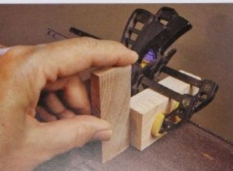
FIG. 5 Here the jig is being used to keep one of the short sides square during sanding. Be careful of your fingertips when sanding these small parts.
