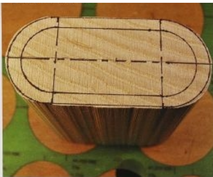
FIG. 2 To make the next box from the previous box's core, make a new plan right on the wood. That way you will be able to keep the piece symmetrical as you sand the sides to form.
