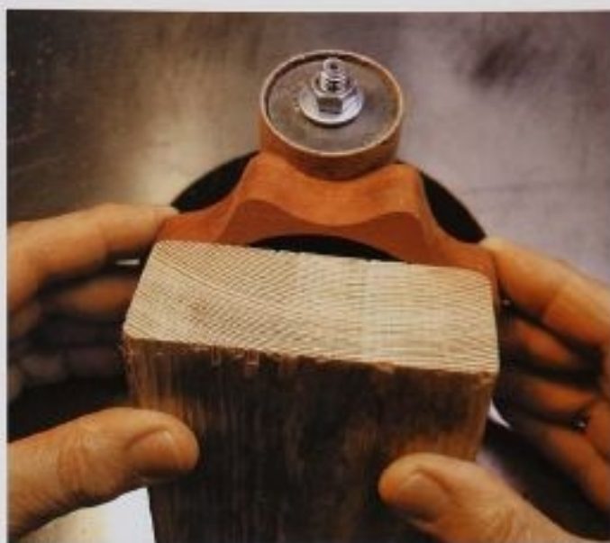
FIG. 6 In this top view of sanding the scallops on the base of the box, you can see that I'm holding the block and box together with both hands. Alternatively, the block could be clamped to the box section.
