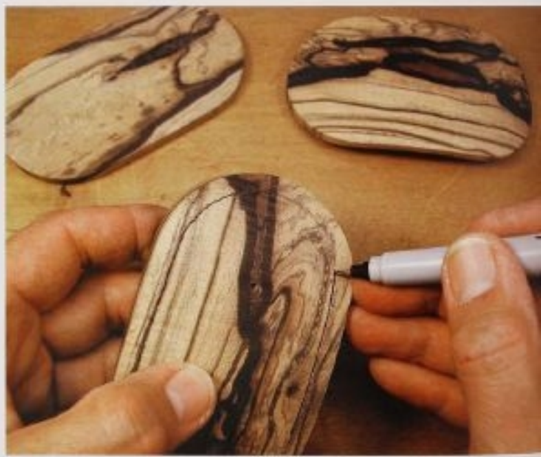
FIG. 4 Use your fingers to space your cut-line mark in from the sanded outer edge of the body, or use a depth gauge or marking gauge.
