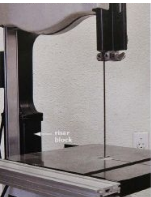
FIG. 8 This 14" machine has a riser block added to its vertical support arm. The 6" block of cast iron raises the top of the machine, enabling 12" resawing.
