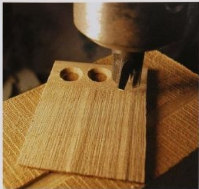
FIG. 6 Be sure to use a backing of scrap wood when using a plug cutter to cut the thin pieces of wood to attach to the magnets.
