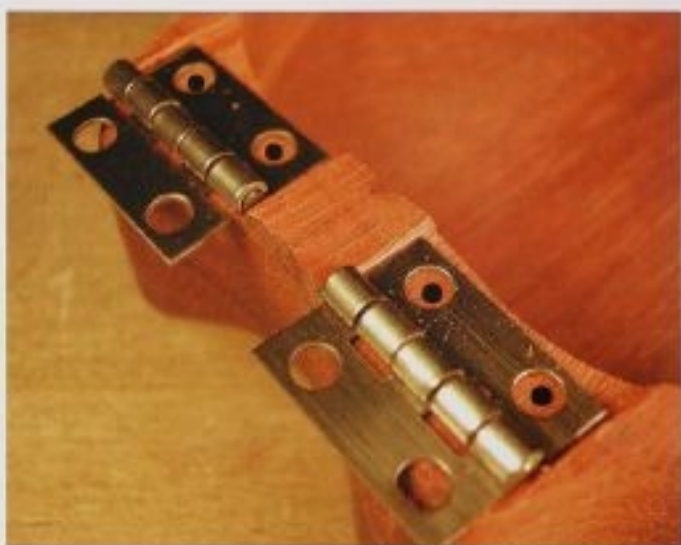
FIG. 4 If you have made your mortises correctly, the hinges should fit snugly into the recesses. Remember, you always can make a mortise larger, but it's difficult to make it smaller.
