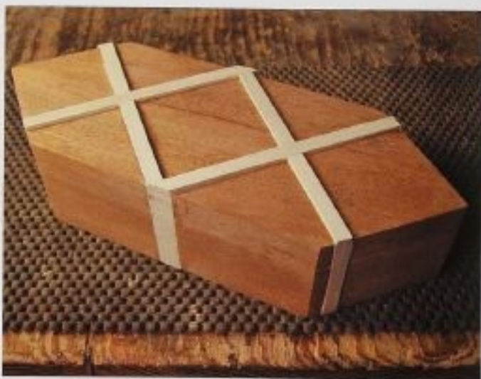
FIG. 4 One option for this box is to leave the inlays above the surface of the box, either just on the lid or all over. It gives a nice pattern and texture to the overall box design. Notice that I cut my box apart before making the inlays—bad idea. Save time and effort by making the inlays first.
