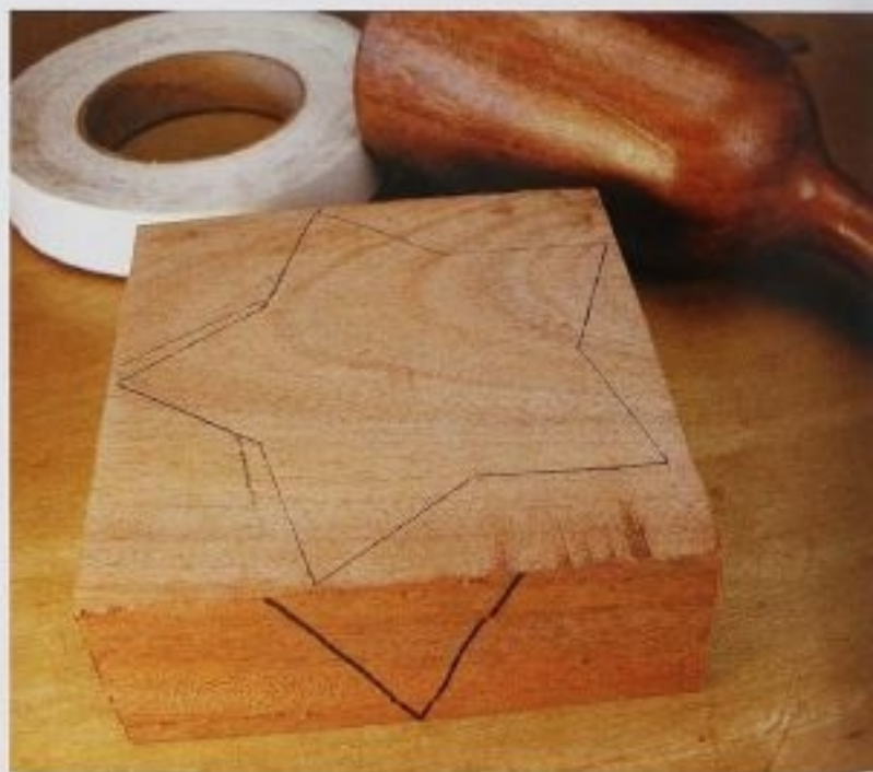
FIG. 9 The block has been reassembled, using the registration marks, with cloth-backed, double-sided tape.
