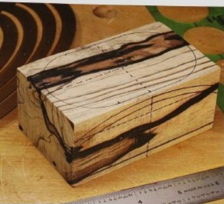
FIG. 1 Center lines drawn directly on the wood are a good way to keep your plan straight. Templates, like the circle and oval templates here, are handy when adapting the given pattern to different sizes of wood blanks.
