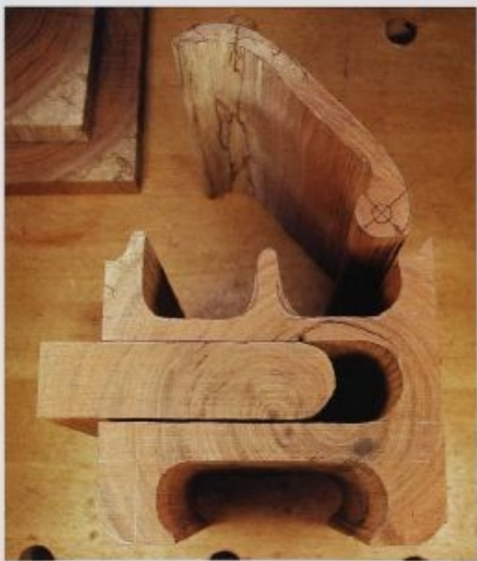
FIG. 2 Be careful when cutting out the body interior. Any misalignments of the block and the band saw blade will result in a badly fitting drawer and require lots of sanding.
