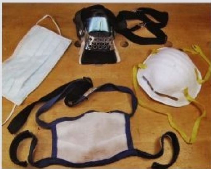
FIG. 5 Dust masks. Clockwise from left: A disposable surgical mask that attaches over the ears; a nuisance dust mask with replaceable filters; an inexpensive, disposable, but uncomfortable paper filter mask; and my personal favorite, the cloth filter that I can wear all day in comfort.
