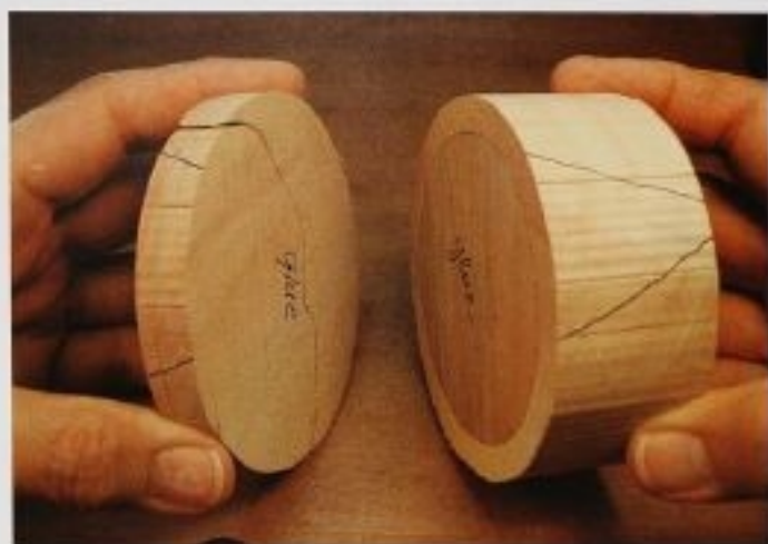
FIG. 4 Registration marks and notes on the mating surfaces will help you to keep the pieces in the right order. With this technique the lid and body will fit together well.
