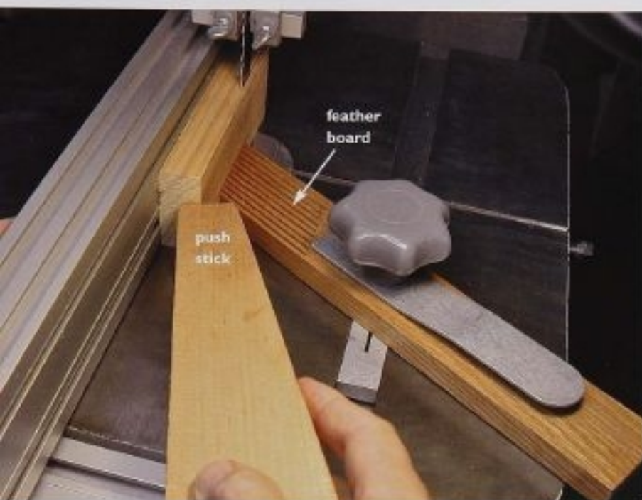
FIG. 16 Use a push stick and feather board to hold your wood in place, which keeps your hands well away from the blade.
