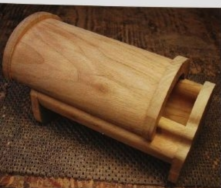
FIG. 12 Now that there is a good fit, round over the edges as needed, and sand the whole box to a smooth, flawless finish. Be sure to sand all traces of glue off the wood, or your finish will be splotchy.
