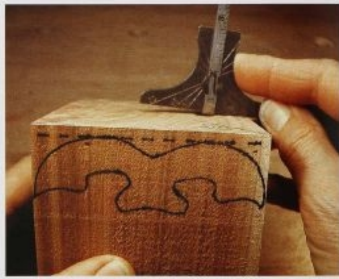
FIG. 5 Double-check the wormhole (key) depth and angle with a depth gauge.
