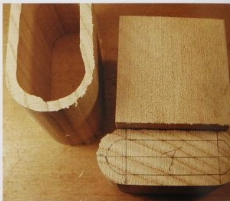
FIG. 4 When cutting out the core from the smaller blocks, you must use a stabilizing block. The irregular edge on the box at left was the result of tilting the block during the interior cut without a stabilizing block. On the right, the smallest box is ready to have its core cut out; the stabilizing block is attached.
