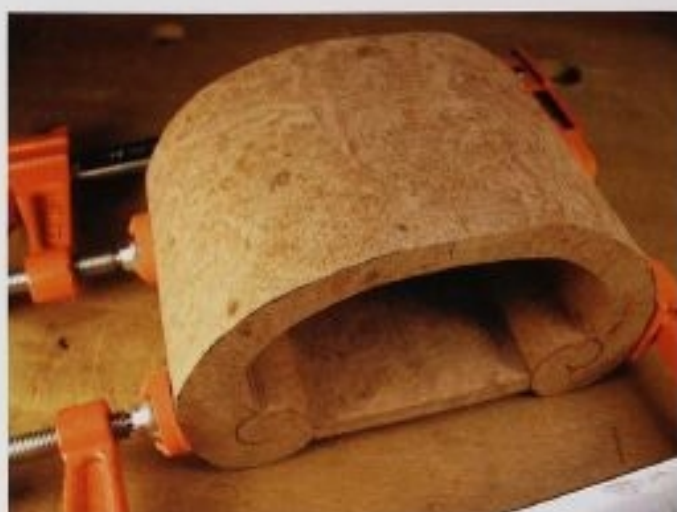
FIG. 2 You will need to bring out the heavy-duty clamps for gluing the base between the legs of the box. By forcing the two legs against the base, the box body will become smaller, which will result in a better drawer fit.
