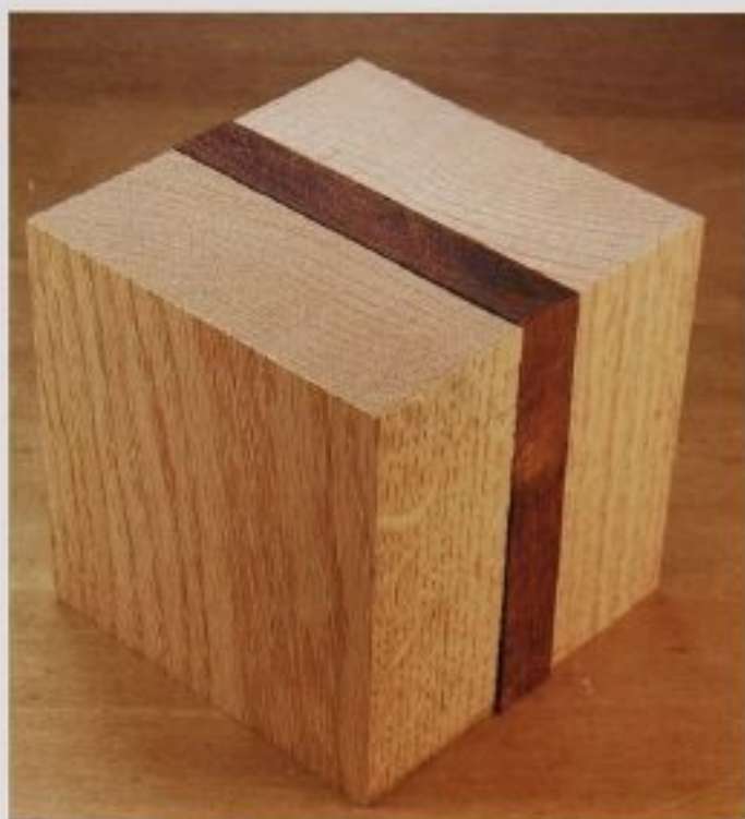
FIG. 2 After they are milled with the planer or sander, the pieces are ready for lamination. They need to fit together without gaps to make a workable block for your boxes.
