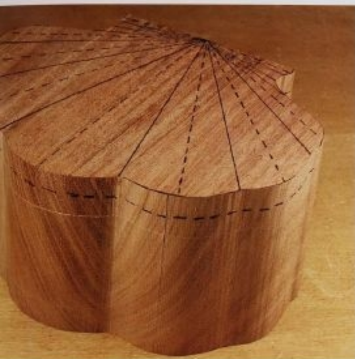
FIG. 4 The box has been marked for carving, with the solid lines marking the lowest areas, where you will make the stop cuts. The broken lines are the centerlines of the scallops and should remain until all the carving is finished. Do not use ink markers, as I did here for the model, because the ink will be absorbed into the pores of the wood and will be difficult to sand away.
