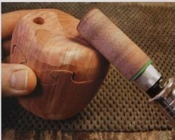
FIG. 19 This is where you get to sand all the imperfections away until what is left is a perfect apple form. Here I'm using a flexible-shaft sanding attachment.
