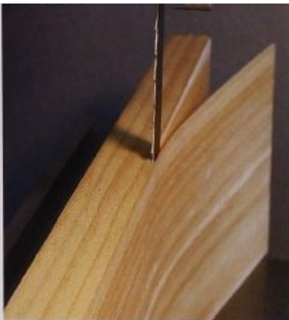
FIG. 11 Resawing (cutting through the thickness of a board to make a board thinner) is made much easier with a good fence.
