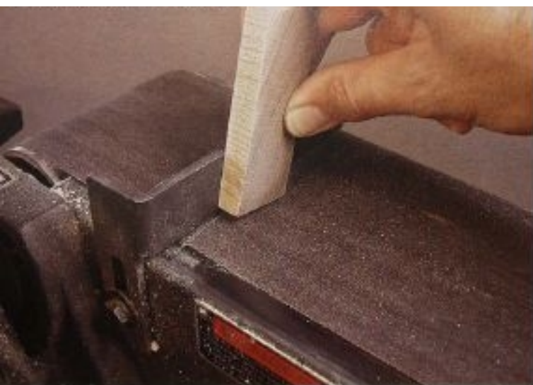
FIG. 3 Sanding freehand will not give you the square ends you need for the short sides of the body because you can easily create an angled gap between the wood and the belt (exaggerated here for the example).
