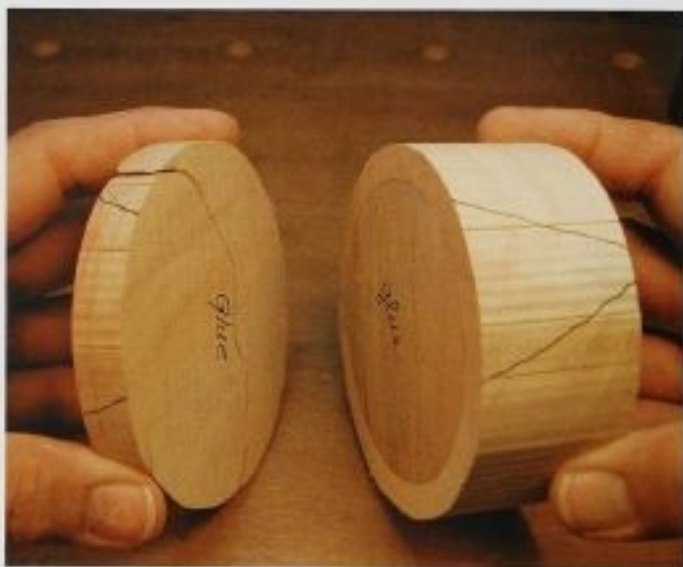
FIG. 47 Making a different lid liner is one way to get a tight-fitting lid when working with round, flat lids. Don't forget to use registration marks so you know how everything fits back together during glue-up.
