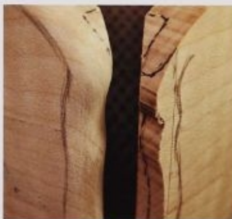
FIG. 7 The wing center on the right has been marked for rounding with the sander, and the wing on the left has been sanded round.
