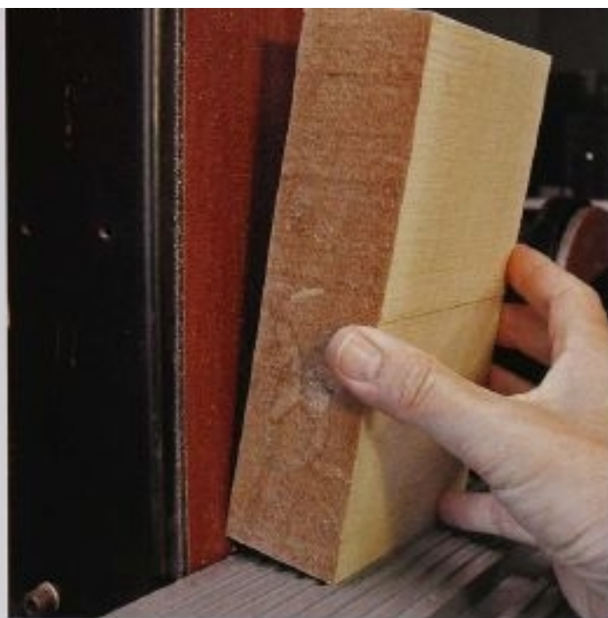
FIG. 29 To avoid accidents at the belt sander, it is important to have the piece of wood supported by the fence or table. Touch the end closest to the support first, and then immediately tip it flat onto the belt.
