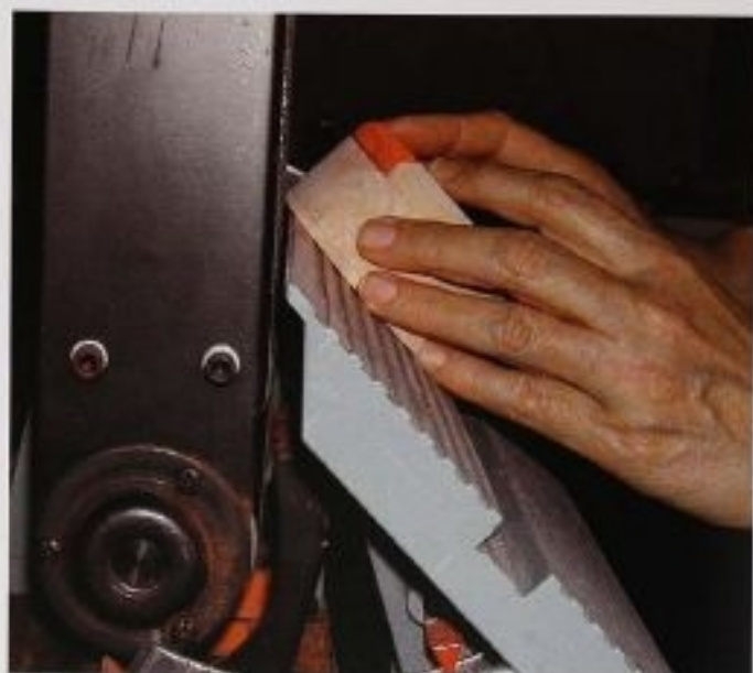
FIG. 10 If you have a tilting belt-sander table, it will be easy to make an even chamfer around the top and bottom edges of your box.
