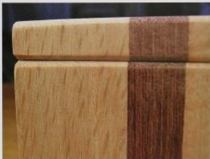
FIG. 8 The alignment of the laminations between the lid and body is less than perfect, as you can see in this straight-on view.
