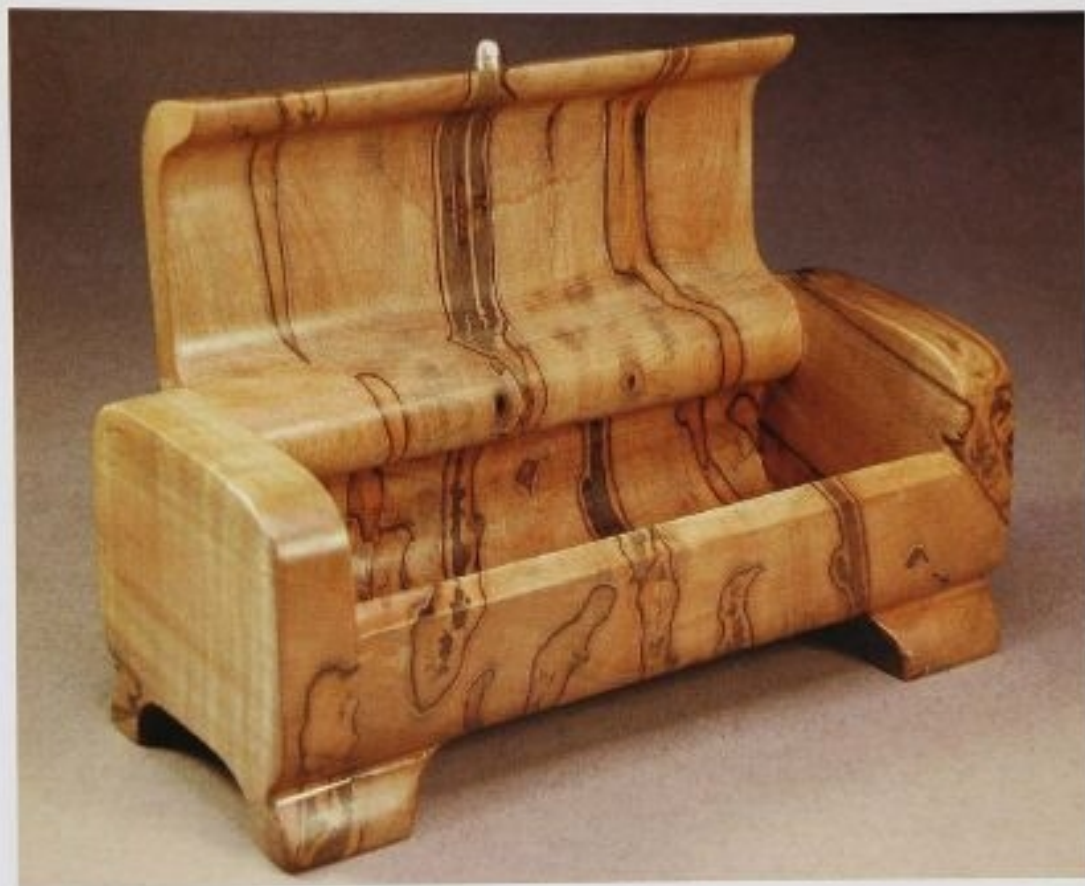
FIG. 11 Where are the hinges? Finished with a tung oil and urethane topcoat, the Ambrosia Box opens without a hint of the pivoting hinges.
