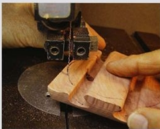
FIG. 16 Notice the location of my fingers while cutting the keyway lid outline. Keep away from the danger zone as you cut the lid piece. Your cut will move slower where the wood is thick, but speed up where it is thinner.
