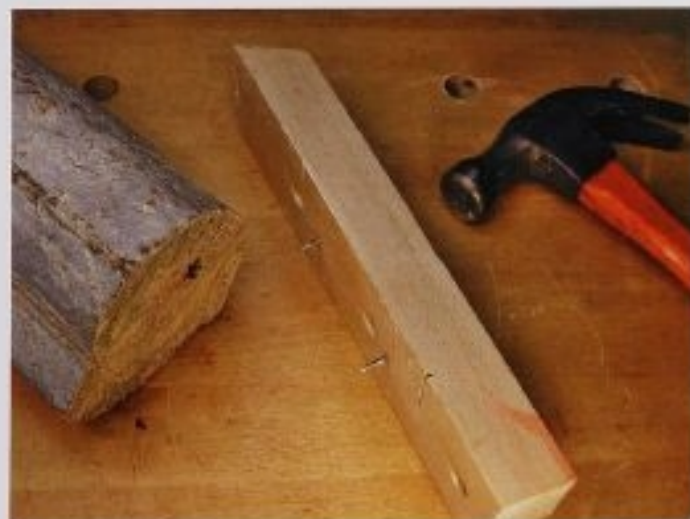
FIG. 14 Working with something as irregular as a log requires a stabilizing piece to be nailed to the log.
