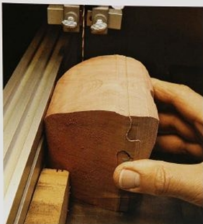
FIG. 9 Keep the cut-off pieces taped to one side of the box so the wood remains square and stable while you cut off the bottom.
