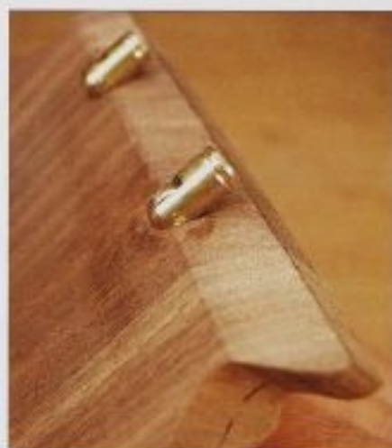
FIG. 16 The best technique for installing the hinges is to epoxy them into the lid first. That way you can easily check that they are oriented perpendicular to the box and that their depth is set correctly.
