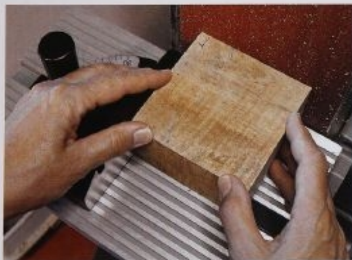
FIG. 31 Sanding the edge of a block squarely is easier when there is a nice big table on which you can rest the block.
