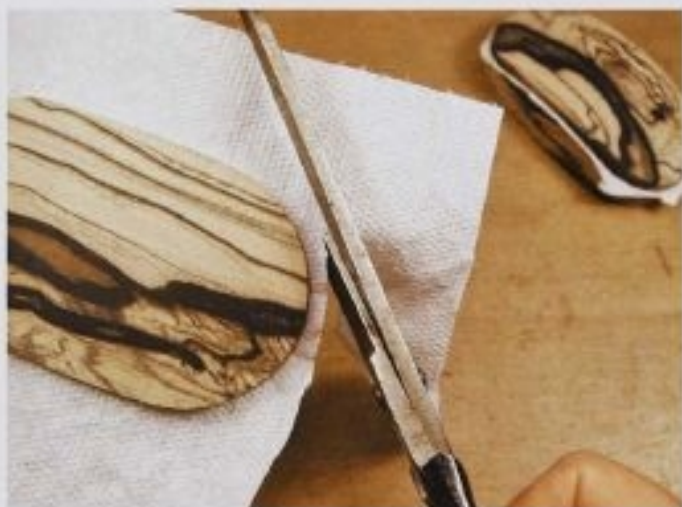
FIG. 7 Here's a trick to keep loose-fitting lids on firmly while sanding the contour: use a piece or two of paper toweling sandwiched between them to tighten up the fit.
