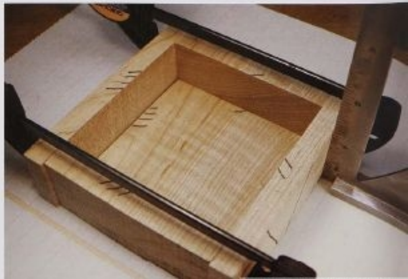
FIG. 6 Always do a dry run with clamps before gluing to check your fit and to make sure that the choice of clamps is correct for the job. Here the assembly has been moved to a piece of lined paper, the lines of which help to keep the assembly square. The paper also keeps glue drips off the workbench.
