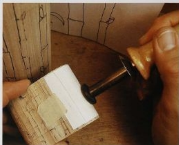
FIG. 7 Using a transfer tool can save time, but the image is difficult to erase if you make a mistake because the pattern ink is wax-based.
