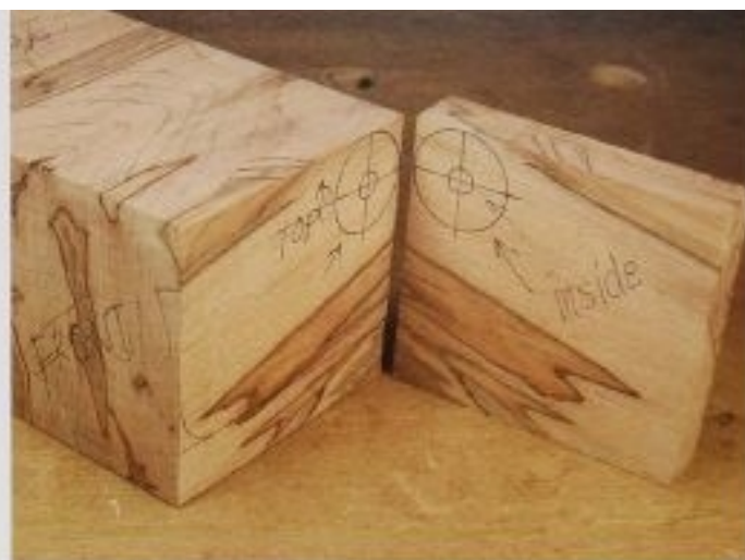
FIG. 2 Carefully mark the hinge hole position on both ends of the top back corner of the block, and then transfer those measurements to the matching end pieces.
