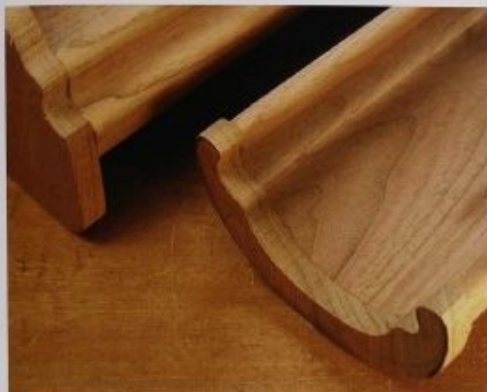
FIG. 8 You can see in this closeup of the box corner that there are a lot of mismatched ends that need to be fixed before the lid will slide on the body.
