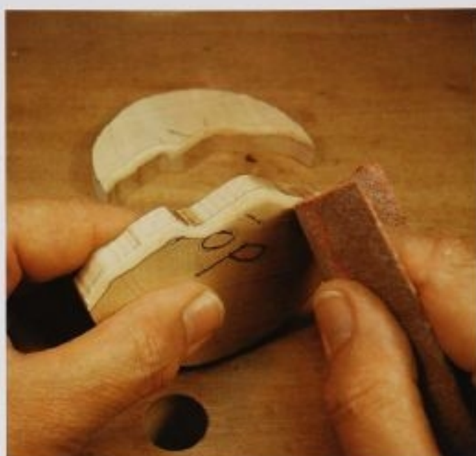
FIG. 2 When you need to remove just a little wood, as in the slight rounding where the two lid pieces meet, you don't want to use power. Power tools are great time- and energy-savers, but you'll have better control under your own power for delicate jobs like this.
