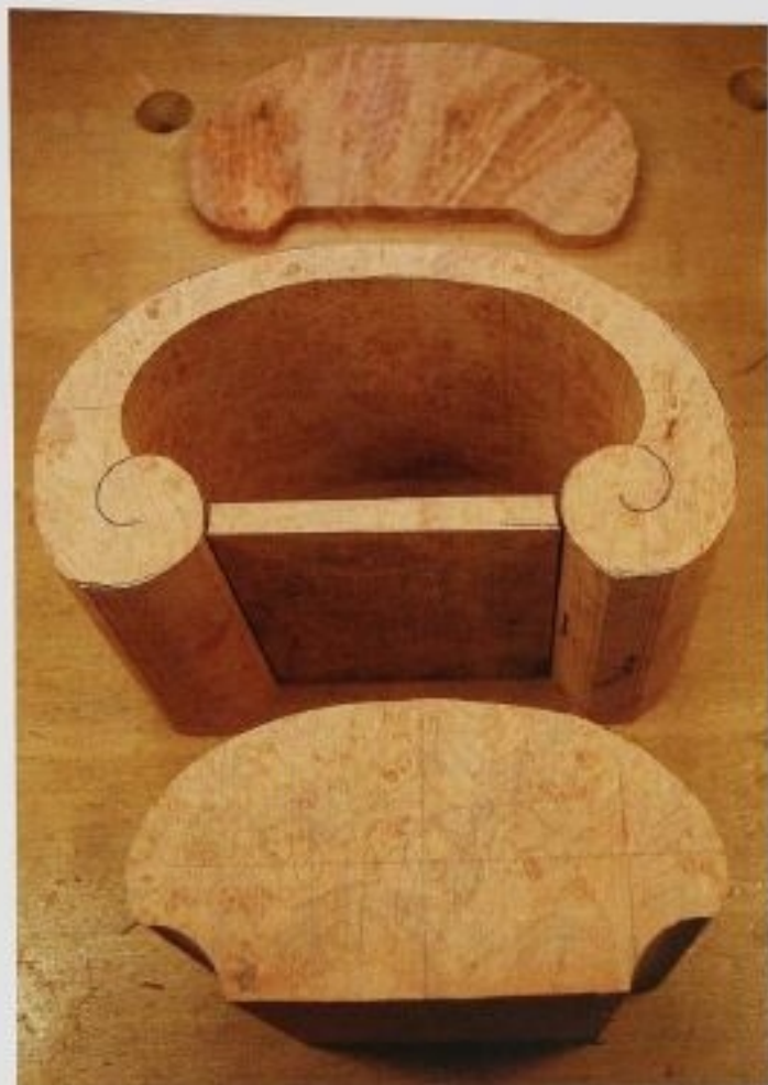
FIG. 1 The back of the box is at the top, the body is in the middle, and the drawer/core is at the bottom. The base of the box has not yet been glued into place.
