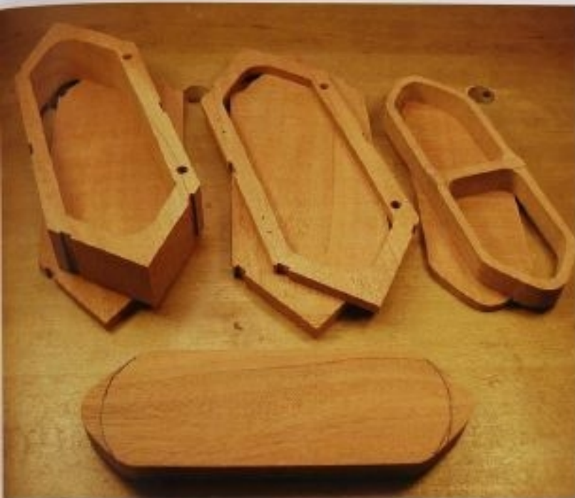
FIG. 5 There are many pieces to this box, so use lots of registration marks to keep them all in the correct order for gluing. For the grain to remain consistent, you need to glue the pieces back where they came from. This is not an easy thing to do. The foreground scrap piece has been marked for cutting to make tray supports.
