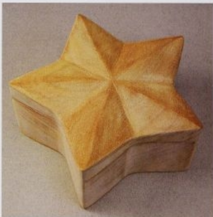
FIG. 21 The box has been sanded to 220-grit. Start with coarse, 80-grit sandpaper to get the carving marks out, and then move to 120-grit before finishing with 220-grit. Wrap the sandpaper around a flat block so the sides of the star's points remain flat.
