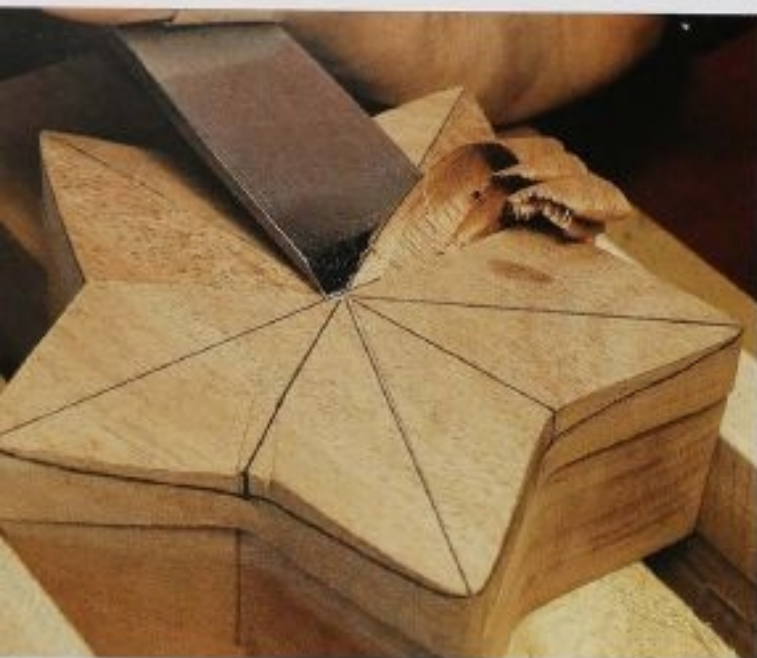
FIG. 19 Carving is almost always a gradual slicing away of wood. In that way you have control over the depth and extent of your cut. If you try to remove too much wood at once, you likely will remove a point from your star.
