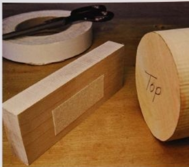
FIG. 13 To attach a stabilizing block to a small or odd-shaped piece to be cut, use cloth-backed, double-sided tape. Thick cloth-backed tape will bridge gaps between pieces of wood better than thin tape. Attach the two pieces while they are both resting on a flat surface so they will act as one unit as they go through the band saw blade.
