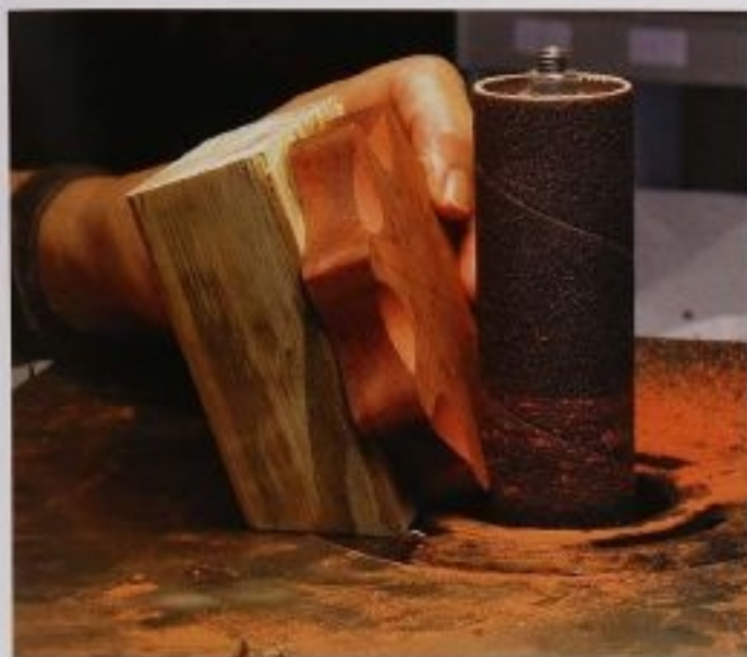
FIG. 5 By using this inexpensive shop-made jig (a cut-off 2x4" scrap), you can control the angle of your scallops on the top and bottom surfaces. Stop frequently to check your depth because it's easy to get the depressions uneven. Note that one hand has been removed in the photo setup for clarity, but this job requires both hands.
