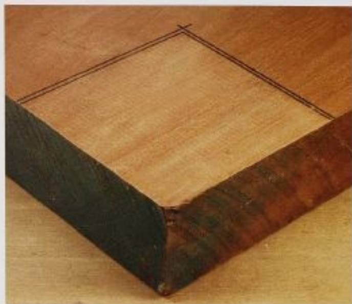
FIG. 1 Double lines will help you to get a clean, square block from a larger piece of lumber. Cut the block first on the outside lines; then, with the newly cut clean sides on the fence, cut off the rough edges.
