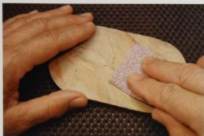
FIG. 35 Use a rubber nonslip mat to keep the piece from sliding around as you work. A soft mat not only protects your box, but also keeps the workbench from getting scratched.
