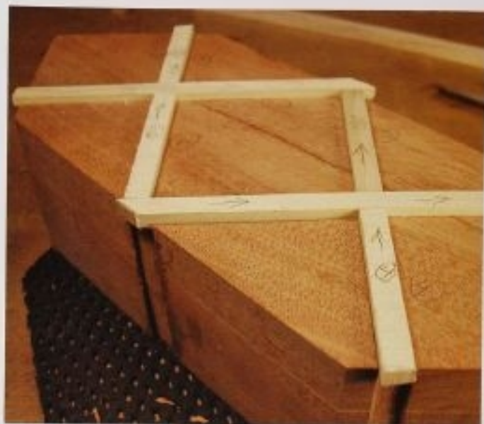
FIG. 3 Fit all the lid inlay sections before gluing. Make the butt joints as snug as possible, and allow the edge pieces to extend over the sides by \frac{1}{8} ". Glue these pieces in place before proceeding.
