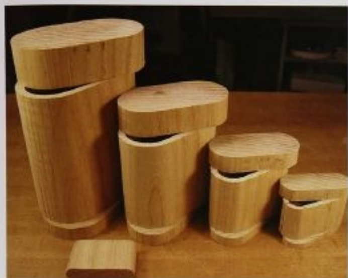
FIG. 5 These four boxes are ready to be glued together. Making many boxes from one piece of wood is a good way to save on wood costs. It also saves setup time.
