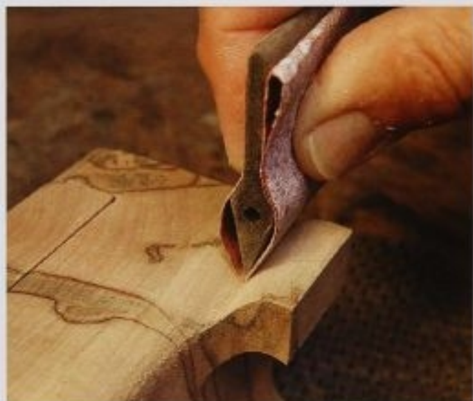
FIG. 10 In places that the belt sander cannot reach, like the groove above the feet, you will need to use either a powered profile sander or lots of elbow grease to get the areas smooth.
