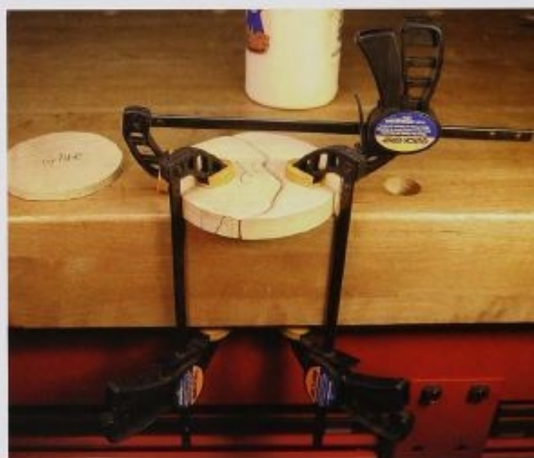
FIG. 3 When you glue the two lid pieces together, they will want to pop up at their joining edges. Avoid that problem by holding the pieces down on a flat surface with clamps during glue-up.
