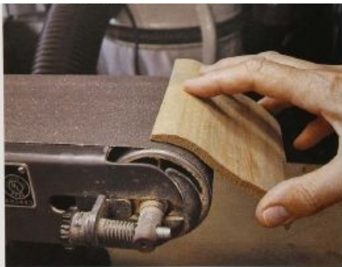
FIG. 33 If you need to sand a curved piece over the rollers, hold onto the wood firmly, but apply very little pressure to the sander.
