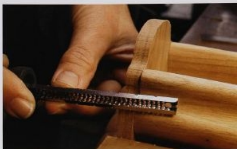
FIG. 9 The quickest way to remove excess wood is with a rasp. This small planing rasp, or micro-rasp, does a great job in these coved areas. Do not go too far. It is safer to carefully sand the last of the wood away. Hold the box in a vise or with clamps for safety. These rasps are very sharp.
