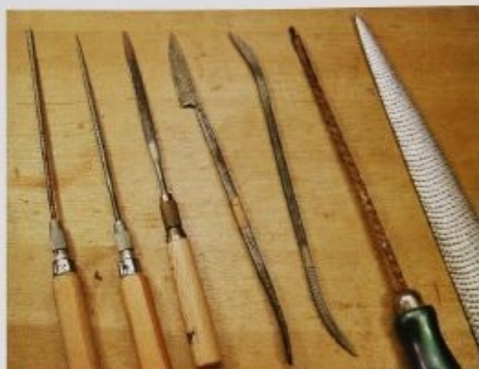
FIG. 40 Rasps come in hundreds of different shapes. Those with fine teeth will give a finer finish, and those with coarser teeth will remove wood faster.
