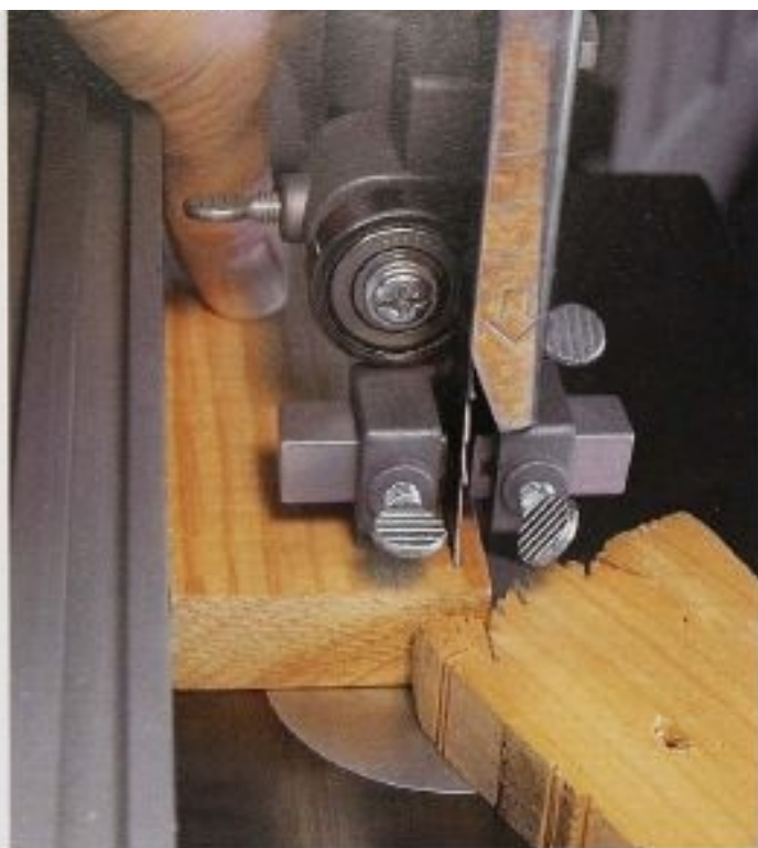
FIG. 10 Use a sacrificial push stick for the last push through a piece of wood. It is better to have a chewed-up, battle-scarred piece of scrap wood hit the blade than to take a chance of cutting your fingers.
