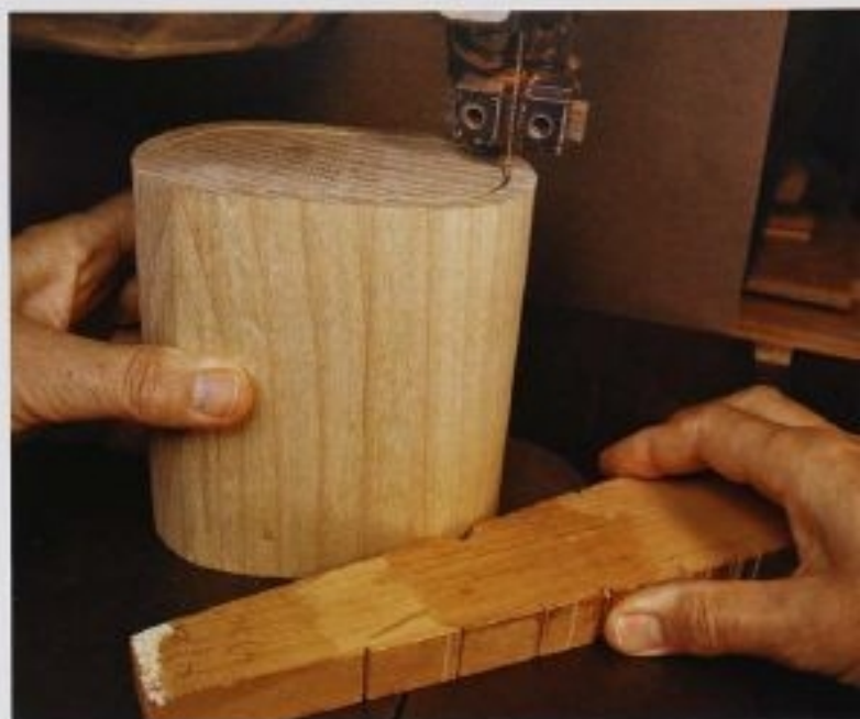
FIG. 1 When making deep cuts with your band saw, be extra careful to position your fingers where they will be safe when the blade comes through the block of wood. Remember the safety zone, and use a push stick to control the piece instead of using your fingers.
