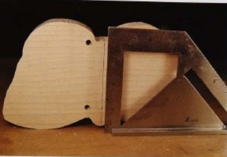
FIG. 1 The centerline of the butterfly body must be perpendicular to the front edges of the wings. If the line is not square, adjust the front edge of the wings until it is square.
