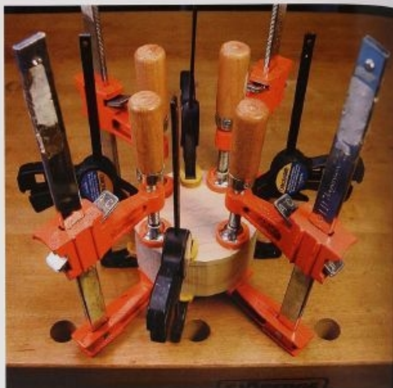
FIG. 5 You will want a lot of pressure when gluing the body to the base. The light-duty quick clamps were positioned first, and then the heavy-duty screw clamps were set in between them.
