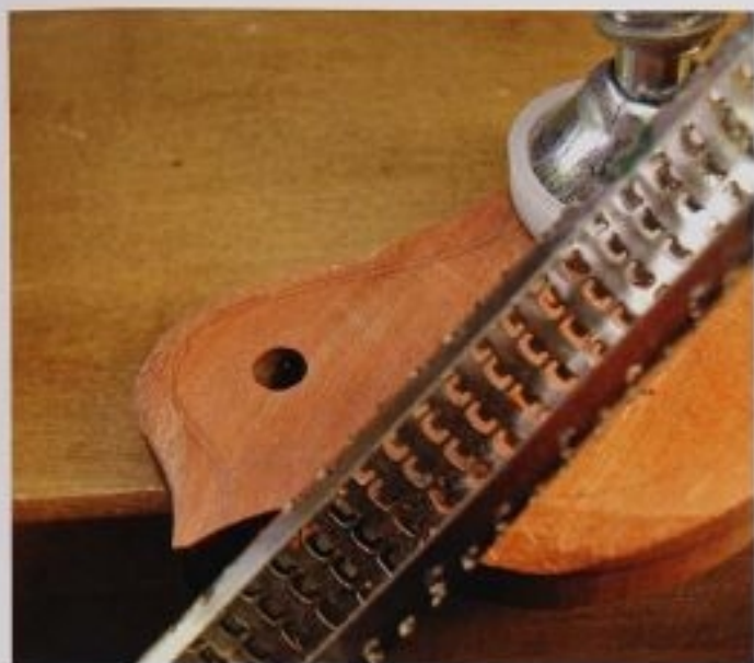
FIG. 9 Be careful when using these rasps. The teeth are as sharp as razor blades and, although they are designed to cut wood easily, they cut skin just as well. Hold the wood securely with clamps or in a vise so you can keep both hands behind the cutting edges.
