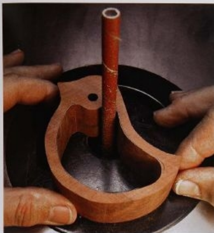
FIG. 4 Sand the interior of the body with coarse sanding sleeves to get the band saw blade's marks out of the wood and to make the sides evenly thick. Switch to finer grit sleeves to smooth the surface as much as possible. A little hand-sanding with 320-grit paper will finish the job. Here I'm using the oscillating spindle sander with a \frac{1}{4} "-diameter sleeve to get into the tight curve.
