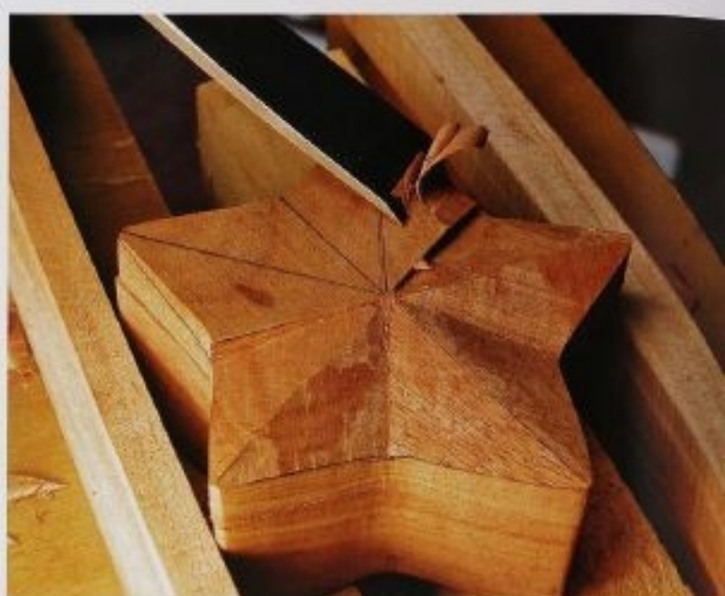
FIG. 20 You need a lot of control to keep your blade from cutting into the wood on the opposite point. Work slowly and carefully.
