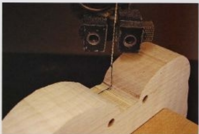
FIG. 4 Making the cuts through the body. Notice the stabilizing block attached to the back of the box to steady the tall block for an accurate cut.
