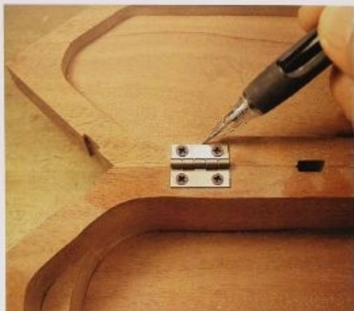
FIG. 7 Screw the hinges in place temporarily, and then trace around them with a fine line. Cut the mortises within these lines for a professional-looking, snug fit.
