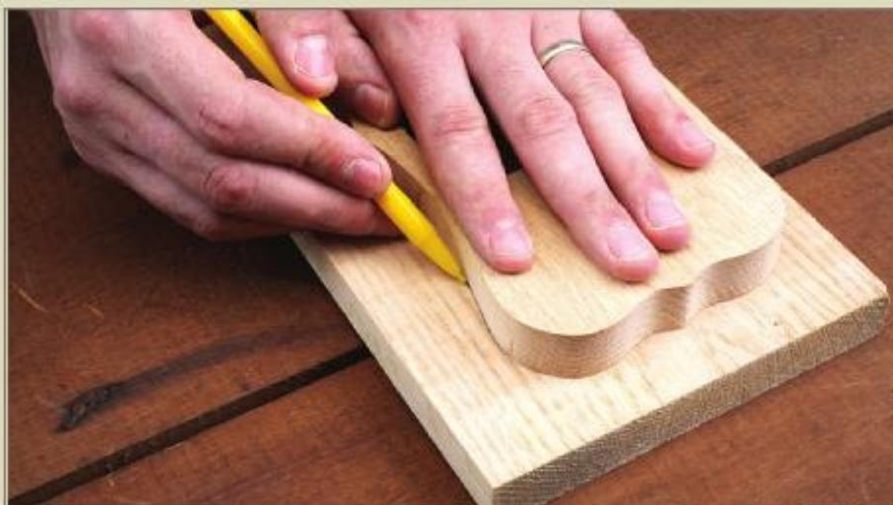
Figure 9. If you don't have 1½" wood for the frame, use two pieces of ¾"-thick wood. Once you have cut the first frame piece, attach it to the second piece of wood with screws. Then, trace the shape of the frame onto the bottom workpiece.
