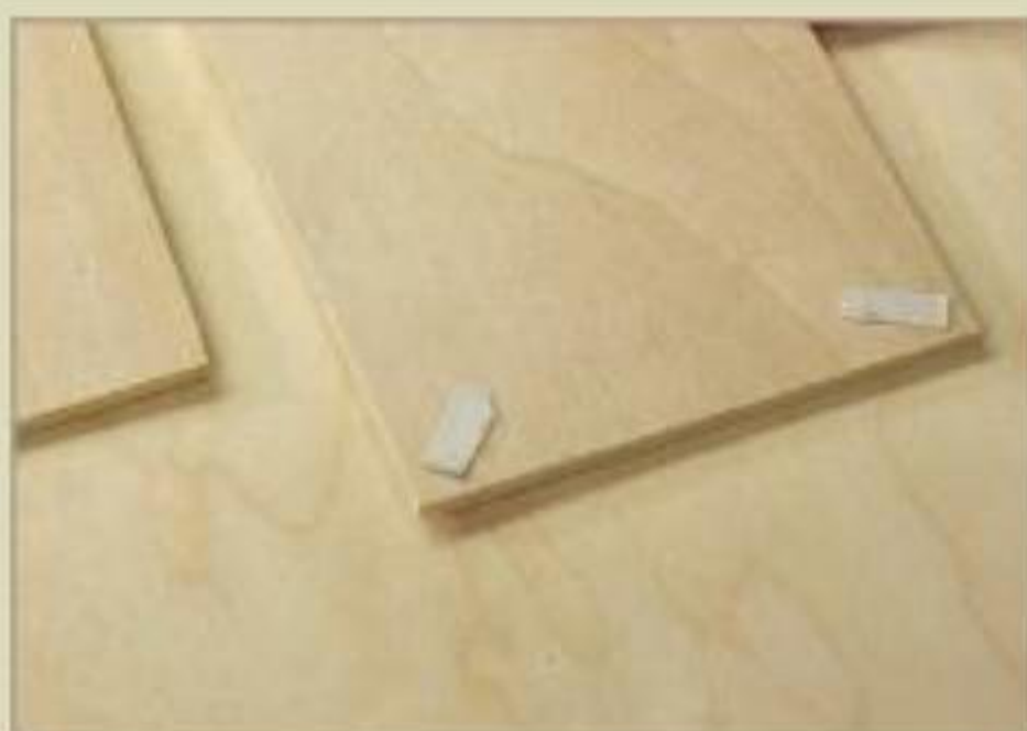
Figure 11. Masking tape or painter's tape (shown) placed around the edges can be used to hold a stack together. Some scrollers also like to cover the surface of the wood with tape before adhering the pattern to help lubricate the blade as it cuts. Placing double-sided tape in the corners of the stack can also be an effective method of holding the stack together.
