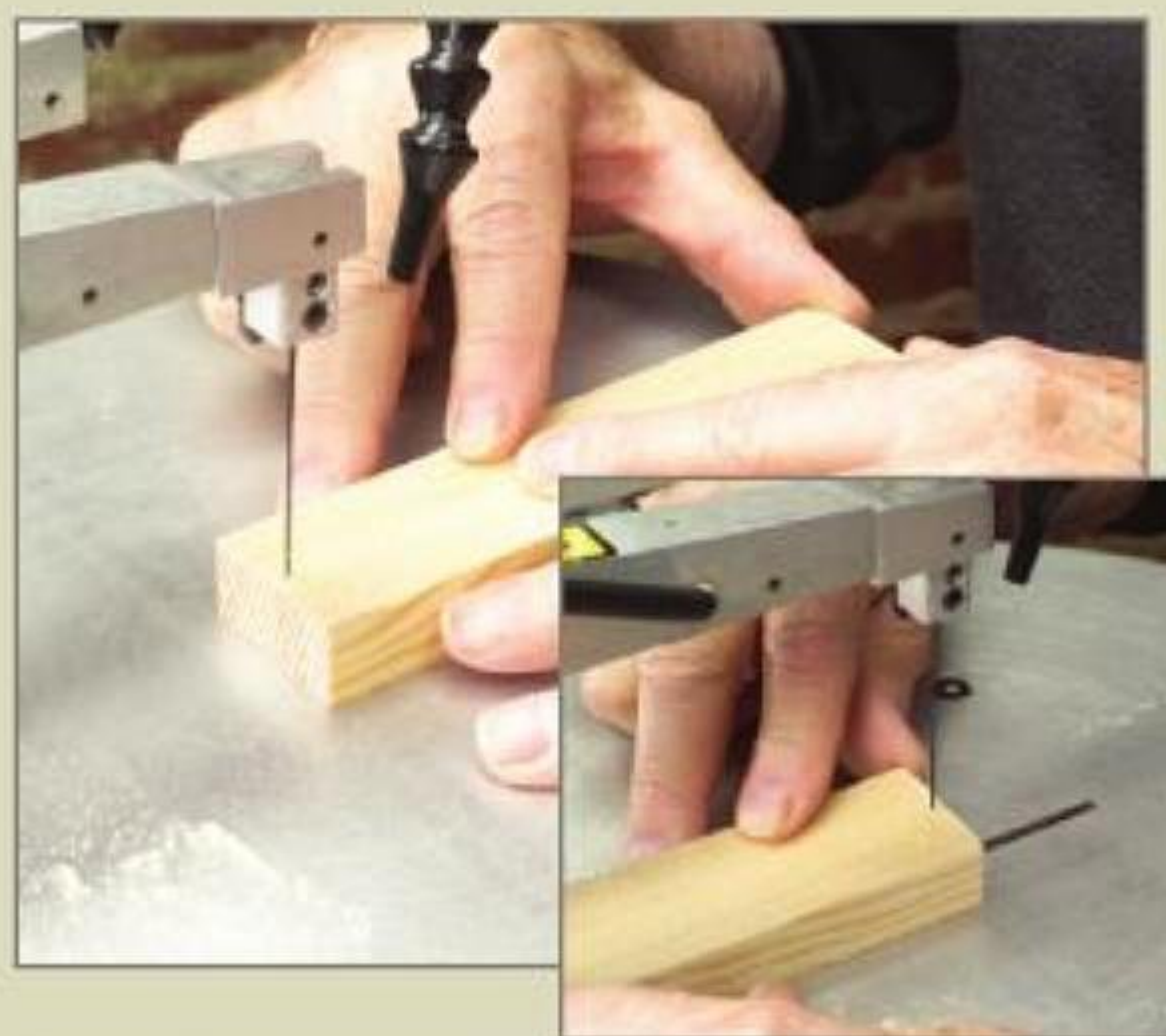
Figure 6. If you don't have a square, you can use a piece of scrap wood to square the table to the blade. First, make a small cut in the piece of scrap wood. Then, slide the cut toward the blade from the back. If the blade fits into the cut easily, the table is square to the blade.
