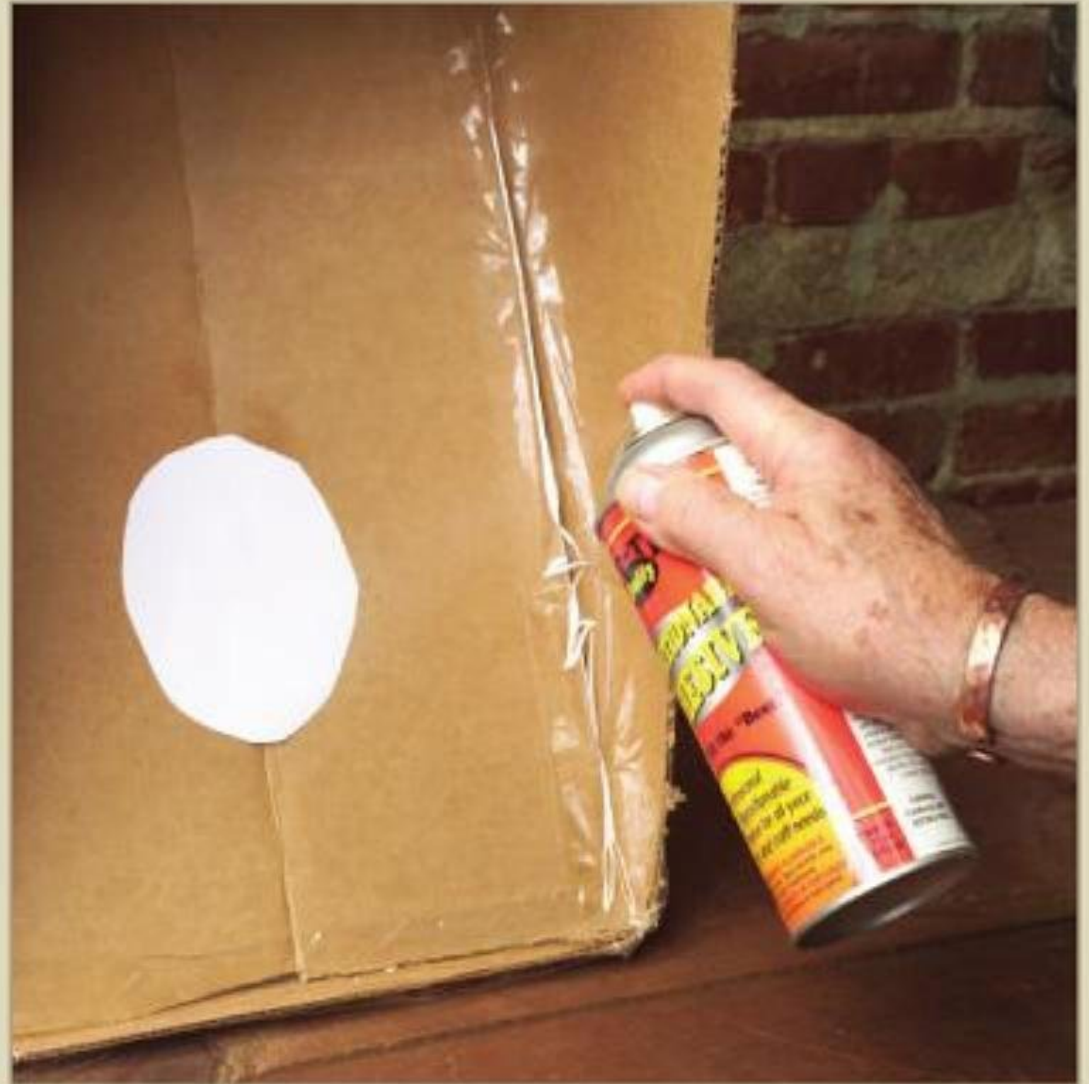
Figure 2. Use "repositionable" spray adhesive to adhere your patterns to the wood. A simple glue box, made from a common cardboard box, helps to confine the adhesive.
