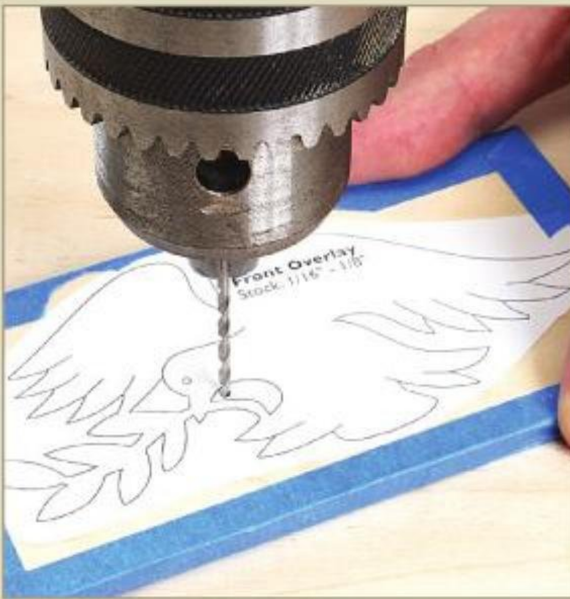
Figure 7. Drill any blade entry holes after adhering the pattern to the wood. Locate the blade entry holes close to corners so that it will take less time for the blade to reach the pattern line.
