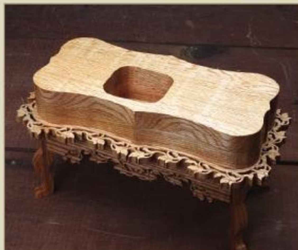
Figure 16. Set the frame in place to be sure that the music box movement is aligned correctly.
