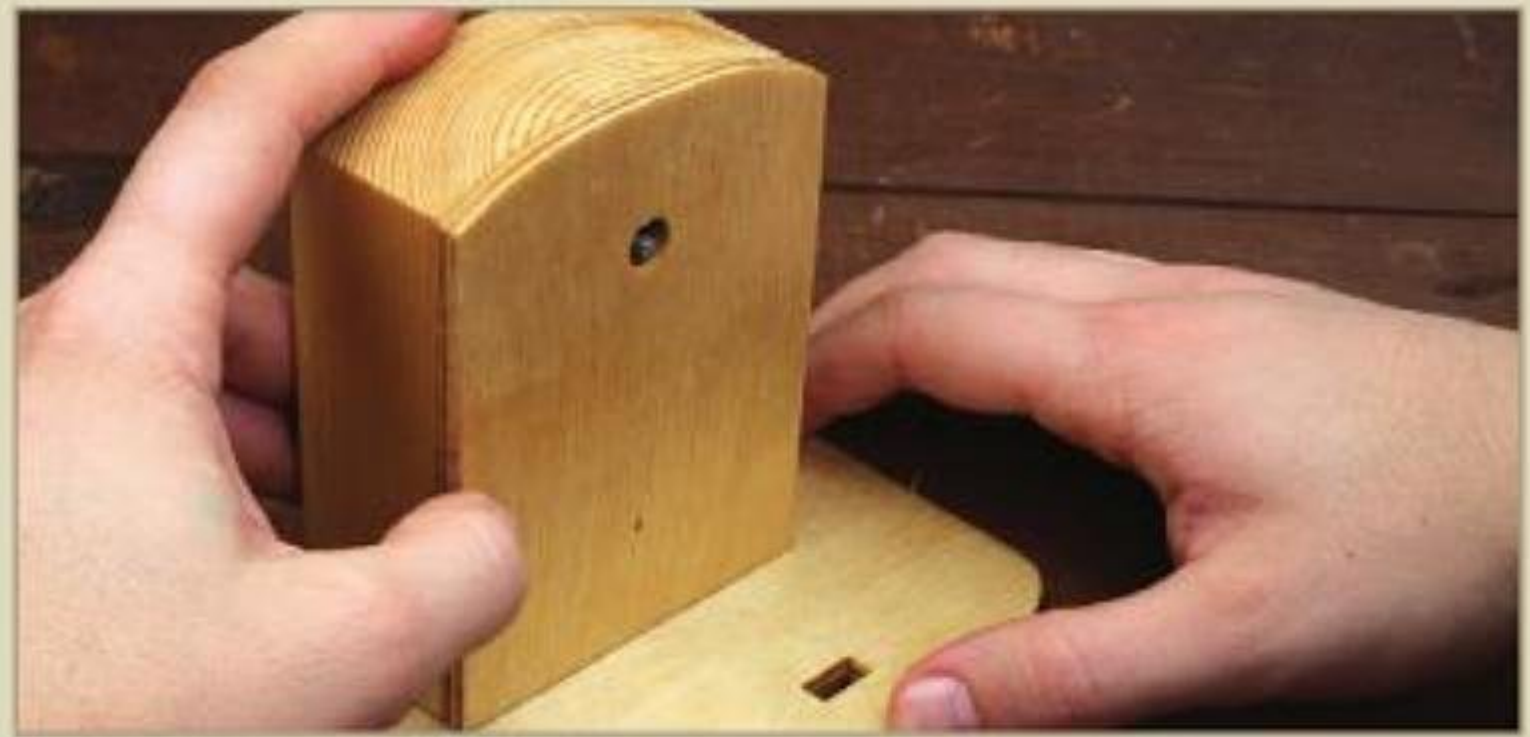
Figure 14. Attach the frame to the base. Due to the style of our music box, we attached the back cover to the front of the frame.
