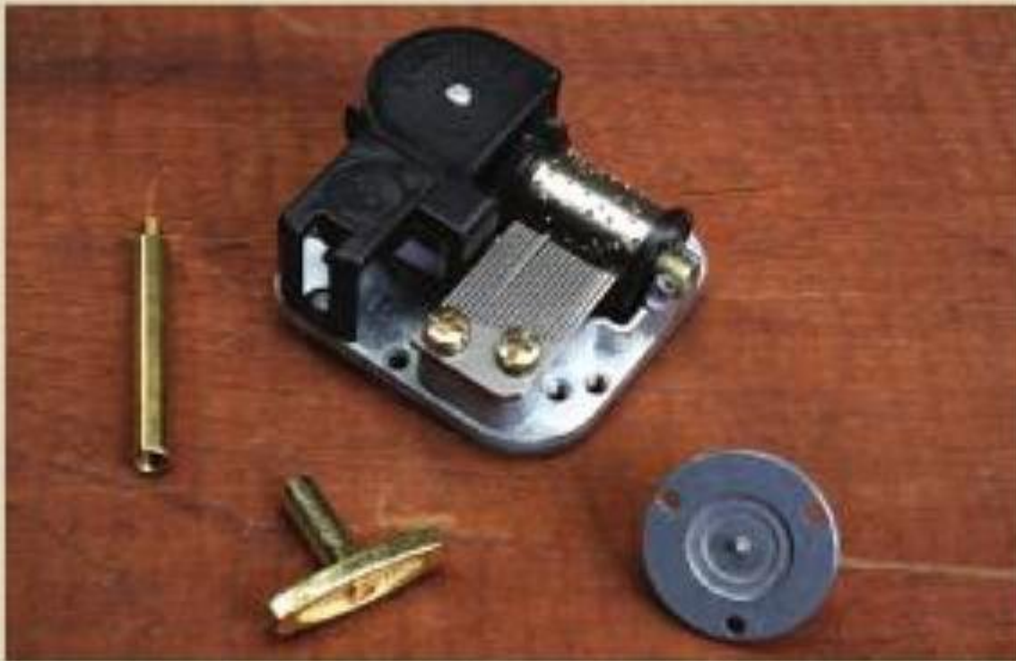
Figure 13. The music box movement and components you choose will depend on personal taste and on what is available in your area. Pictured here, clockwise from the top, is a music box movement, a turntable, a key, and an extender.
