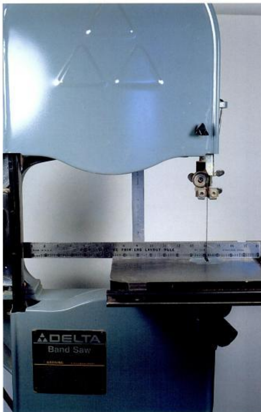
Photo 1-1 Make certain your band saw's clearances are adequate for the box design you decide to make.
