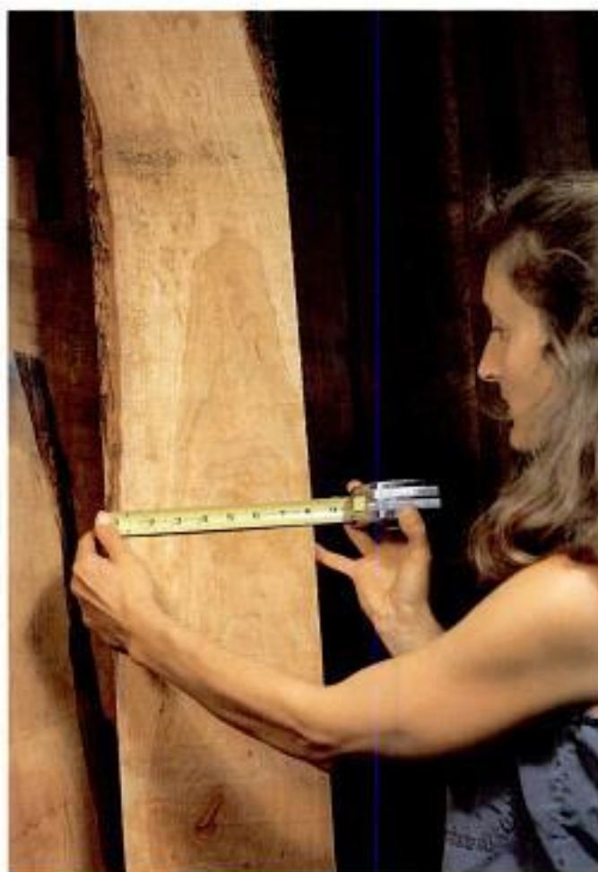
Photo 2-2 Keep your project dimensions in mind in order to minimize waste when selecting stock. Also remember that a board with sapwood can become a stunning band saw box.
