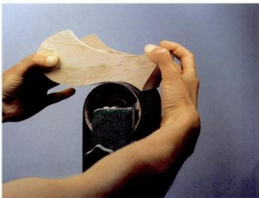
Photo 4-8 Sand the drawers carefully and thoroughly, but don't remove too much wood.
