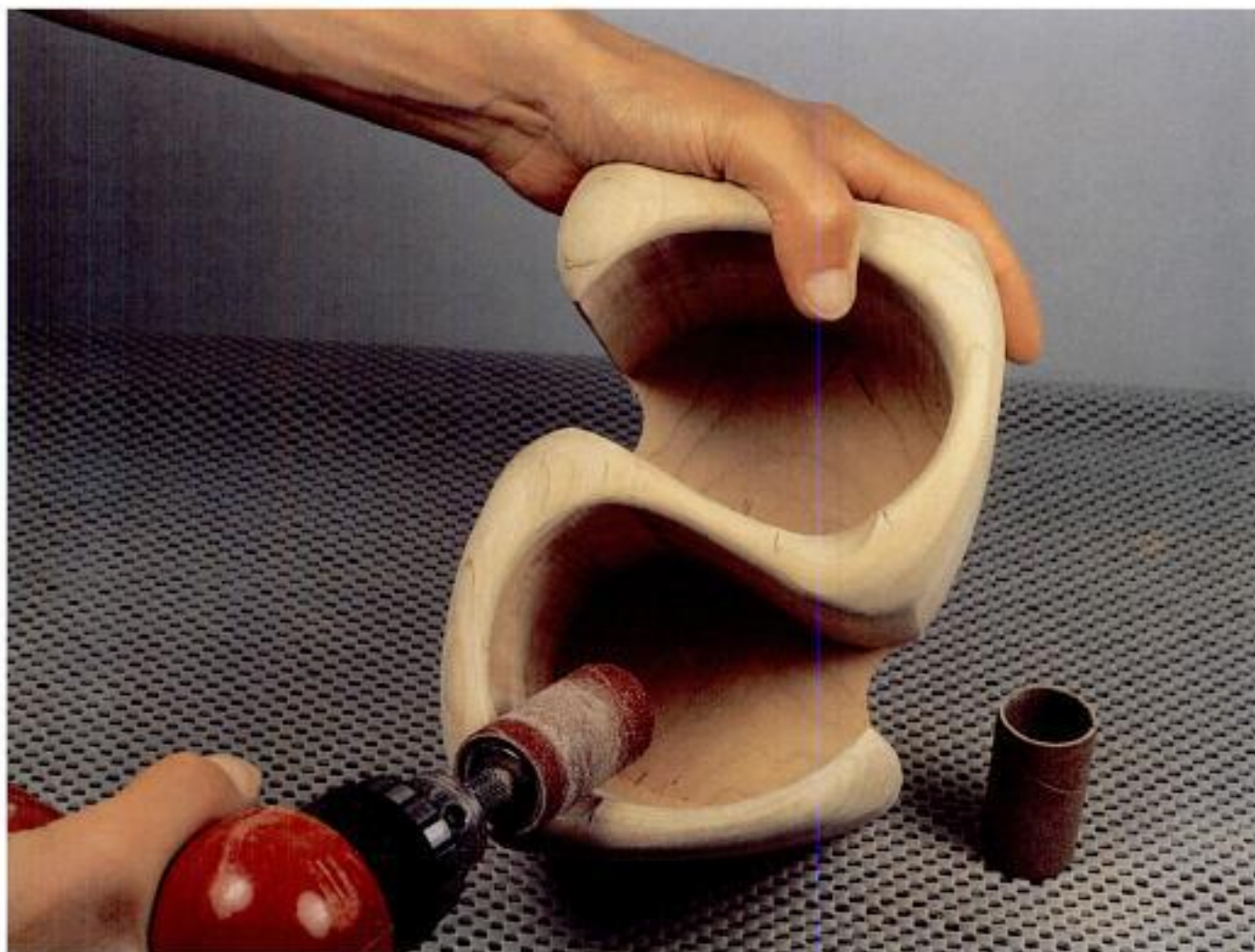
Photo 4-25 Shape the box slots in the same manner as the drawer slots. During the process, try the drawers to make sure the slots line up. Don't remove too much material!
