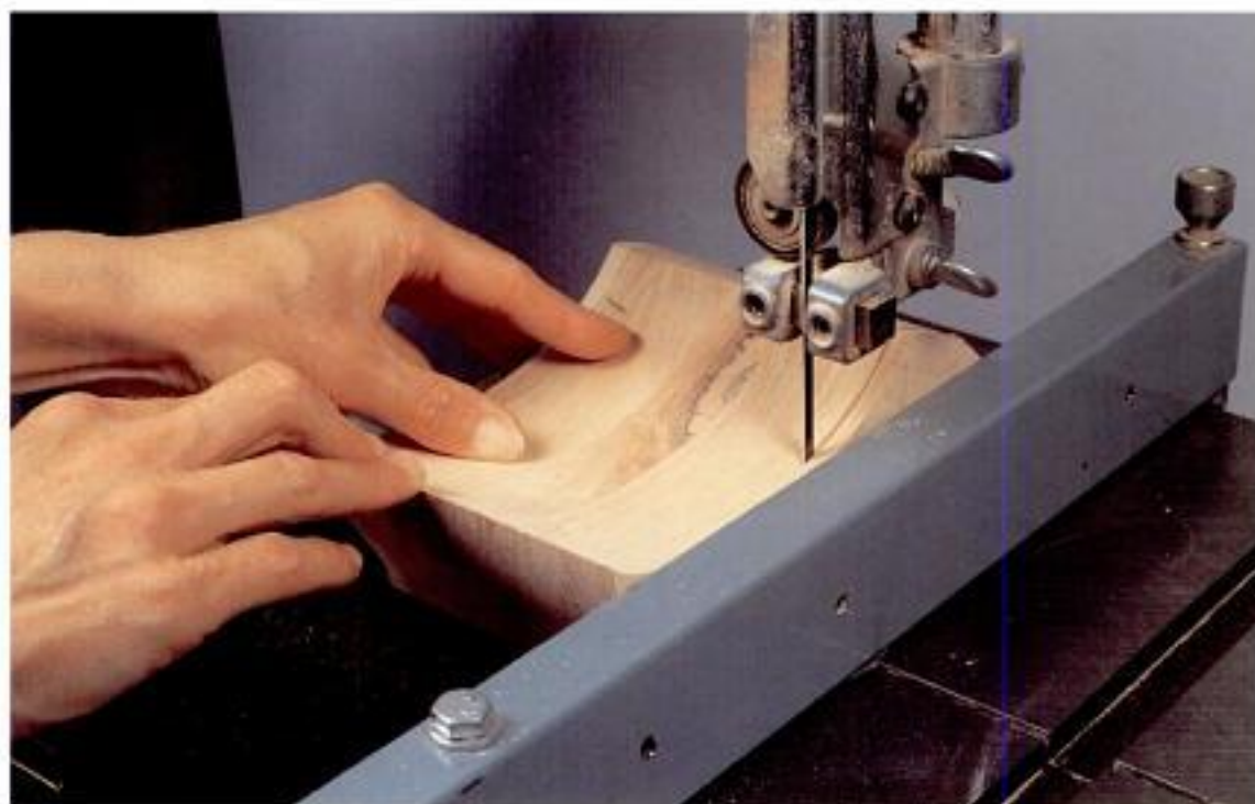
Photo 3-9 Rip \frac{1}{4} " (6mm) off the backs of the drawer blocks. When finished with all the blocks, reset the fence to \frac{1}{8} " (1.3cm) and rip the drawer fronts off.
