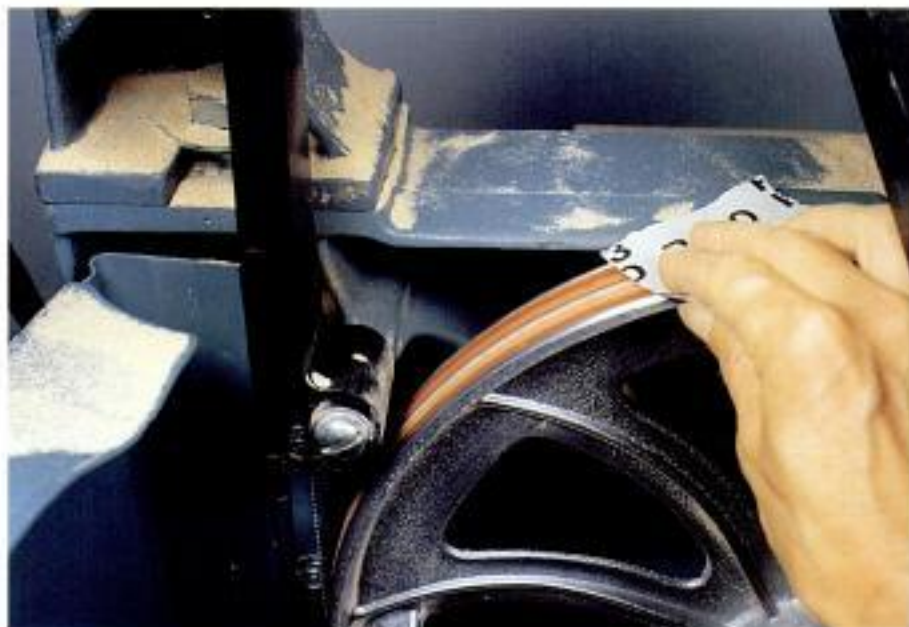
Photo 3-2 Clean band saw tires will improve the quality of your cuts.
