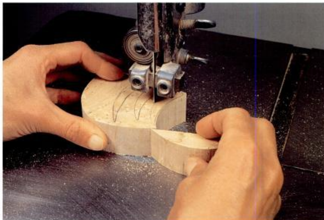
Photo 3-20 Always use a push stick or equivalent to assist in cutting out the tiny drawer pulls.
