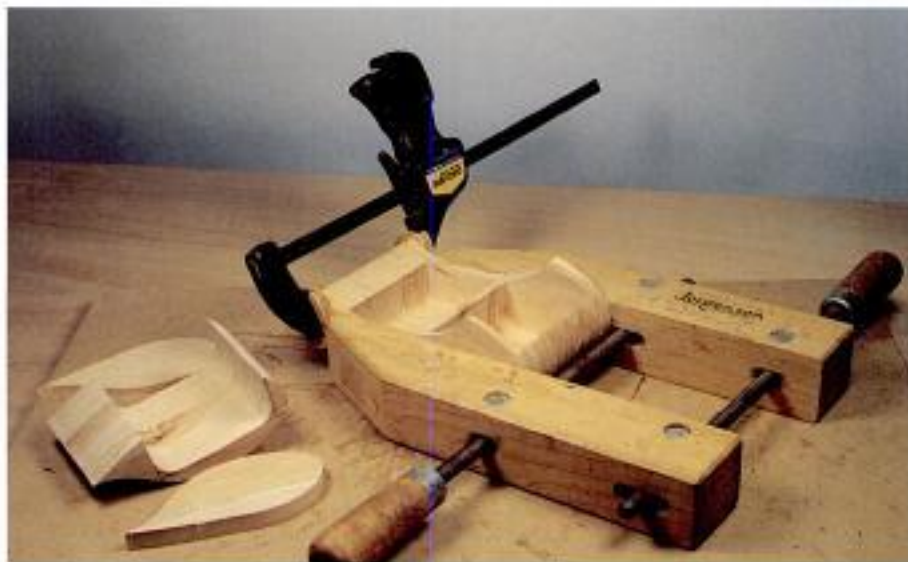
Photo 3-17 A hand screw and a flat surface simplify the task of clamping drawers. In most cases, you'll have to work with the pieces to keep them even while you clamp.
