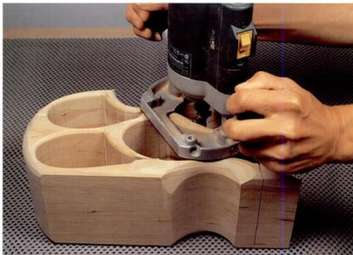
Photo 4-12 Round over the drawer opening with a \frac{1}{4} " roundover bit.
