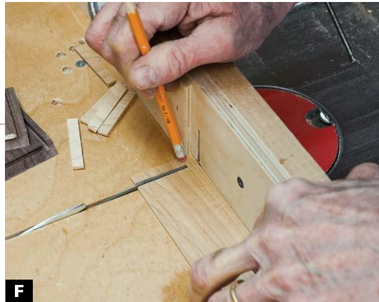
CUT THE SPLINE STOCK to exact length using the crosscut sled and stop block.
