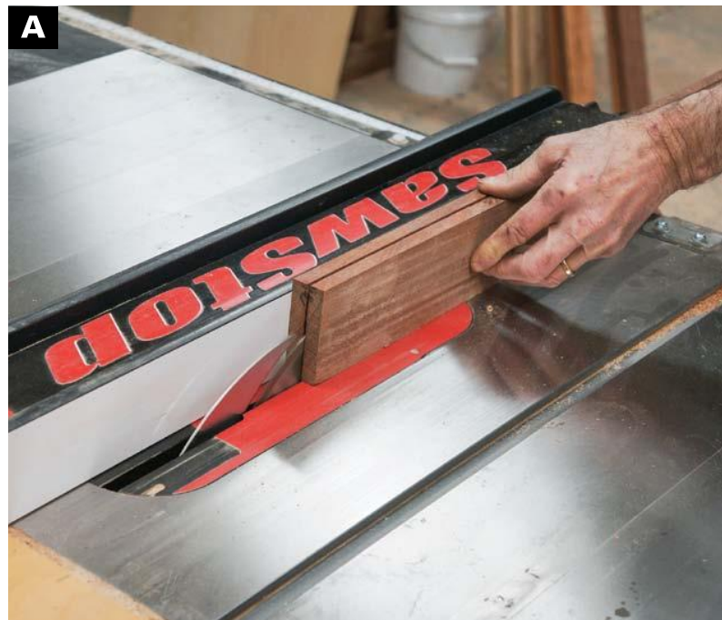
USE THE TABLESAW (or bandsaw) to resaw stock for the box sides. Keep the tablesaw blade set at just barely above half the thickness of the stock.
