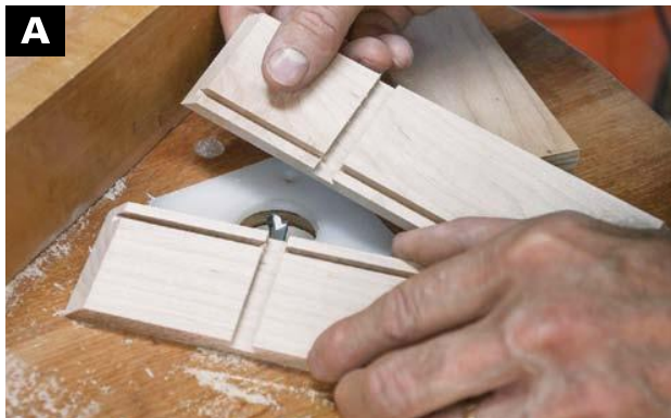
ROUT THE SIDES between stops in matched pairs for the installation of the dividers. Use a dovetail bit or straight bit. The dovetail adds greater interest.
