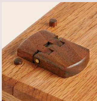
This flat shopmade hinge is screwed from underneath.
