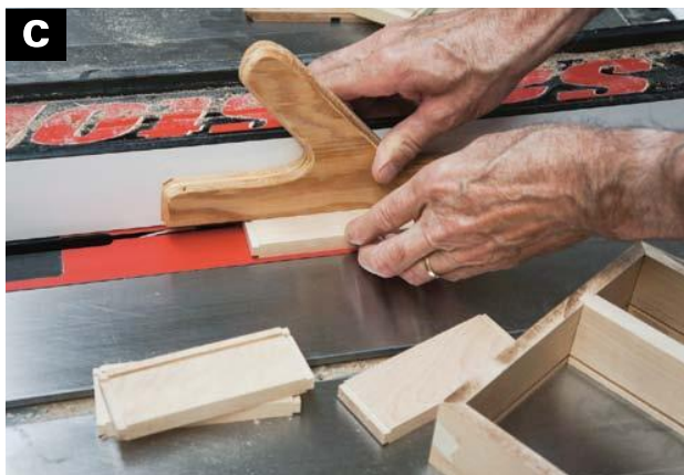
USE THE TABLESAW to cut grooves in the dividers for the bottom panels.
