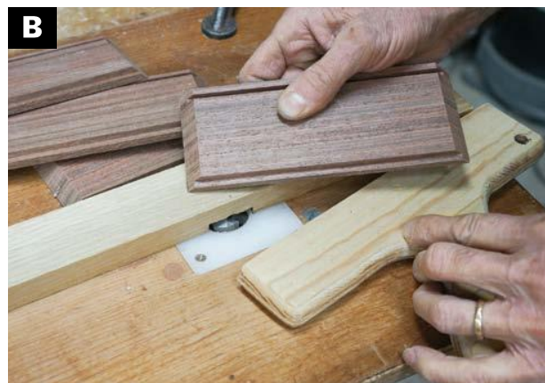
USE THE TABLESAW to cut grooves in the sides for the bottom panel to fit. Cut \frac{3}{16} in. deep.
