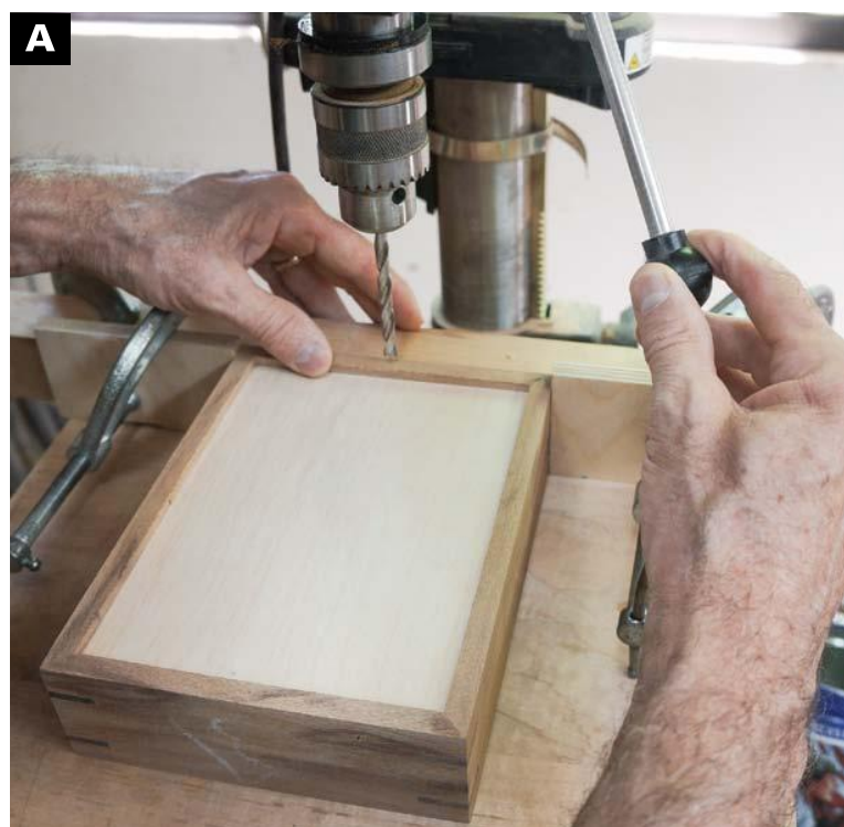
TO DRILL TO FIT the rare earth magnets, set up the drill press with a fence in position so that the tip of the \frac{1}{4} -in. drill falls at the center of the \frac{3}{8} -in. stock. Set up stop blocks on the left and right to position the box so that the drill will hit dead center from each side.
