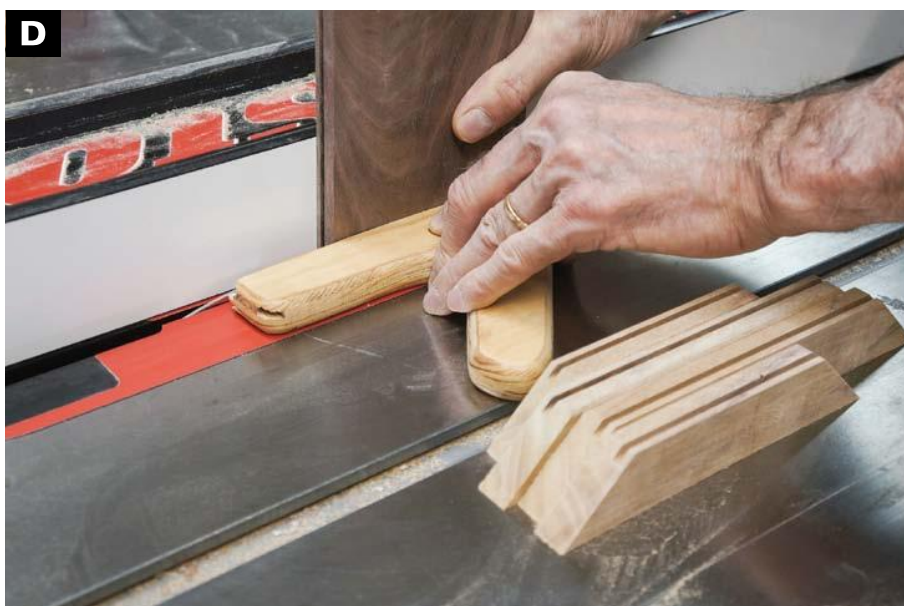
CUT THE GROOVES in the lid frame parts and then make a matching cut along each edge of the top panel.
