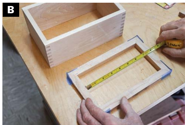
TRIAL ASSEMBLE THE BOX LID FRAME and close the corners tightly with tape so that you can accurately measure the size of the floating panel for the top.
