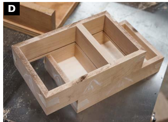
CUT THE BOTTOM panels to fit, proceed with assembly, and install the magnets at the center of each divider strip.
