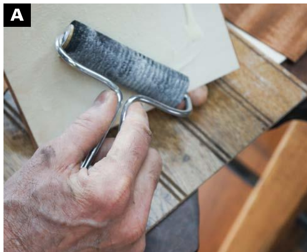
SPREAD GLUE on the Baltic-birch plywood panel for the top.
