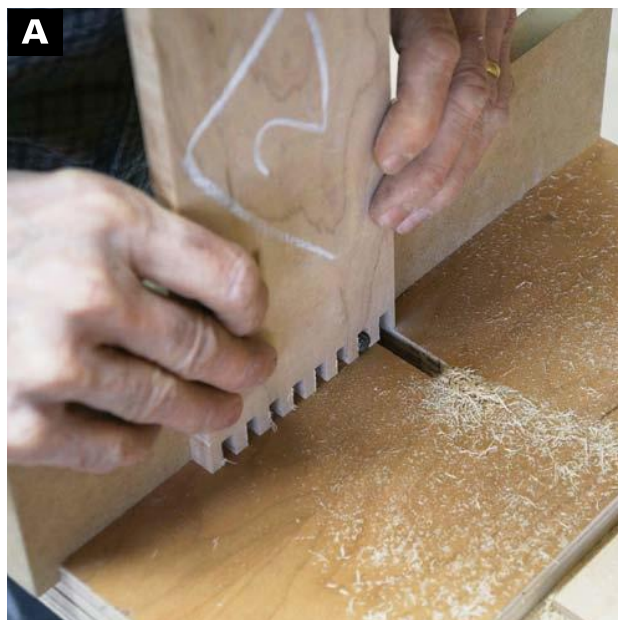
USE A ROUTER TABLE SETUP for finger joints to cut the finger joints in the box front and back. The guide pin positions the stock for each cut.
