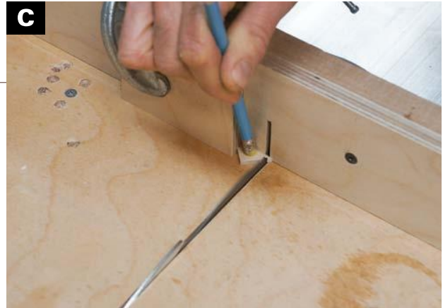
MAKING A TINY LIFT TAB takes some rather close work. Cut the tab from an extra miter key. Set the stop block on the sled and use the eraser end of a pencil to hold it tight as you make the cut.
