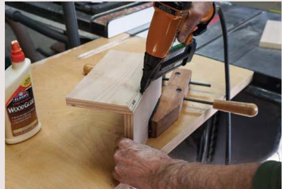
USE A BRAD or pin nailer to strengthen the cradle joint after the glue sets.
