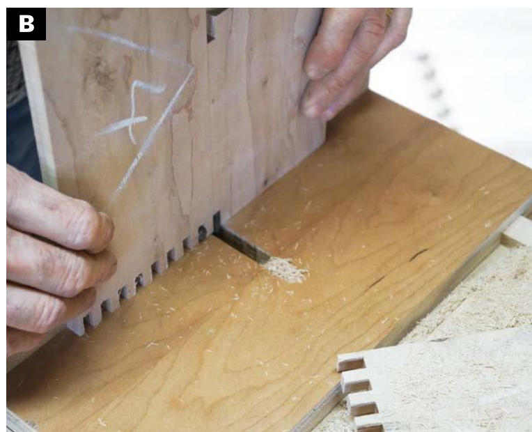
FLIP ONE OF THE FIRST CUT PARTS over and use it to position the first matching cut in each of the box ends.
