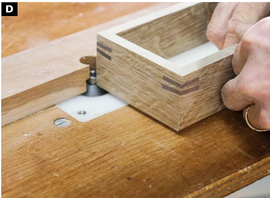
AFTER SANDING on the stationary belt sander, rout the bottom edge with a 45-degree chamfering bit.
