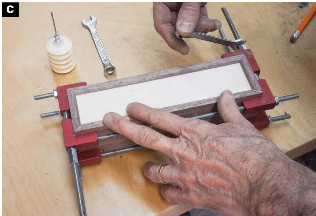
USE CLAMPS to pull the corners tight.
