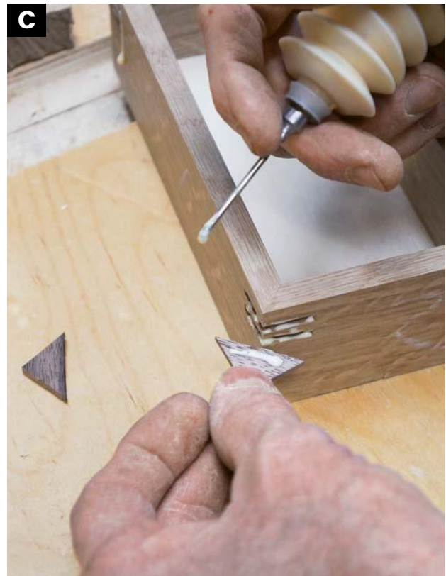
SPREAD GLUE in the key slots and then individually on each key as it is pushed into place.
