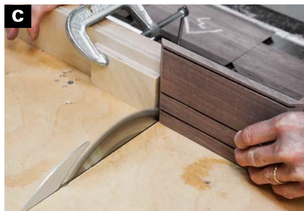
CUT THE FRONT edge of the box sides to allow for the drawer front. The blade height needs to be set carefully to cut no higher than the opening for the drawer.
