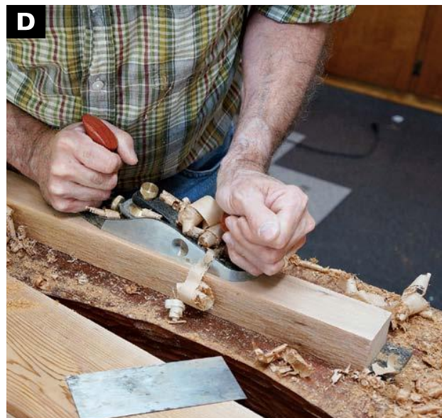
PLANE THE MATERIAL for the box sides smooth and square on all sides.
