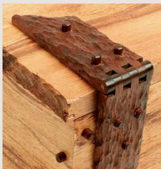
Wood pins secure an L-shaped shopmade hinge.
