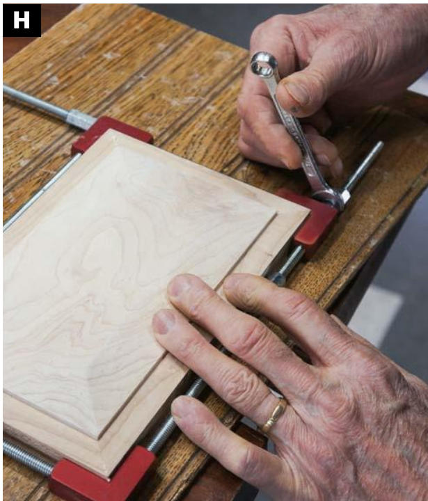
USE A FRAME CLAMP to hold the lid parts tightly as the glue sets.
