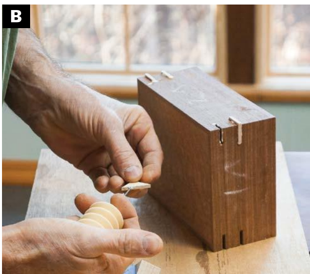
INSTALL AND GLUE all the keys in place.
