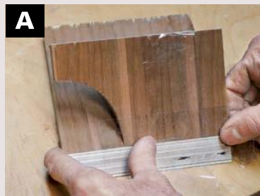
USE TAPE TO ALIGN the front part of the jig to the base.
