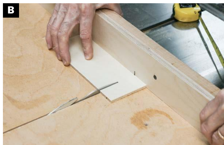
USE A CROSSCUT SLED on the tablesaw to cut the Baltic-birch plywood bottom to length.
