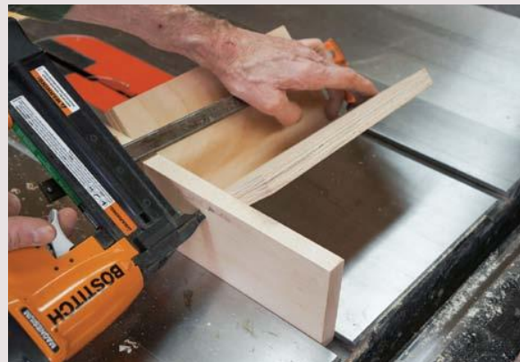
DRIVE BRADS OR pins through the slider into the "V"-shaped body of the jig.
