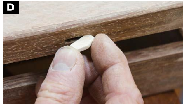
PUT JUST A DAB OF GLUE in the slot before you glue the lift tab in place.
