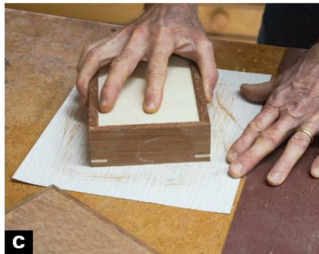
USE A SHEET OF SANDPAPER on top of the workbench to sand the edges of the lid and body of the box flush.
