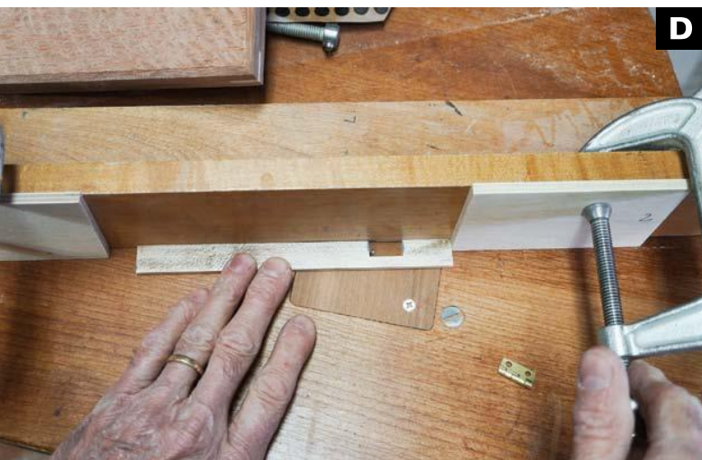
SET STOP BLOCKS left and right to control the travel of the box lid and body on the router table.
