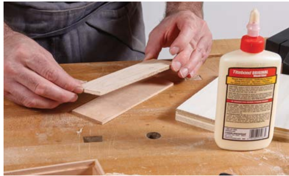
2. Glue the veneer (smooth face down) to the outside face of the bottom.
