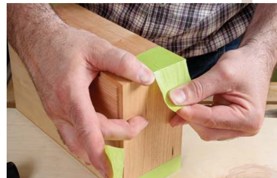
6. Stretch tape over the last mitered corner to apply clamping pressure.
