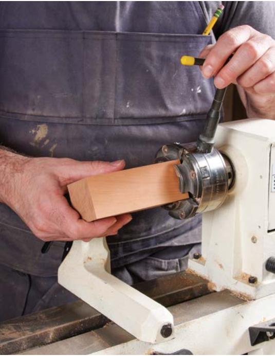
1. Mount the box in the lathe chuck.
