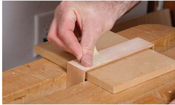
2. Sand the surfaces, starting with 320-grit paper and working up as far as 600-grit (for highly figured woods).
