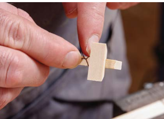
10. Start the wrap next to the inside edge of the foot.
