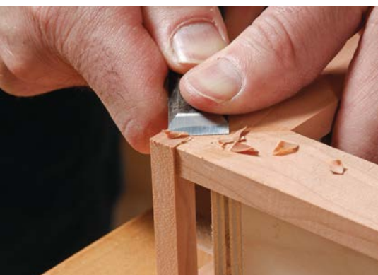
10. Pare the leg length flush to the frame.
