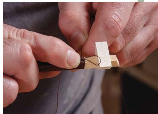
12. Form a loop in the thread and put it under the wrap.
