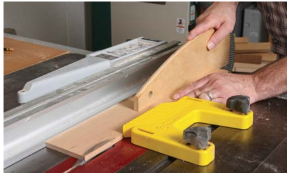
8. Trim excess width from the overhang of one board.
