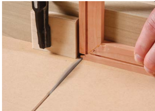
4 & 5. Notch the frames to accommodate the "legs."
