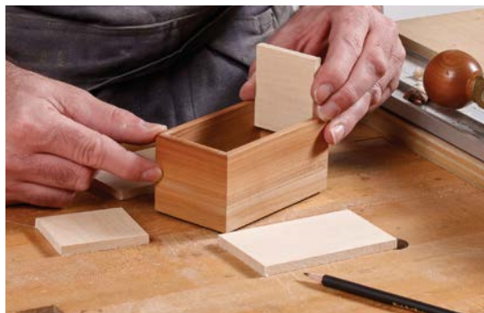
2. Trim the sides of the bottom box pieces to fit into the lid box.
