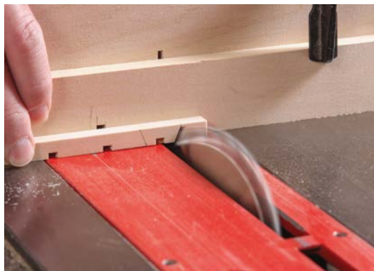
5. With the sawblade angled, cut the first beveled side of the foot. The notch is over the tab.
