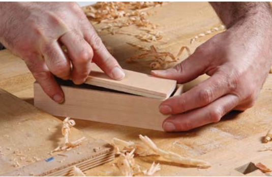
5. Fit the veneered bottom in the box.
