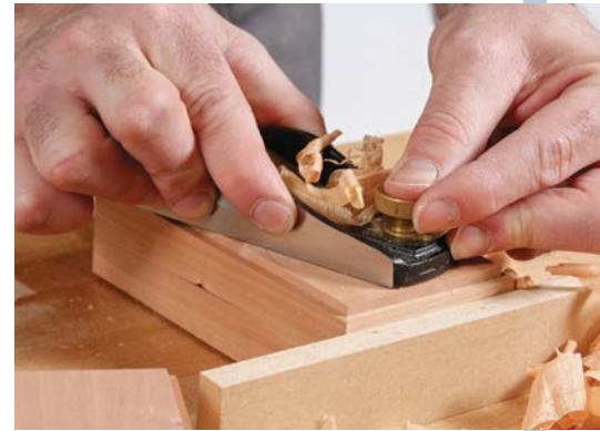
3. Plane the box tops to dial in the reveal between layers.
