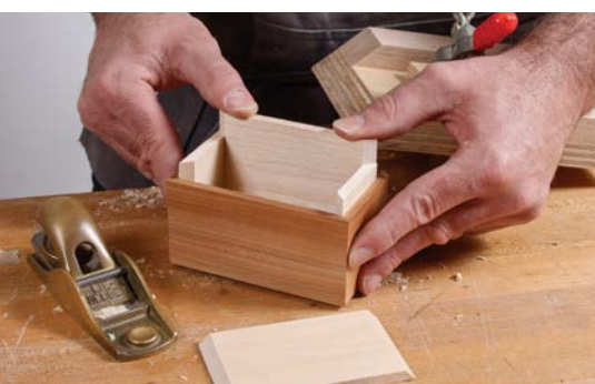
4. Test the fit by placing the bottom box sides into the lid.
