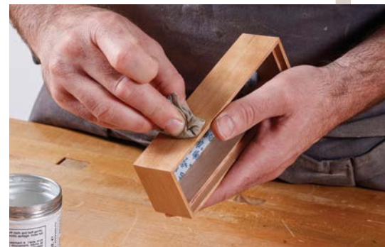
6. Finish by waxing all the shellacked surfaces.
