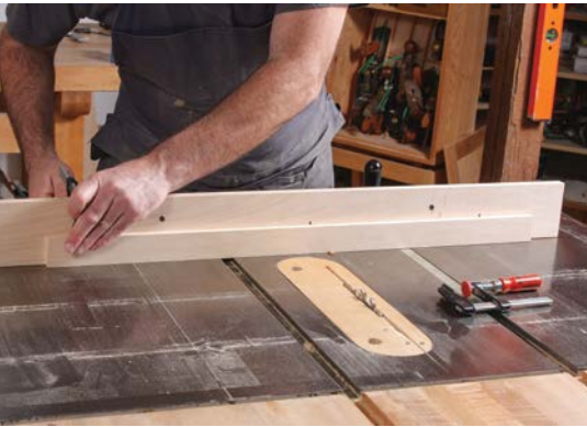
1 & 2. Clamp the notching jig (with attached tab) to the sled fence.
