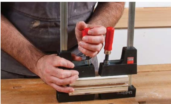
3. Clamp between cauls, and allow an hour or two for the glue to dry.
