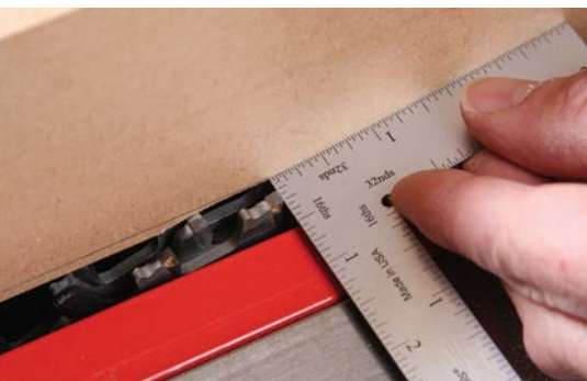
4. Set the fence to cut the width of the rabbet.
