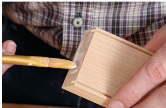
2. Spread the size on the mitered joints.
