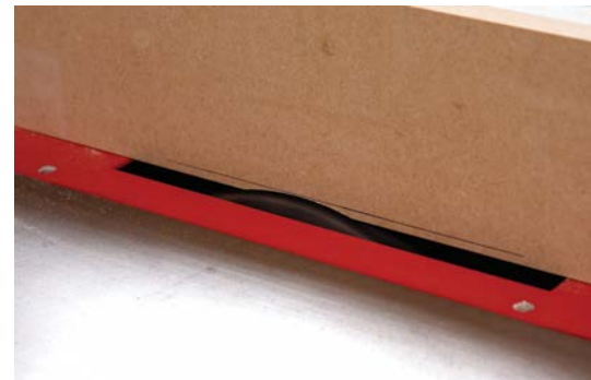
3. Raise the dado head until it reaches the mark on the auxiliary fence.
