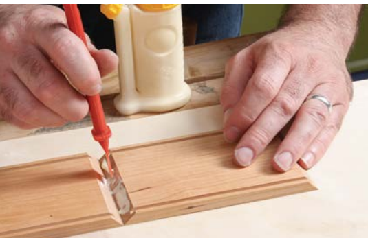
4. Carefully spread glue over the miter joints, except the open ends.
