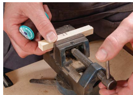
9. To prepare to wrap the pull, clamp the thread in a vise.
