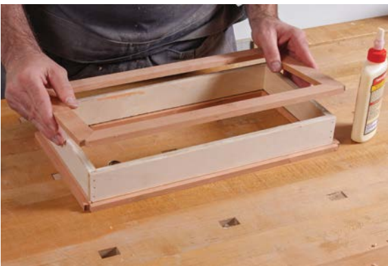
7. Glue the frames to the inner plinth.
