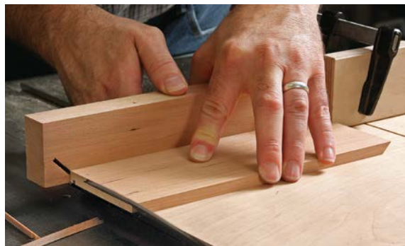
2. With the top corner of the side aligned with the edge of the kerf in the sled fence, cut the miters at the tablesaw.
