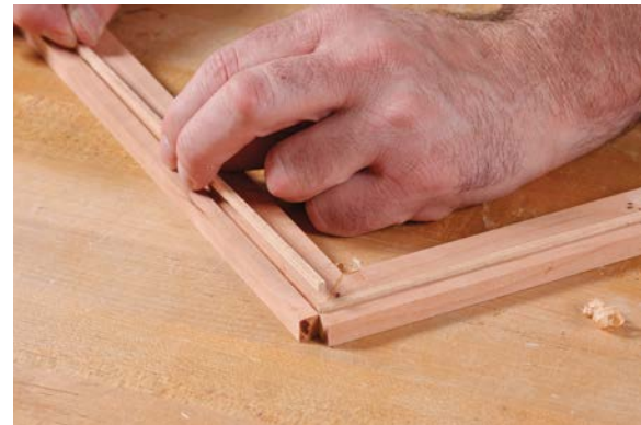
6. Set strips of wood into the grooves.
