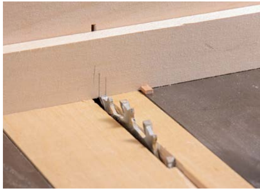
1 & 2. Clamp the notching jig (with attached tab) to the sled fence.
