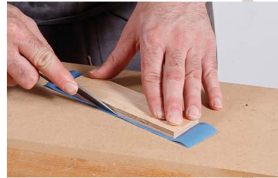
7. Trim the tape flush with the edges of the bottom.
