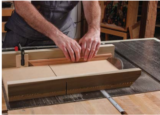
2. Miter the frame parts.
