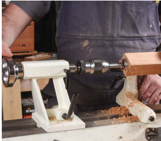
2. To drill the hole, advance a 1½-in. Forstner® bit into the end of the box.
