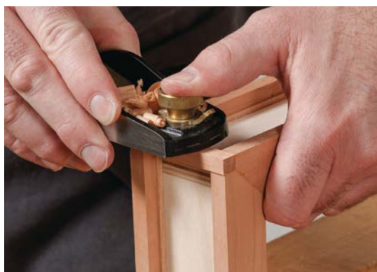
11. Plane the leg thickness flush to the frames.
