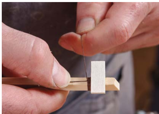
11. Continue wrapping the pull.
