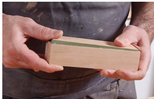
15. Press the bottom into the rabbet.
