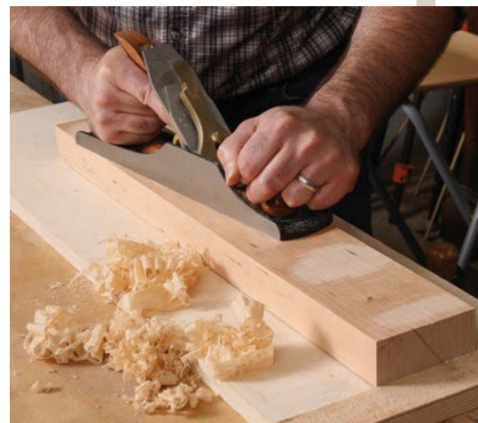
6. Re-joint the original face with a No. 5 jack plane.
