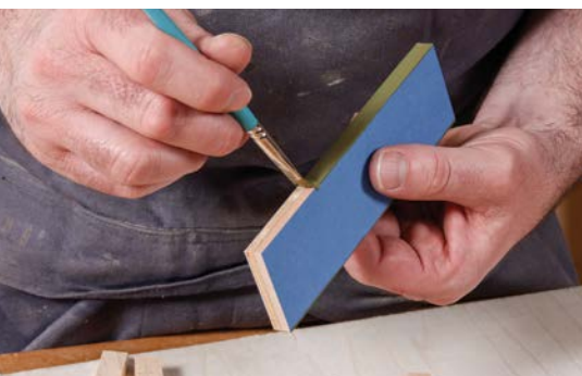
8. Paint the edges of the bottom with milk paint.
