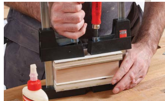
16. Using cauls to protect the edges, clamp the bottom to the box.
