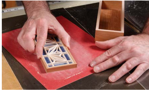
2. Sand the cut edges with a circular motion.
