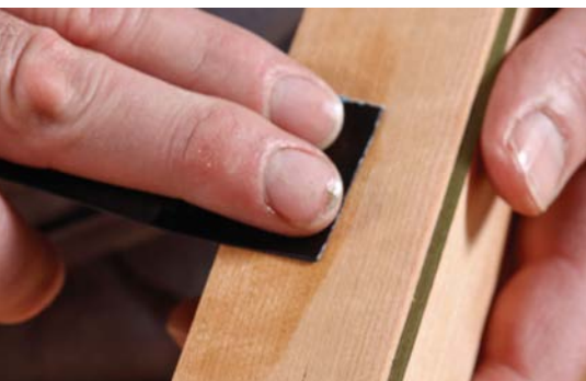
4. Wet sand with 800-grit wet/dry paper and mineral spirits. Apply a third coat and let dry.
