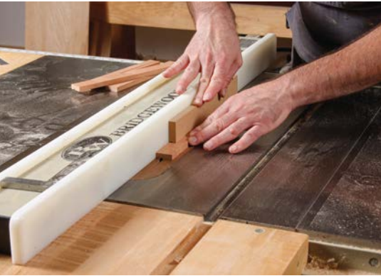
1. Cut a groove into the frame parts.
