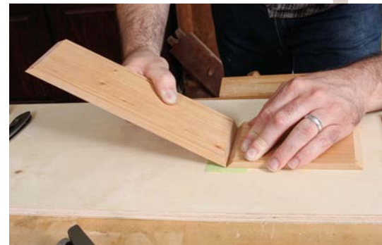
3. Keeping the two mitered tips tight together, tape up the first joint.
