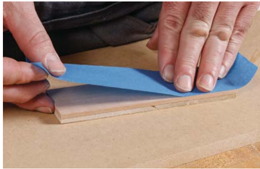
6. Completely cover the veneer face with blue painter's tape.
