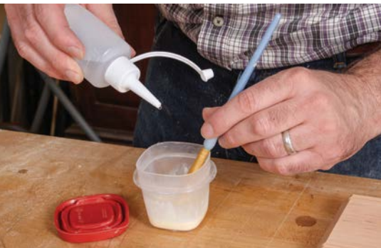
1. Mix the glue size using equal parts yellow glue and water.
