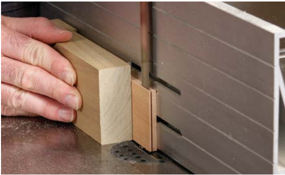
1. Resaw a veneer that's a little wider and longer than the plywood bottom.
