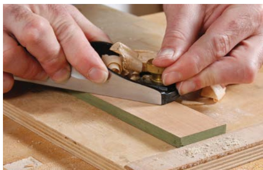
9. Remove the tape and plane the veneer after the milk paint dries.
