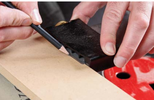
1. Mark the depth of the rabbet on the auxiliary fence.
