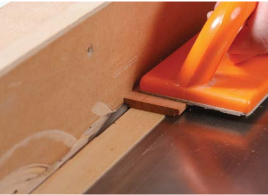
1. Cut the rabbets in the sides at the tablesaw.
