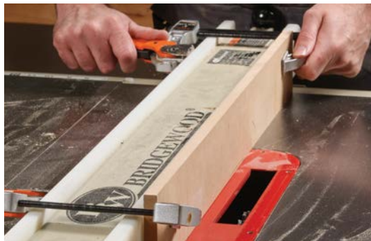
2. Clamp the auxiliary fence to the tablesaw's rip fence.
