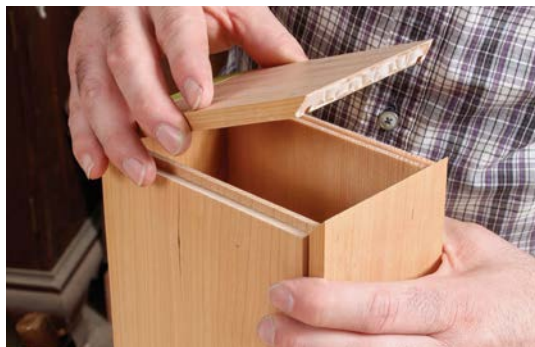
5. Place the top and bottom in the grooves in the sides and fold the sides around them. Before closing the final corner, apply glue to the miter faces there.
