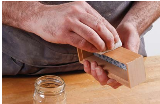
2. Wipe on the first coat.
