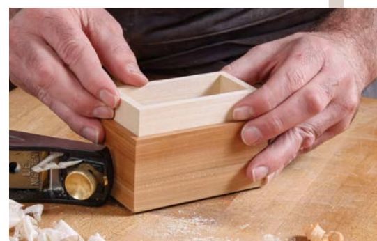
6. Slide the bottom box into the lid box.
