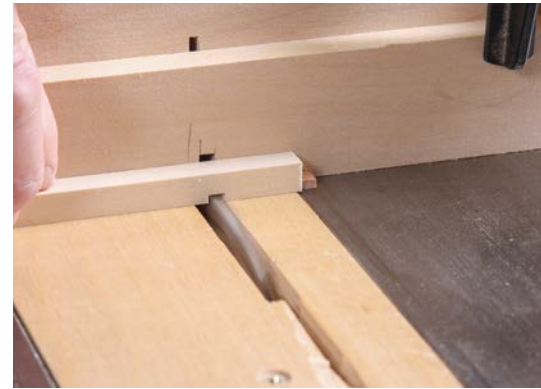
3. With the pull/feet blank registered against the tab, cut the first notch.
