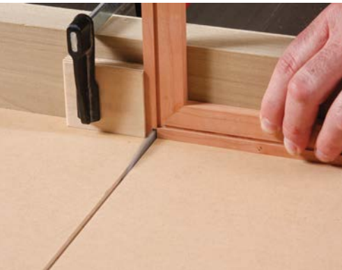
4 & 5. Notch the frames to accommodate the "legs."
