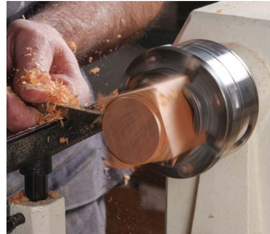
3. Turn the lid “tenon” that fits into the inside of the box.
