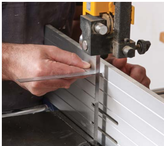
2. Check to make sure the fence face is parallel to the blade.
