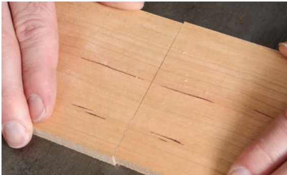
7. Adjust the sides up and down until the grain aligns along the two boards.
