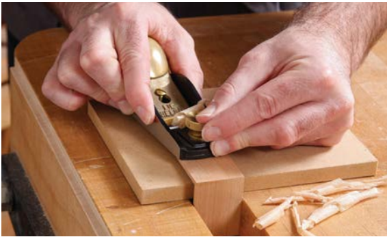
1. Plane the surface to get rid of machine marks.
