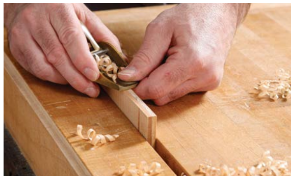
4. Trim the veneer flush to the plywood.
