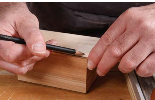
1. Measuring from inside corner to inside corner, mark the length of the side of the box.
