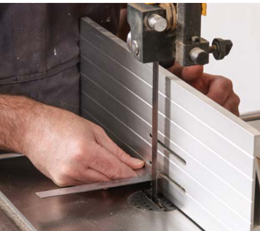
1. Set the bandsaw fence to cut the board a little thicker than the side's final thickness.
