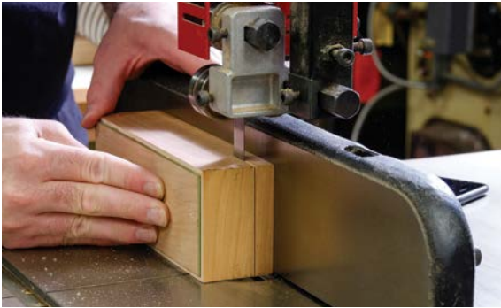
1. Cut the lid off the box at the bandsaw.
