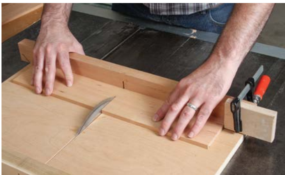
1. With a stop block clamped to the crosscut sled, cut the box sides to length.
