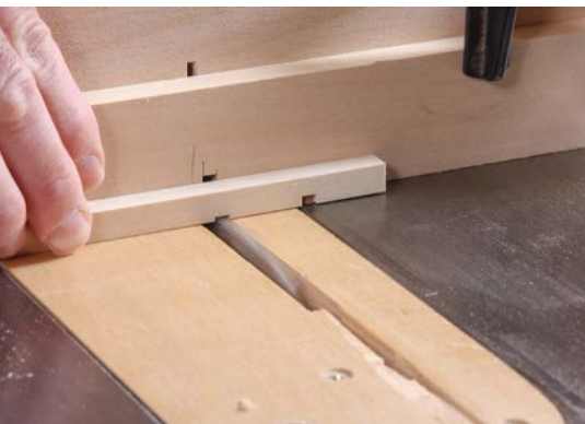
4. Place the first notch over the tab and cut the second notch.
