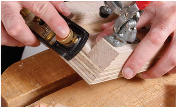
3. Using a miter shooting board, miter the sides of the liner.
