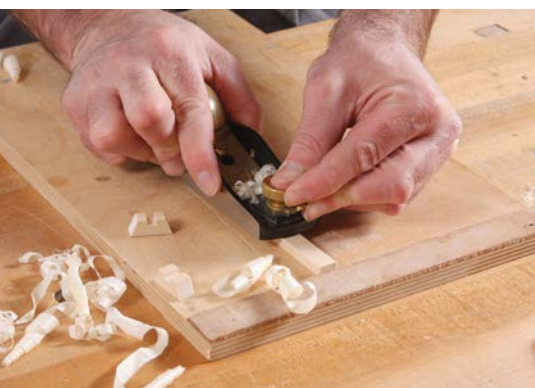
7. Plane the bar of the pull to fit the notches in the two feet.
