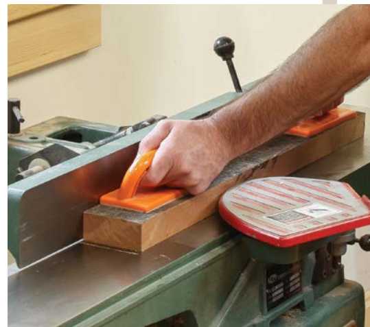
3. Joint one face of the board.
