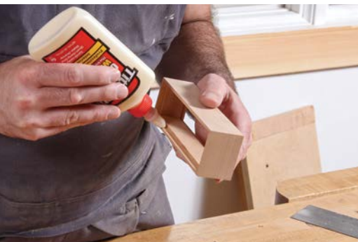
14. Apply a bead of glue to the rabbet in the box sides.
