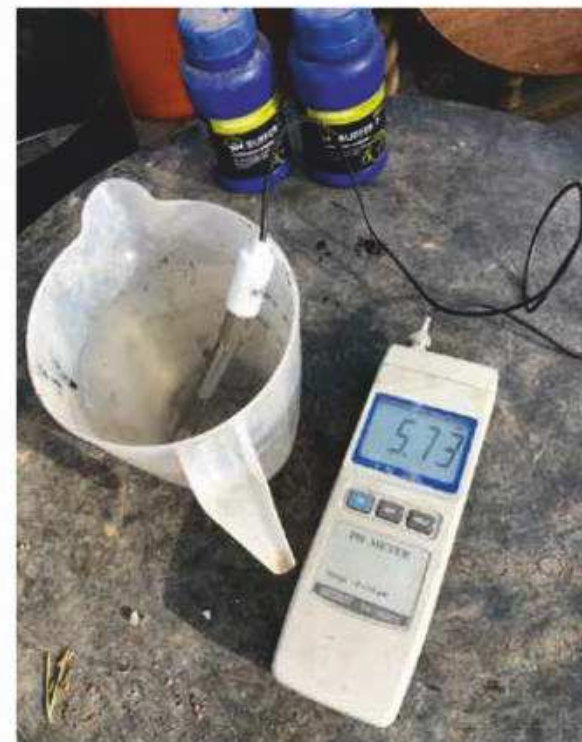
Measuring the pH of rainwater: it is acidic.
