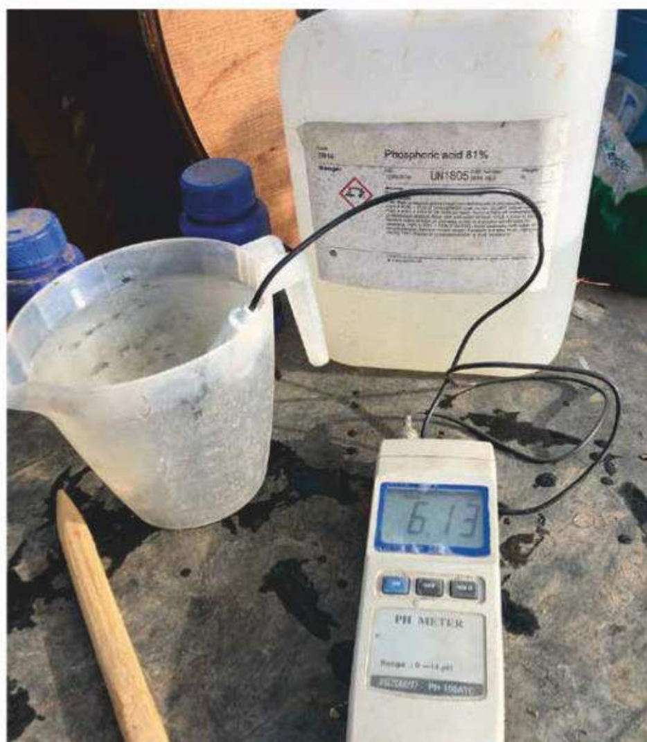
Adding phosphoric acid: the pH drops.
