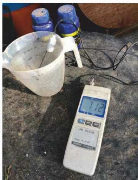
Measuring the pH of tap water: it is too alkaline.
