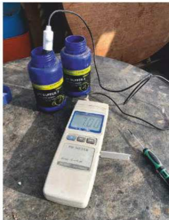
Calibrating the pH meter with a buffering solution.
