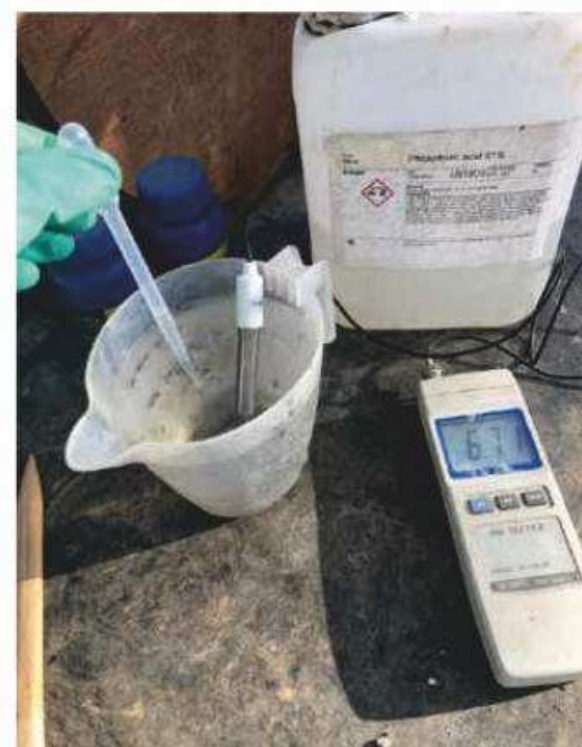
Adding phosphoric acid: the pH drops.
