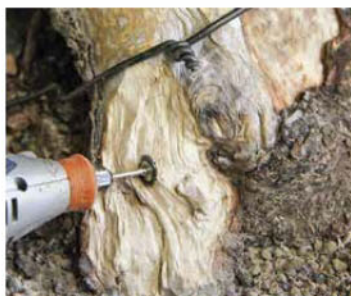
Extended polishing with a wire brush eliminates the marks of the router bit and gives an aspect of age to the work.
