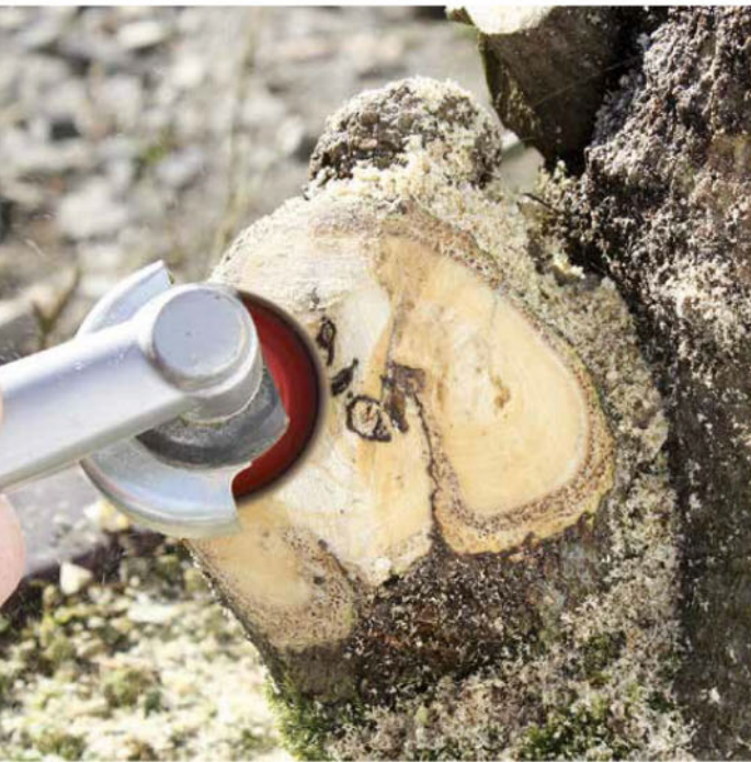
④ An angle grinder is used to pare back the corners.
