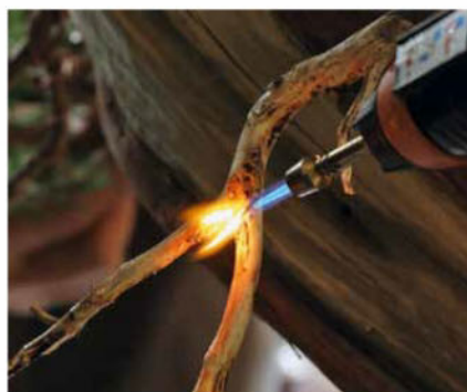
Don't hesitate to apply very strong heat to the area that is to be bent.
