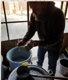
Glazing around the feet and all the other details before dipping the pot and spraying it
