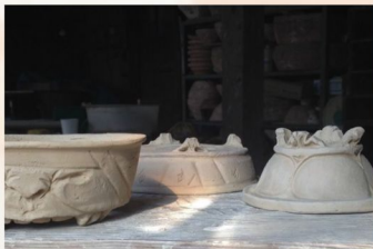
Before final polishing and glazing the pots have to be flipped while drying
