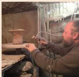
Applying glaze on one of my pots by spraying. It guarantees that you get a really even, thick glaze on the piece
