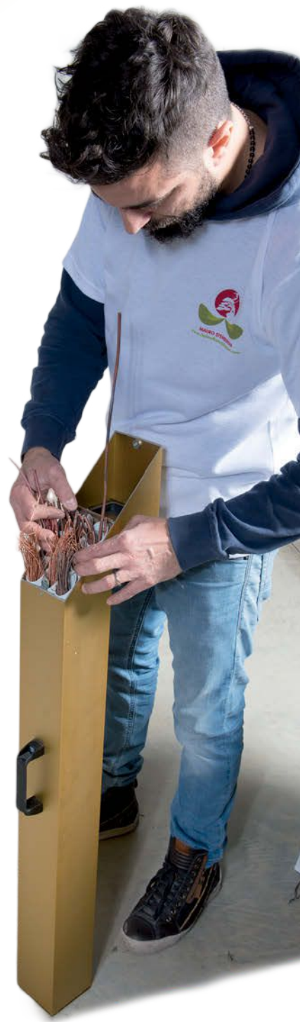
The so-called wire tower has all the sizes pre-cut in length ready for use; easier than those coils of wire which always mess up when you need a specific length. A neat design by Mauro and made by Massimo.
