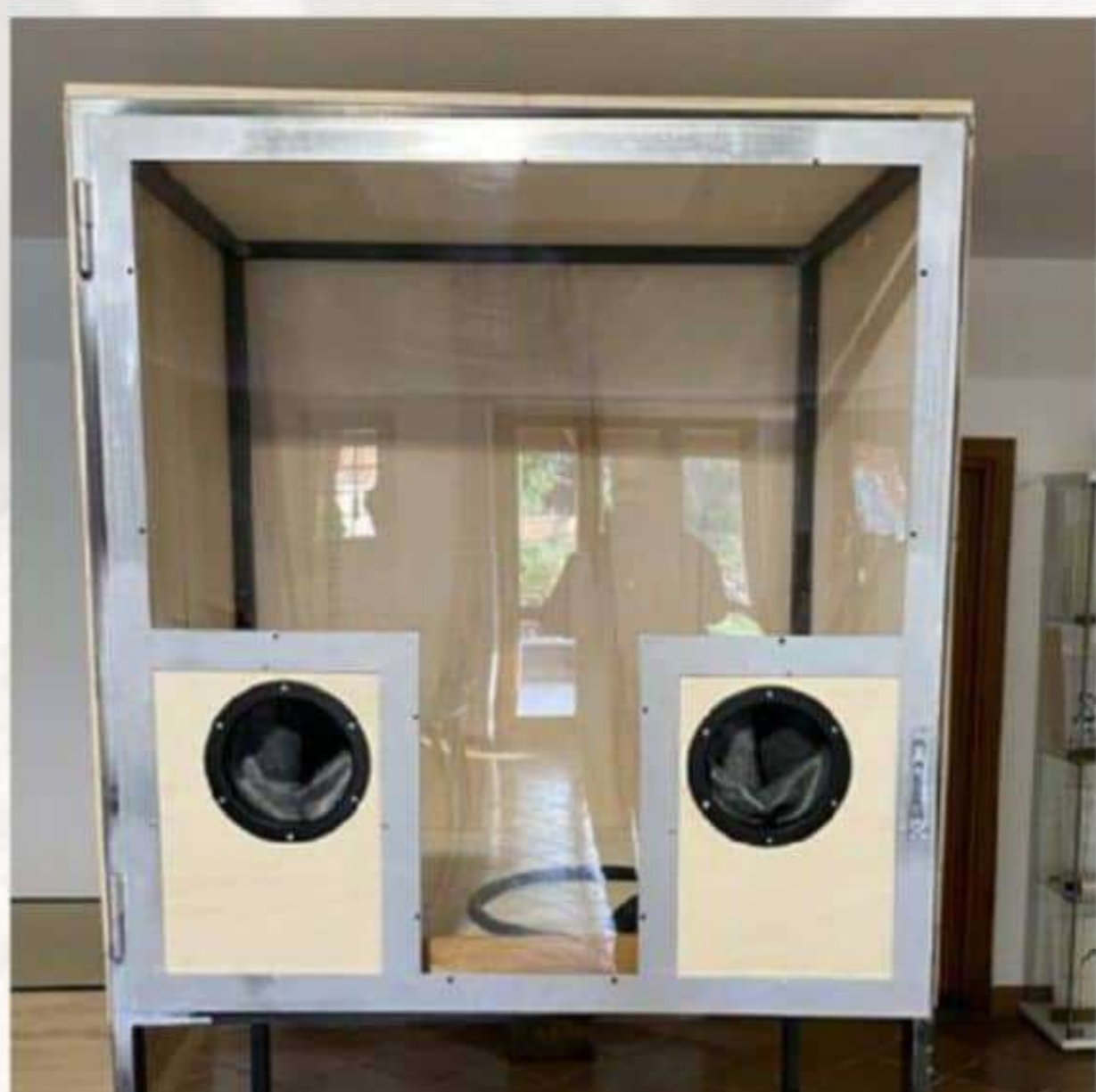
Because I teach bonsai as well, I needed to build a box for the sandblaster, suitable for the lessons I give to students, which take place in my studio
