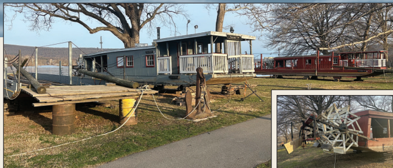
Left —Hauled out on the riverbank each fall, FALCON III , left, and ROARING BULL V , right, and their associated car barges undergo refits each spring before relaunching in May. Inset —The boats have dual stern wheels and long, horizontal sweep rudders
