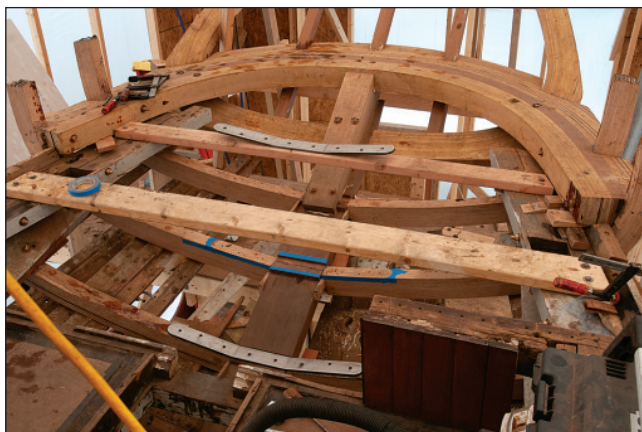
The restoration undertaken by Doug Hazlitt was thorough and dealt with areas untouched during Gannon & Benjamin's efforts, namely the stern structure and deck. Cayuga Wooden Boat Works rebuilt the transom (above left) and transom framing (above right). Some frames aft needed to be replaced before her deck was laid anew with sprung teak.
