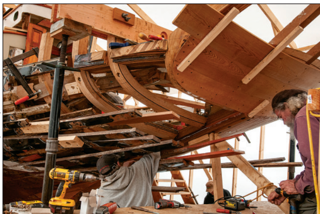
The restoration undertaken by Doug Hazlitt was thorough and dealt with areas untouched during Gannon & Benjamin's efforts, namely the stern structure and deck. Cayuga Wooden Boat Works rebuilt the transom (above left) and transom framing (above right). Some frames aft needed to be replaced before her deck was laid anew with sprung teak.
