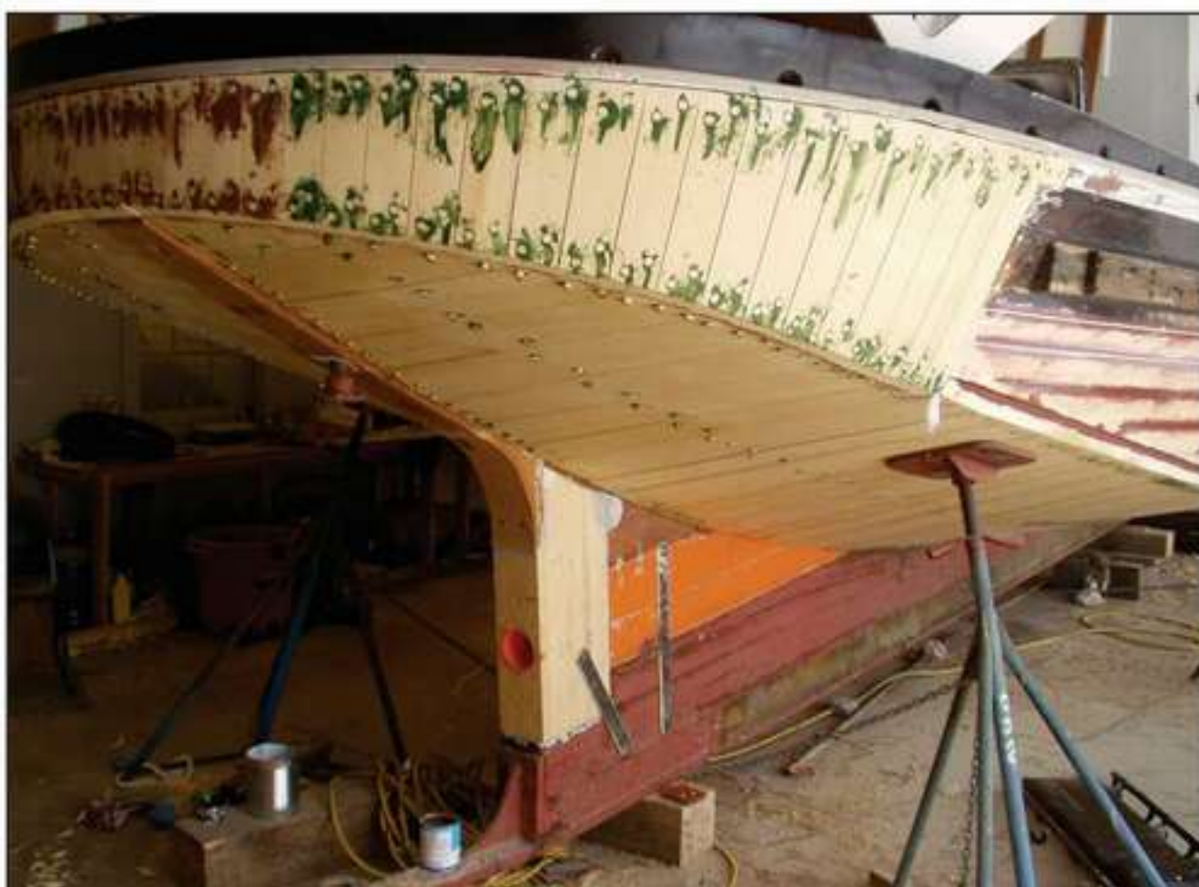
Phase One work also included replacement of the crosswise bottom planking in northern white cedar (above right), and replanking the elliptical transom (above left). The boat was caulked, painted, and put into service for the season following these projects.
