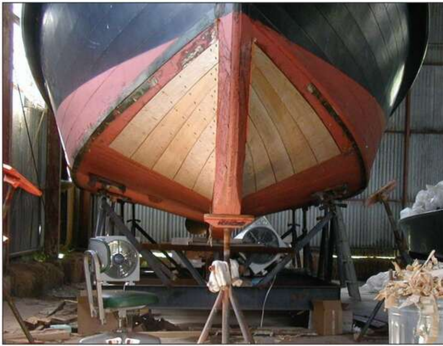
Phase Two of the project, accomplished in 2010, involved the replacement of the short fore-and aft below-waterline bow planking. In the final phase, done in 2018, the Dutch doors in the pilothouse were replaced and a portion of the afterdeck was reframed.
