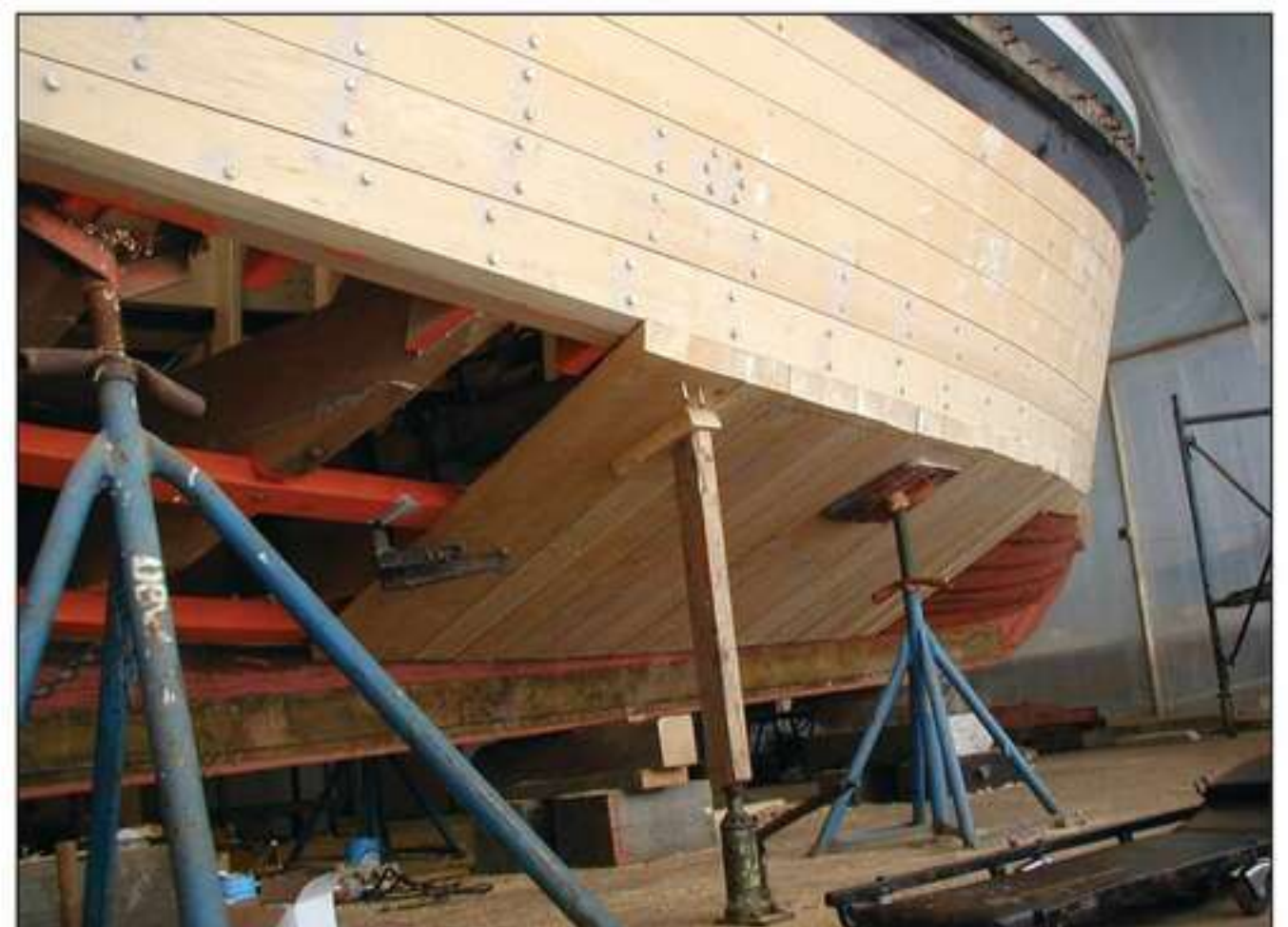
Phase One work also included replacement of the crosswise bottom planking in northern white cedar (above right), and replanking the elliptical transom (above left). The boat was caulked, painted, and put into service for the season following these projects.
