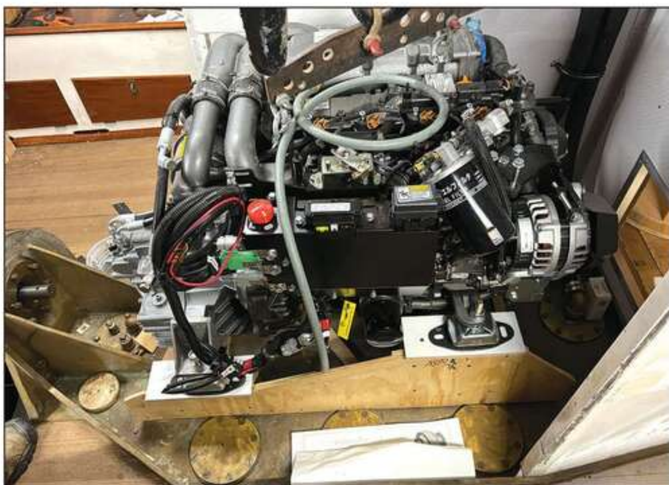
Above and right —The existing 80-hp engine was replaced with a 110-hp Yanmar. The engine connects to a chain drive that turns a long shaft that runs the length of the bilge beneath the saloon. Re-engineering of the chain drive was part of the project.
