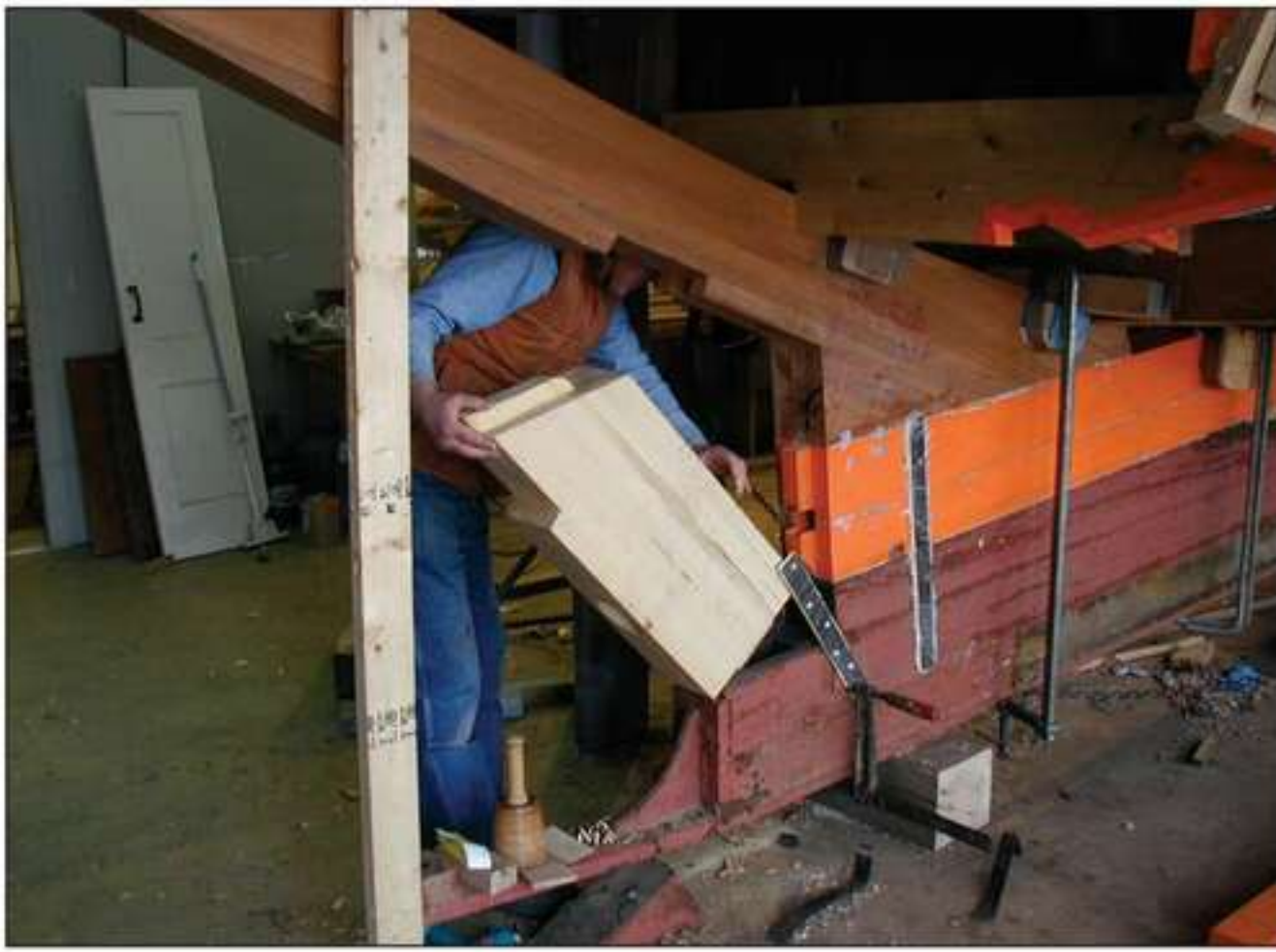
The early restoration phase also saw replacement of the boat's white-oak sternpost, as well as some topside planking in Alaska yellow cedar.
