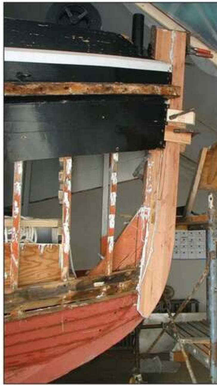
Left —The initial phase of the CHURCHILL's refit involved replacing her stern, which was laminated from mahogany reclaimed from use in vacuum molds for prototype spaceship components. Far left —Charlie Beyer replaced the CHURCHILL's forefoot before the boat's recent move to Buffalo, New York.
