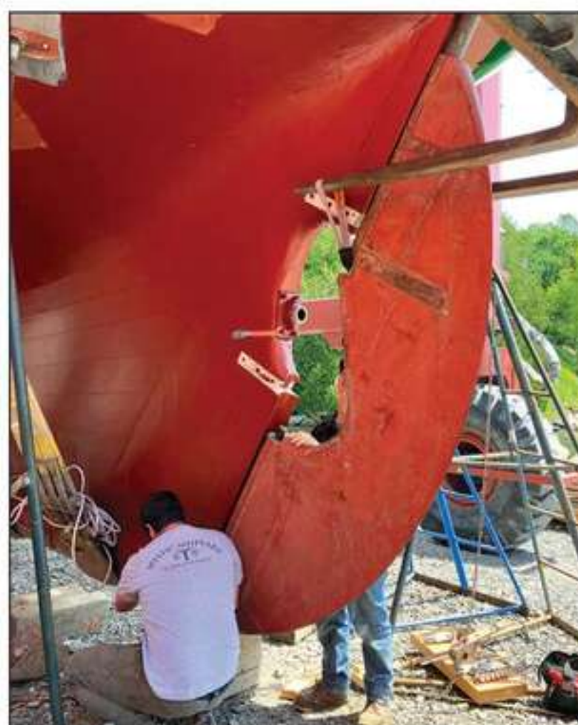
Far left and left —A stopwater aft and low in the deadwood had been pierced by a deadwood bolt, likely during construction. The inspection of this area led to replacement of all of the deadwood bolts. Dropping the rudder allowed access to this area.
