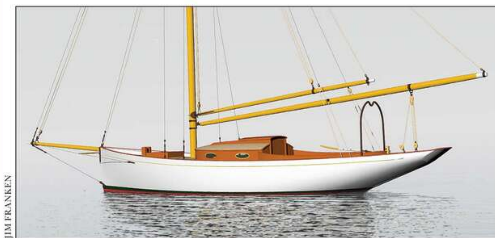
Above —This rendering shows a 26' full-keeled, plank-on-frame yacht designed by Jim Franken of Port Townsend, Washington, that is now under construction at the Northwest School of Wooden Boatbuilding.
