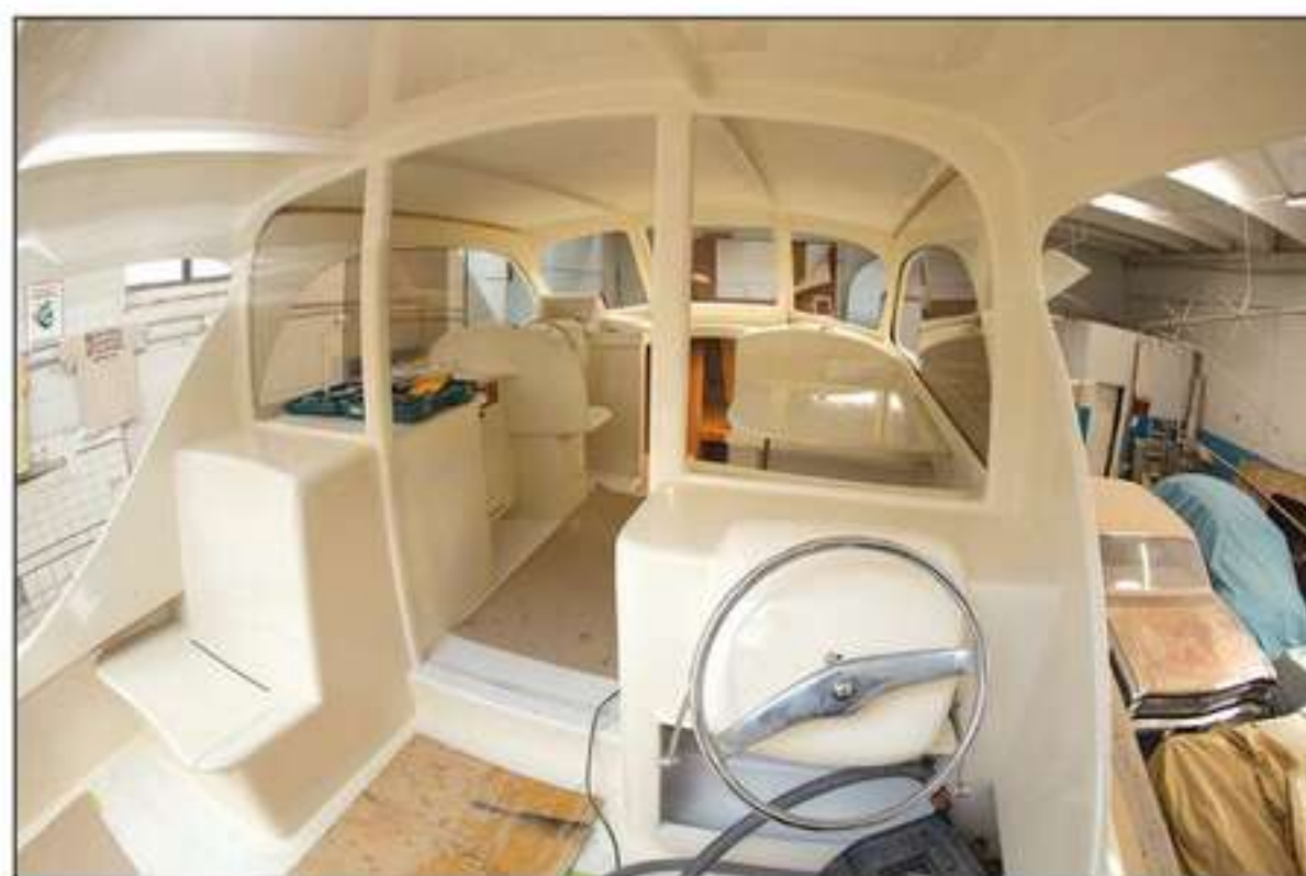
Above left —DRIFTER retains her outboard appearance and original paint scheme, and her new and lighter composite house follows the original 1954 styling. Above right —Building Corecell cabins and superstructures reduced the boats' dry weight from the original 18,000 lbs to 14,500 lbs for DRIFTER and even less, 12,500 lbs, for TIMID TUNA.
