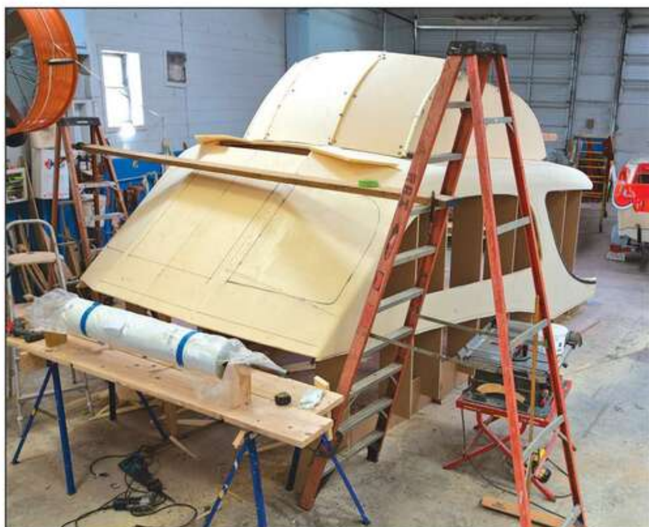
Above left —For TIMID TUNA, a new deckhouse and flying bridge assembly was fabricated of Corecell to reduce weight. Above right —The distinctive shape of a Rybovich handrail was built with foam and E-glass instead of wood.
