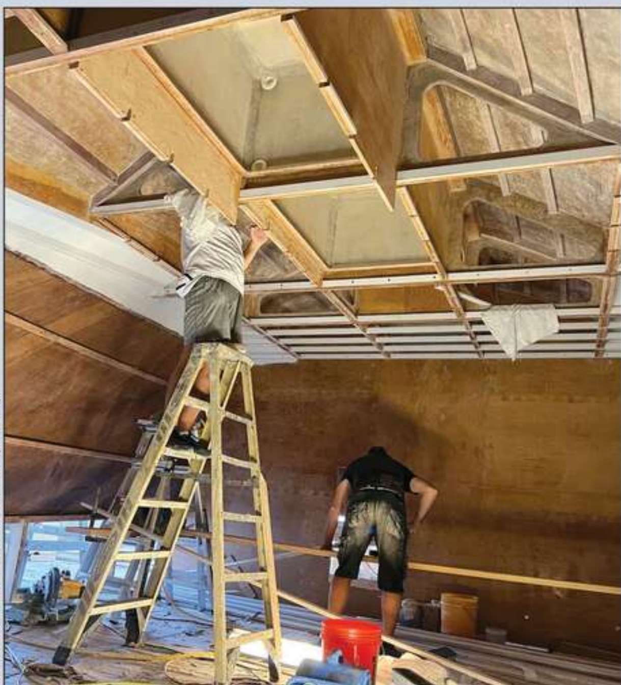
PERLAMAR , like all the other sportfishing yachts bearing the Rybovich name, was built with a cold-molded hull (left) and her cabin, too, was built of wood (right).
