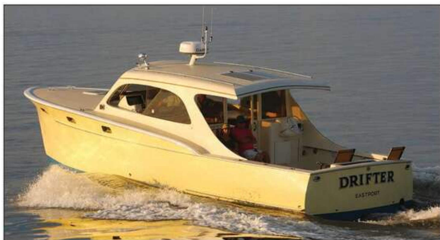
Above left —DRIFTER retains her outboard appearance and original paint scheme, and her new and lighter composite house follows the original 1954 styling. Above right —Building Corecell cabins and superstructures reduced the boats' dry weight from the original 18,000 lbs to 14,500 lbs for DRIFTER and even less, 12,500 lbs, for TIMID TUNA.
