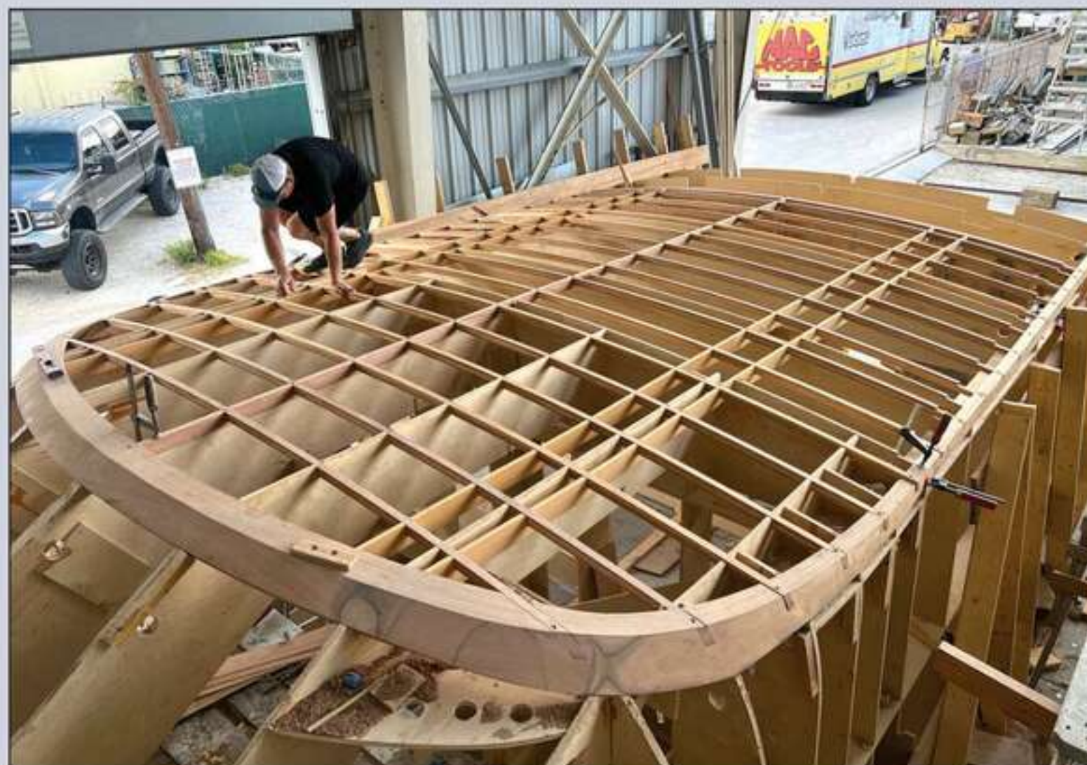
PERLAMAR , like all the other sportfishing yachts bearing the Rybovich name, was built with a cold-molded hull (left) and her cabin, too, was built of wood (right).
