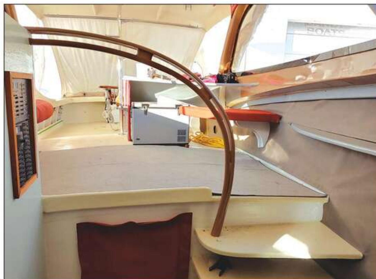
Above left —For TIMID TUNA, a new deckhouse and flying bridge assembly was fabricated of Corecell to reduce weight. Above right —The distinctive shape of a Rybovich handrail was built with foam and E-glass instead of wood.
