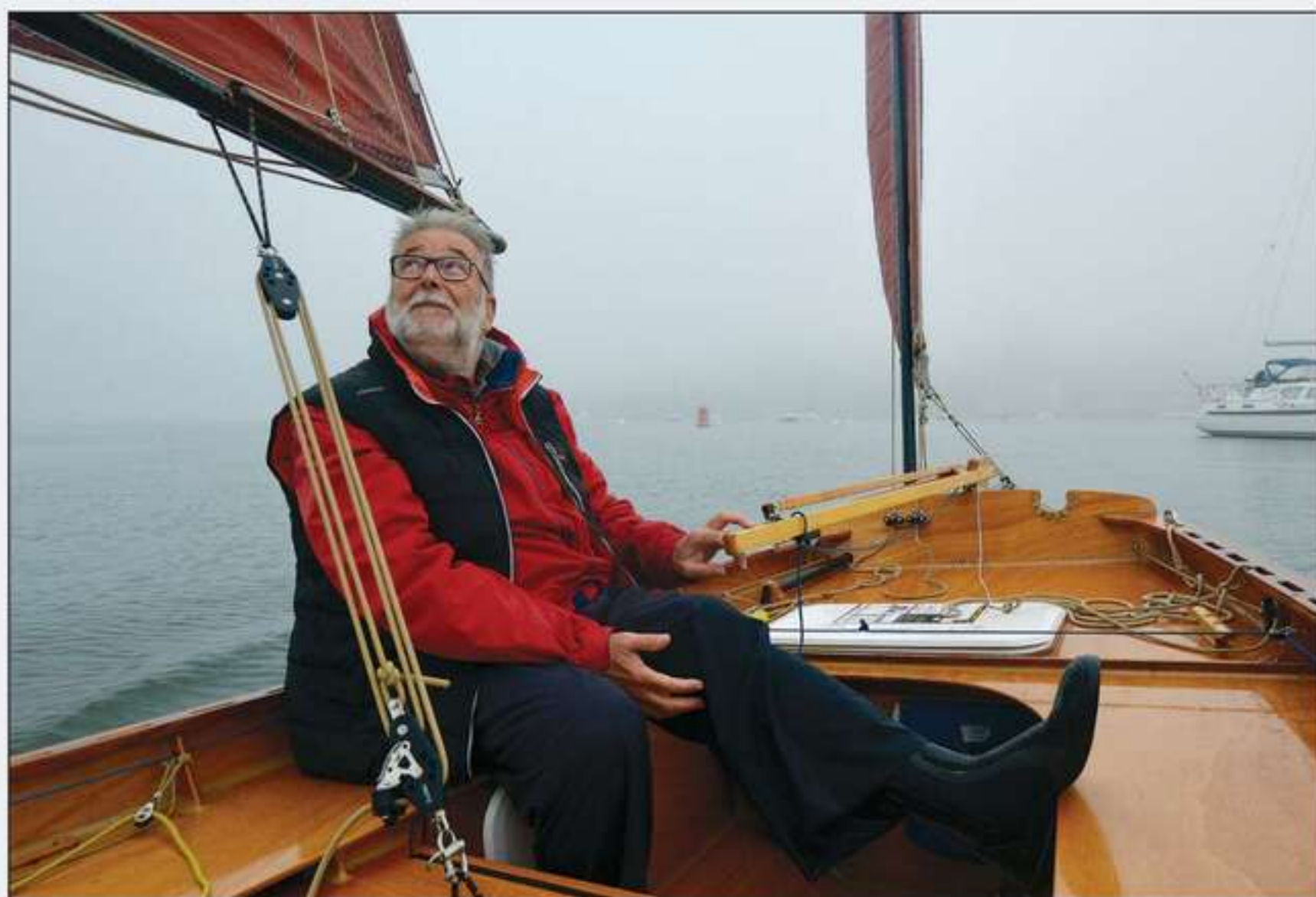
Emmanuel at the helm of the Grand Silmaril VITA BREVIS. For steering while sailing singlehanded, the helm has control lines on each side that run forward to the mast.
