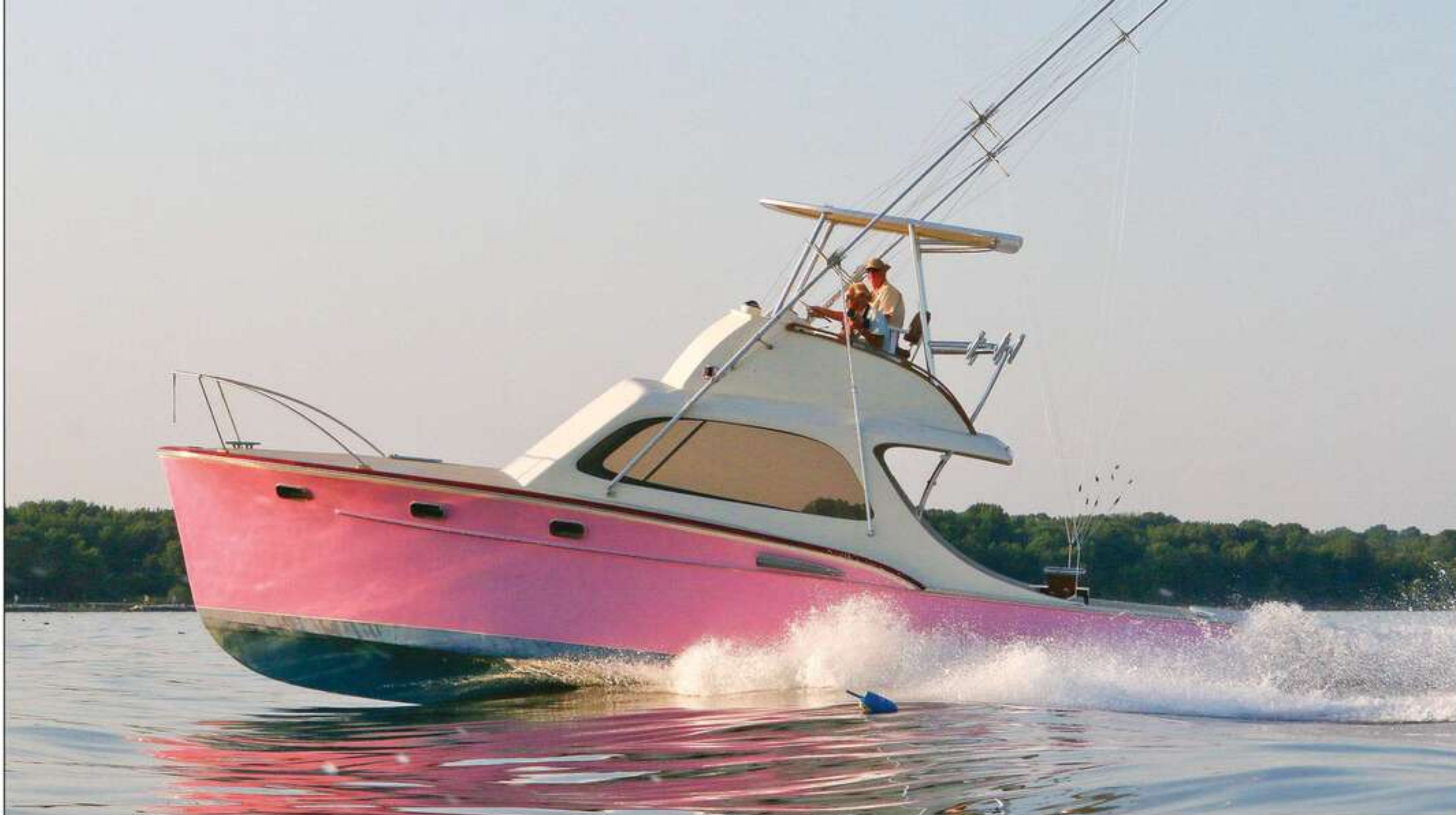
The top speed of TIMID TUNA, a 1955 36-footer, increased from 25 knots to 35 knots after Bandy reimagined her for his own use, greatly reducing the weight of her upper structure but respecting the Rybovich styling.
