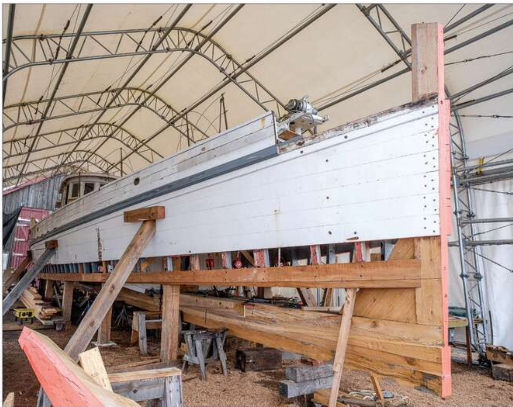
Above—The 1920 buy boat WINNIE ESTELLE is undergoing a thorough restoration at Chesapeake Bay Maritime Museum in St. Michaels, Maryland. Left—WINNIE ESTELLE was brought ashore by crane to the museum shipyard so that its 80-ton marine railway would remain open for work on other vessels.
