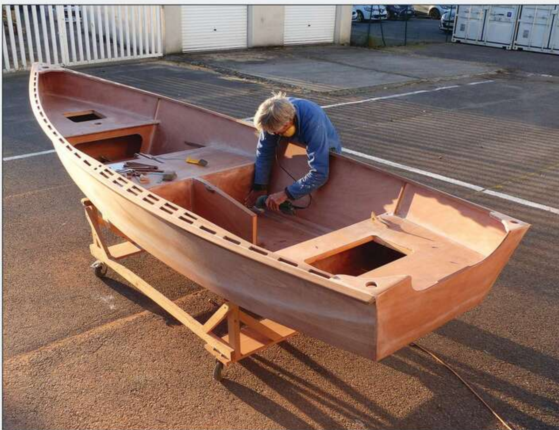
The Goat Island Skiff EPIK, under construction in November 2020, shows a modified centerboard trunk and wide inwales for hiking out.
