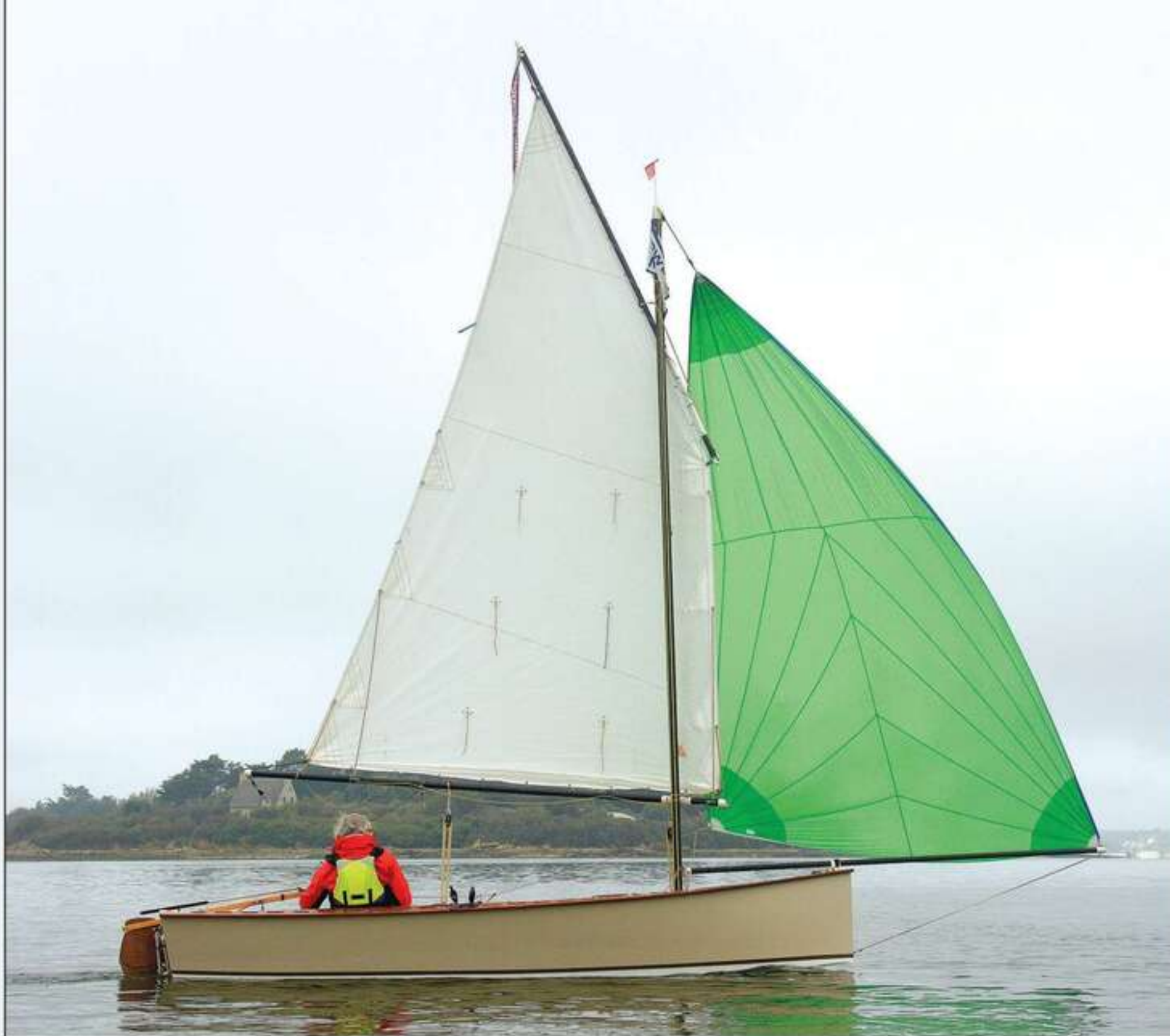
A lightweight gennaker set on a carbon-fiber bowsprit more than doubles EPIK's sail area, compared to a standard Goat Island Skiff.
