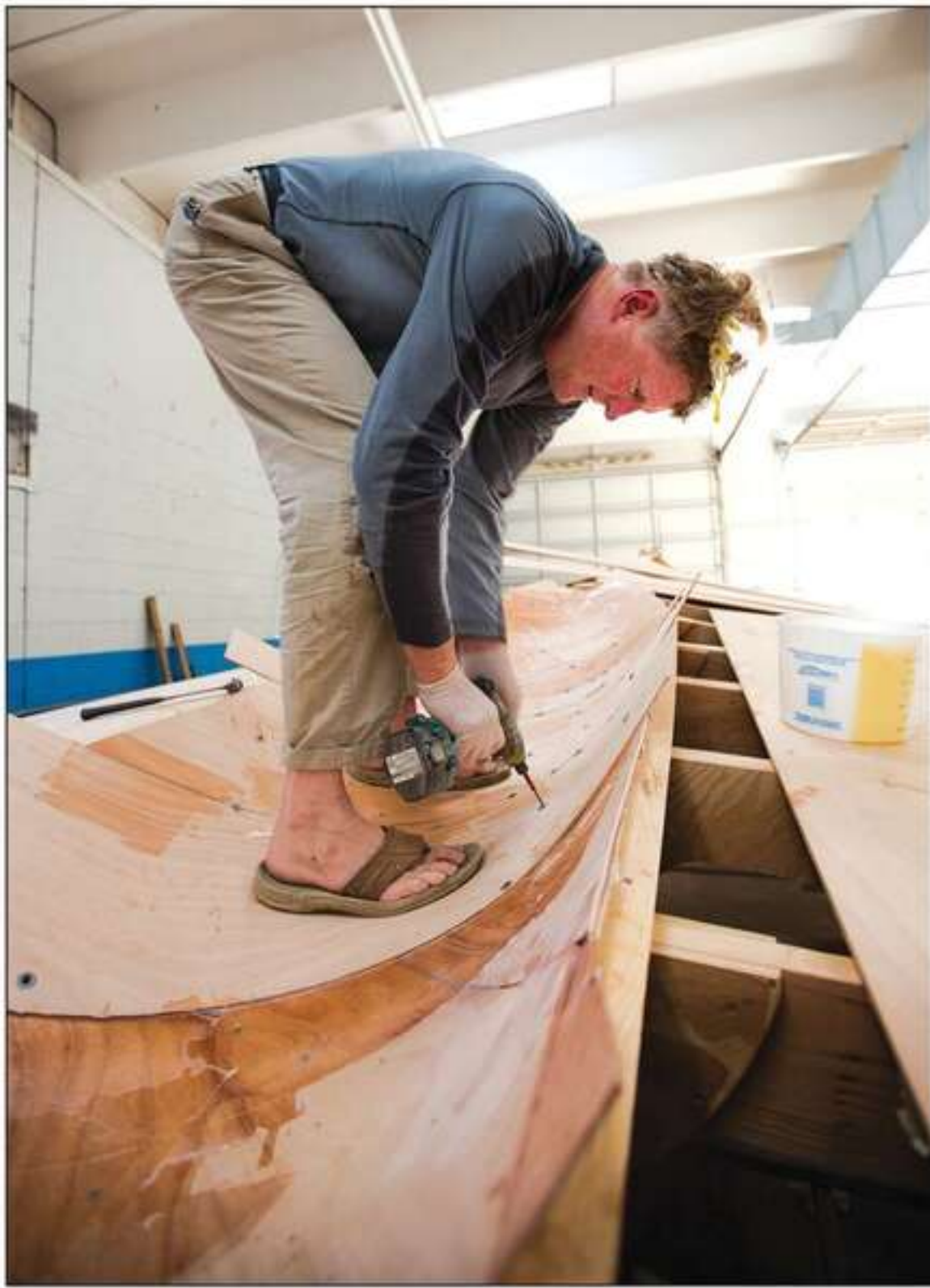
For TIMID TUNA, Bandy built a cold-molded tunnel into the hull bottom aft to accommodate the propeller-shaft's angle reduction from 12 degrees to 6 degrees.
