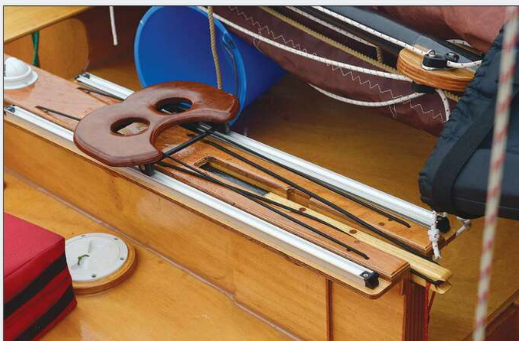
Yves has fitted a sliding seat in TRUK 2 to facilitate rowing, an important element of the raid concept.
