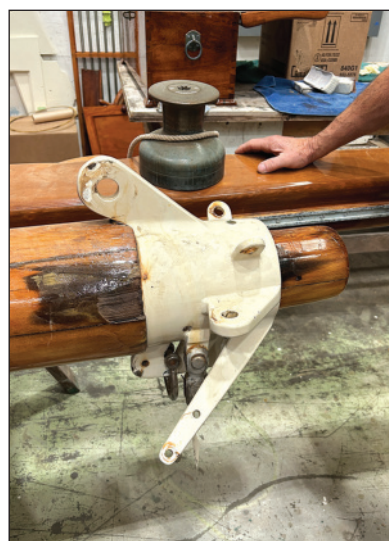
Above —The William Fife III yawl LATIFA is hauled out for "deep maintenance" in Port Townsend, Washington. Left —Much of the work will involve rerigging; wood deterioration in way of the crane iron may require a new bowsprit, and she may need a new mizzenmast as well.
