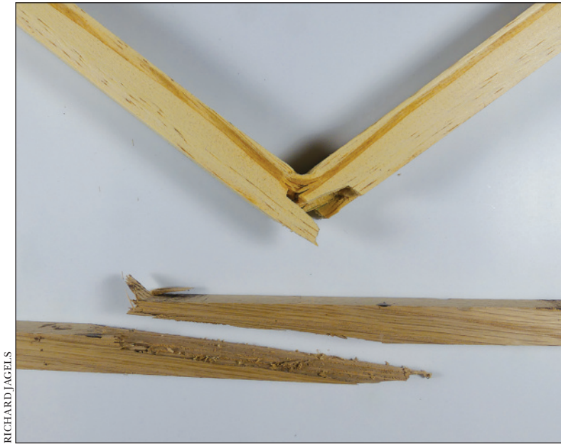
Photo 2—Using small-dimension beams cut to identical dimensions, comparative breaking strengths can be tested. The top example shows an example of a brash break, a characteristic of weak wood. The long-splinter break in the bottom example demonstrates strong wood.
