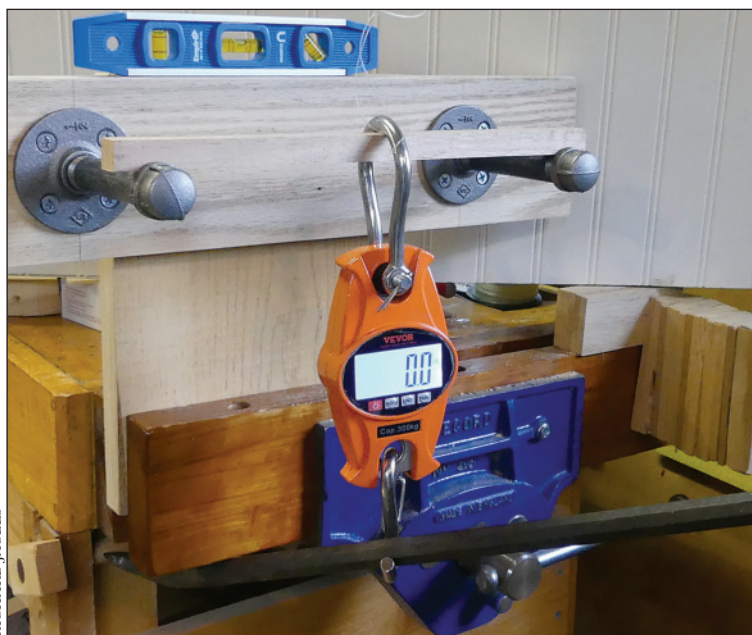
Photo 1 —A simple device for measuring comparative wood-bending strength characteristics uses a pair of 1/2" x 5" black-iron pipe nipples capped and screwed into pipe flanges mounted 12" apart on a 5/4-thick oak plank. When this assembly is clamped into a bench vise and leveled, a hanging-crane scale with 300kg (660 lbs) capacity measures the bending force to the point of fracture.
