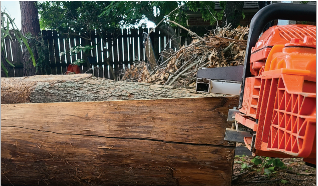
Even with one hand on the saw and the other holding the mill's grip, it can be easy to tilt the saw without noticing at the start of a cut and also at the end. The saw guide must be flat on the face of the log; here, its upward tilt to the left is clear.
