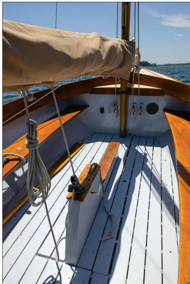
The Haven 12½'s centerboard trunk does not intrude on the cockpit. Rather, it provides a handy footrest, as well as a place to secure the mainsheet block.
