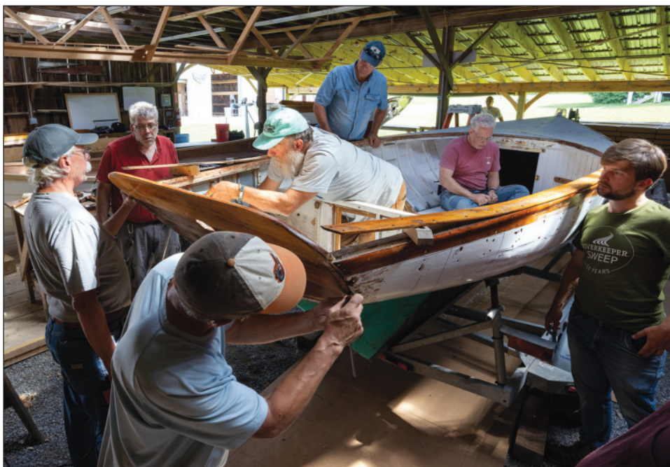
A WoodenBoat School class in July 2024, taught by Pat Mahon (standing at the transom, in the blue cap) conducted a thorough survey of Herreshoff Hull No. 2008, a Quincy Adams-built Herreshoff 12½. After this, they developed a repair plan and removed floor timbers, some planking, and the transom. Transom replacement was well underway at the end of the two-week class; the project will continue in future classes.
