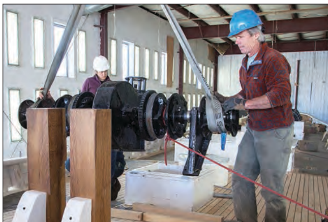
Shipwright-sailor Greg Smith guides BOWDOIN's windlass into place on the new deck.
