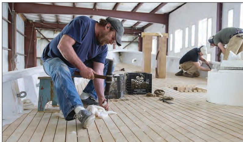
Jim Parker drives cotton into a seam in BOWDOIN's newly replanked deck. Each seam received a single strand of cotton followed by two strands of oakum. The seams were then payed with a two-part black polysulfide compound.
