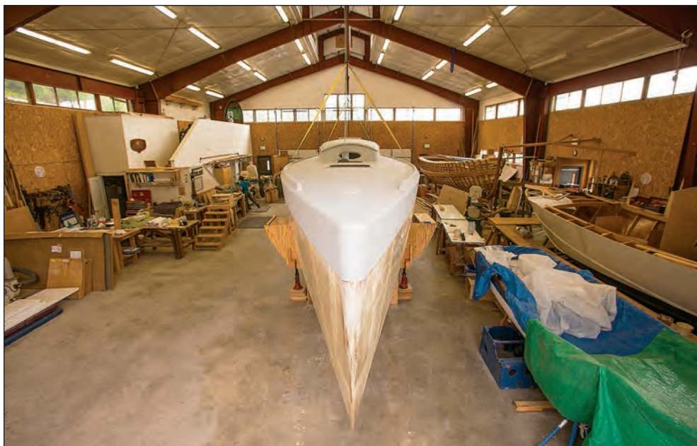
The wood-composite hull—strip-planked in 1"-thick western red cedar and sheathed with E-glass set in epoxy—was built by the Northwest School of Wooden Boatbuilding. Her beam is only 9'10" for her overall length of 62'.
