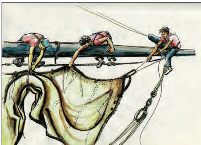
Langert's approach to rigging combines historical research with technical analysis but also incorporates an artistic sensibility. Many of his own drawings document shipboard life—such as this one, showing sailors bending a sail onto one of the yards of the French frigate L'HERMIONE.
