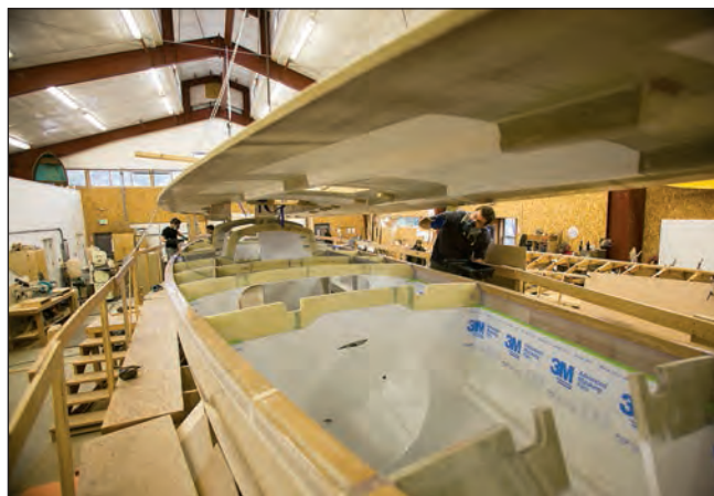
Some components of the boat were built as subassemblies, separate from the hull, most notably the one-piece deck, cockpit, and trunk cabin. Russell Brown of Port Townsend Watercraft led construction of this foam-cored composite assembly. Here, the deck unit is being installed after the hull was turned right-side up.
