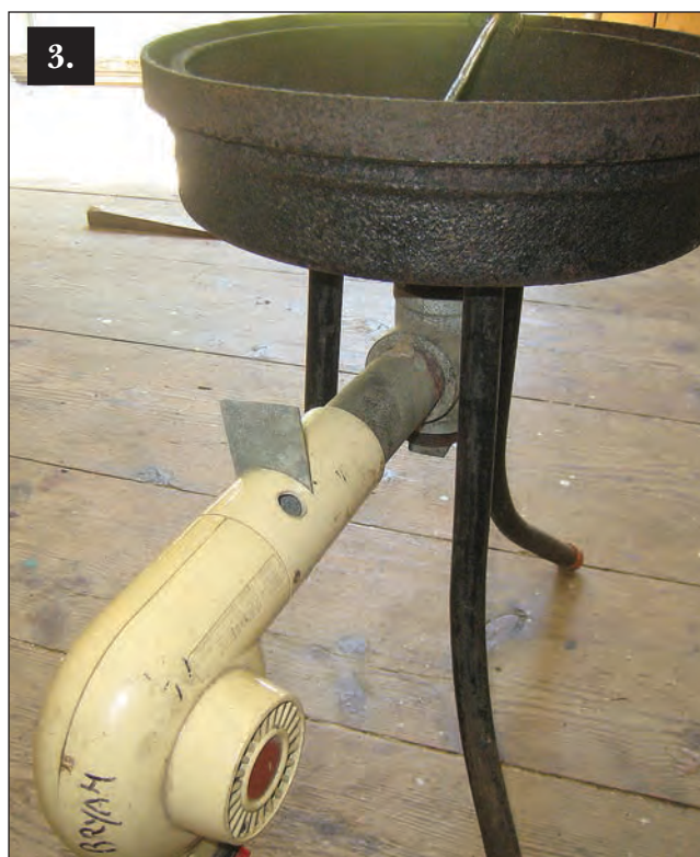
A sheet-metal damper controls the volume of air reaching the fire. It fits into a slot sawn in the neck of the hair dryer.
