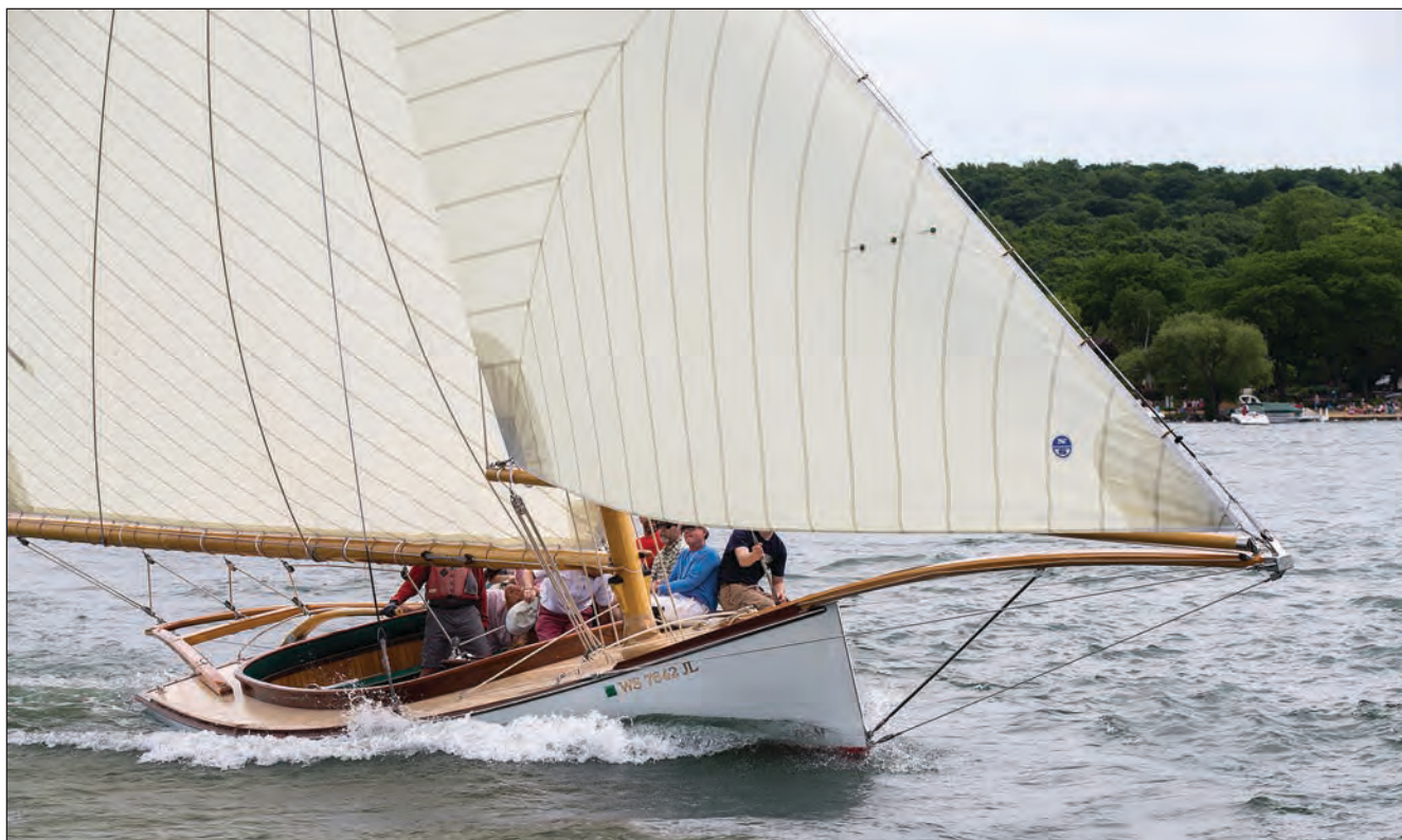
TATTLER II is more of a big dinghy than a yacht. The lengthy bowsprit and boomkin are held in place by custom fittings that allow easy removal. The deck resembles painted canvas, but is made of plywood and Dynel.
