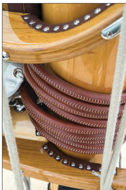
Left—The mast hoops, like the boat’s other hardware, take their aesthetic cues from older designs but are thoroughly modern; they are built of hand-leathered aluminum.
