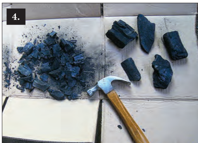
Chunks of charcoal larger than the volume of a golf ball should be broken up with a hammer before being placed in the forge.
