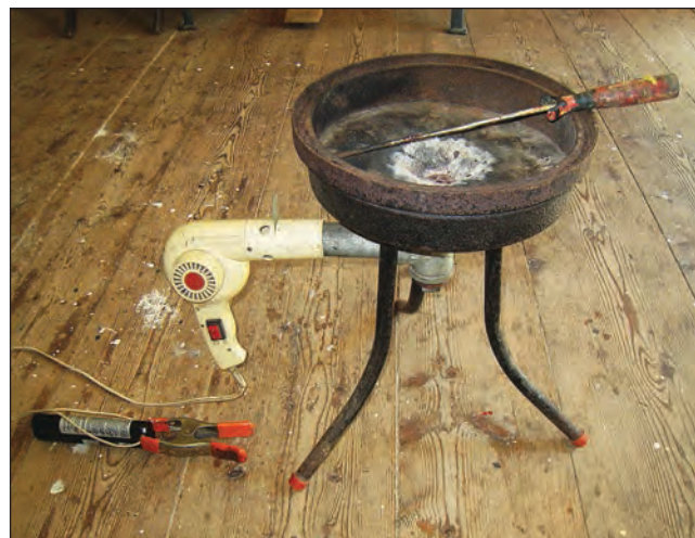
The forge completed. Note the depression in the sand-mix lining, with the fender washer at the bottom. The poker is made from a straightened-out paint roller frame.
