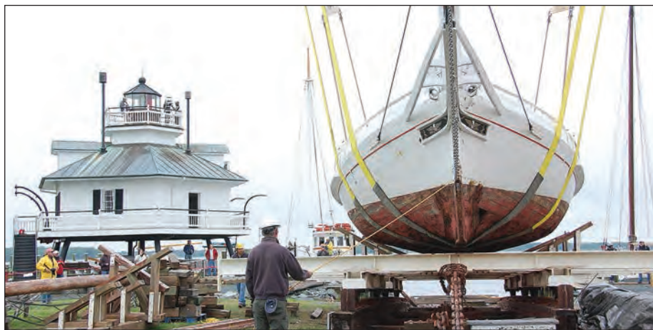
Above —The 1889 bug-eye EDNA E. LOCKWOOD has been hauled out for an extensive reconstruction at the Chesapeake Bay Maritime Museum. The last of her type, she was built in the unique Chesapeake style of log-bottomed construction. For the project, nine loblolly pine logs (inset), all about 55' long and 3' in diameter, were donated to the museum to be shaped into a new bottom.
