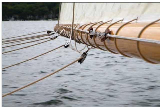
The mast and boom are both built of Sitka spruce; the mast is hollow, but the 300-lb boom is solid. The main topping lift is thus critical to safety, and is labeled in red.
