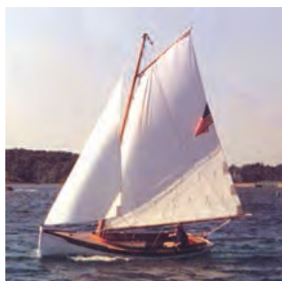
PRETTIEST BOAT IN THE Harbor—19' Buzzards Bay gaff-rigged sloop. Pete Culler design built by The Landing School. Lapstrake Honduras mahogany over oak. Sitka-spruce spars. Bronze fittings. Excellent condition. 8-hp outboard, trailer, oars, etc. $14,500. 603-431-7876.
