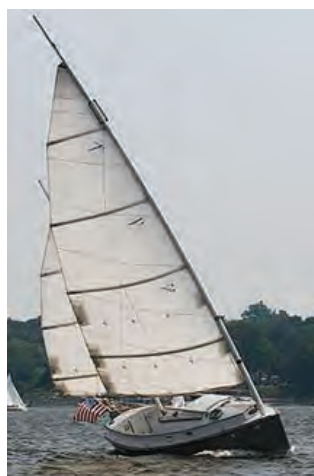
26' NORWALK ISLAND SHARPIE. Bruce Kirby design. Beam 7'11", Draft 12" board up. Fast, fun boat. Easily single-handed. Built by professional yacht rigger. Launched 1992. Bruynzeel plywood, epoxy and glass. Fiberglass masts, aluminum booms. Fresh paint and ready to go. $23,000 or best offer. dajames@optonline.net .
