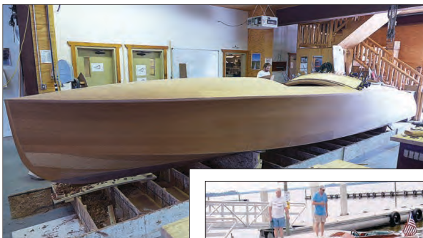
Reconstructions of the 1923 John Hacker-designed Gentleman's Runabout Gold Cup racer MISS APBA have represented a fruitful collaboration in which the GLBBS second-year students build these complex hulls that are later finished
