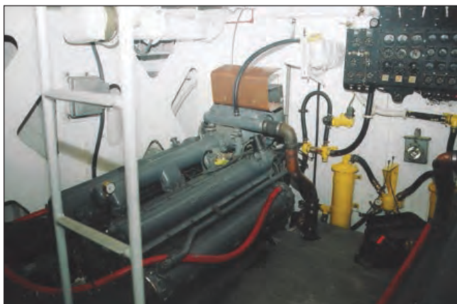
PT-658's portside Packard V-12 engine is one of three that drive the boat at speeds up to 42 knots. The engines develop 1,850 hp each.
