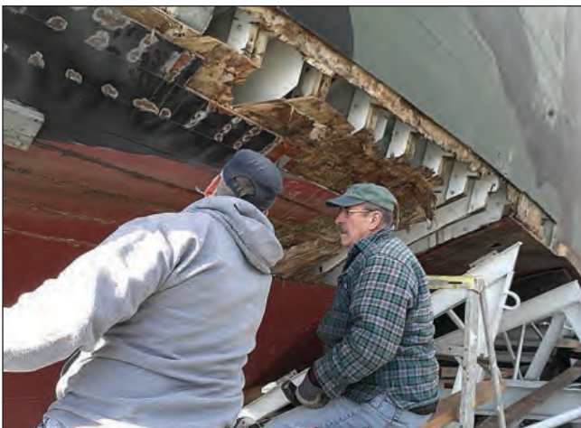
Fred Juras and Lowell Gillespie remove planking from the forward port side, winter 2012-'13.
