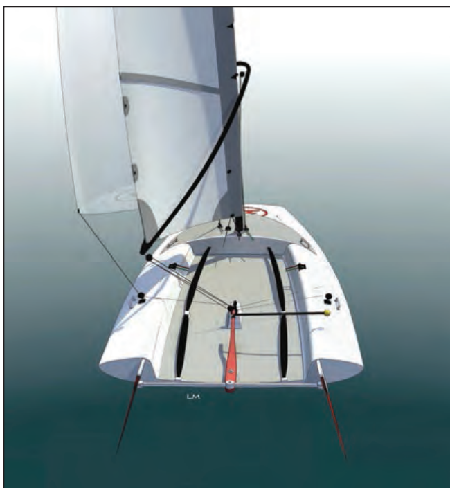
The extra-wide beam allows easy movement around the boat. There are hiking straps for a crew of three, plus handholds.
