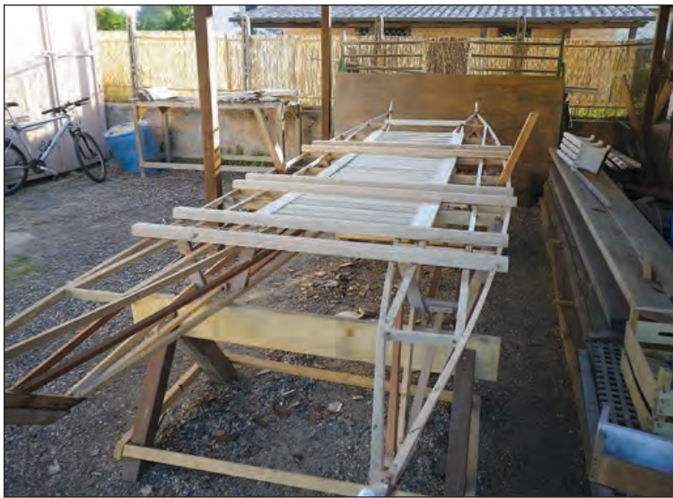
The author has recently been building pattinos to the classic form but has updated the construction by introducing stringers and plywood. Traditional pattinos were built of heavy planks joined together with galvanized iron nails.
