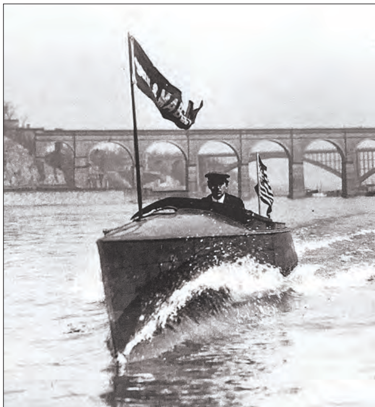
VINGT-ET-UN, later called “the first auto-boat,” is shown here in 1903 on the Harlem River, where she reportedly achieved a speed of 26 mph. The 770-lb, 21-hp boat was built for Smith & Mabley by rowing-shell builder Tom Fearon to plans by Clinton Crane.
