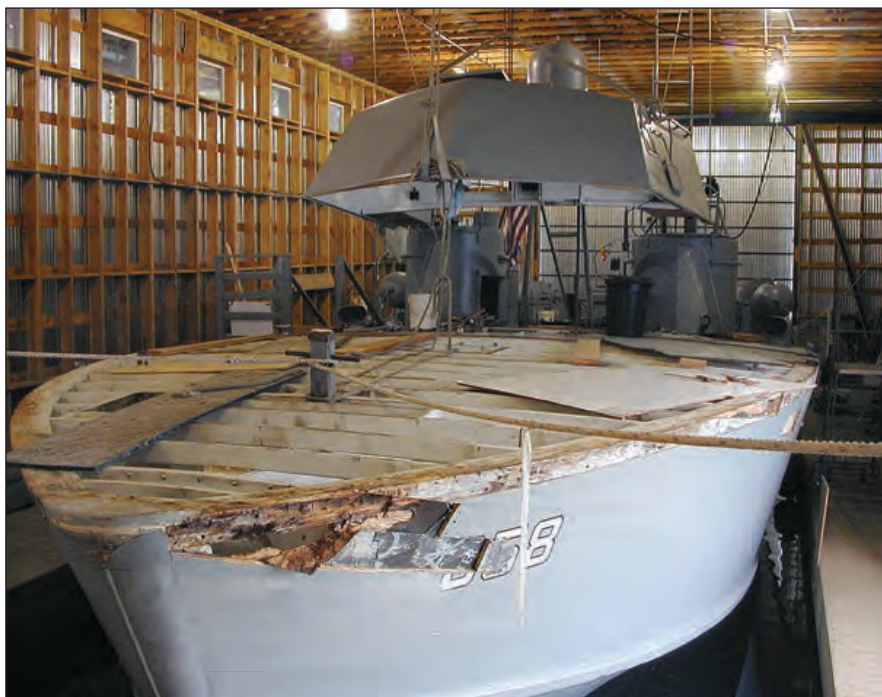
Major deck work was accomplished during the 2009-'10 phase of the restoration. Here, the chart house has been cut loose and lifted so the deteriorated decking can be stripped away.
