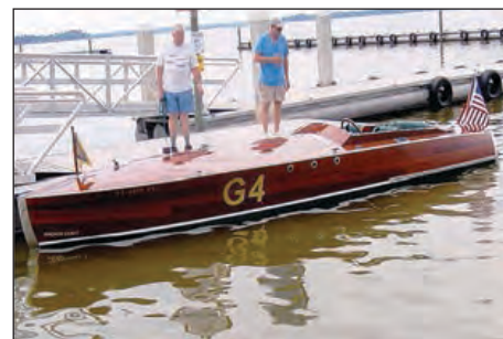
Reconstructions of the 1923 John Hacker-designed Gentleman's Runabout Gold Cup racer MISS APBA have represented a fruitful collaboration in which the GLBBS second-year students build these complex hulls that are later finished
