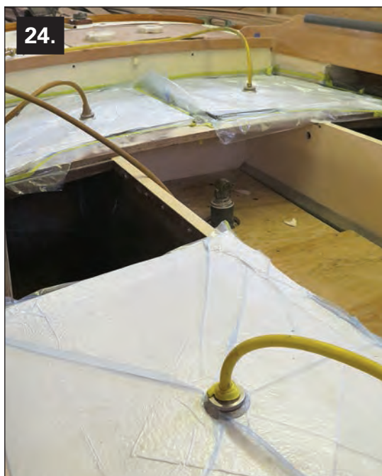
Photo 24 —After all the vacuum bags were checked and rechecked for leaks, we left the vacuum pump on overnight, pressing down with 14.7 lbs per square inch on the panels while the epoxy cured. The seat hatches and cockpit sole pieces were also vacuum-bagged, but they were done on the workbench, since they were much simpler.
