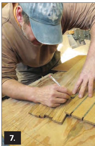
Photo 7 —After cutting and finishing the outboard side of the first panel, including its nibs, Mike cut to the line and finished off the edges with a block plane, chisel plane, and sandpaper. Then he transferred the shapes to the opposite side and made the same cuts there. Next, he traced the outboard profile of the seat panels directly onto the margin board, as shown here.
