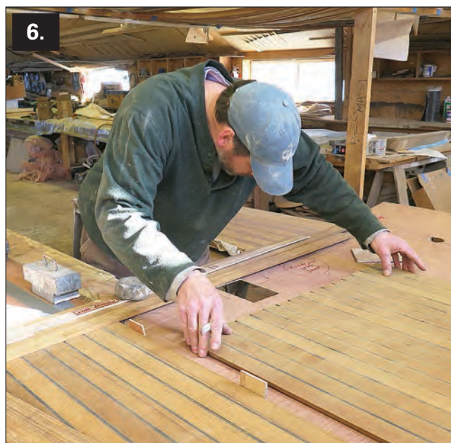
Photo 6— We planned to nib the planks into the margin boards to avoid feather edges and to give the planking a traditional look. It's the right thing to do. Here, Mike laid out the nibs to blend in well with neighboring pieces, for example the seat hatches and a wide athwartships strip that fits under the mainsheet traveler. Especially at the hatches, we didn't want to leave a small piece of a nib extending past the hatch seam where it would look out of place. The nibs also matched side-to-side, in mirror image.
