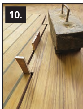
Photo 10 —Once all the cutting and finishing were done, the margin board (port side in this case) was aligned with the planking panel using spacers. Lead bricks hold things in place, ready for crossbars to be hot-glued to hold the spacing while the seam was filled with caulking, making it part of the panel.
