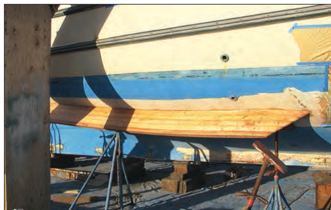
These 15'-long rolling chocks, built in Port Townsend, Washington, considerably reduce COMPANERA 's roll in beam seas—especially when used in combination with sails.
