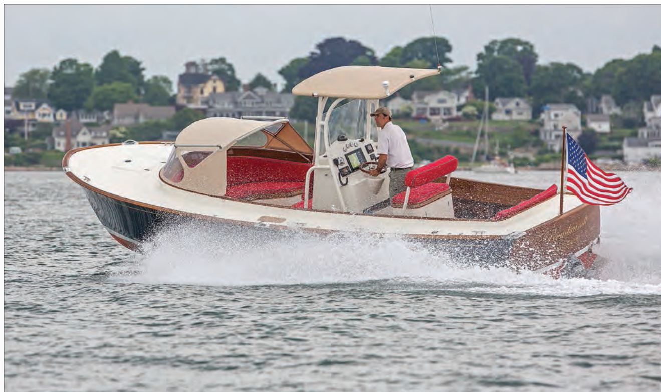
The boat is driven by a 200-hp diesel inboard motor coupled to a Volvo stern-drive.
