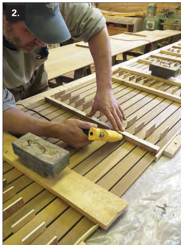
Photo 2—Using the patterns, we determined the layout of the panels and laid out the strips following the pattern—in this case, for a panel that runs the length of the cockpit and the curvature and width of the side seat, minus trim. Spacers of \frac{1}{4} " plywood guaranteed a uniform seam width. The planks were wedged together from the sides to keep the setup tight. Lead bricks held everything down. When ready, Mike hot-glued crossbars down to hold the spacing.
