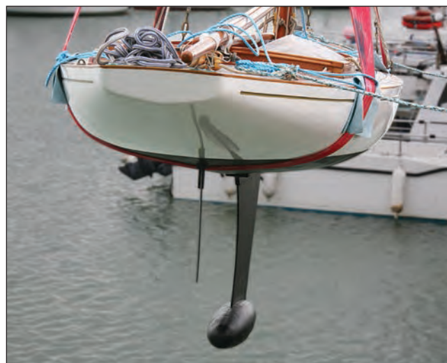
Designer Sibbick was an early advocate of fin keels with ballast bulbs, which were radical innovations in the late-19th century. The new DIAMOND has a stainless-steel fin and a 187-lb lead bulb, cast in halves and bolted to it.
