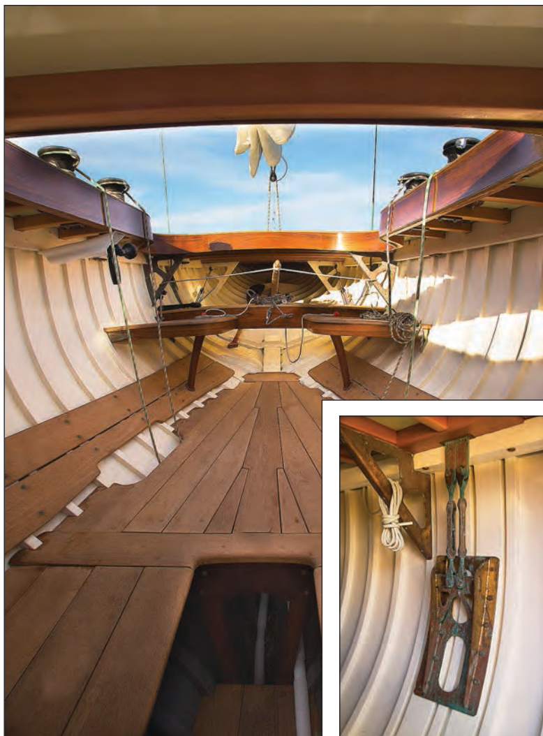
SAGA's simple layout includes separate cockpits for the helmsman and headsail trimmers, and a "trench" in the sole between them for easy passage. Inset—Custom bronze fabrications spread the chainplate load over two oversized frames, and bronze hanging knees help support the deck.
