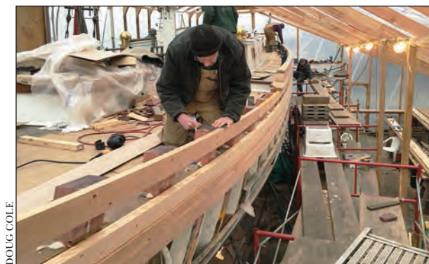
Dave Hartford works on topside replanking aboard the 1977 schooner SPIKE AFRICA at Seaview North Shipyard in Bellingham, Washington.
