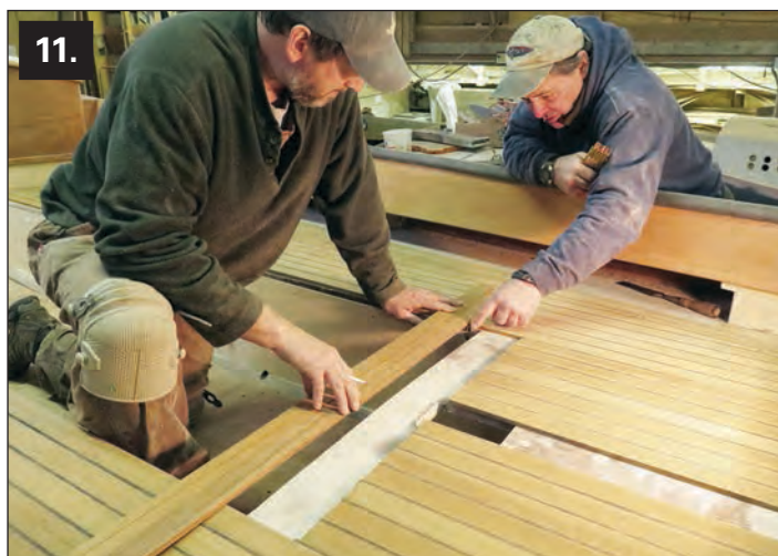
Photo 11 —During test-fitting, more decisions had to be made, almost all of them based on aesthetics. Here, Mike and I were puzzling out the fit of the plank located under the mainsheet traveler. We also talked about the type of trim to use in way of the mizzenmast, and exactly where to cut the hatches. I knew I wanted margin boards at the forward and aft ends, but I hadn't decided on their widths. It's easier to visualize these details when the panels are in place. I wanted the forward and aft margin boards to butt tight to the side margins. By this stage, the two small panels that form part of the aft seat had been edge-glued with caulking to the long side panels, making the kingplank's layout clear, and we decided the width of the aft margin board and the mizzen trim. There are several ways you could treat it. You could border the hatches out, but I'm not a big fan of bordering everything. I like a more traditional look, based on what would have been done if it were a real laid deck. It's all aesthetics, and therein lie some decisions and changes.
