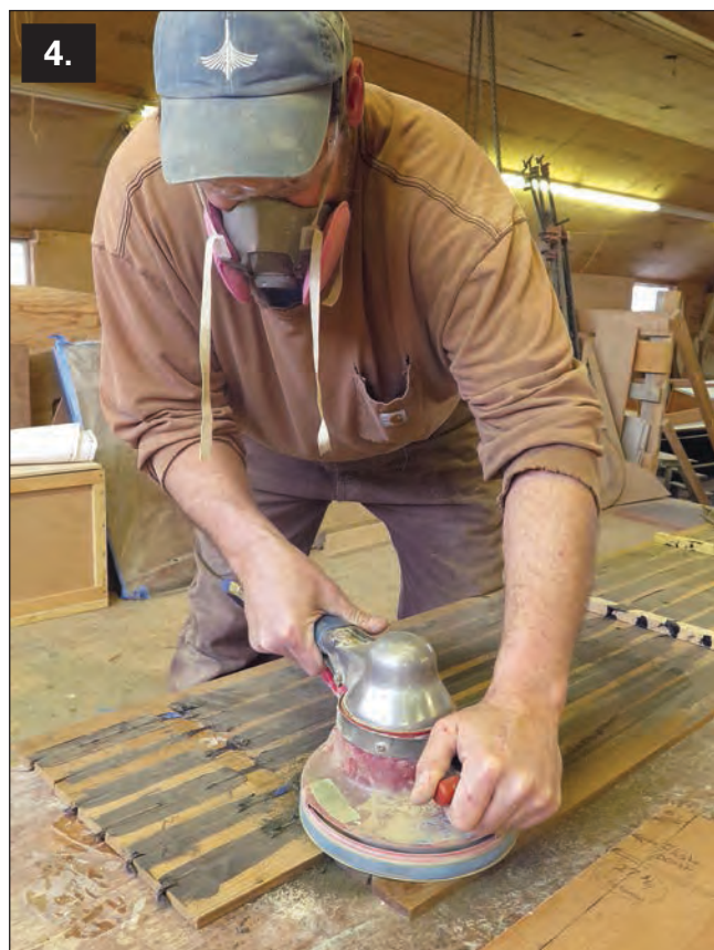
Photo 4— It takes two days for the caulking to cure fully. During that time, Mike worked on fairing mating surfaces on the boat, then came back to work on the panels again. He used a heat gun to loosen the hot glue on the crossbars and a putty knife to pry them off. An 8" sander-grinder with 60-grit discs made short work of the excess caulking, taking care to sand as little of the wood as possible.
