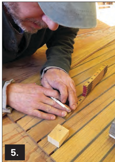
Photo 5— On the workbench, Mike lined up the new panels on the patterns. In the middle part of the aft seat, we planned one broad panel with an even number of planks, which would then be cut down the middle. Each side piece was glued to its corresponding side panel, leaving a centerline gap that would be filled by a kingplank. Careful work both in planning how pieces fit together and how margin boards, bullnose pieces, and trim would fit with the run of the strips paid off later. The curved piece visible at the lower left is a margin board laminated up of four
