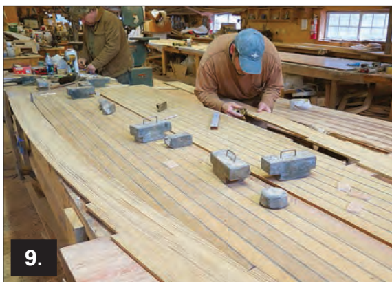
Photo 9 —We used the completed port-side panel to make a mirror-image for the starboard side. Fortunately, things on the boat were pretty close to symmetrical, and any minor errors could be taken up during the margin board's final fitting. The point of doing all this fitting so carefully on the workbench, with lead bricks holding everything in position, was to fit the margin boards so that we could glue them to the panels using the adhesive caulking. That way, we would be final-fitting only one full-length panel per side, from the cabin bulkhead to the aft bulkhead, with everything lined up, nice even caulking seams, and matching grain.
