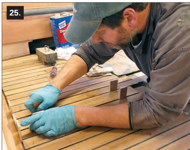
Photo 25 —After the epoxy cured, only minor cleanup was needed, after which the remaining pieces were fitted and glued in place individually. Here, the kingplank between the aft seat panels takes shape, soon to be followed by fitted pieces fitting around the box-sectioned mizzenmast, rails on the sides, a piece under the mainsheet traveler, and bullnose pieces along the edge of the cockpit seats. Caulking these final seams finished the job.
