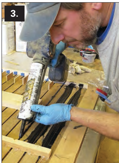
Photo 3— Using a power caulking gun, Mike filled the seams with caulk, taking out spacers as he went along and making sure to fill the space under the crossbars. The best way to fill a seam is to push the caulking gun, rather than drag it. In my experience, one advantage of caulking the seams before gluing down the strips is that the caulk adheres to the
