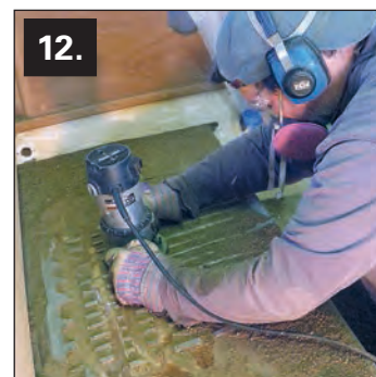
Photo 12 —While caulking seams were curing, Mike turned to surface preparation and fairing. He used a router to cut a uniform depth in a checkerboard pattern, then followed up with a broad chisel to break out the pieces. Even though there was a little variation in the thickness of the old veneer, we could mill off an even amount. After that came sanding. That's boatbuilding—90 percent of it is sanding. And if I'm wrong about 90 percent, then it might be 95.
