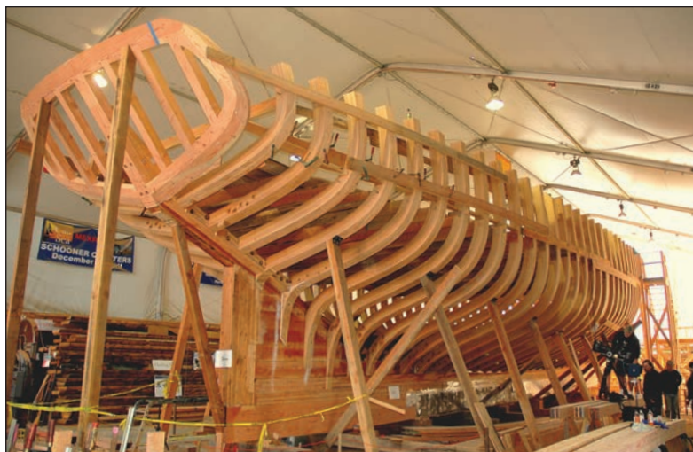
The hull framing for the brigantine MATTHEW TURNER, 100' on deck, was completed by December 2014, when a full view of her shape was possible before the planking scaffolding encased her. The sail-training vessel is based on a 19th-century ship built by her namesake, a noted San Francisco Bay Area shipbuilder.
