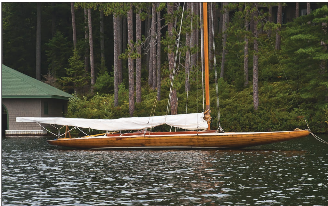
Excessive rigging tension contributes to sheer deformation in way of the shrouds and running backstays—but it plays no role in “hogging,” or drooping of the ends. Hogging is painfully evident in this archival photograph of a fine-ended and lightly built Idem-class sloop, one of a fleet at St. Regis Lake in New York’s Adirondack Mountains. Dating to 1899, many of the boats have been through thorough restorations.
