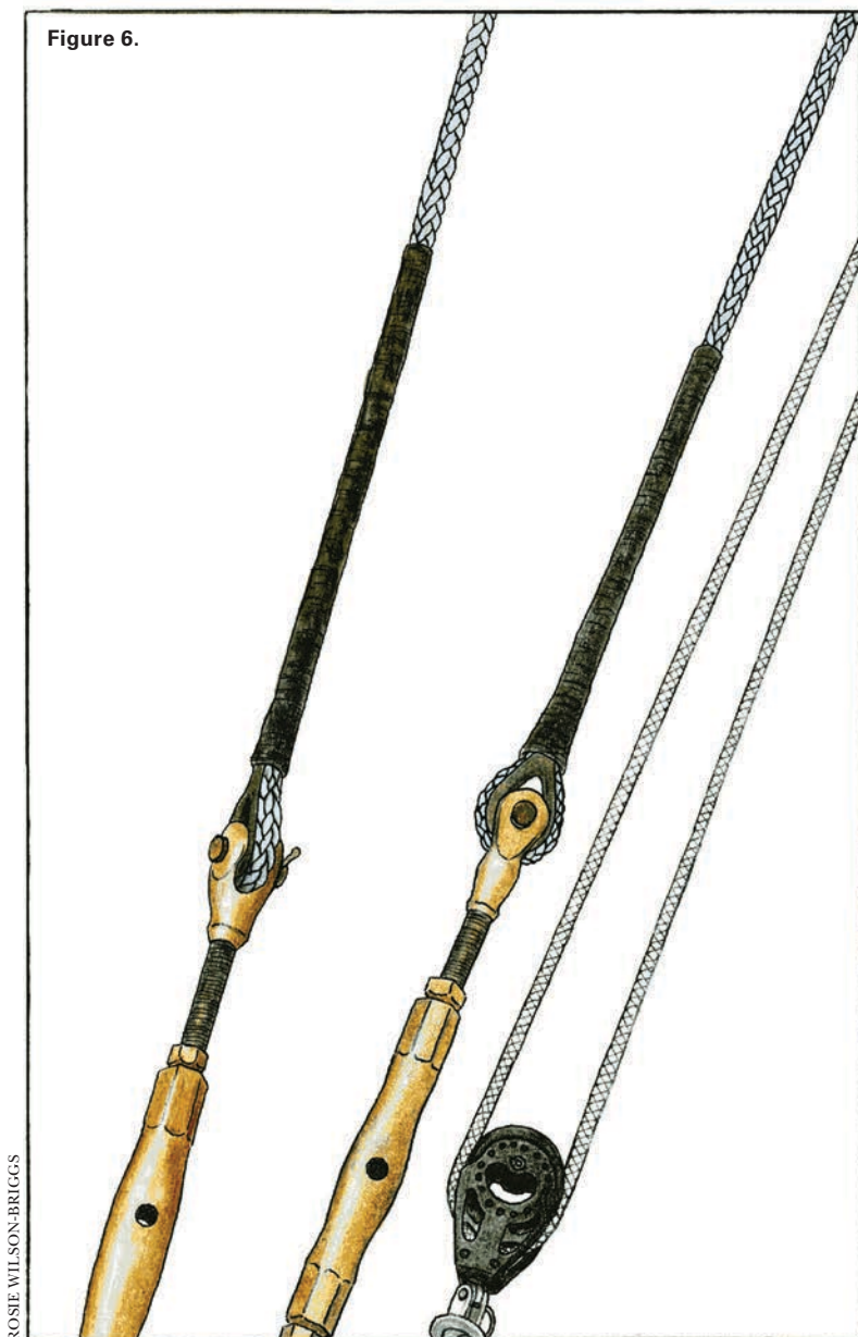
Figure 6—Modern synthetic lines such as Spectra and Dyneema are sound choices for the standing rigging of wooden boats, since they have exceptionally low stretch and great strength in use, and impose lower loads than steel standing rigging over time when the boat is at rest.
