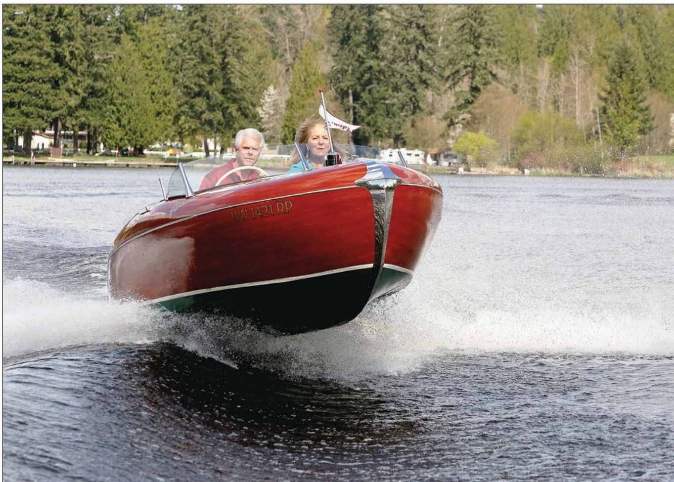
NO KA 'OI is powered by a four-cylinder, 140-hp MerCruiser—a lighter and more powerful engine than the original six-cylinder Graymarine.
