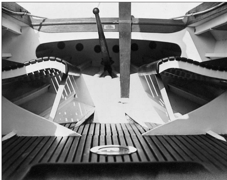
This view of the YANKEE's cockpit shows what her web-frame construction looked like.
