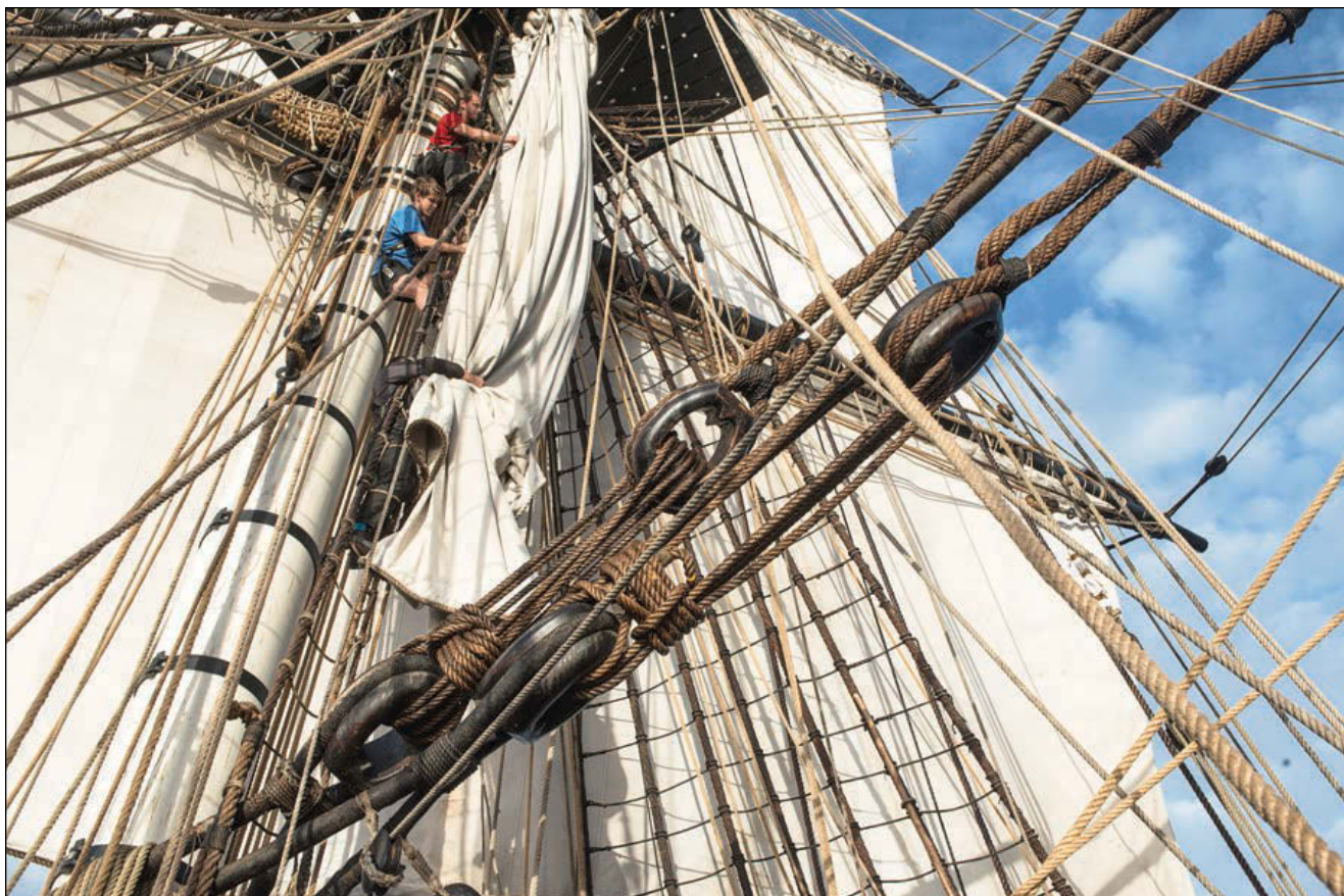
L'HERMIONE's three masts are supported by almost 5 miles of hemp standing rigging, and its natural linen sails are controlled by more than 10 miles of manila running rigging. Rigging practices accurate to the late 18th century were used throughout.
