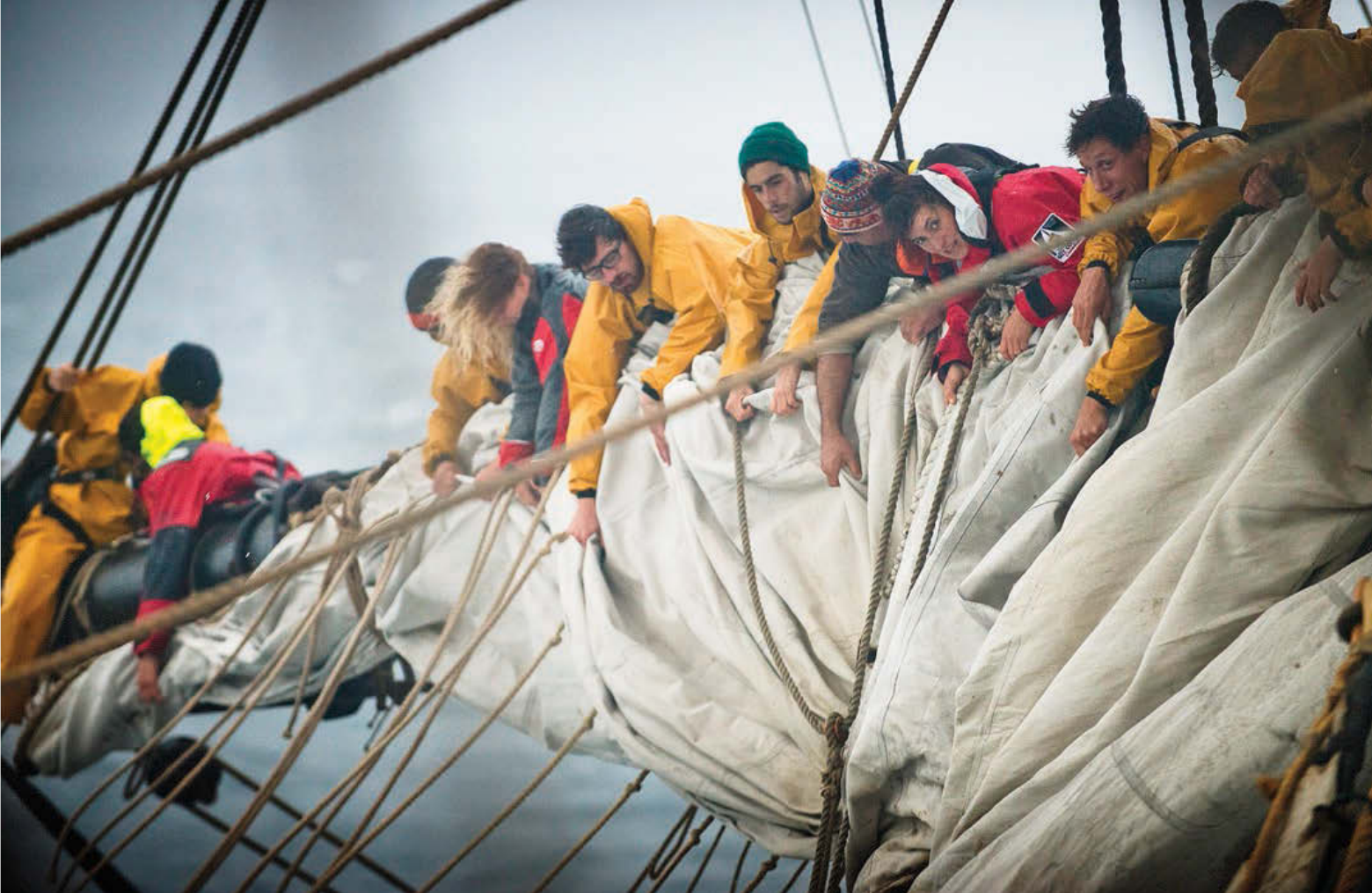
The mainsail weighs 1,600 lbs dry and takes 30 crew more than half an hour to furl. The author had direct experience of working aloft, including furling sail, during the ship's Bordeaux-to-Brest passage in 2014.
