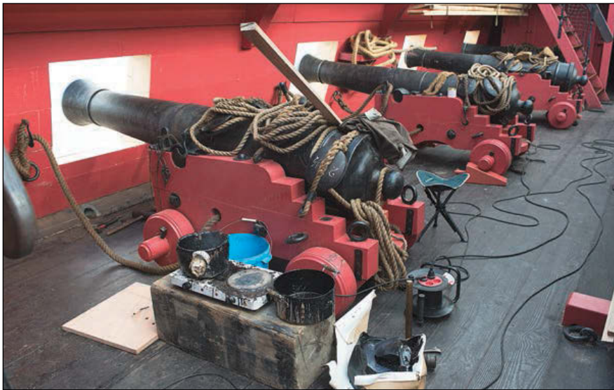
Above left —Thirty-one cast-iron cannons were fabricated in forges in Angoulême, where foundries made cannons in earlier centuries for the Rochefort dockyards. The ship's 32nd cannon is an original, recovered from the wreck site of the 1779 L'HERMIONE. Above right —Arélien Velot and his crew made most of the ship's ironwork at a quayside blacksmith shop in Rochefort, which became a popular public exhibition of their skill.
