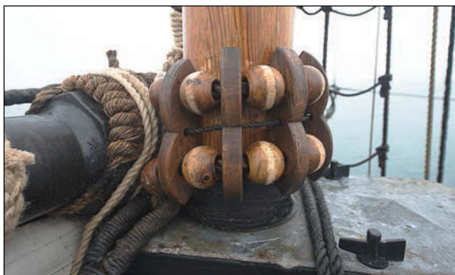
Parrels for a topmast yardarm sling are but one example of wooden components used throughout the frigate's rigging. Replacement pieces are made by hand on board as needed and installed while underway.
