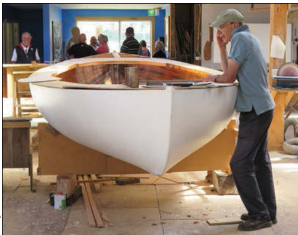
A 23' double-ender, planked in recycled King Billy pine, is under construction by Andy Gamlin in the former Wooden Boat Centre Tasmania, which he ran and recently sold to Franklin Working Waterfront Association. The sliding-gunter sloop, water-ballasted, is of Gamlin's own design.
