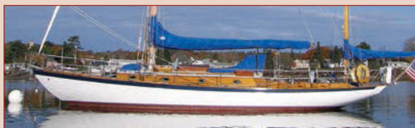
MALAY: 39'-10" Concordia Yawl, No. 77, built 1960 by A & R. Laminated white oak frames; African mahogany planking. 1982 Yanmar 3 cyl. diesel. A widely known Concordia. Extensively equipped and well maintained.
