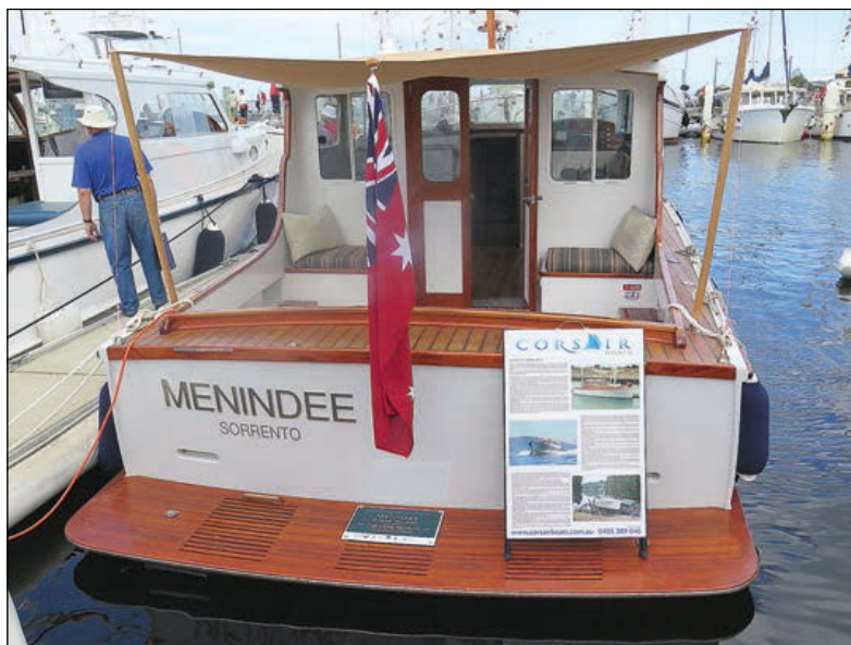
Taking inspiration from Maine lobsterboats, Mark Abbott of Corsair Boats recast the type as a cruising powerboat for Australian waters. MENINDEE , 37'6" LOA with a sheathed strip-planked hull, is the smaller of two such designs the company is building.
