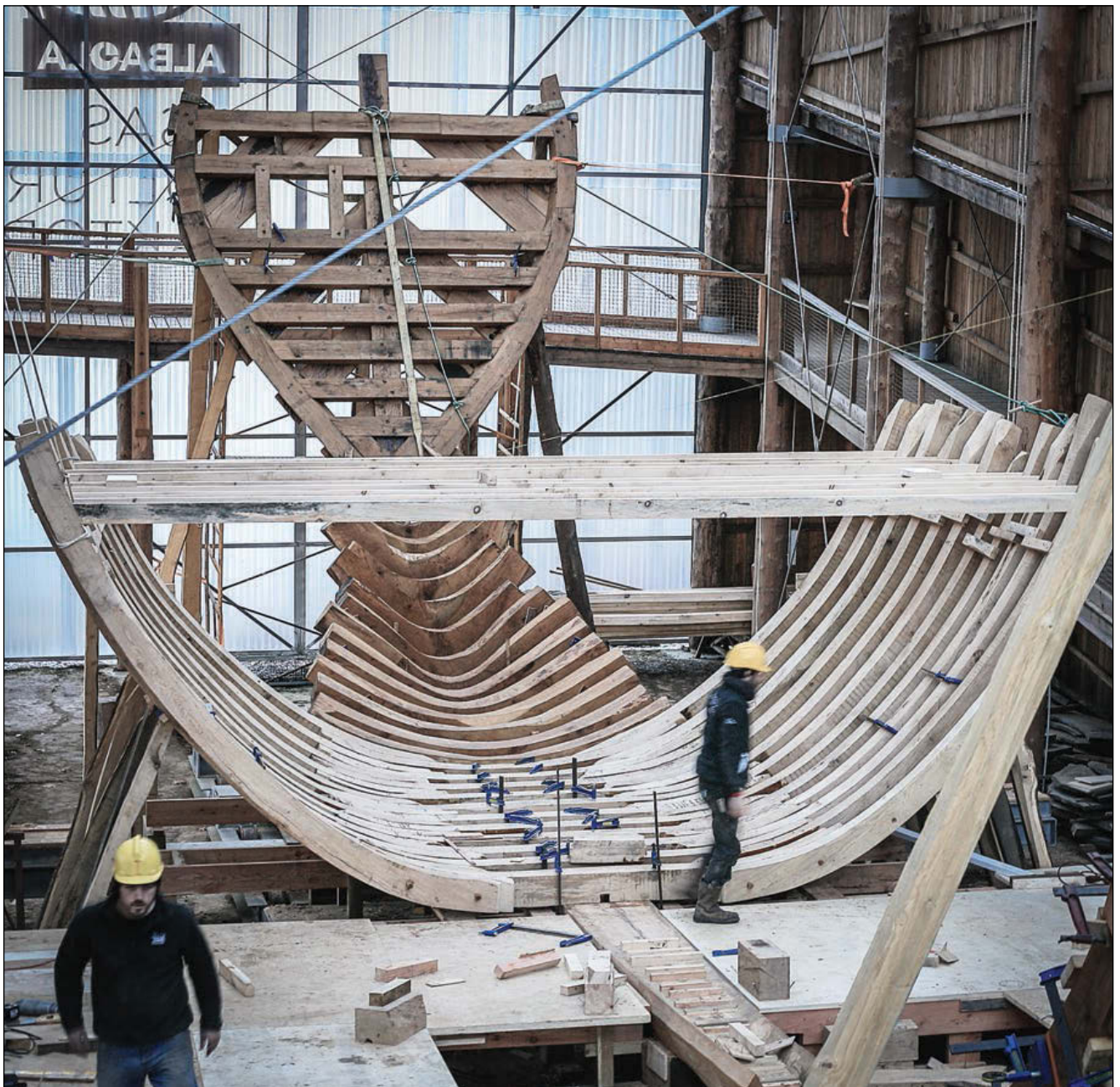
As of January, SAN JUAN's first few frames had been raised; by the time this magazine is printed, planking will have commenced.
