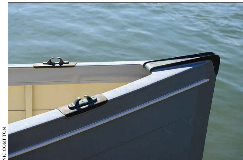
GRÉTA's custom-cast bronze mooring line fitting replaces the conventional bow roller.
