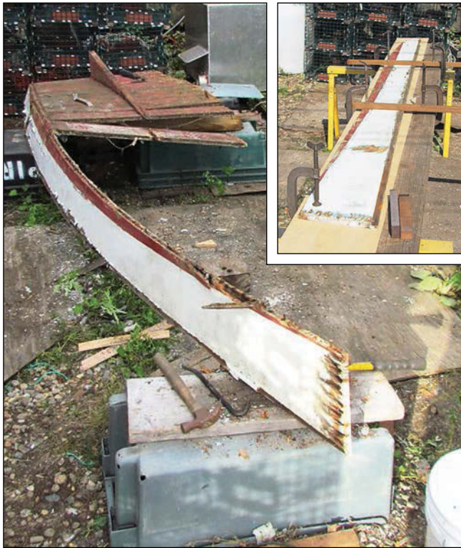
Once the boat was measured and photographed, it was dismantled for patterns. Inset —A starboard plank is clamped to new white-pine stock, ready for duplication.
