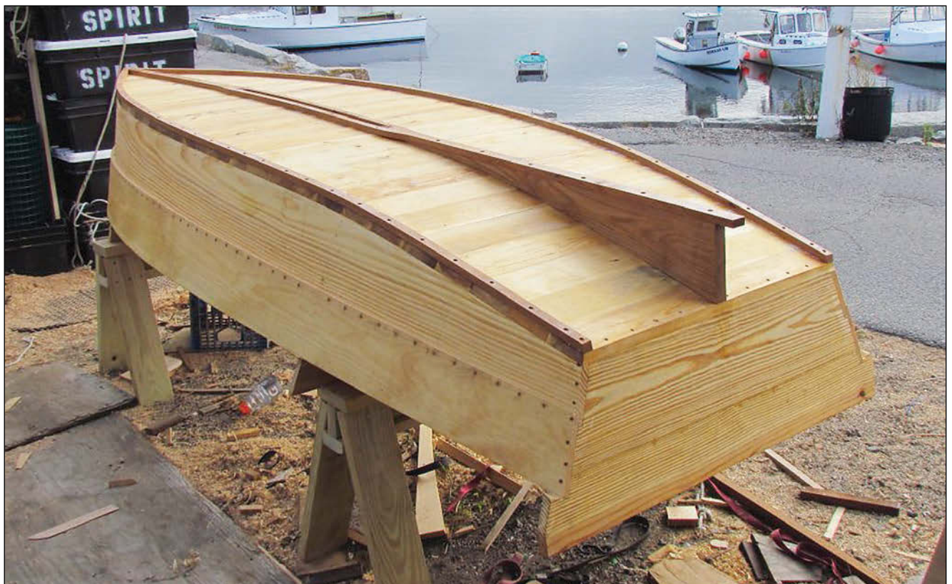
The bottom was cross-planked with short cedar stock. Guardrails, keel, and a skag of white oak were then added.
