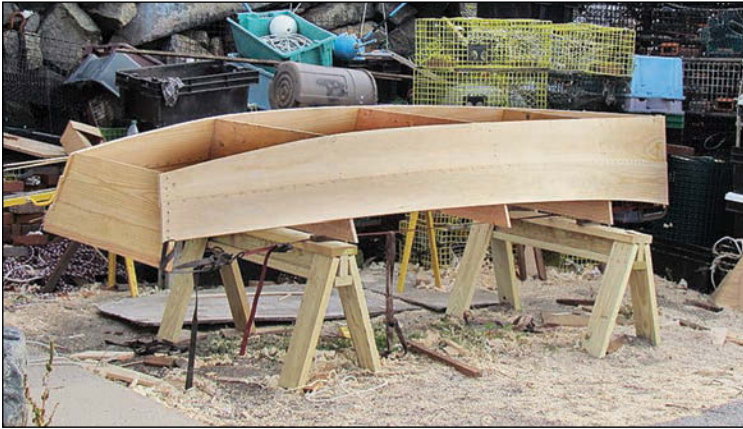
The partially completed boat was inverted on sawhorses, in preparation for bottom planking.
