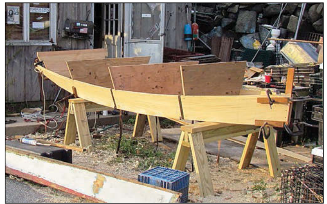
Once the boat was measured and photographed, it was dismantled for patterns. Inset —A starboard plank is clamped to new white-pine stock, ready for duplication.
