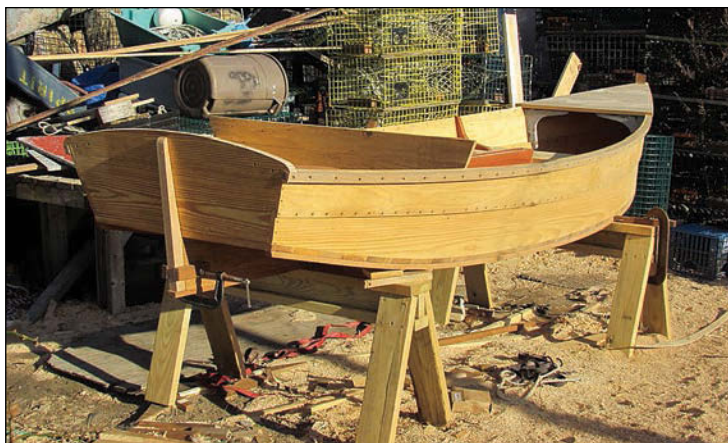
The finishing touches included a short foredeck, the centerboard trunk, and sternpost.
