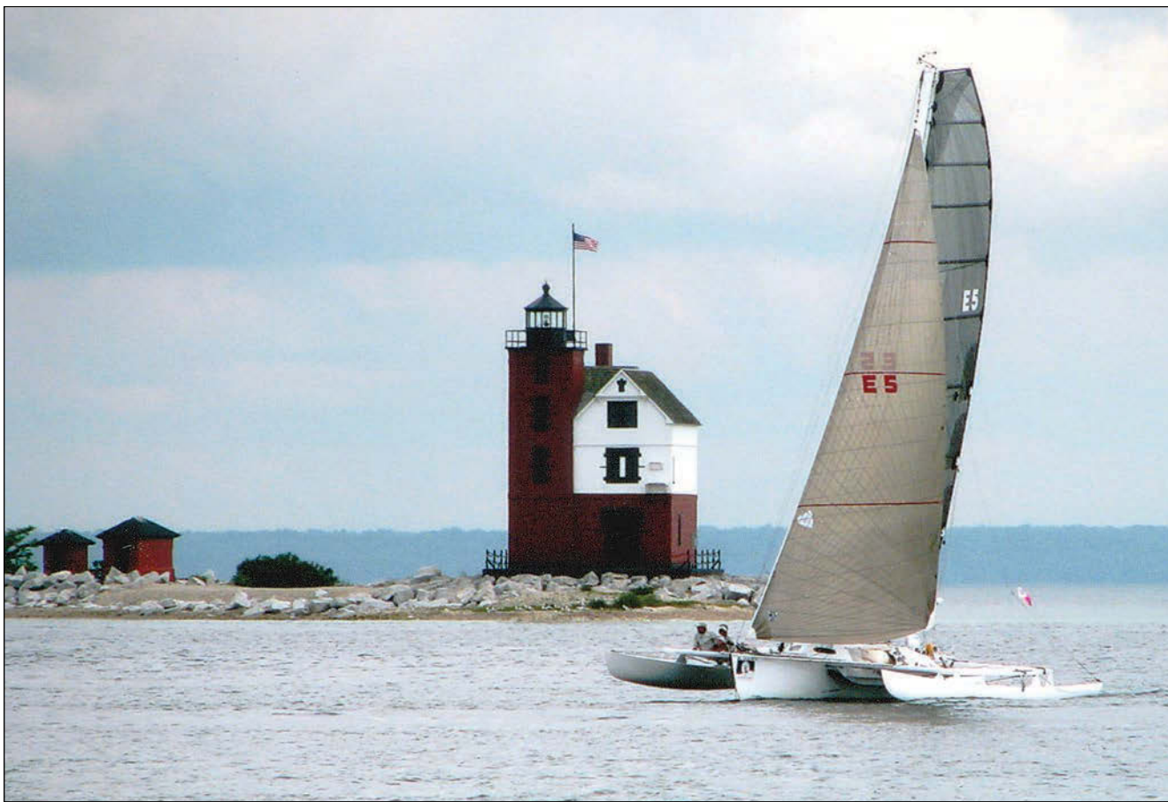
Meade and Jan Gougeon built the 35' offshore triamara ADAGIO in 1969. She was the first large wood-epoxy boat built without fastenings, and has served as a test bed for the longevity of wood-epoxy structures. She completed the 2002 Chicago to Mackinac Race, in which she survived a storm with wind topping 69 mph. ADAGIO's top speed in that race—her fastest ever—was over 30 knots.
