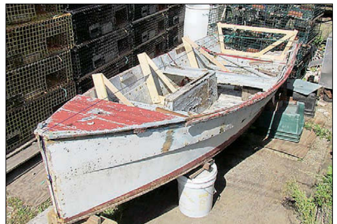
Here, the original boat is pulled back into shape, with three molds and a transom pattern holding it to its lines.
