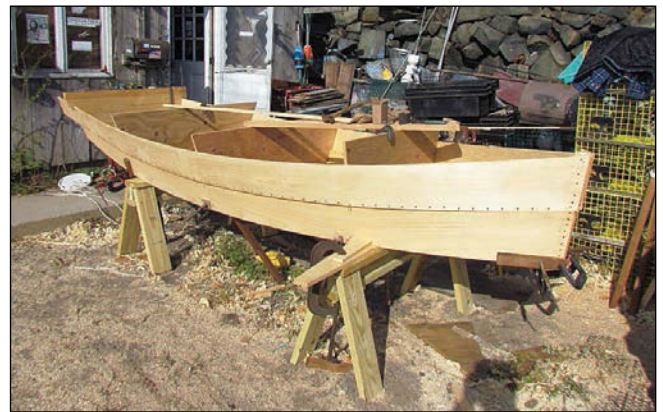
With the major pieces cut to shape, the boat went together quickly. Top —The lower side planks are fastened to the stem. Middle —While molds were not used in the original construction, three were used in the replication to carefully control the boat's shape. Once these were installed, the side planks were bent to the transom and fastened. Bottom —The sheer planks are installed, riveted along their entire length.
