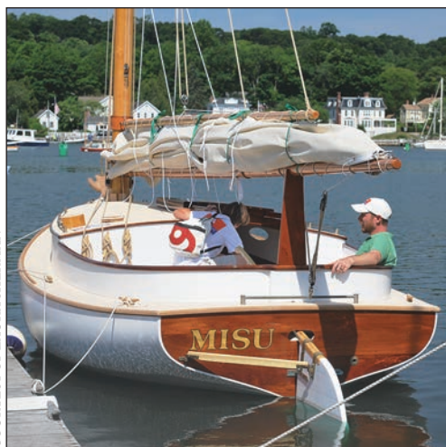
MISU, a 23' cold-molded catboat, was the final boat constructed at Suzanne Leahy's Pleasant Bay Boat and Spar Company on Cape Cod, Massachusetts.
