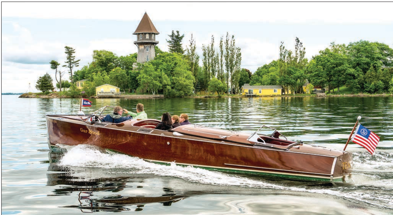
The 28' TEAL is one of the museum's newer boats. It was built by Gar Wood Custom Boats of Brant Lake, New York, in 1989, to a 1939 triple-cockpit runabout design by Gar Wood himself.
