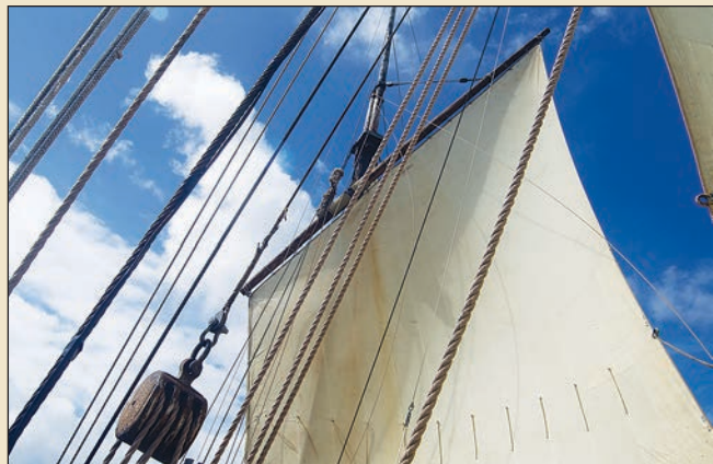
Lug-rigged vessels—in which the head of the sail is laced to a yard that is hoisted alongside the mast—became known for eluding square-riggers by outperforming them in sailing to windward.
