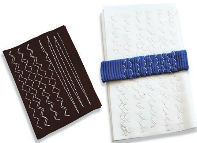
A stitch sample from the Sailrite LSZ-1. The machine is rugged enough to sew through eight layers of Dacron. It will also stitch through webbing, and 10 layers of canvas.
