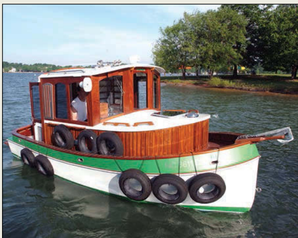
Above —This 18'-long mini-tugboat was built by Bill McComb from plans by Glen-L Designs ( www.glen-l.com ). L'L MCTUG has a marine plywood hull, teak deck, and teak and mahogany trim. Bill launched her last May on Lake Norman near his home in Davidson, North Carolina. She is powered by a Yanmar inboard diesel.
