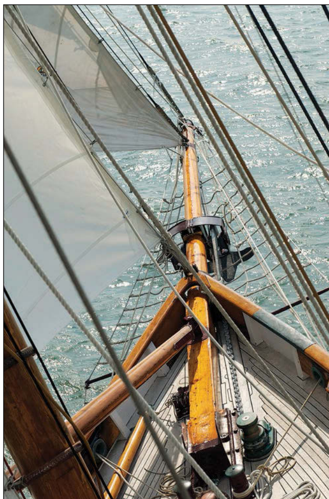
A new rode system, using rollers housed in a substantial bowsprit fitting, allows efficient anchoring.
