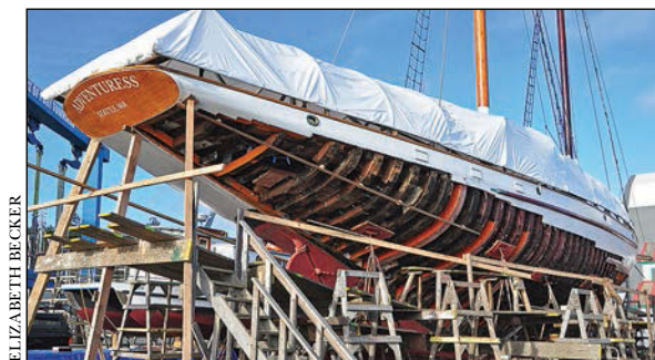
The 101' LOD schooner ADVENTURESS, a B.B. Crowninshield design from 1913, is undergoing a fifth phase of restoration, this time replanking and reframing the lower starboard side, at Haven Boatworks in Port Townsend, Washington.
