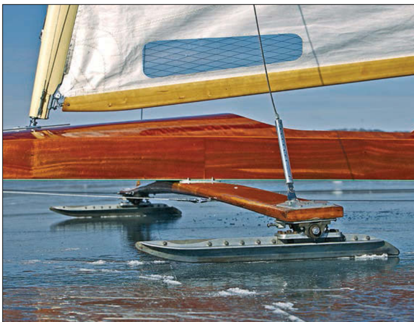
The runners, stiffened with aluminum angle cheeks, are mounted in pillow-block bearings so that even in a steep hike they are free to articulate.
