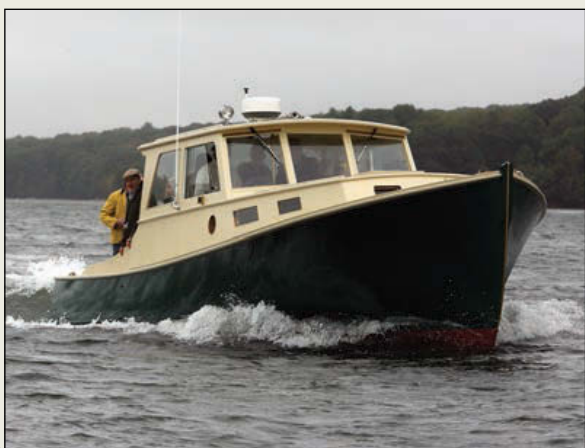
Above —Under direction from Eliot Spalding, Alex Hadden took the lines from Vinnie Cavanaugh's MARIAH WILLO and, from them, built JUDY SUE. She is a 36' lobsterboat traditionally built of cedar on oak with bronze fastenings. Powered by a 265-hp Yanmar, she cruises easily at 14 knots and will make 20 knots wide open. Contact Alex at haddenboat@gmail.com for more information.
