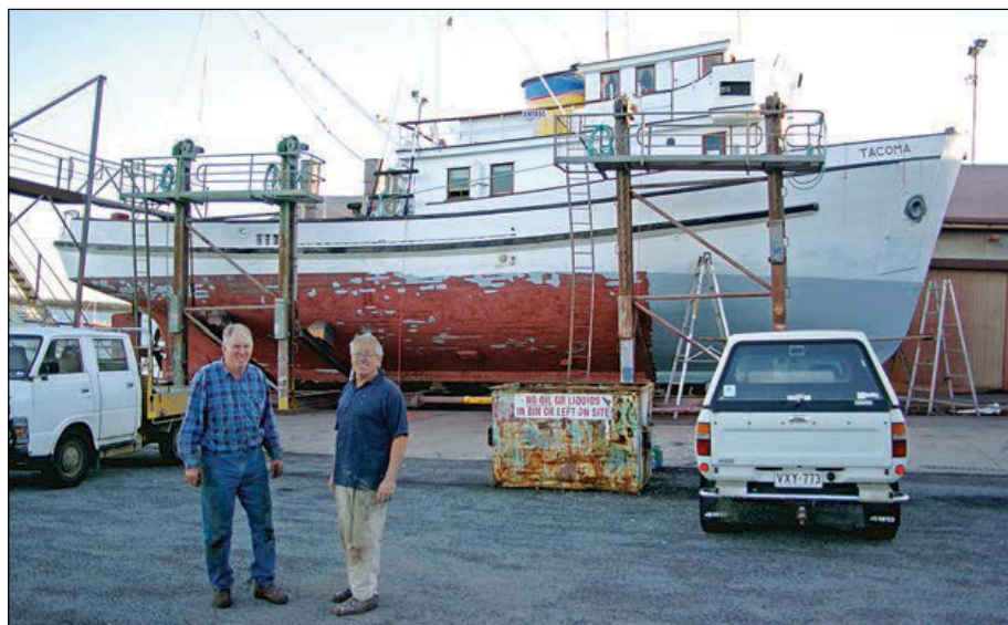
TACOMA with Haldane cousins Andrew and Ross at the Boston Marine slip Port Lincoln preparing for the 2,500 mile round trip to the 2011 Australian Wooden Boat Festival in Hobart, Tasmania. TACOMA retired from active fishing in 2003. Her bow has just been refastened with 4" silicon-bronze screws.
