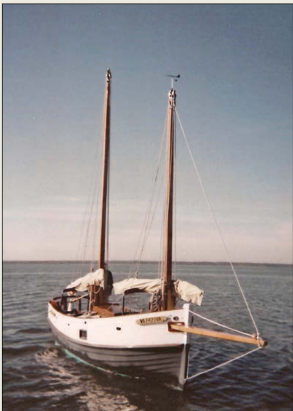
Above —After 40 years as a family doctor, John Gremer built this 25' lug-rigged schooner as a retirement project. He was inspired by Phil Bolger's St. Valery design in WB No. 157. The schooner's hull is built of okume plywood, the interior of Honduras mahogany, and exterior trim of teak. The spars are Douglas-fir and the sails were sewn by HT Sails. John sails SARABAND in Chesapeake Bay.
