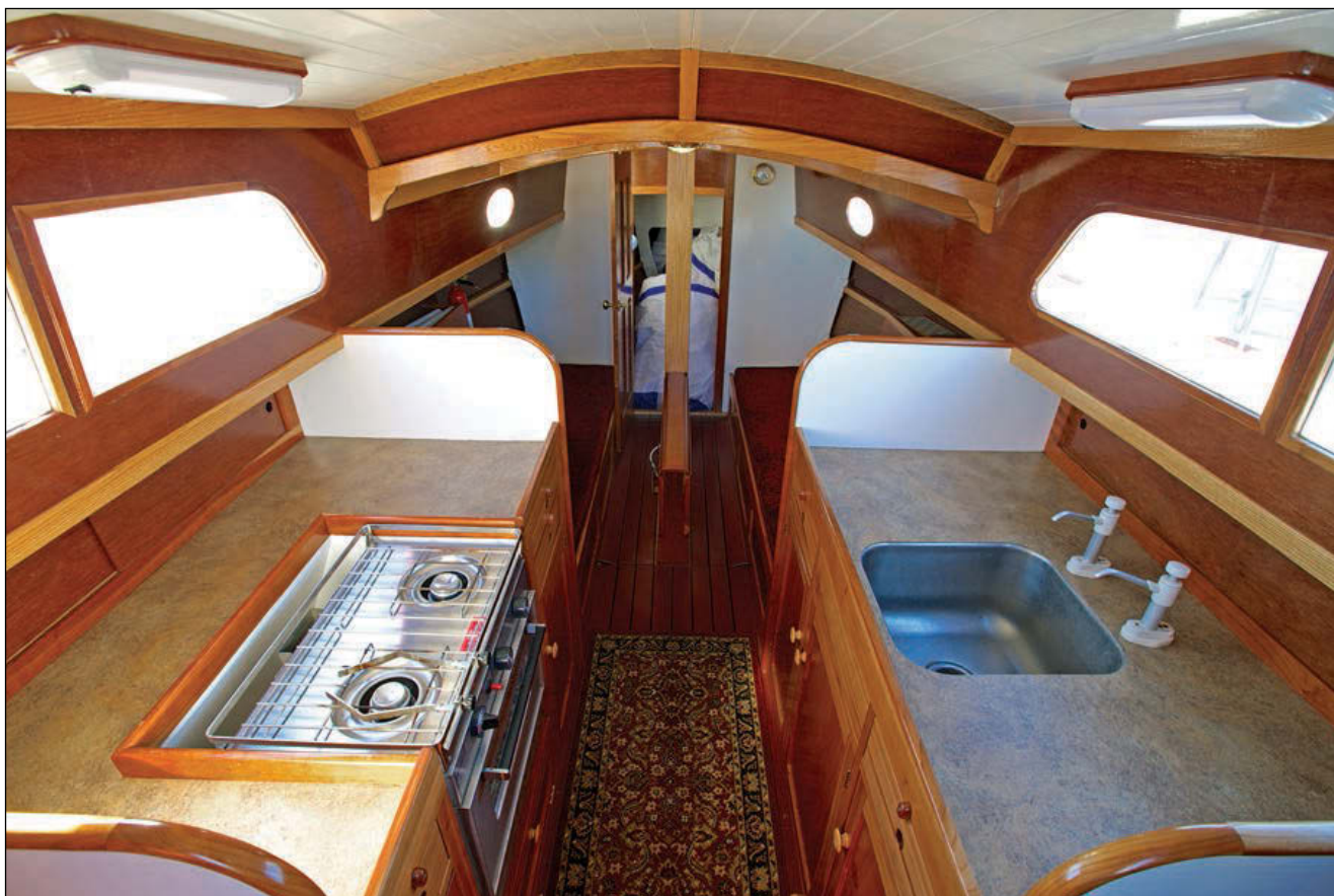
GRACE EILEEN's tidy, symmetrical cabin includes a galley that spans the width of the boat, and a narrow passage for safe and easy work in a seaway.
