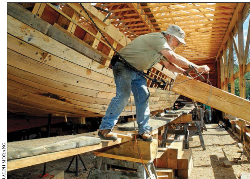
Shipwright Dennis Glidden receives a plank from the steambox ready to fit it in the stern. While a small group of shipwrights were employed, around 5,000 volunteer hours went into the building of the new gundalow.
