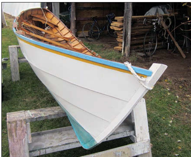
This 18' Peter Chase–designed and –built Cape Rosier Guide Boat evokes the builder's Scandinavian heritage. The boat is meant for recreational rowing, fishing, and guiding, and can be rowed from three different stations—or by three people at once. It's planked in local cedar and framed in oak, and the interior is finished in oil.
