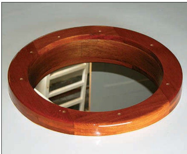
The author built this teak hatch coaming to replace a large portlight that had been doing duty as a hatch.
