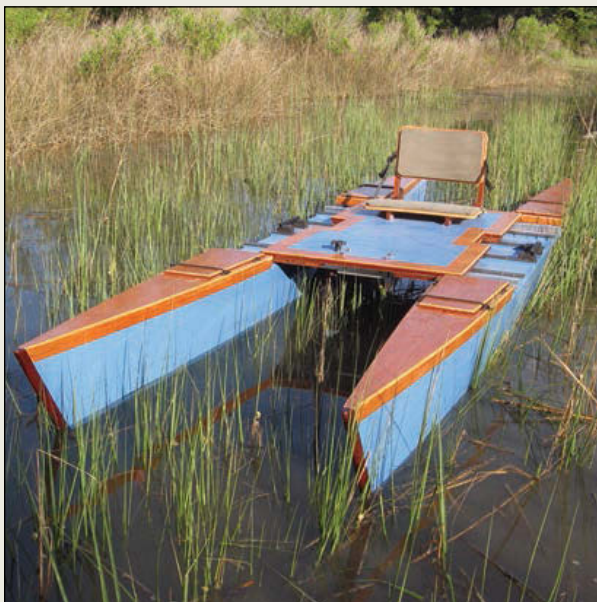
Above —Aaron Baldwin of McClellanville, South Carolina, designed this plywood-and-epoxy 12' "biyak," SKIMMER. A biyak is built from two enclosed hulls connected by a deck between them. The beam, adjustable while afloat, is either 30", suitable for paddling from the chair, or 46", stable enough for him to stand up and fish. Contact Aaron at aaronbaldwin8@gmail.com .
