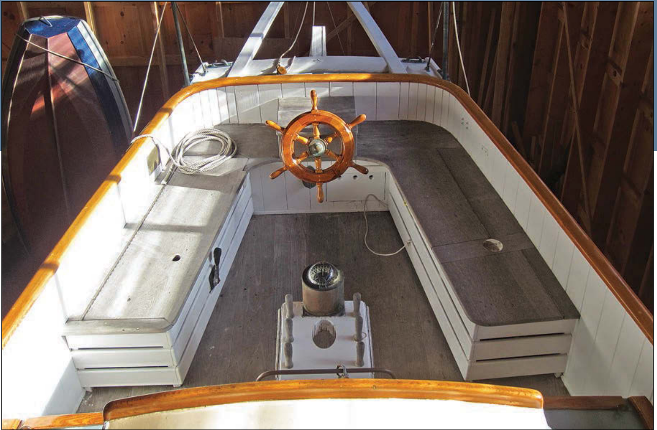
Peter Chase built this new cockpit for the author's Concordia 31 ketch VITAL SPARK. The new work had to fit seamlessly with the original, so as not to appear "grafted on." Chase took joinery design cues from the original, and topped it all off with a coaming cap of local locust.
