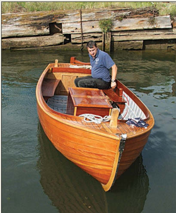
Above —DEJE is a 16' launch built by students at the International Boatbuilding Training College ( www.ibtc.co.uk ) in Lowestoft, England. Her owner took the lines off a local yard launch while an IBTC student, then later groups of students, completed her. She has carvel larch planking on oak frames, and is powered by an inboard Yanmar GM10.
