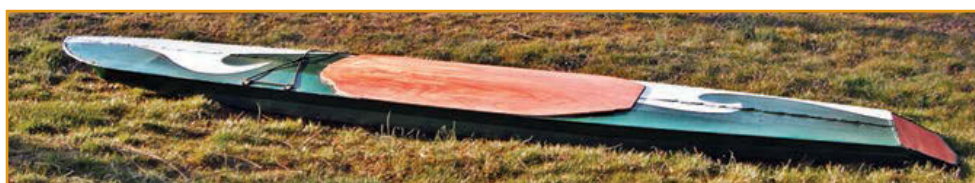
LANUI—from Gentry Custom Boats Skin-on-frame standup paddleboard LOA 13'; Beam 30"; weight 25 pounds; $800
