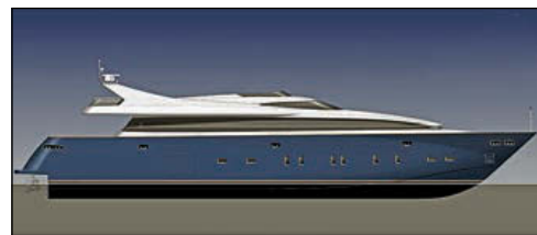
A 125' megayacht with water-jet propulsion—all in a cold-molded wooden hull—is under construction in Lavagna, Italy.
