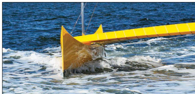
Left —Lightweight and strong plywood-epoxy construction is exposed during the rollover of the proa's 31' main hull, which has a waterline beam of less than 24". Above —Like any proa, MADNESS's most distinctive element is its slender outrigger, whose weight is kept 15' to windward by crossbeams. (In this photo, the daggerboard is retracted.)
