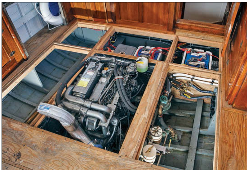
The rebuilt Yanmar engine, new electrical wiring, and other systems are carefully installed under the new wheelhouse sole.
