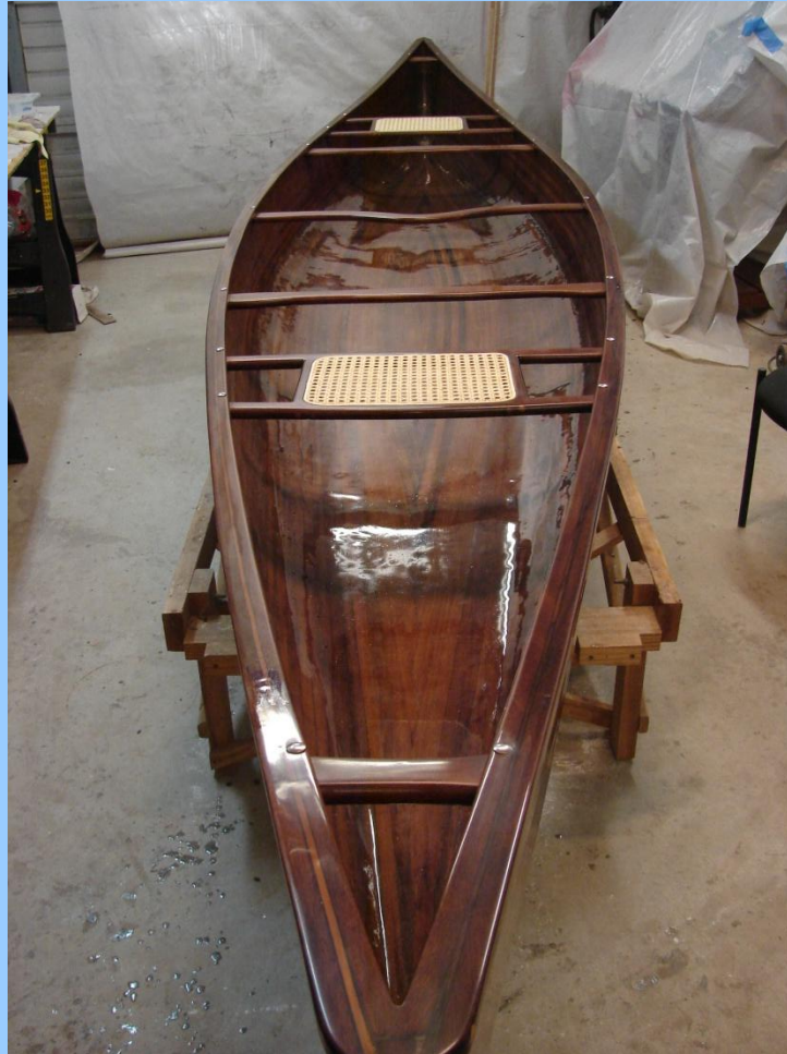
Redwood Strip-built Canoe Restoration (after)
