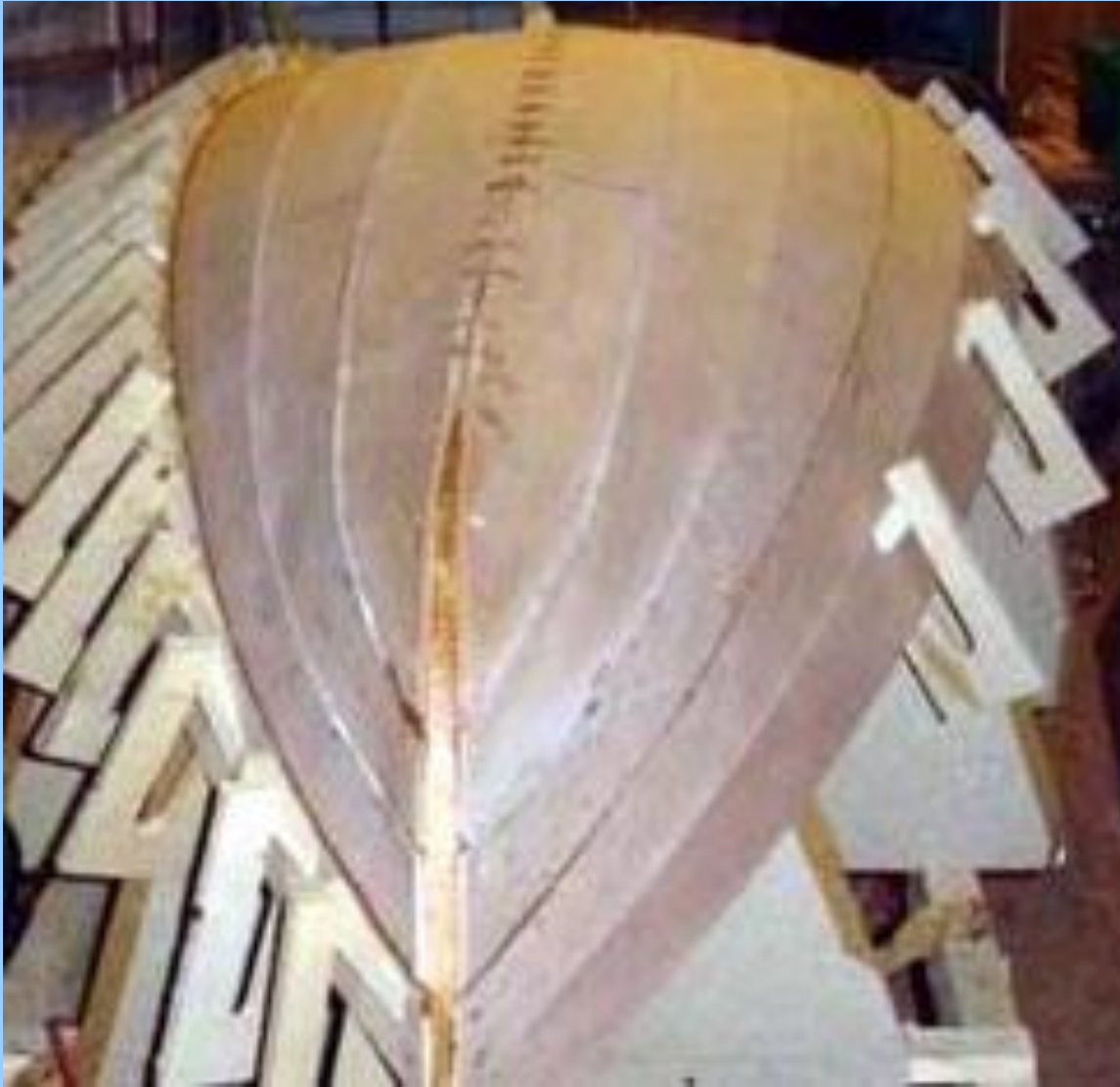
Strakes installed using shop-built C-clamps and wedges
