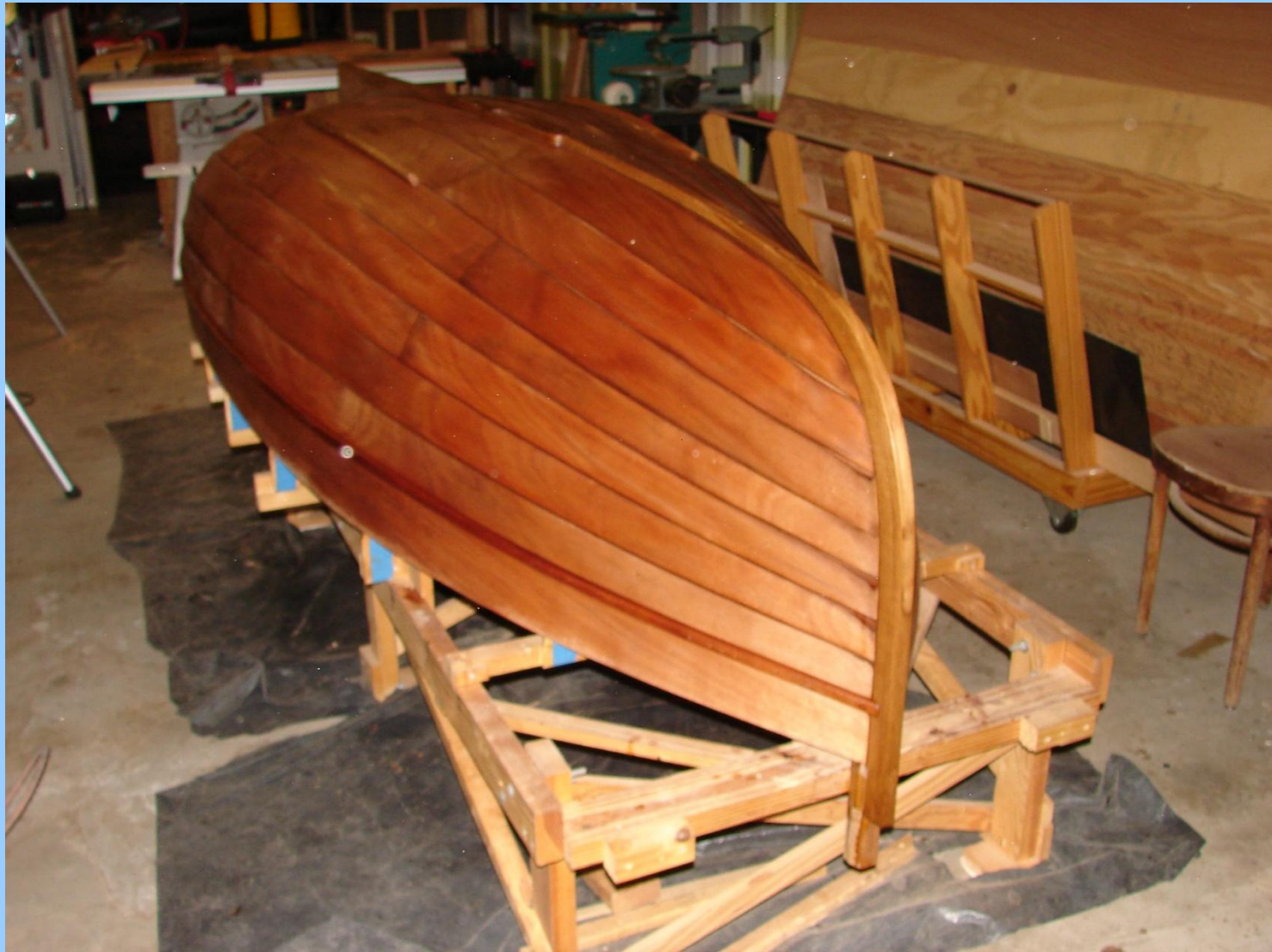
The sealed hull showing White Oak stem, Okoumé plywood strakes and Mahogany rub rail.
