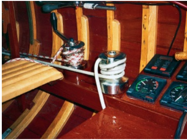
FIGURE 98 } Sistered ribs provide strength where the original ribs are overloaded.
