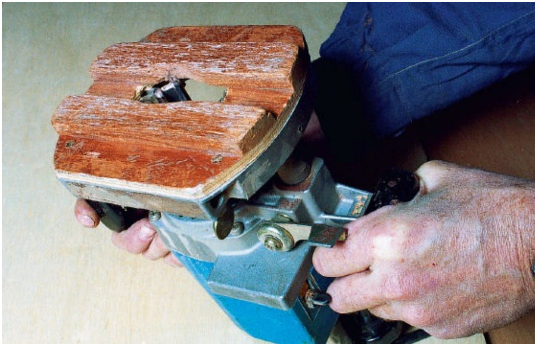
FIGURE 102 } Router with spacers. The blocks are screwed to the plate and the router cutter set out so that they are a little bit under the tops of the blocks. The blocks then slide along the planking while the cutter routers of the exes of the plugs.
