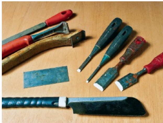
FIGURE 49 } Chisels and a Japanese pull saw, scraper, hardwood floor scraper, Sandvik's paint scraper with replaceable carbide blades, mill saw file.
