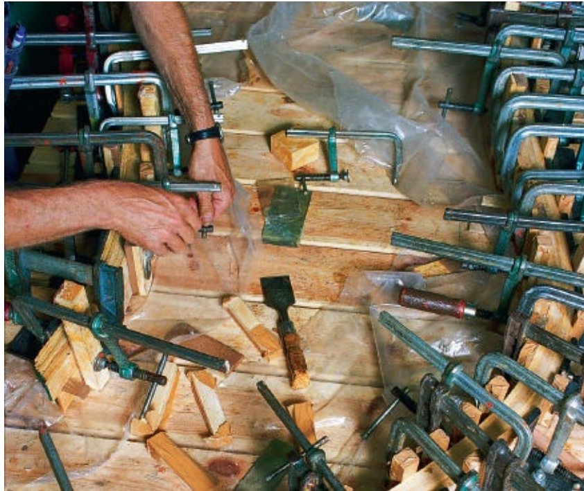
FIGURE 90 } It takes a lot of clamps to glue frames. The template consists of a wood table with removable supports made of clamps. The clamps are fastened with a bolt and washer in the groove in the table.
