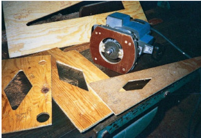
FIGURE 56 } Router with a copying ring and router templates of plywood. The hole in this case will be \frac{1}{16} " (2 mm) smaller than the template and will end with a rounding of the router steel's diameter.
