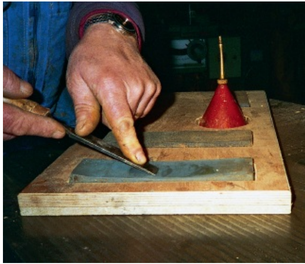
FIGURE 57 } Sharpening on an oilstone. The chisel is moved with the sharp side flat against the stone with an even rotating motion.
