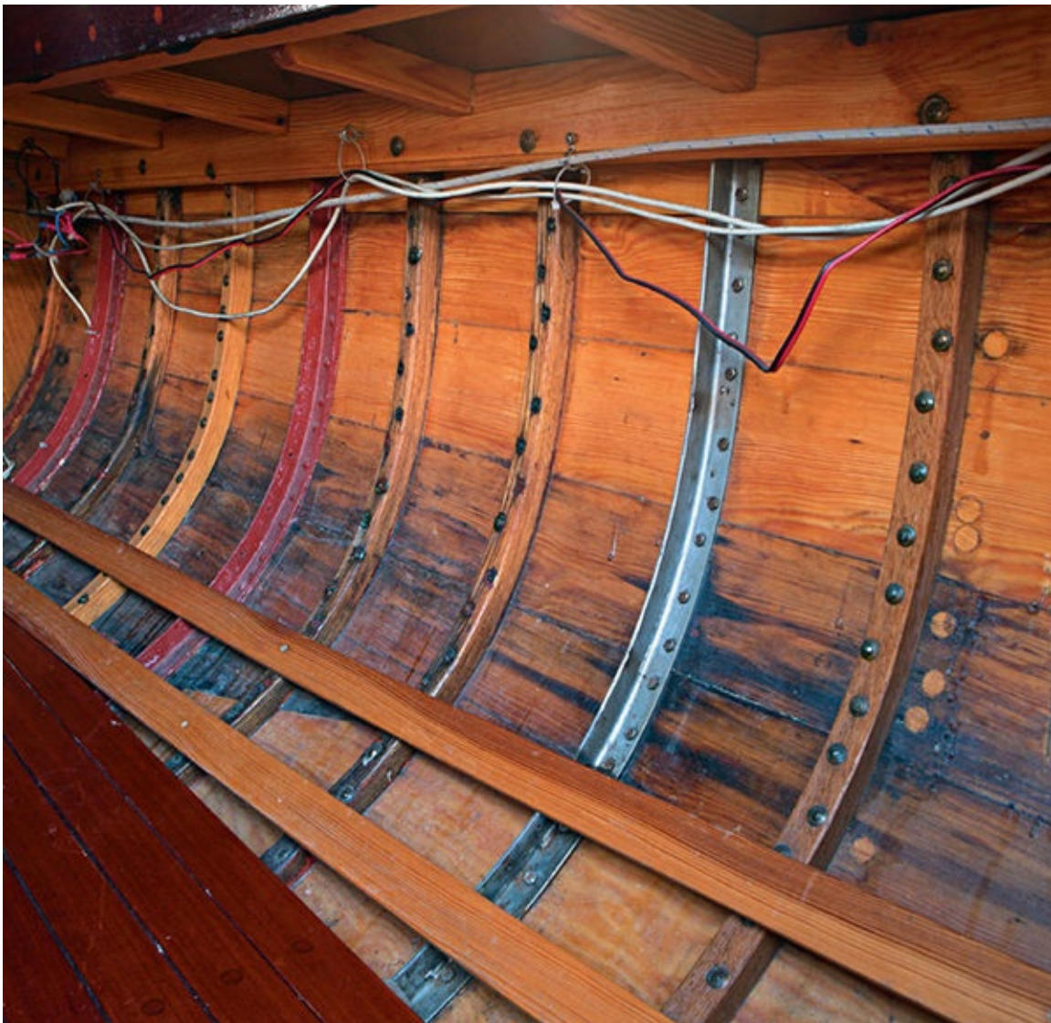
FIGURE 98 } Sistered ribs provide strength where the original ribs are overloaded.
