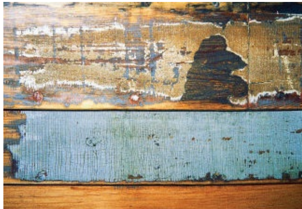
FIGURE 4 } Extremely cracked oil paint. Saved as a color sample in the renovation of a steam sloop from the 1800s.
