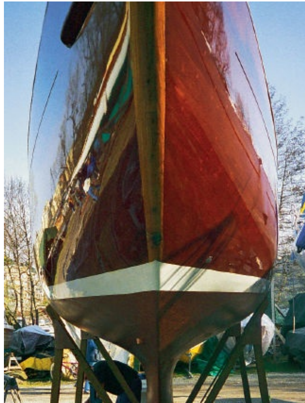
FIGURE 11 } Glossy topside at launching. The long sanding block gives smoothness; the sanding gives the glossiness. The surface has been obtained with a roller and a foam brush. Total varnish used for the final coat was 1.2 qt (1.2 liters) to 172 sq ft (16 m 2 ) of topside.
