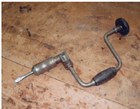
FIGURE 42 } A brace drill with chisel is the best tool to loosen old screws and also to tighten screws during the last assembly of the planking.
