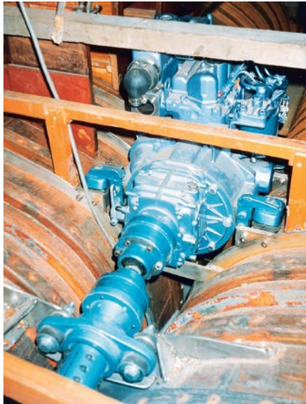
FIGURE 205 } Engine mounted with a thrust-bearing joint with a bulkhead (shaped like steel floors in this case). This sort of shoehorn assembly requires that the motor be used as a template.
