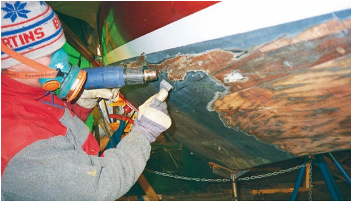
FIGURE 5 } Scraping the paint using a heat gun.
