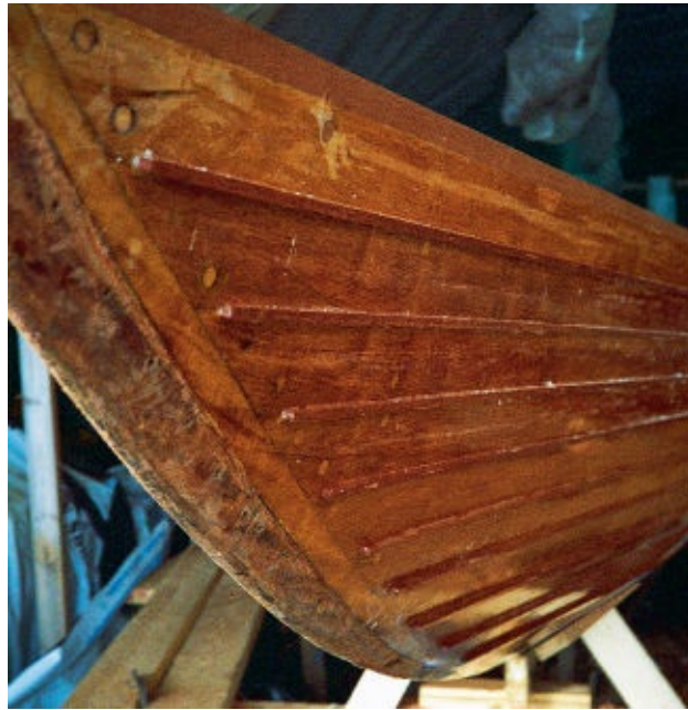
FIGURE 77 } Splined topsides. If the old varnish is left on the hull while splining, it will make it easier to remove splining residue. The strips are cut by the bow with the same shape as the circular saw blade.
