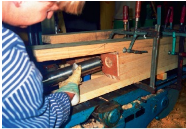
FIGURE 151 } Drilling a shaft hole with a pipe drill.
