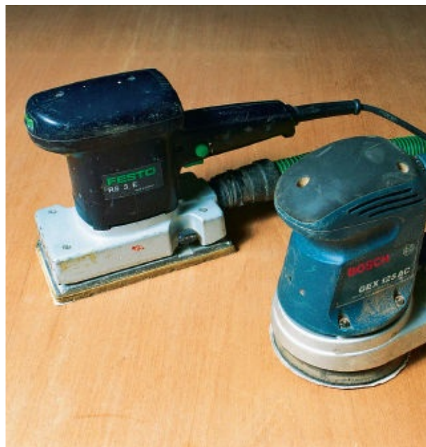
FIGURE 9 } Sheet palm sander and random orbital sander.
