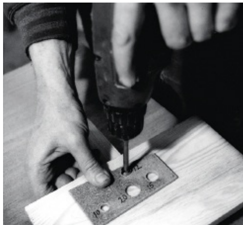
FIGURE 52 } Drilling the plughole. Plug-hole drilling with Forstner drill bits. Using a piece of MDF or a thin piece of wood with pre-drilled holes to provide good guidance for the Forstner bit when old holes are being enlarged. The uneven grid of the MDF also provides a good friction against the surface underneath. For more about the drills, see Chapter 10 on tools.
