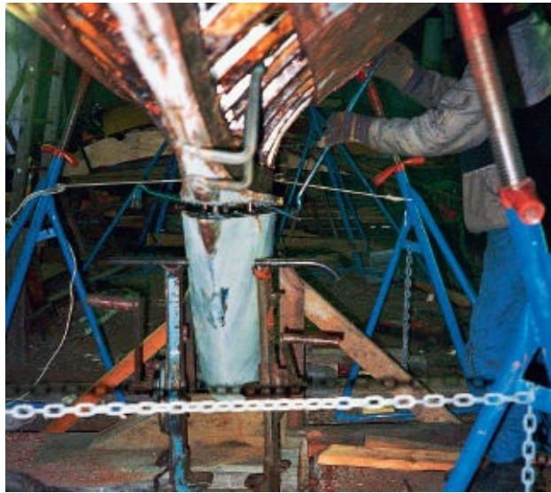
FIGURE 141 } Rigging jacks on the 6-meter racer Lillevi . Two jacks are mounted on a beam through a keel pocket, and a hydraulic jack is under the keel's aft edge.
