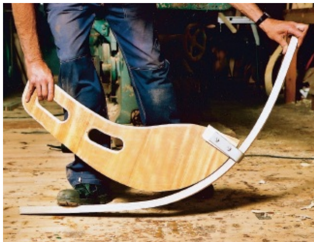
FIGURE 95 } Lever for pre-bending and over-bending the rib. If the rib has been over-bent while warm and not broken, it will have fewer residual tensions in the cold.
