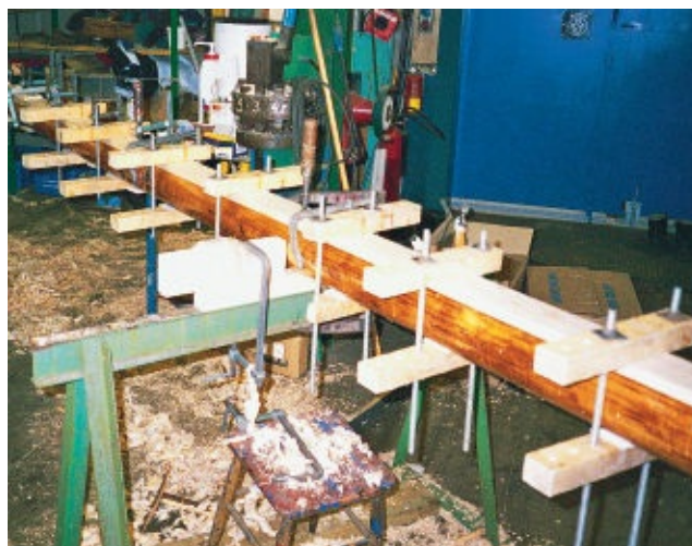
FIGURE 201 } Mast clamps are inexpensive and easy to make; all it takes is planed timber, 2\frac{1}{2} \times 1\frac{1}{2} " (60 × 40 mm), and a threaded rod with a nut.
