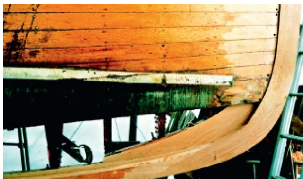
FIGURE 150 } The stem knee continues behind the old planking above the waterline. The good grain direction in the
