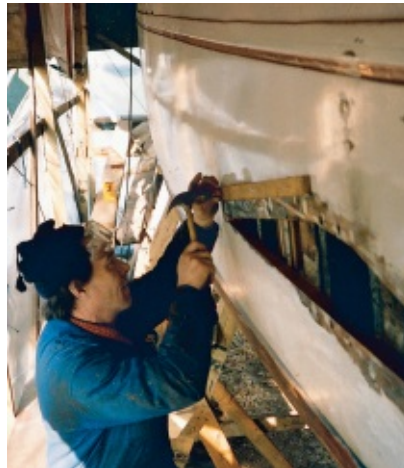
FIGURE 71 } The backing block is cut out, the butt joint is moved to the right of the frame, the plank has a spliced joint to the left.
