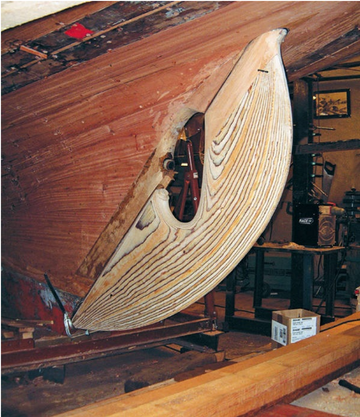
FIGURE 204 } Hole in a sailboat rudder for a propeller. The rudder is made of plywood and is coated with epoxy and matt. The height curves in the plywood make it easier to cut out the rudder to accurate shape.
