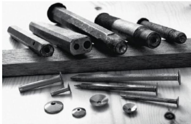
FIGURE 31 } Tools for riveting. Homemade sets and fasteners and a combination tool that was previously sold in hardware stores. Round copper rivets and square copper nails and roves, i.e., cupped copper washers.
