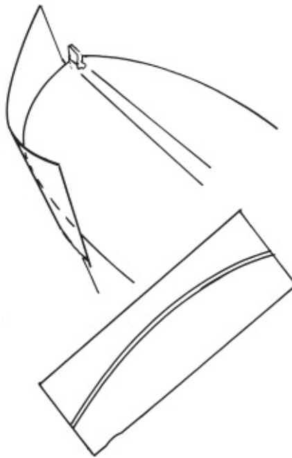
FIGURE 185 } The curve on the semicircular trim at the bow of motorboats is often highly curved in the vertical direction. The trim is stiffer vertically so the curve can then be templated and then sawn up.
