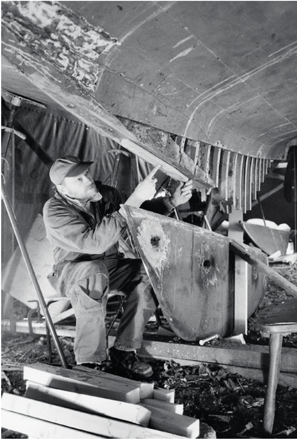
FIGURE 3 } Limiting the scope of work is one of the greatest difficulties with renovation. Repairs to the stem in conjunction with replacing the wood keel.
