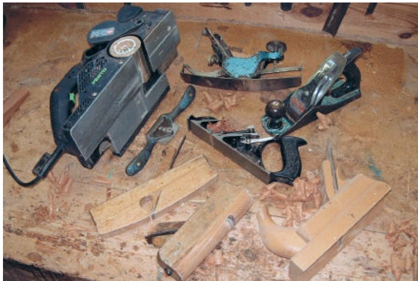
FIGURE 48 } An electrical hand planer with unlimited cutting depth. The cutter head is stored only on one edge, so there is nothing sticking out on the other side. It makes it a good planer for rabbets. The finishing planer is a good all-around planer. The iron shoulder plane is used for corners. The wood shoulder plane is good for rabbets. The adjustable circular plane is a boatbuilding tool. The bowl plane and the mast-cutting plane provide concave and convex surfaces. A spoke shave is great for frames.
