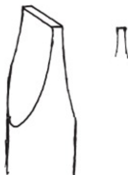
FIGURE 50 } If you are going to get anywhere with screws that are stuck, you have to have sharp edges on your screwdriver, preferably with a little hook.
