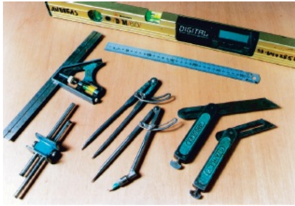
FIGURE 44 } Various measurement tools: digital level, adjustable square, steel ruler, marking gauge, divider and compass, and sliding T bevel—the right one is cut to be used in shallow rabbets.
