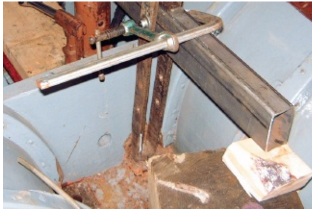
FIGURE 157 } One way to arrange a yoke with a lever and jack; most boats are different in the bilge, and you can experiment with different solutions.
