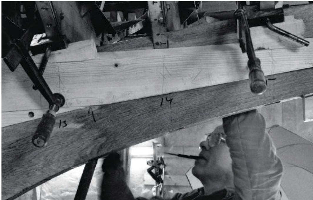
FIGURE 131 } Planks wedged with clamps of the type that are used by plyms at the Neglinge shipyard. Here you can also see the numbering of the ribs.
