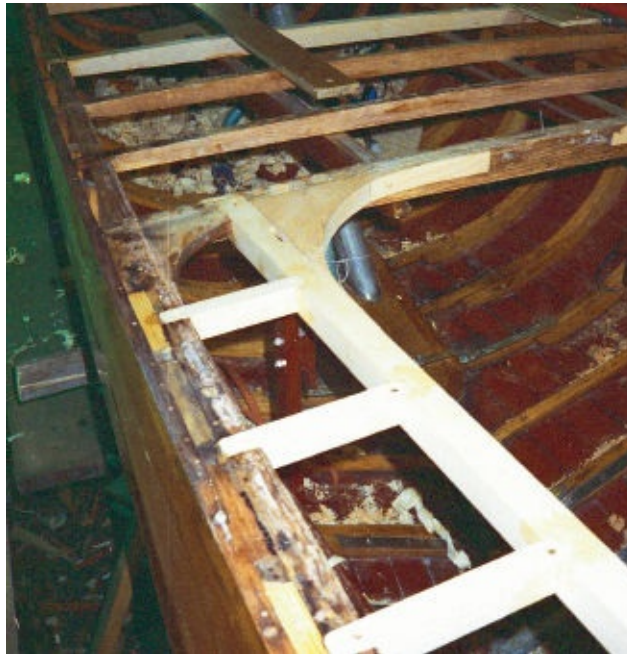
FIGURE 168 } Make sure to replace decayed and weakened deck beams; it's a chance that you won't get again.
