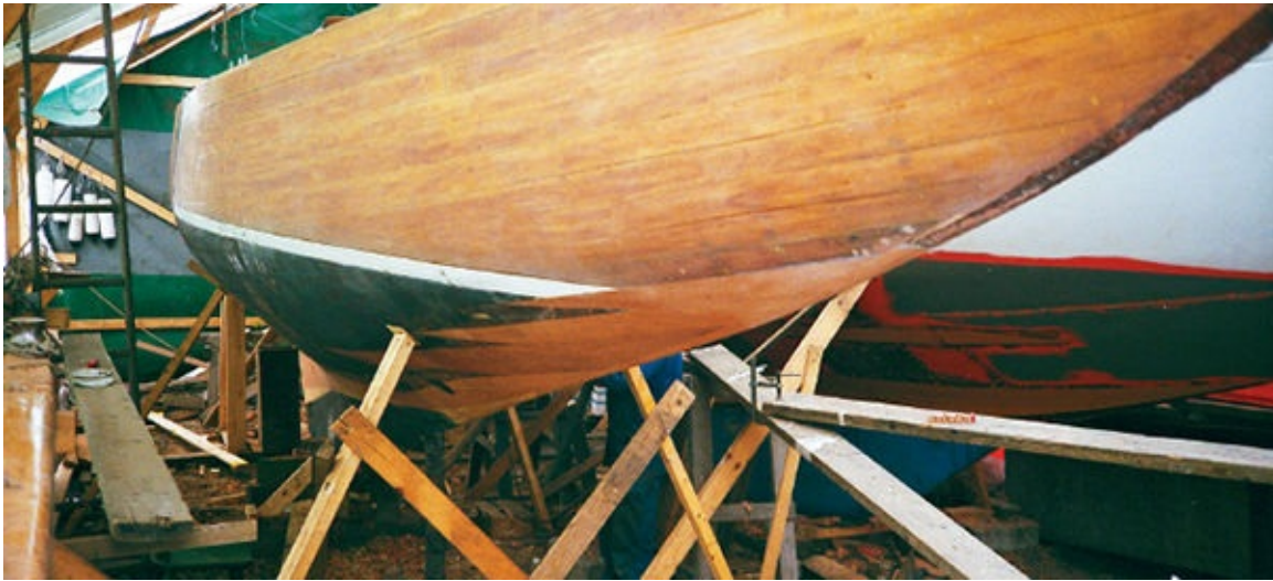
FIGURE 16 } Here, the bow has been replaced below the waterline; the ability to glue joints has made it possible to replace the planking, which had frozen apart, without replacing the entire bottom.
