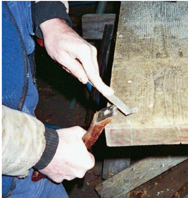
FIGURE 7 } Sharpening the scraper. Push the file diagonally away from yourself, and from the edge of the scraper. Hold the scraper on a steady surface.
