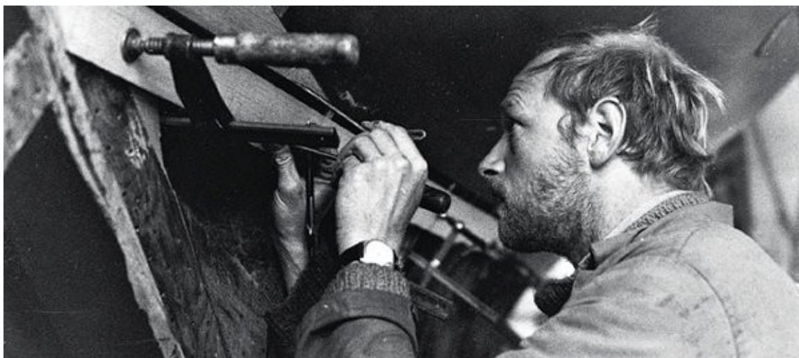
FIGURE 128 } Measuring the plank with a stick caliper and a spiling board.
