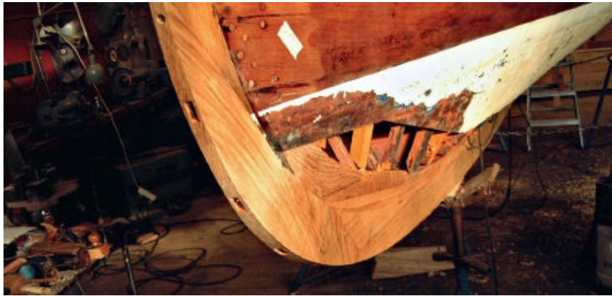
FIGURE 144 } Stem joint with knee. The bolts have T-heads so that they fit on the stem front.
