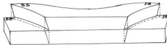
FIGURE 109 } You can't be sure that the floors are equilateral in an old boat, so you have to keep track of which is starboard and which is port.
