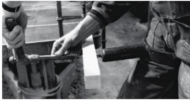
FIGURE 30 } Riveting. The rove is applied to the nail with the help of the rove set and a ball-peen hammer. Note that the bucking iron is made to fit the thigh.
