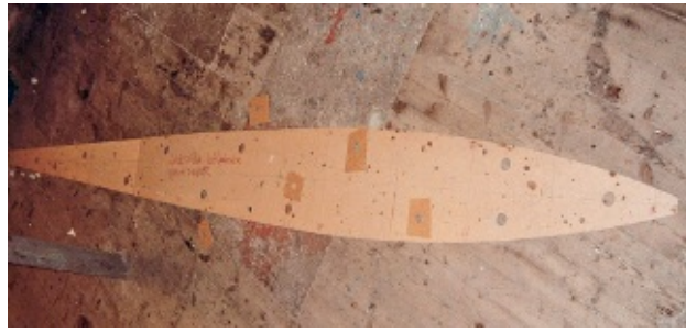
FIGURE 143 } Keel template. The holes in the keel template are made in excess. The template is placed on the ballast keel, and keel bolts are inserted into the holes. Then cut the small pieces with precise holes, place them down over the bolts, and glue them to the template.
