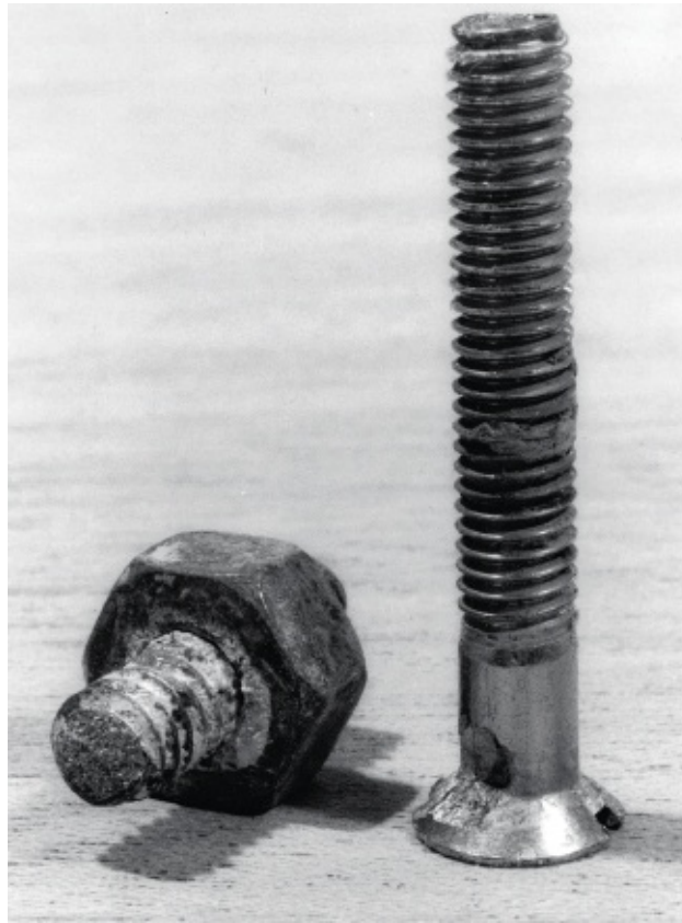
FIGURE 37 } Corrosion and burns in an eight-year-old stainless steel bolt and crystalline surface fractures of a forty-year-old stainless steel screw.
