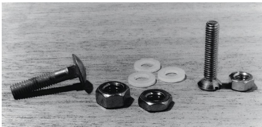
FIGURE 26 } Carriage bolts and flat, machine-threaded screw. If you want a smoother boat interior, then a low nut could be an alternative; its strength is enough to hold a screw in wood. Polyamide washers are used to isolate the stainless steel nuts from galvanized steel frames.
