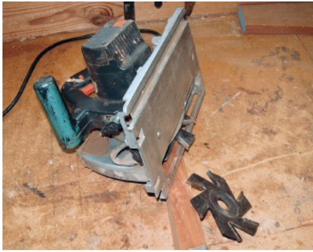
FIGURE 80 } A saw blade with tapered teeth. The teeth are \frac{3}{16} " (5 mm) in front and \frac{1}{4} " (6 mm) 1" (25 mm) from the front. The blade has only six teeth in order to eject the chips properly. In this case, the blade is in a circular saw with a lowering function. That is, the saw blade is lowered by the plate after it's started.
