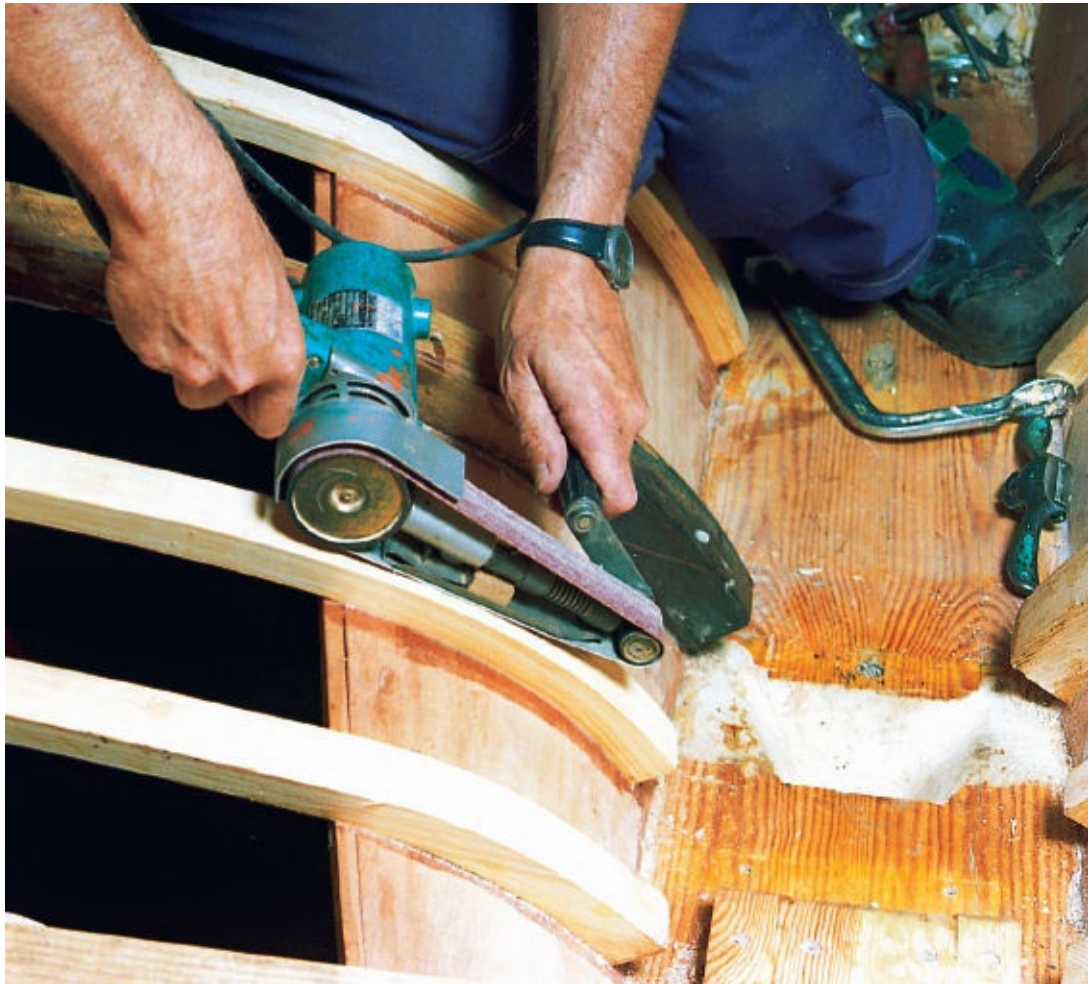
FIGURE 51 } The belt sander (Makita's belt sander) is a practical tool for polishing wood and grinding in templates.
