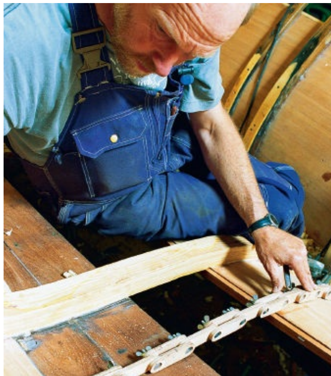
FIGURE 91 } This template is a quick way to make a rough template of the frame.
