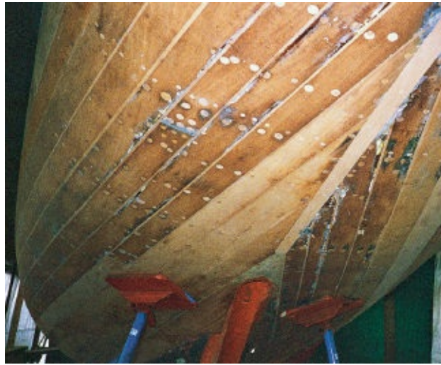
FIGURE 15 } This kind of planking would need to be exchanged without the ability to seam glue and glue in old plugs.
