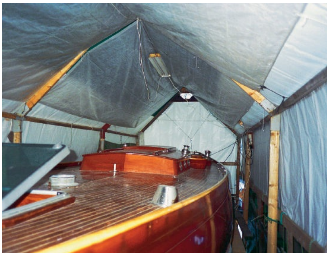
FIGURE 2 } Cover stand with inside tarps to prevent condensation. Note the ventilation hole at the ridge. The rack is built out of studs with bracket tubing. The truss has an angle of 90^\circ , so most of the snow will slide off. The most common hardware has a 60^\circ roof angle and requires snow removal, or it may break from wet snow.
