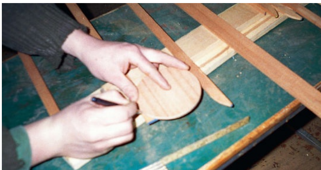
FIGURE 83 } Rounding off the seam trim ends using a template.
