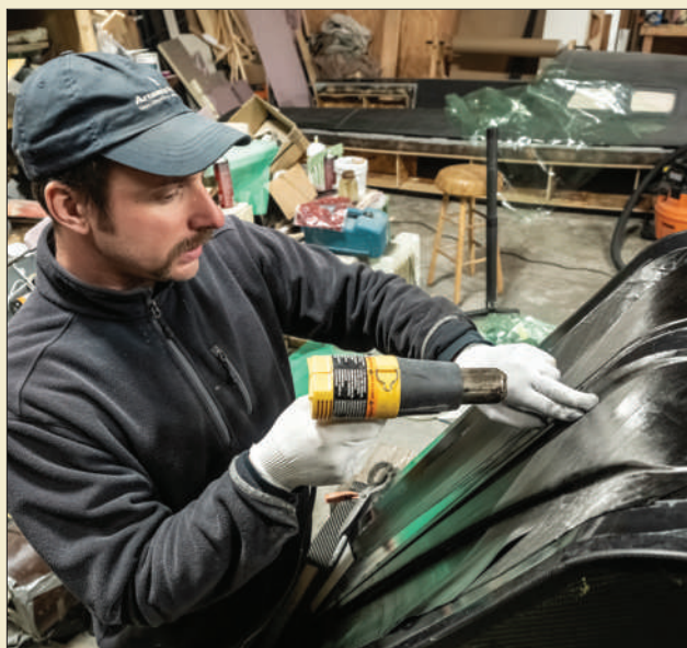
Simon Miles heats the prepreg to bond it to an adhesive film he put down onto cured substrate in the foil mold.
