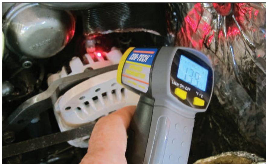
A laser heat gun, or a thermal-imaging camera, is a terrific tool for measuring the case temperature of alternators run hard. If not properly managed, this heat—frequently more than 100°C (212°F) and sometimes much higher—can destroy the alternator.
