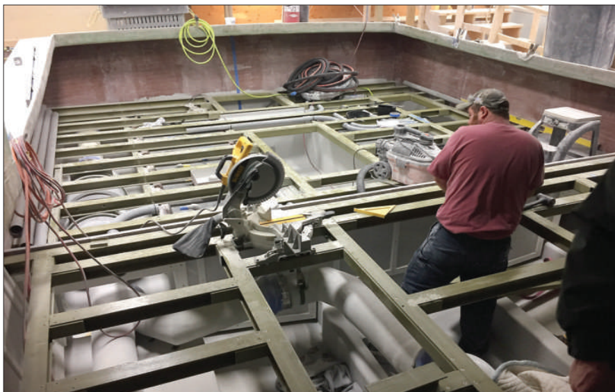
Left —The support grid of beams and stringers prior to deck installation reveals the mechanical systems and ample tankage space below the broad, open cockpit. Below —Full-size mock-ups helped inform final decisions like the one to not carry two Rocna anchors on bow rollers.
