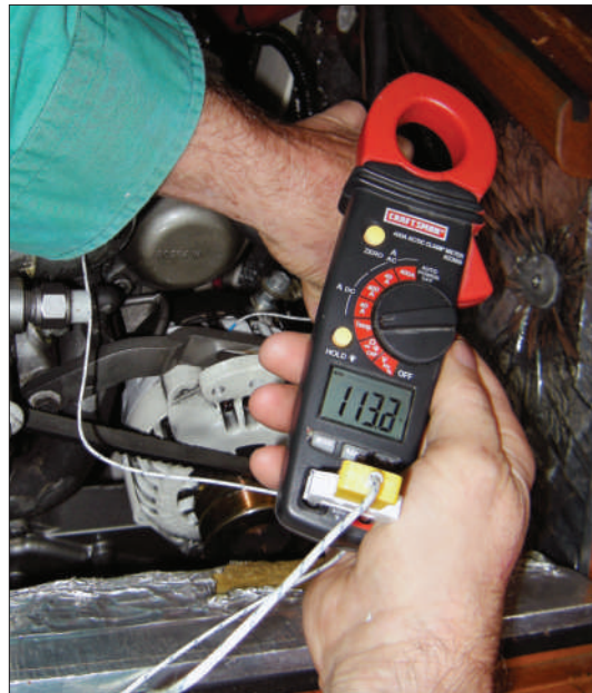
Another way to measure alternator case temperature is to attach a thermocouple to a multimeter and place the thermocouple on the case. The temperature on this alternator is just over 113°C (235.4°F).
