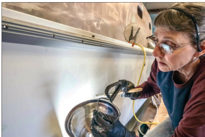
A lamp helps master finisher Naomi Bishtok find and fill pinholes in the primer coat on Scout's hull before the boat goes from Hylan & Brown to the paint booth at Brooklin Boat Yard.
