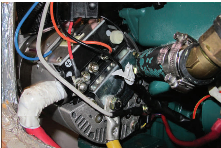
A 195-amp, 25V large-frame alternator is a tight fit on a Volvo Penta D2-75 engine. Most smaller alternators are grounded through the case and engine block, but on high-output alternators it is common to add a ground cable. In that case, two heavy cables (red and yellow) hang off the back of the alternator. They must be well supported close to but not in contact with the (hot) alternator case, and secured against vibrating loose.
