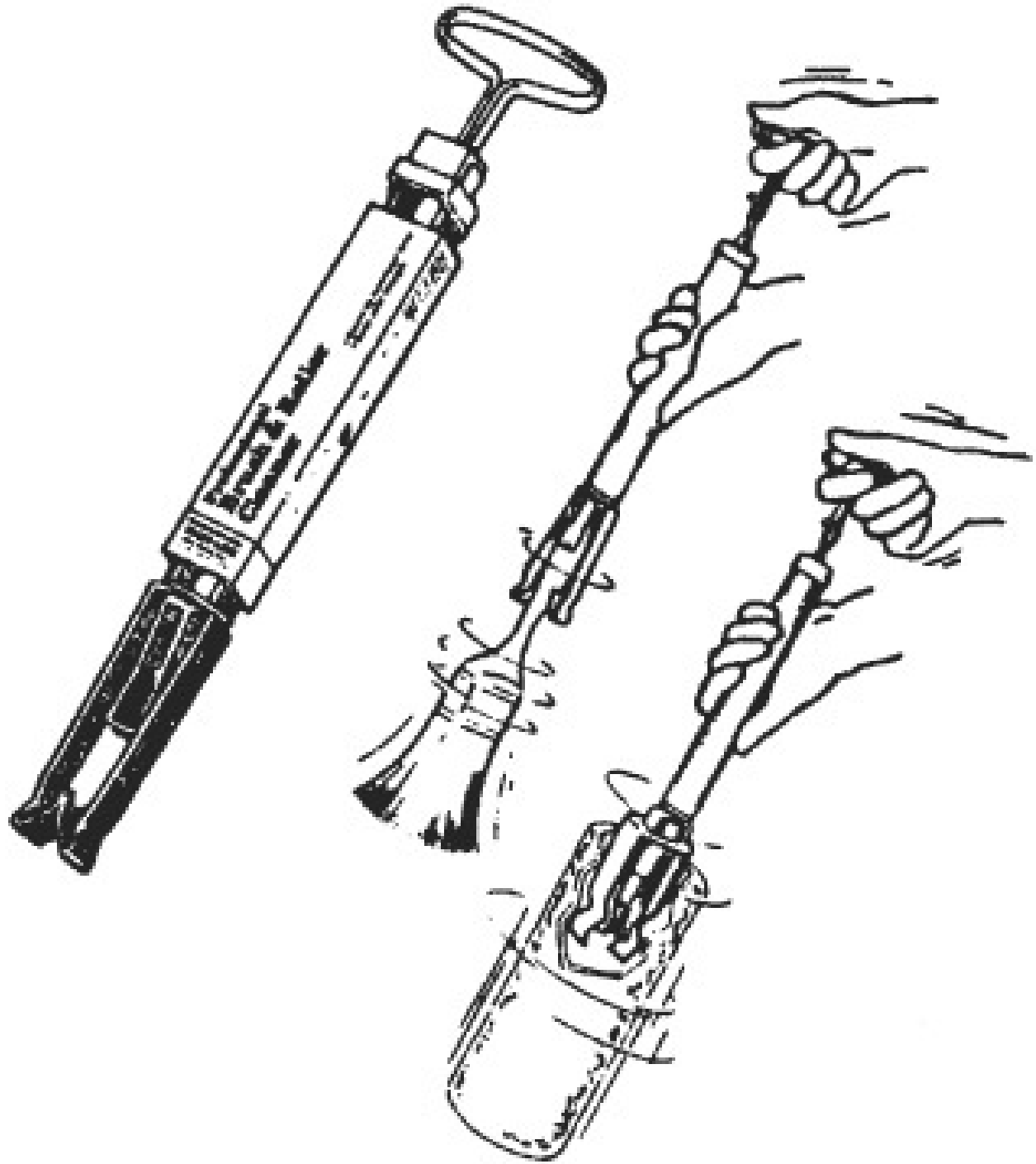
FIGURE 16-5. Spinner for cleaning paintbrushes and rollers.
