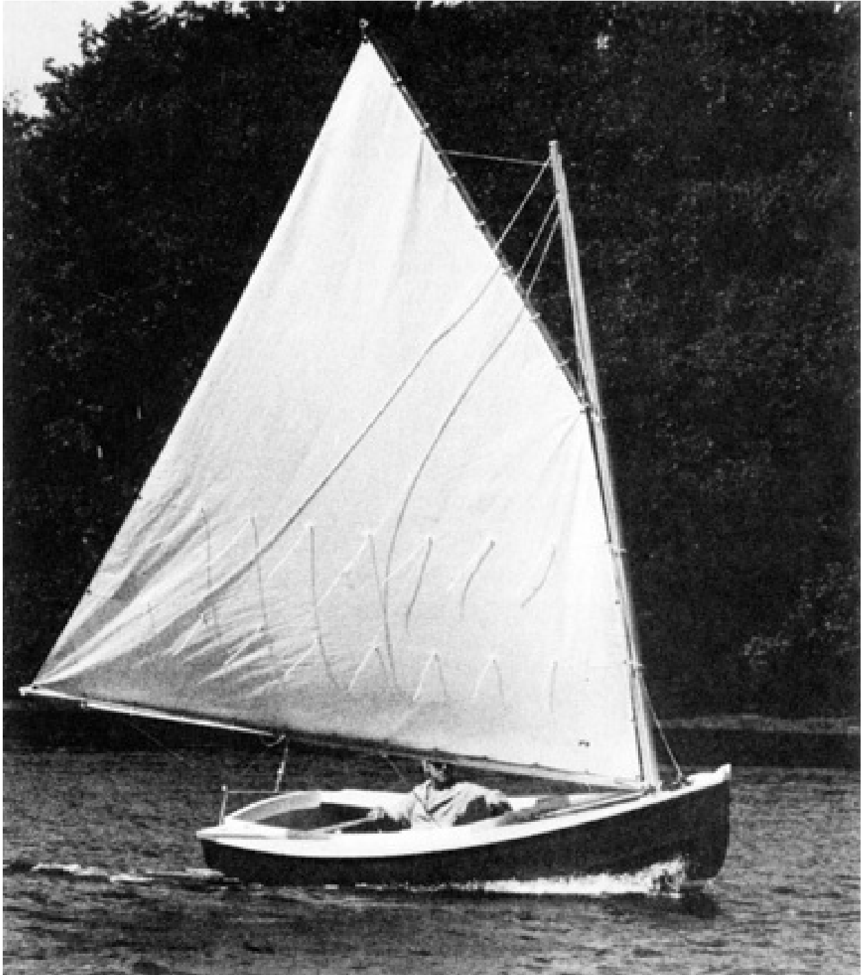
FIGURE 11-38. Another Bolger/Payson tack-and-tape plywood hull, the 12' 3" Bobcat, built from eight panels of \frac{1}{4} \times 4' \times 8' plywood. Plans are available from Payson. ( Dynamite Payson )
