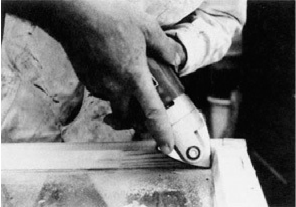
FIGURE 3-14A. An oscillating sander simplifies working in corners and on edges.
