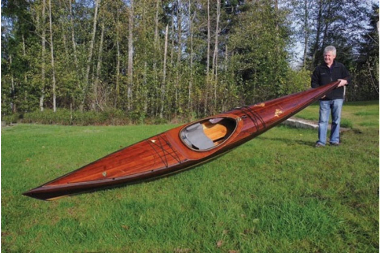
FIGURE 1-13. An 18' cedar strip-built King kayak from Redfish kayaks, which sells kits, like the one pictured, and finished kayaks. ( Redfish Kayaks )
