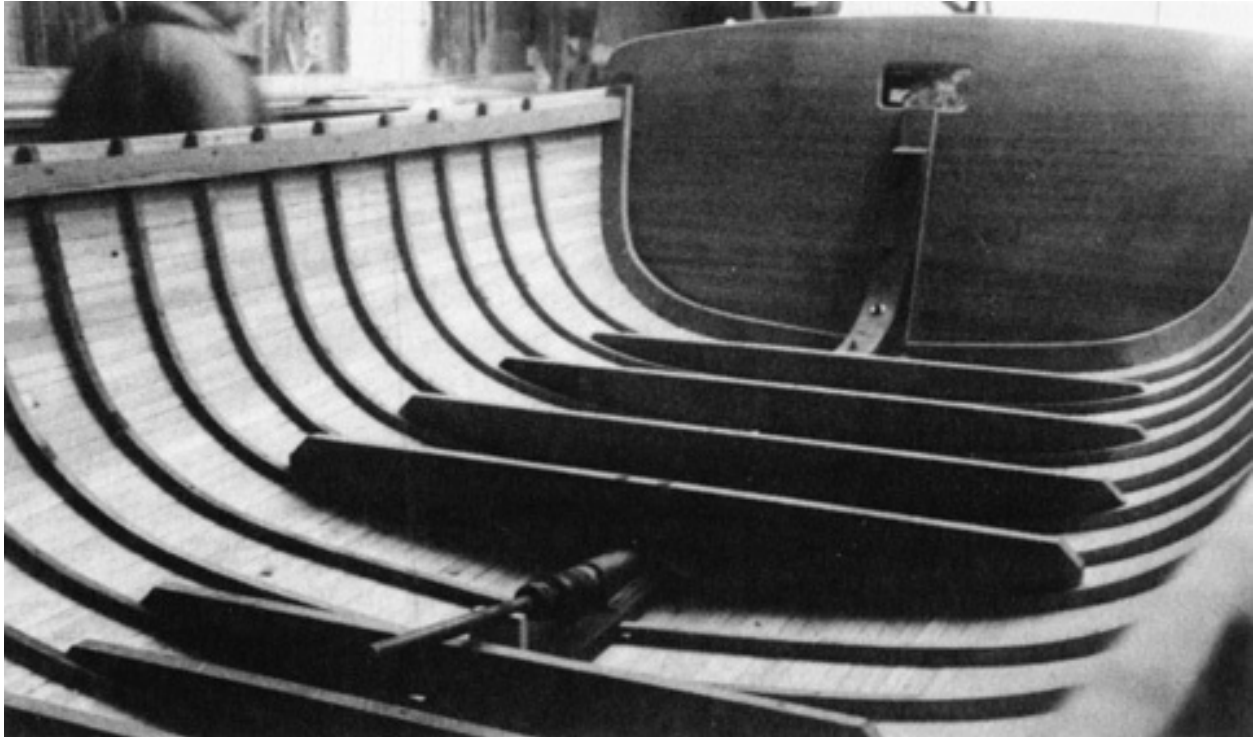
FIGURE 10-9. Floor timbers installed in a professionally built 18'7" utility launch, this one my Barbara Anne design.
