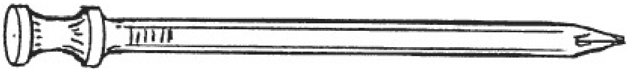
FIGURE 6-18. Two types of temporary fasteners: A bugle-head drywall screw (top) and a double-headed scaffold nail.
