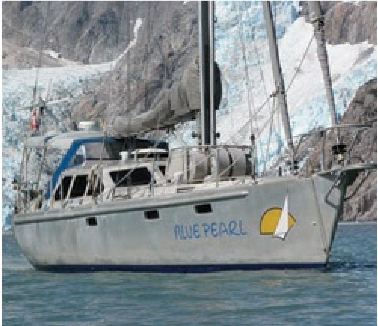
This Dix 43, built in aluminum, is shown at anchor in Antarctica. ( Franz Joho )
