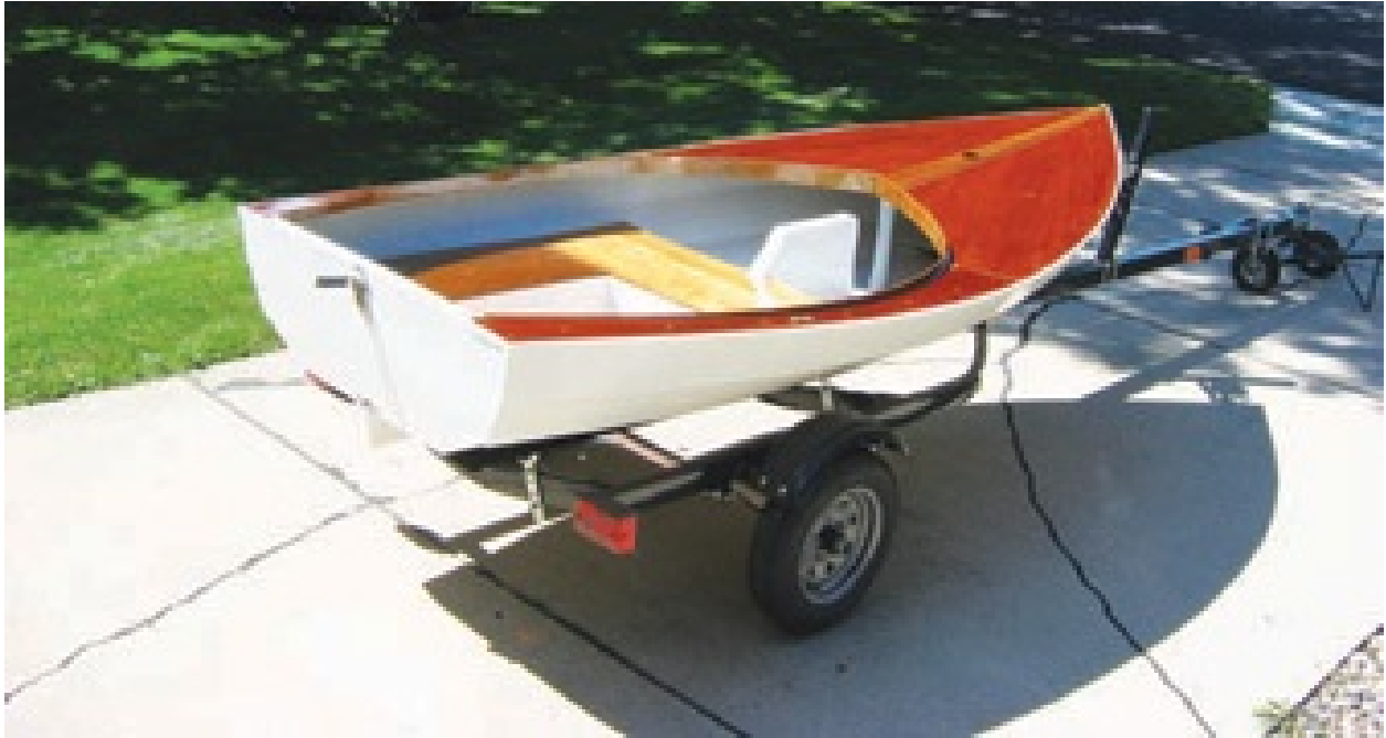
FIGURE 1-11. The Swiftly 11, a glued plywood lapstrake version of the Norwegian holmsbupram, is manufactured by Shell Boats. A sailing rig is available. ( Shell Boats )
