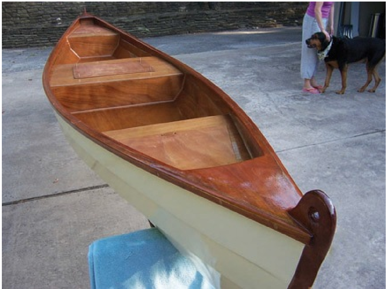
FIGURE 1-15. Arrowhead Custom Boats and Canoes makes the kit for this 16' glued lapstrake canoe they call The Flyfisher. ( Arrowhead Custom Boats and Canoes )
