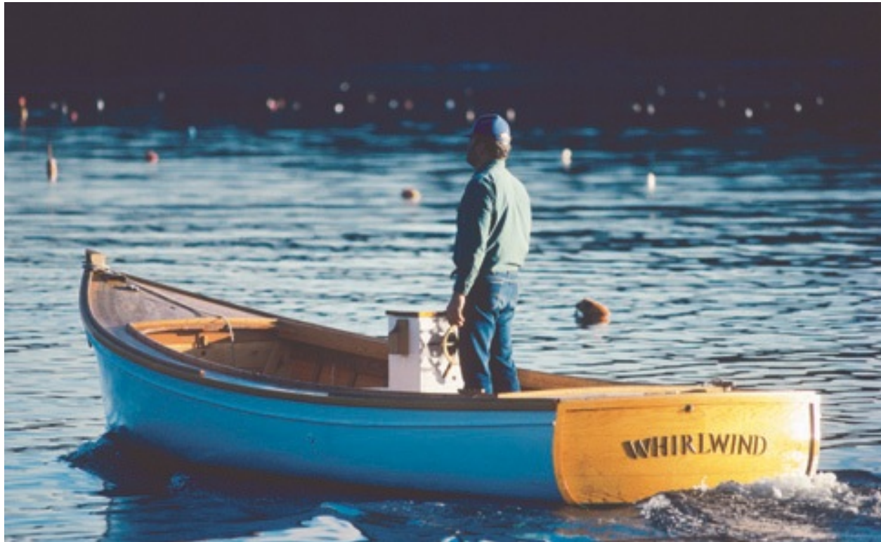
FIGURE 11-28. A 22-foot strip-planked Hampton utility launch. ( Peter Ralston photo courtesy Richard Pulsifer )
