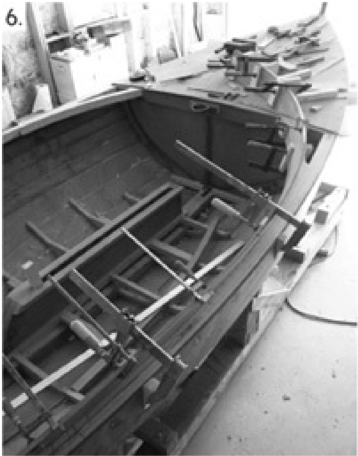
After the plywood foredeck is installed over the deck framing, temporary forms are fastened to the deck and the laminated coamings are glued up and dry-fit to
