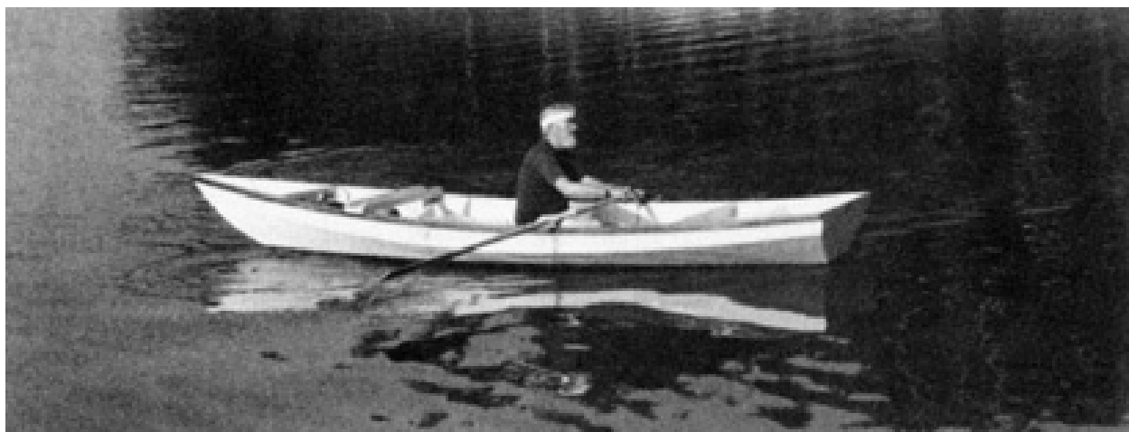
FIGURE 11-37. Gypsy, a 15-foot plywood Phil Bolger tack-and-tape design built by H. H. “Dynamite” Payson, from whom plans are available. ( Dynamite Payson )
