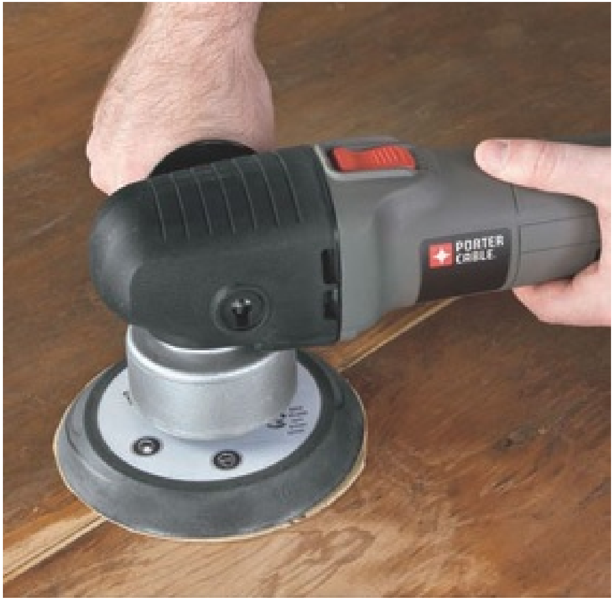
FIGURE 3-13B. The Porter-Cable 7345 random-orbit sander. ( Porter-Cable )
