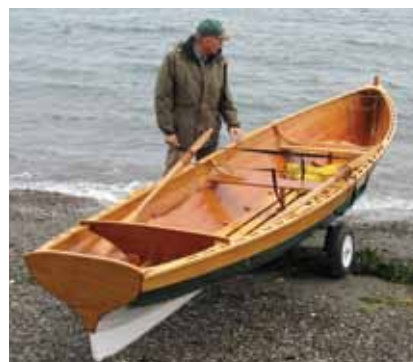
Acorn 17, on a jinker, easy one person launching! Note luxurious aft passenger seat. This one is set up for single or double (in line) rowers, with plenty of room for camping essentials.
